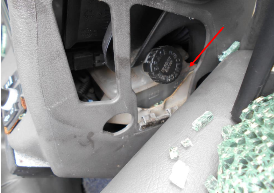
Photo 15 shows the brake fluid of the Motor Van at the time of our inspection. The fluid was observed to be of sufficient level and without any visible contamination.
