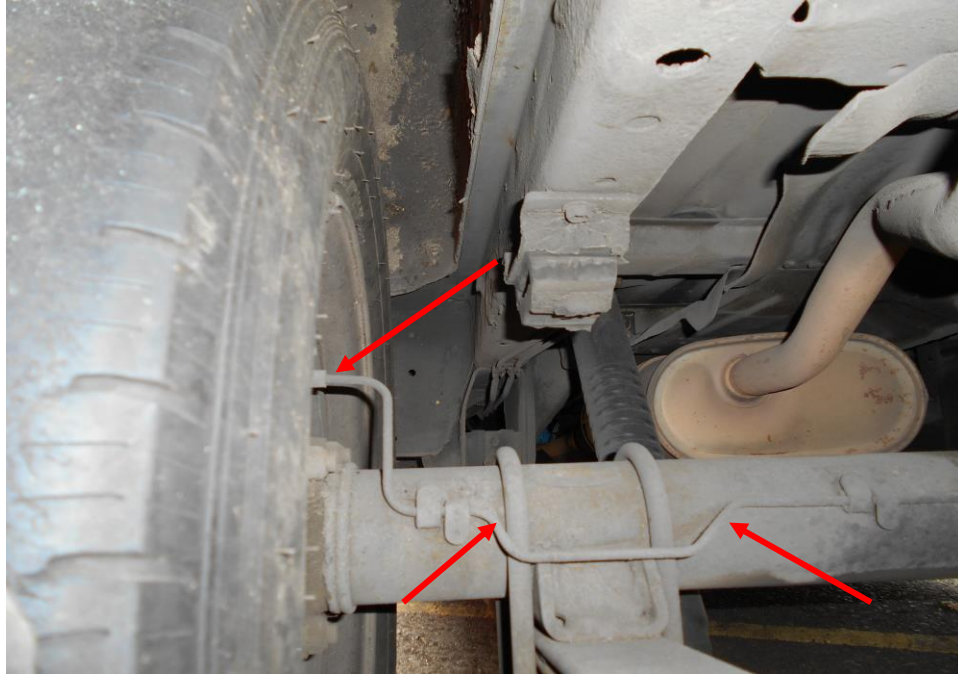
Photo 19 shows the various undercarriage components at the rear left wheels of the Motor Lorry. There was no sign(s) of brake fluid leakage along the brake hoses and brake pipes.
