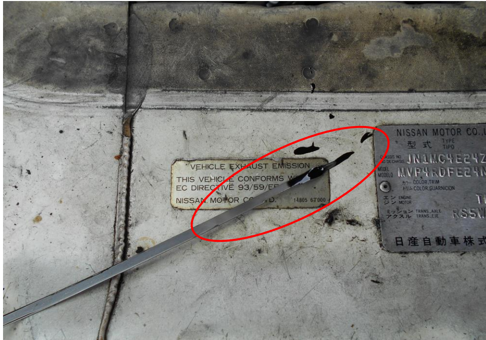
Photo 13 shows the engine dip stick of the Motor Van at the time of our inspection. The engine oil was observed to be of sufficient level and without any visible contamination (circled).
