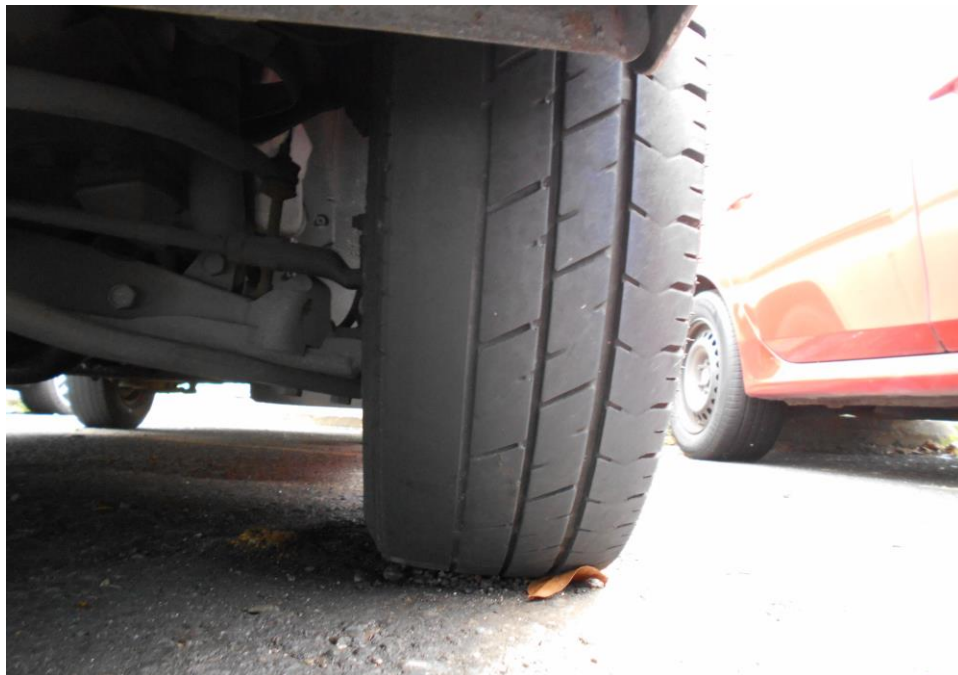
Photo 7 shows the condition of the front left tyre of the Motor Van, which was observed to be in serviceable condition with remaining tread depth of approximately 5mm. The tyre, which was wrapped around standard alloy wheel rim, was also observed to be sufficiently inflated for vehicular operation.
