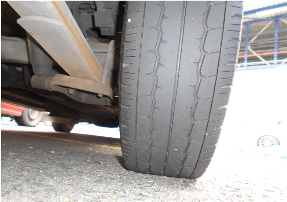
Photo 10 shows the condition of the rear right tyres of the Motor Van, which were observed to be in serviceable condition with remaining, tread depth of approximately 2mm.
