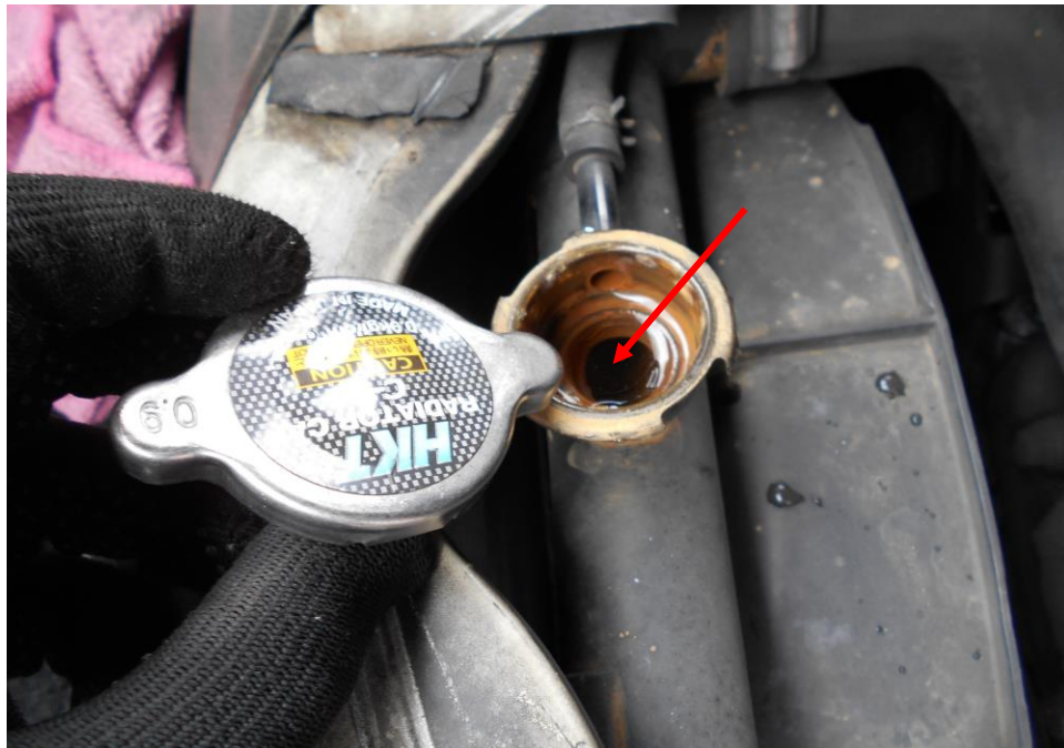
Photo 12 shows the engine coolant tank of the Motor Van at the time of our inspection. The engine coolant was observed to be of sufficient level and without any visible contamination (arrowed).
