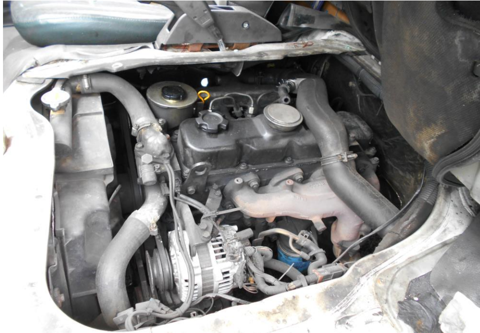
Photo 11 shows a general view of the Motor Van's engine compartment, which was accessed by lifting the front passenger seat of the Motor Van. The various parts and components inside the engine compartment were unaffected by the accident. There was also no sign(s) or indication(s) of fresh fluid leakage and/or fluid stain within the engine.
