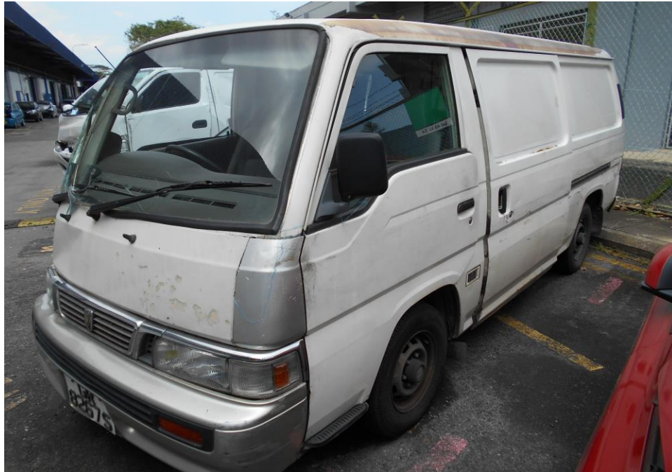
Photo 5 shows a general view of the front left portion of the Motor Van at the time of our inspection. The Motor Van was observed to be in good condition unaffected by the accident's impact.
