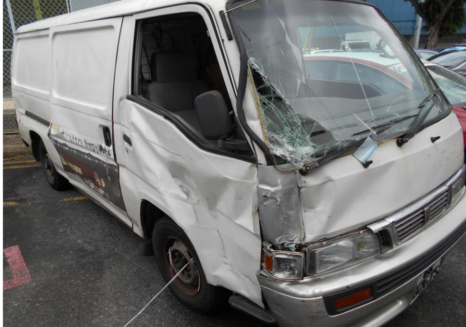
Photo 3 shows a damaged headlamp, centre panel, windshield, right sliding door and right door likely due to the accident's impact.
