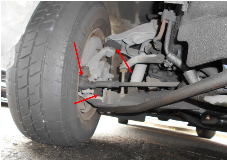
Photo 17 shows the various undercarriage components at the front right wheel of the Motor Van, in particular the steering tie rod end (arrowed). The various undercarriage components of the Motor Van were all found to be intact without any visible damage. There was also no sign of fluid stain(s) observed on the various undercarriage components.
