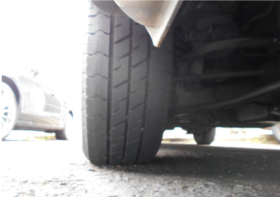
Photo 8 shows the condition of the front right tyre of the Motor Van, which was observed to be in serviceable condition with remaining tread depth of approximately 5mm. The tyre, which was wrapped around standard alloy wheel rim, was also observed to be sufficiently inflated for vehicular operation.
