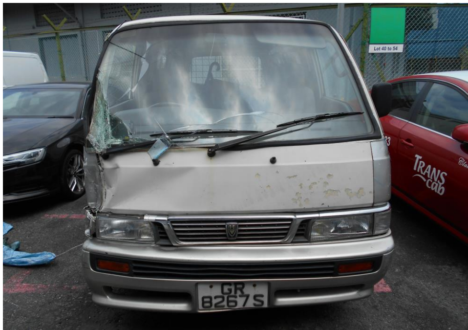
Photo 2 shows a general view of the front portion of the Motor Van at the time of our inspection. The Motor Van was observed to have sustained extensive damages at its front right headlamp; front right lower bumper and its right driver door were amongst the body parts that were damaged as a result of the accident.
