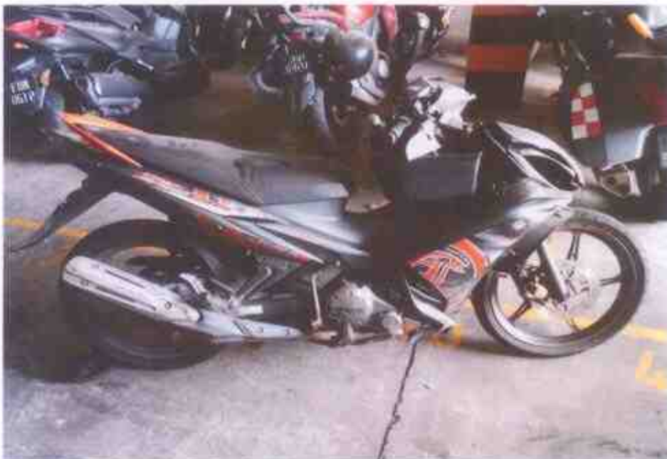
Photo 11 shows a general view of the right portion of the Motorcycle at the time of our inspection. The Motorcycle was observed to have sustained relatively extensive impact including damages to the steering system as a result of the accident collision.
