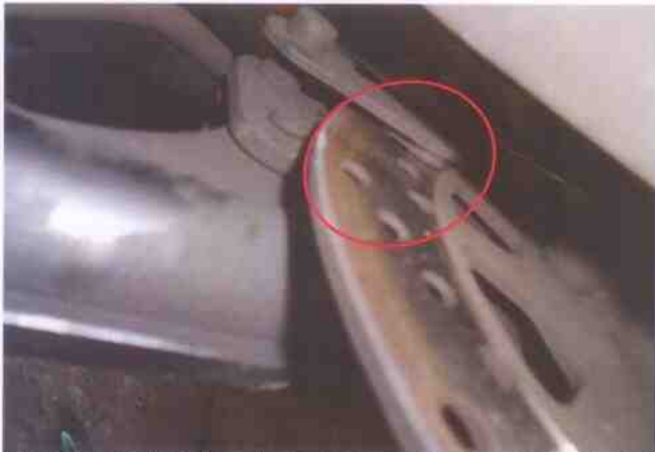
Photo 26 shows the brake pad was noted to be with sufficient frictional material at time of our inspection.
