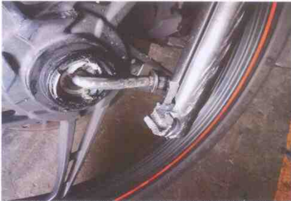
Photo 8 shows a close-up view of the front fork of the Motorcycle front wheel at the time of our inspection. It was observed to be damaged due to the accident collision.
