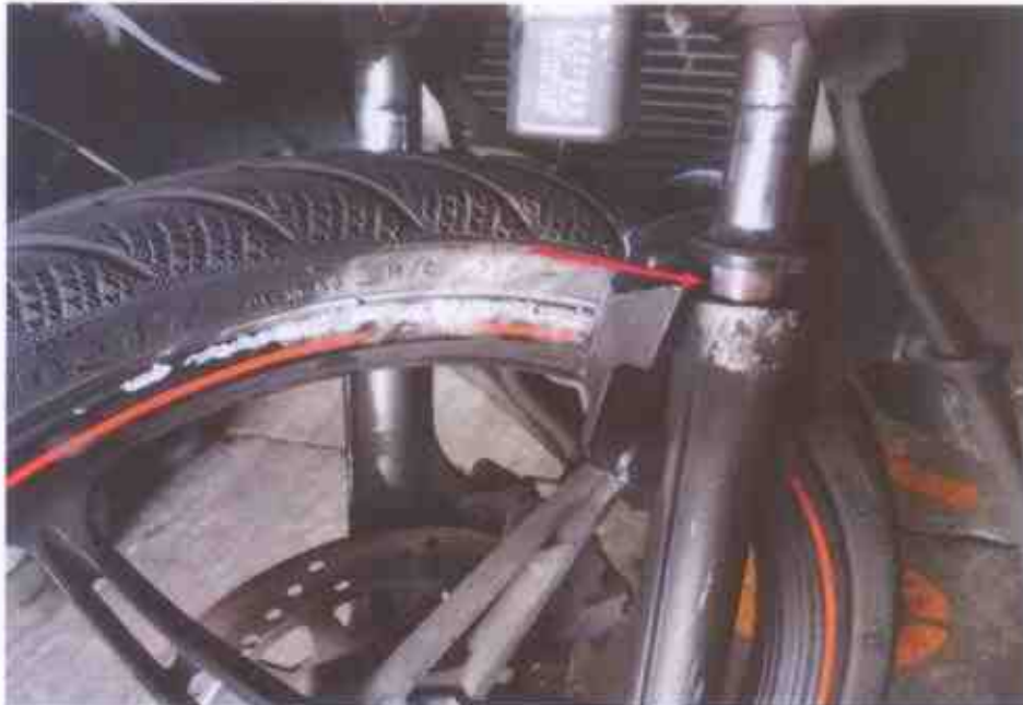
Photo 20 shows the front fork (arrowed) was observed to be damaged as a result of the accident.
