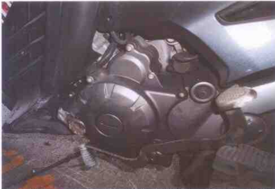
Photo 16 shows no sign(s) or indication(s) of fluid leakage observed around the engine's area of the Motorcycle.
