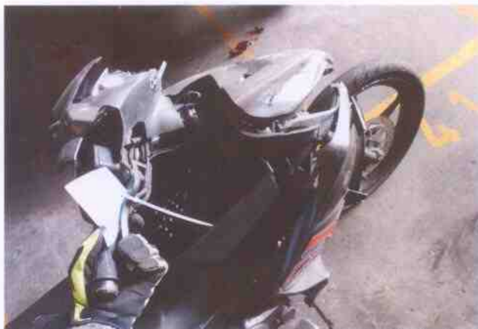
Photo 25 shows the static test conducted to the front hand brake. It was observed to be in serviceable condition unaffected by the accident's impact.
