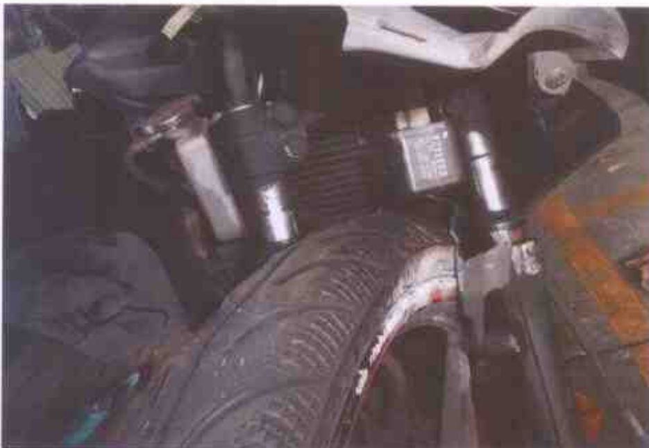
Photo 5 shows a close-up view of the front fork of the Motorcycle at the time of our inspection. It was observed to be damaged due to the accident collision.
