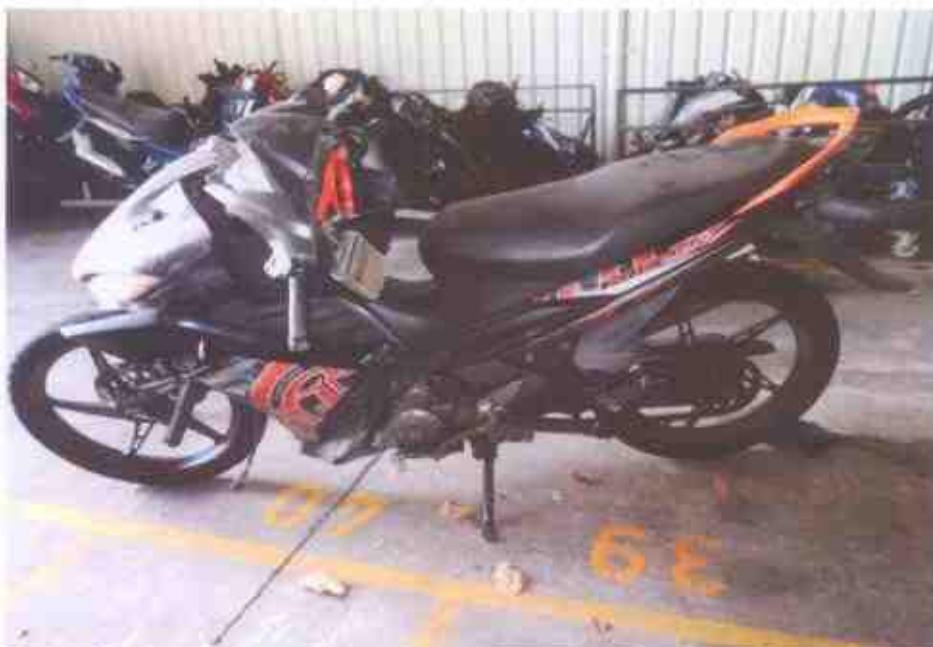
Photo 12 shows a general view of the right portion of the Motorcycle at the time of our inspection. The Motorcycle was observed to have sustained relatively extensive impact including damages to the steering system as a result of the accident collision.
