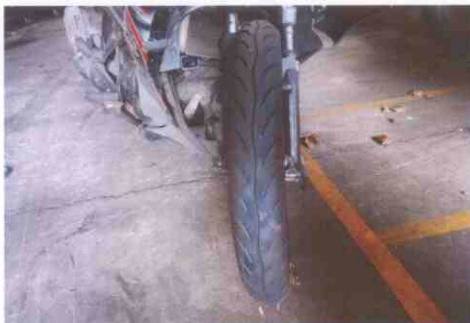
Photo 14 shows the front tyre of the Motorcycle at the time of our inspection. The pattern of the tread was clearly visible with remaining tread depth of approximately 3mm. There was no tear, burst mark(s) and/or punctured hole(s) on the sidewalls as well as across the tread of the front tyre.
