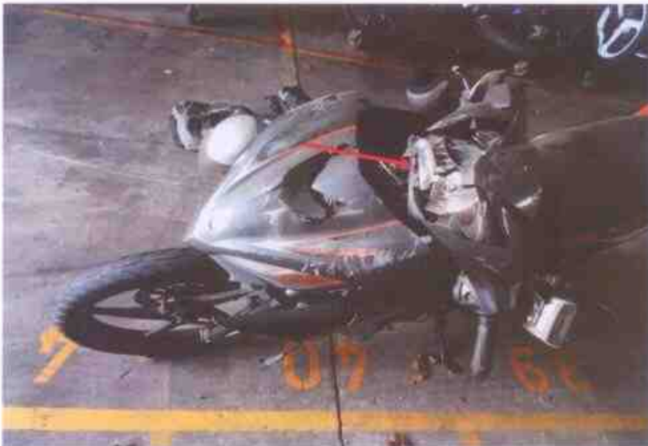
Photo 21 shows the handle bar (arrowed) was observed to be dislodged from the original installation as a result of the accident.
