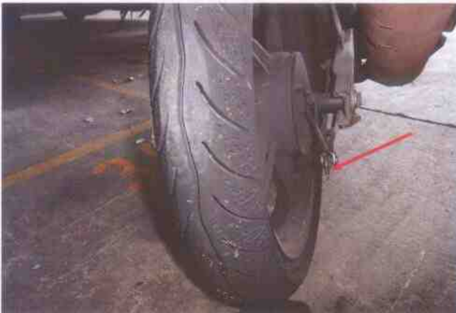
Photo 23 shows the rear foot brake pedal components (arrowed) was observed to be in serviceable condition unaffected by the accident's impact collision.
