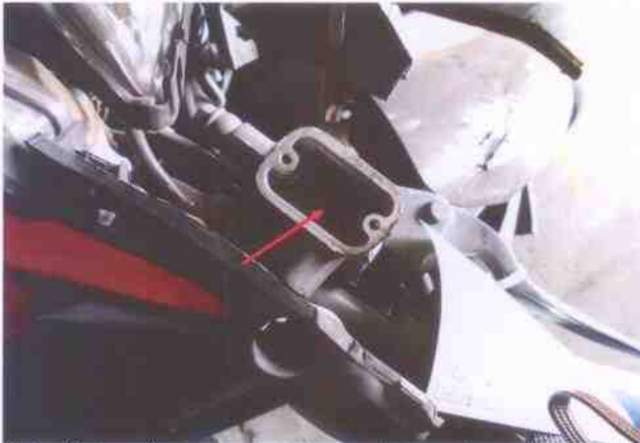
Photo 22 shows the front brake fluid reservoir (arrowed) was observed to be unaffected by the accident. It was observed to be of sufficient level & not contaminated at the time of our inspection.
