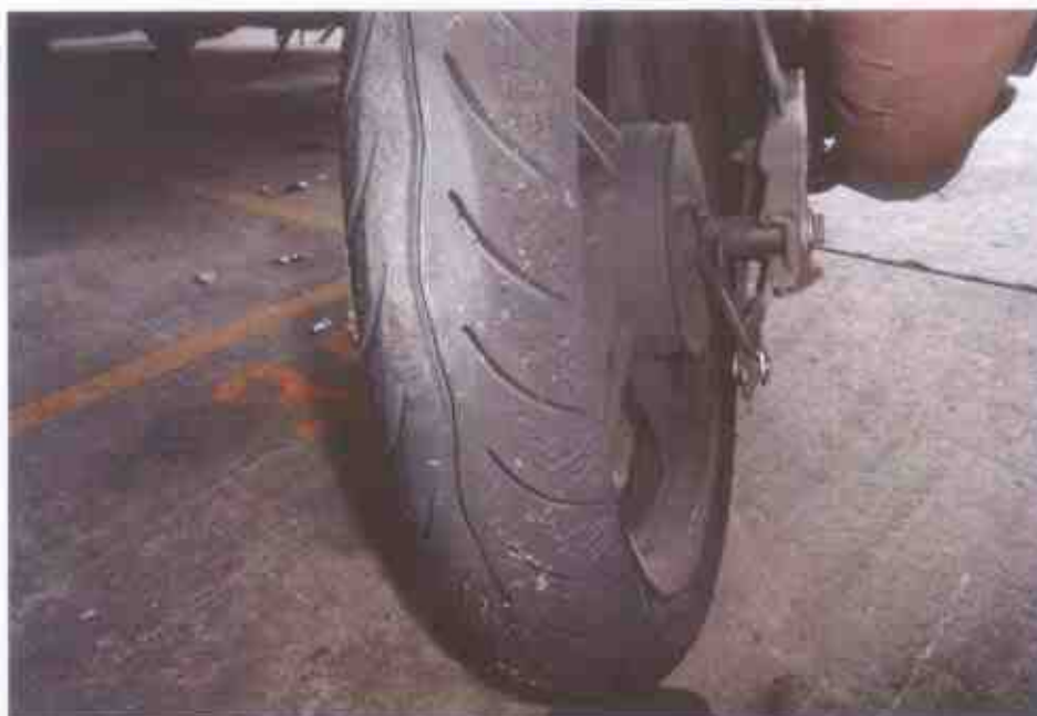
Photo 13 shows the rear tyre of the Motorcycle at the time of our inspection. The rear tyre was observed to be in serviceable condition with remaining tread depth of approximately 4mm. The tyre was also observed to be sufficiently inflated for vehicular operation. There was no significant damage observed on the rear wheel rim & tyre.
