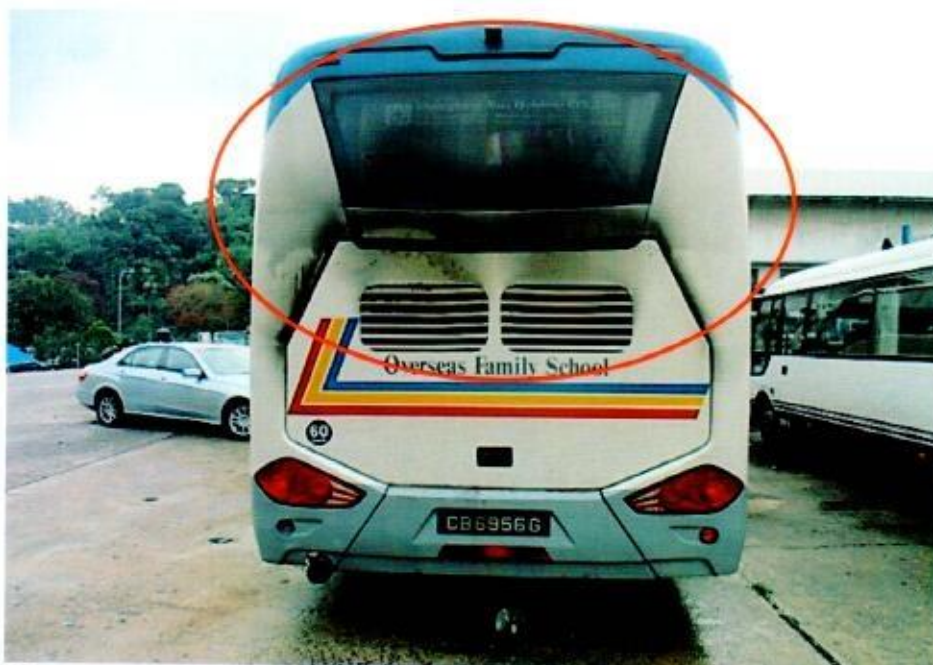
Photo 6 shows the general view of the rear portion of the Insured Vehicle at the time of our inspection. The Insured Vehicle had sustained fire damage at the rear portion. Affected parts had included the rear windscreen and engine panel, amongst others (circled).
