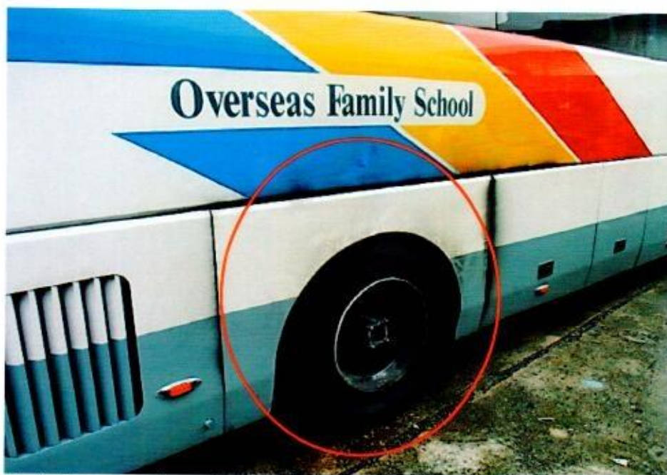
Photo 5 shows a closer view of the right portion of the Insured Vehicle at the time of our inspection. The fire damage to the Insured Vehicle was confined to its centre portion. Affected parts had included the right side panel, right rear wheel rim and right rear tyre, amongst others (circled).
