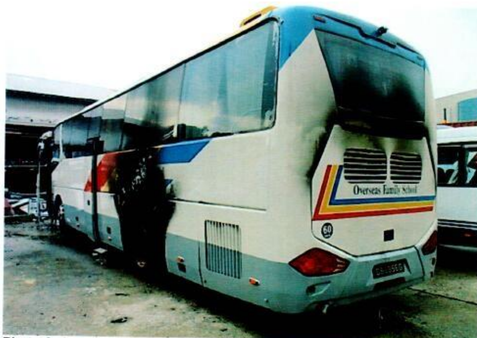
Photo 2 shows the general view of the rear left portion of the Insured Vehicle at the time of our inspection. The exterior body of the Insured Vehicle had sustained fire damage at the centre portion as well as rear portion. Affected parts had included the side panels, rear tyres, rear wheel rims, left glass panel, rear windscreen and engine panel, amongst others.
