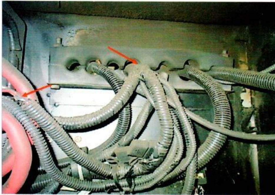
Photo 13 shows a close up view of the several burnt stretches of original factory fitted wirings leading from the battery (arrowed).
