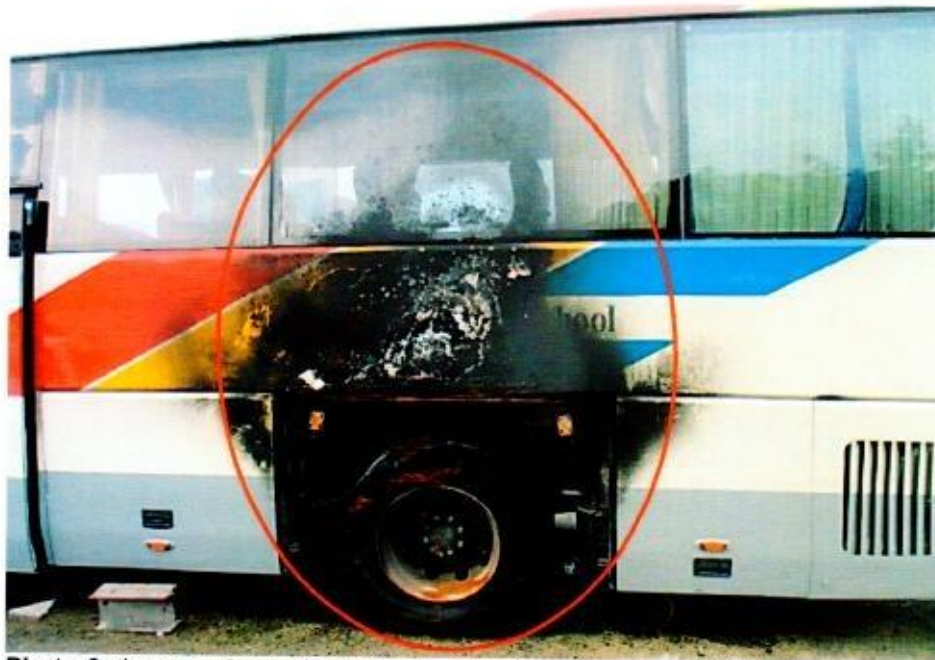
Photo 3 shows a closer view of the left portion of the Insured Vehicle at the time of our inspection. The fire damage was observed to be most severe at its left centre portion. Affected parts had included the left side panel, left rear wheel rim, left rear tyre and left glass panel, amongst others (circled).
