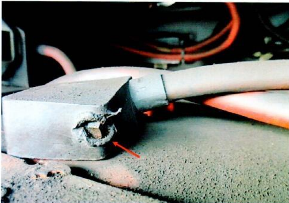
Photo 14 shows a close up view of the several burnt stretches of original factory fitted wirings leading from the battery (arrowed).
