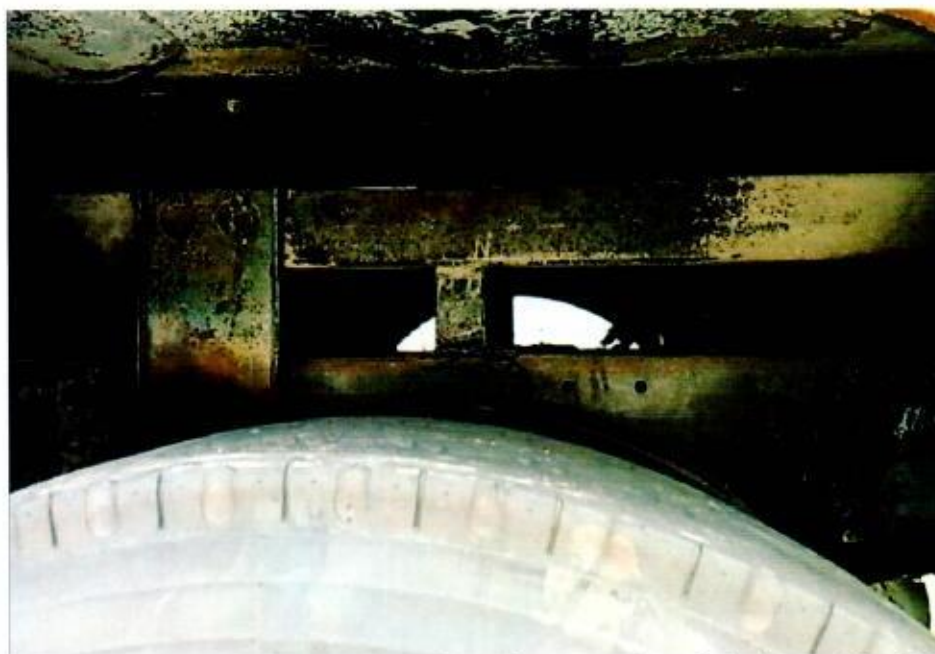
Photo 19 shows a close up view of the left rear portion of the Insured Vehicle post- incident. In general, the extensive damages sustained to this portion of the Insured Vehicle had corresponded to the events that were related to us by Mr Kwek, which is the fire had started from the left rear portion of the Insured Vehicle.
