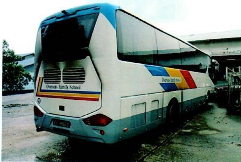
Photo 4 shows the general view of the right rear portion of the Insured Vehicle at the time of our inspection. The exterior body of the Insured Vehicle had sustained fire damage at the centre portion as well as rear portion. Affected parts had included the side panels, rear tyres, rear wheel rim, rear windscreen and engine panel, amongst others.
