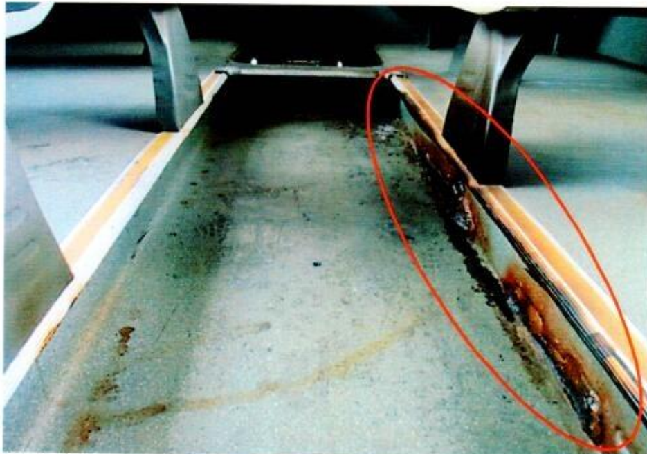
Photo 10 shows a closer view of the floorboard towards the rear portion of the rear cabin of the Insured Vehicle which was found to be partially burnt and/or melted as a result of the fire (circled).
