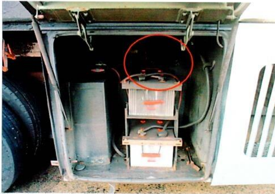
Photo 11 shows a view of the left rear portion of the Insured Vehicle, near to the vicinity where the battery is located. We had found several burnt stretches of original factory fitted wirings leading from the battery (circled).
