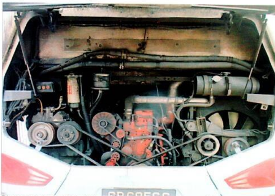
Photo 8 shows a general view of the engine compartment of the Insured Vehicle at the time of our inspection. The engine compartment of the Insured Vehicle was significantly affected by the fire. Most of the parts inside the engine compartment were found to be partially burnt and/or melted as a result of the fire.
