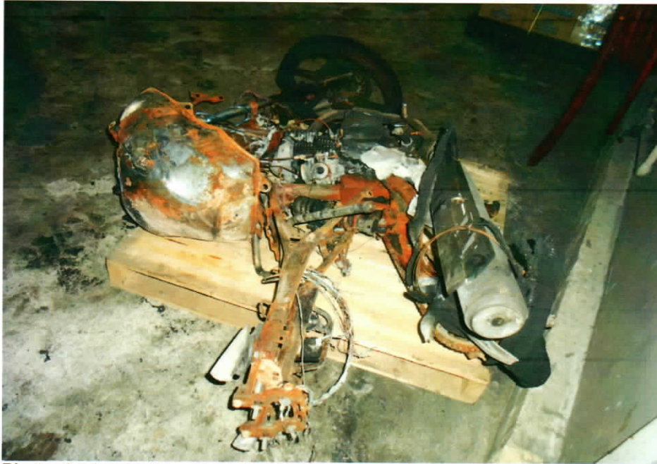
Photo 3 shows the rear left side of the Insured Vehicle at the time of our inspection. The Insured Vehicle was noted to have sustained fire damages that severely effected on the entire parts of the Insured Vehicle.
