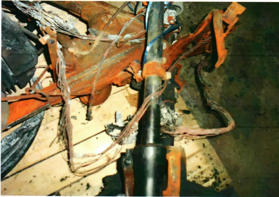
Photo 6 shows the front portion of the Insured Vehicle at the time of our inspection. Several stretches of wiring burnt internally to its bare copper state.
