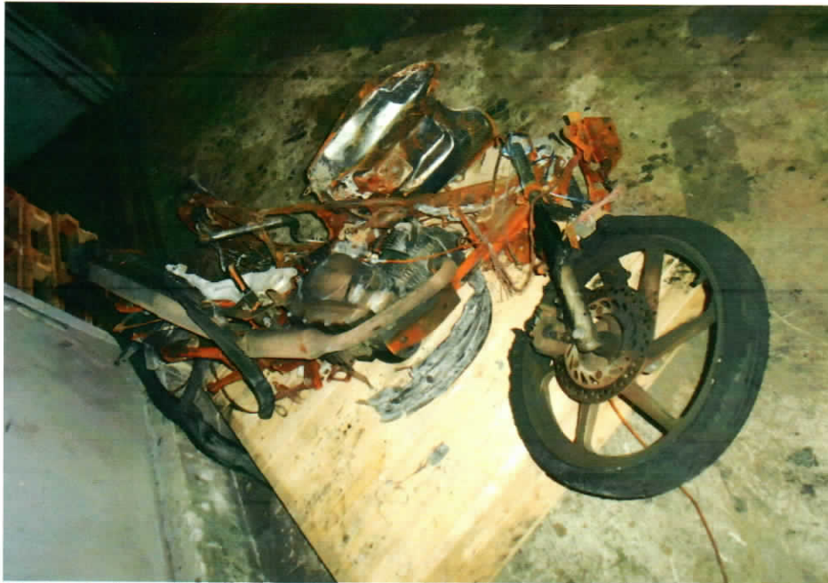
Photo 1 shows the right portion view of the Insured Vehicle at the time of our inspection. The Insured Vehicle was noted to have sustained fire damages that severely effected on the entire parts of the Insured Vehicle.
