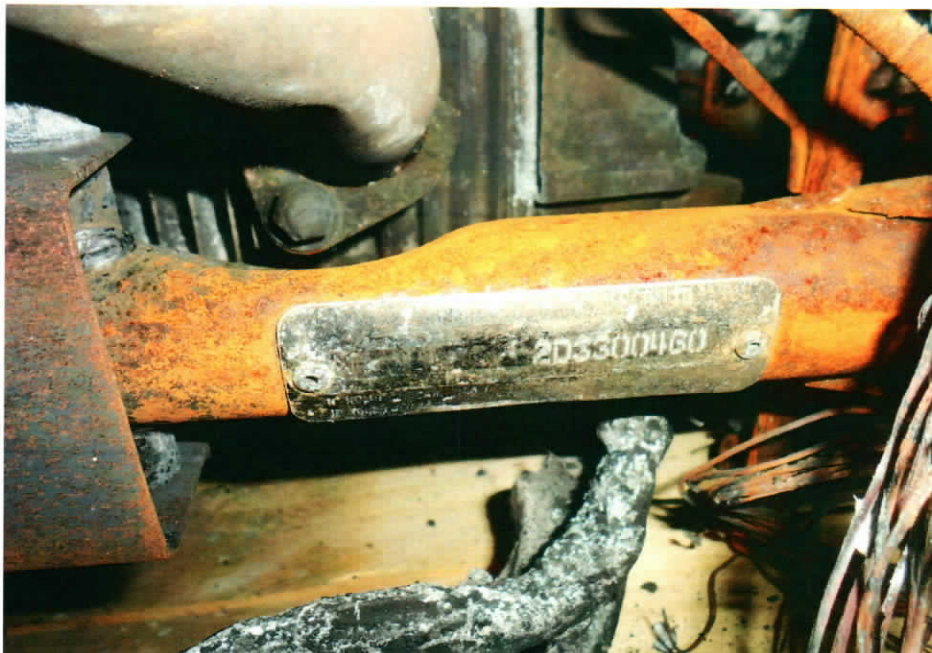
Photo 4 shows the chassis number plate that was still intact despite of the severe burnt on the entire Motor cycle.
