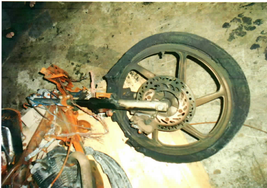
Photo 2 shows the frontal portion view of the Insured Vehicle at the time of our inspection. The Insured Vehicle was noted to have sustained fire damages that severely effected on the entire parts of the Insured Vehicle.
