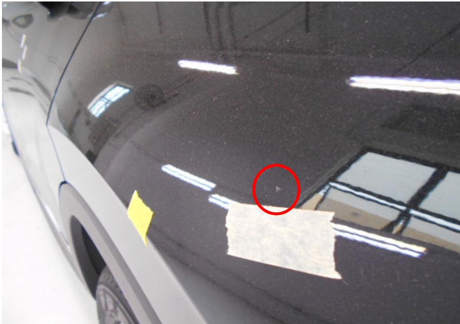
Photo 24 shows a close-up view of the scratch mark (circled) that was found on the rear left fender. Similar type of scratch marks was also found on the front left fender, rear left door, rear tailgate and rear right door of this unregistered Tiguan model Volkswagen motor car.
