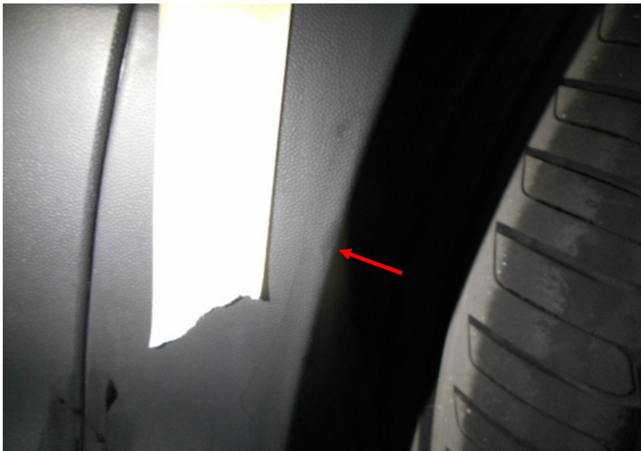
Photo 13 shows a close-up view of the relatively minor cut mark that was observed on the right side rear fender protector pad.
