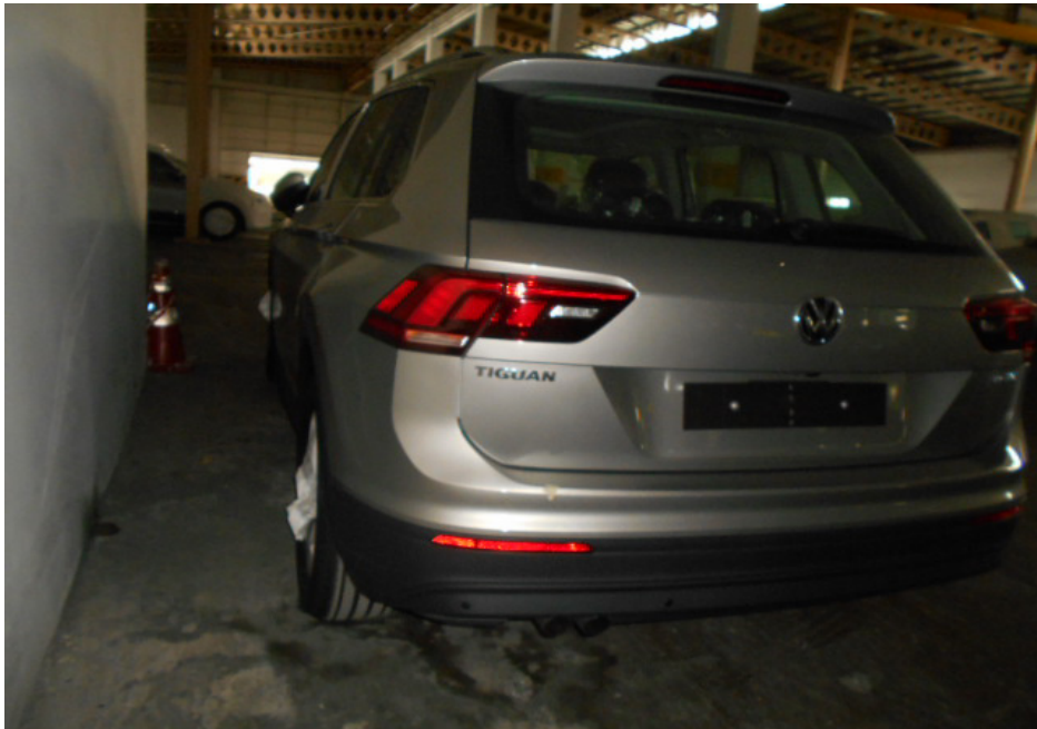
Photo 16 shows a general view of the rear body of the second unregistered Tiguan model Volkswagen motor car that was affected by the Incident. For this chassis number, the rear bumper, rear bumper lower spoiler and rear right taillamp were damaged.
