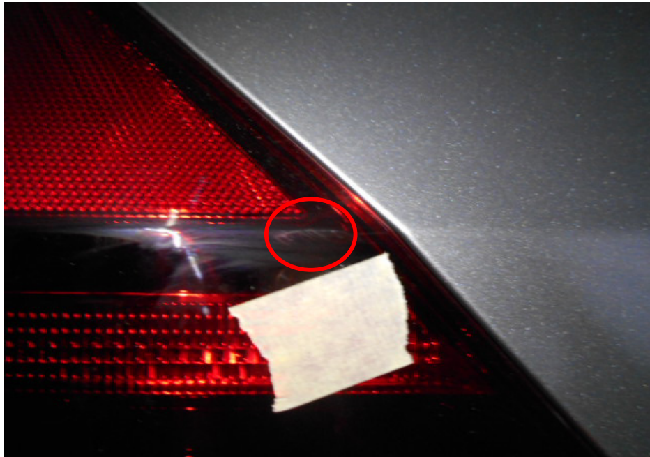
Photo 20 shows a close-up view of the scratch mark (circled) that was observed on the rear right taillamp cover.
