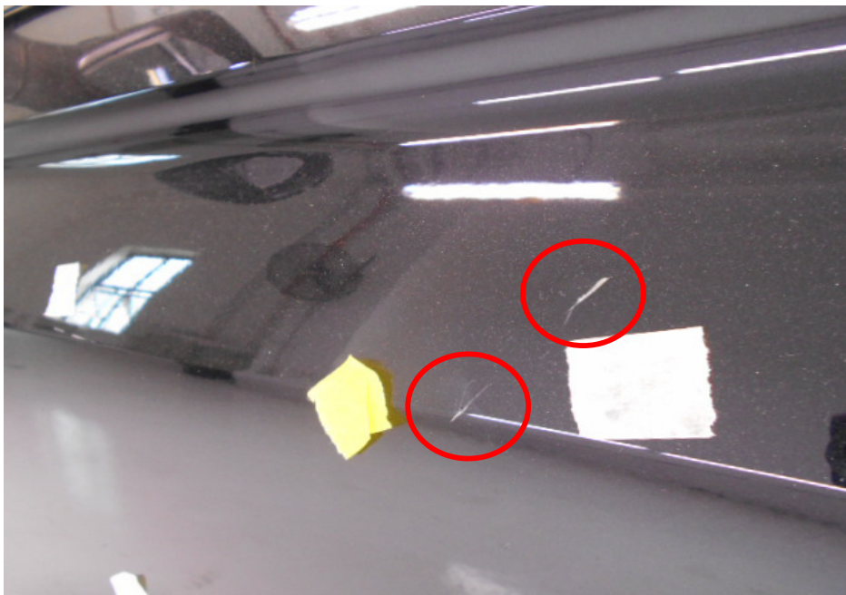
Photo 23 shows a close-up view of the scratch marks (circled) that were found on the front left door. Similar type of scratch marks was also found on the front left fender, rear left door and rear tailgate of this unregistered Tiguan model Volkswagen motor car.
