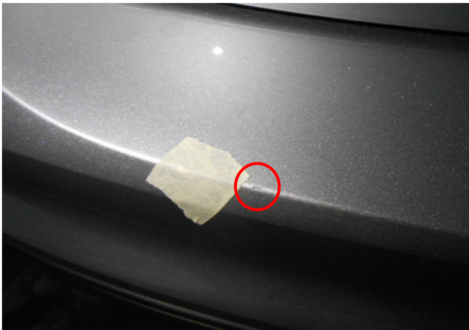
Photo 17 shows a close-up view of one of the cut marks (circled) that was observed on the rear bumper.
