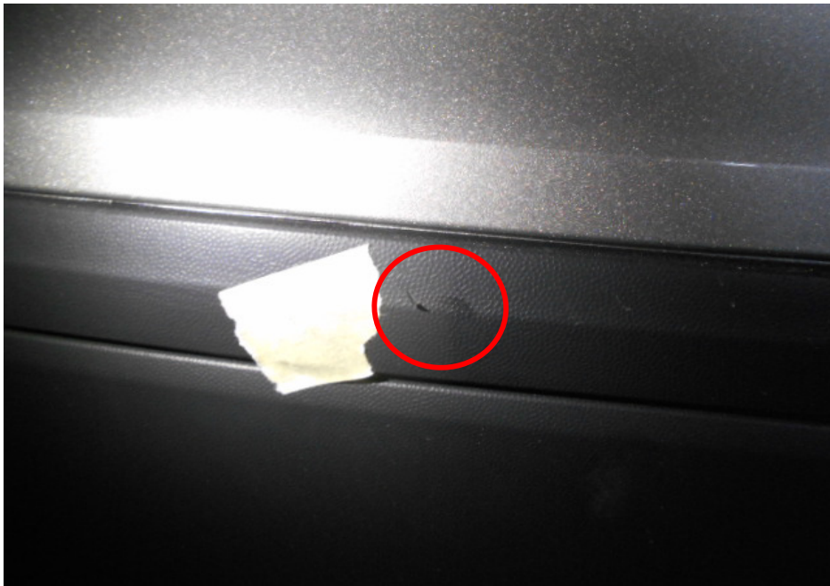
Photo 19 shows a close-up view of the cut mark (circled) that was observed on the rear bumper lower spoiler.
