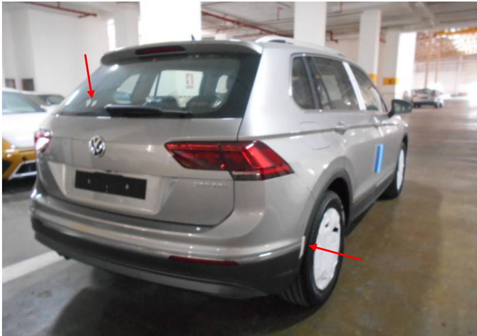
Photo 12 shows a general view of the rear right body of the first unregistered Tiguan model Volkswagen motor car that was affected by the Incident. The rear fender right protector pad and rear windscreen were found to be damaged at the area indicated by the red arrows.
