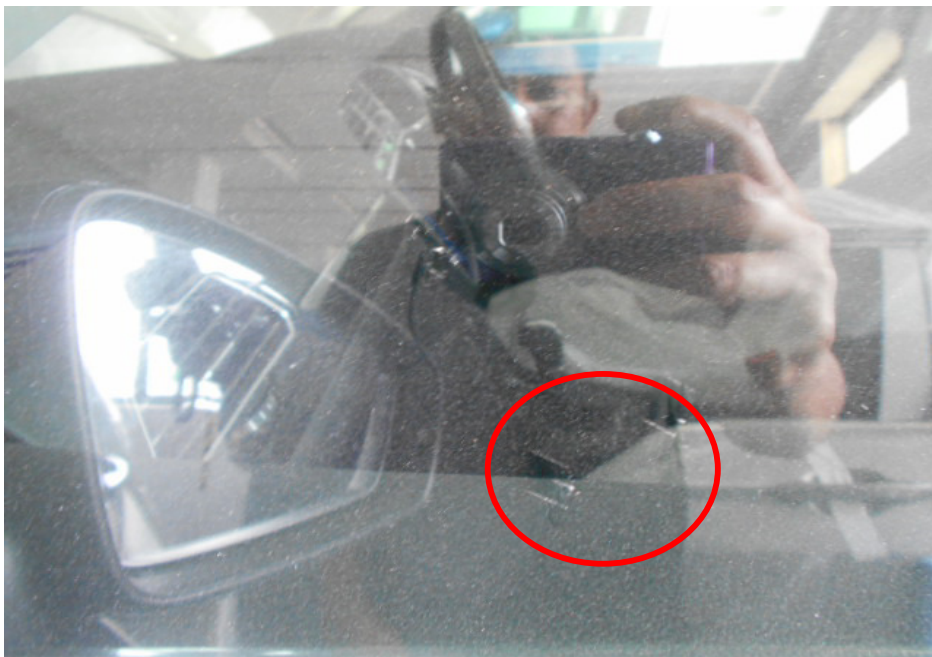
Photo 25 shows the relatively small chip marks (circled) that were found on the front left door window. Similar type of marks was also found on the rear windscreen of this unregistered Tiguan model Volkswagen motor car.
