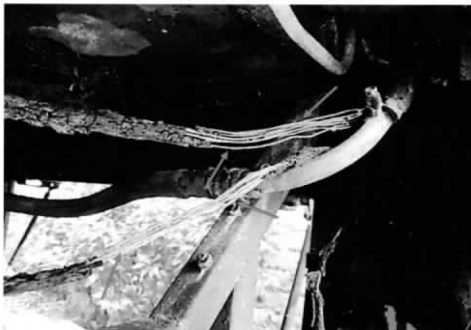
Photo 9 shows a closer view of the greenish residue that was found on several burnt stretches of original factory fitted wirings around the rear right portion of the engine compartment (arrowed) of the Insured Vehicle.
