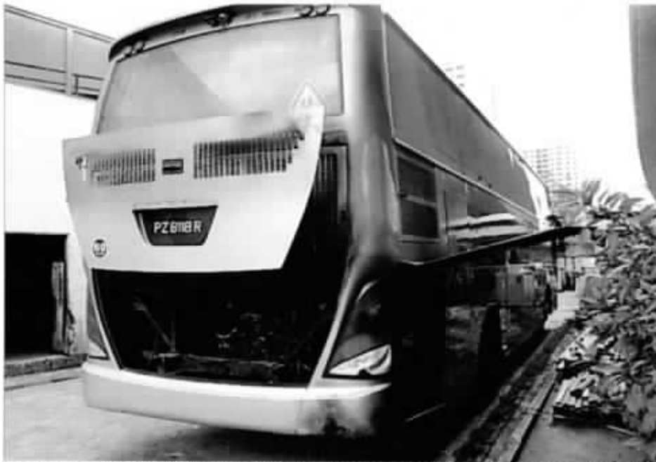
Photo 3 shows the general view of the right rear portion of the Insured Vehicle at the time of our inspection. The exterior body of the Insured Vehicle had sustained significant fire damage at the rear right portion.
