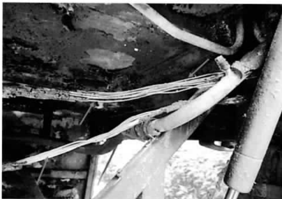
Photo 10 shows a close up view of the greenish residue that was found on several burnt stretches of original factory fitted wirings around the rear right portion of the engine compartment (arrowed) of the Insured Vehicle.
