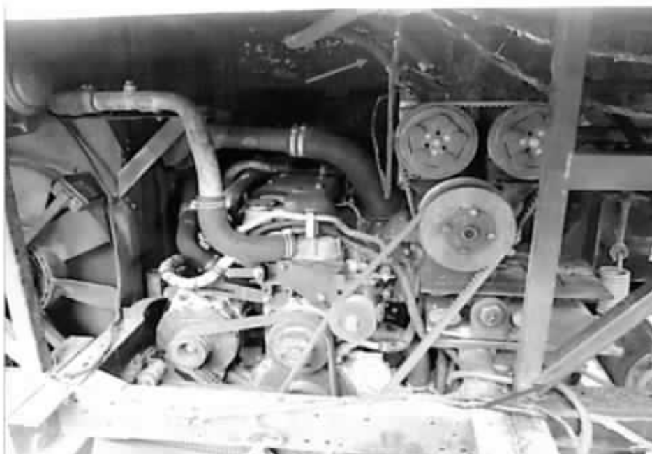
Photo 7 shows a closer view of the burnt engine compartment of the Insured Vehicle. The fire damage was more extensive at the rear right portion (arrowed). The rear left portion had sustained minimal fire damage.
