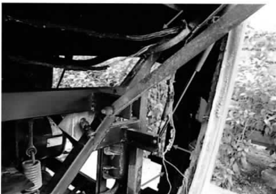
Photo 8 shows a view of the greenish residue found on several burnt stretches of original factory fitted wirings around the rear right portion of the engine compartment (arrowed) of the Insured Vehicle.
