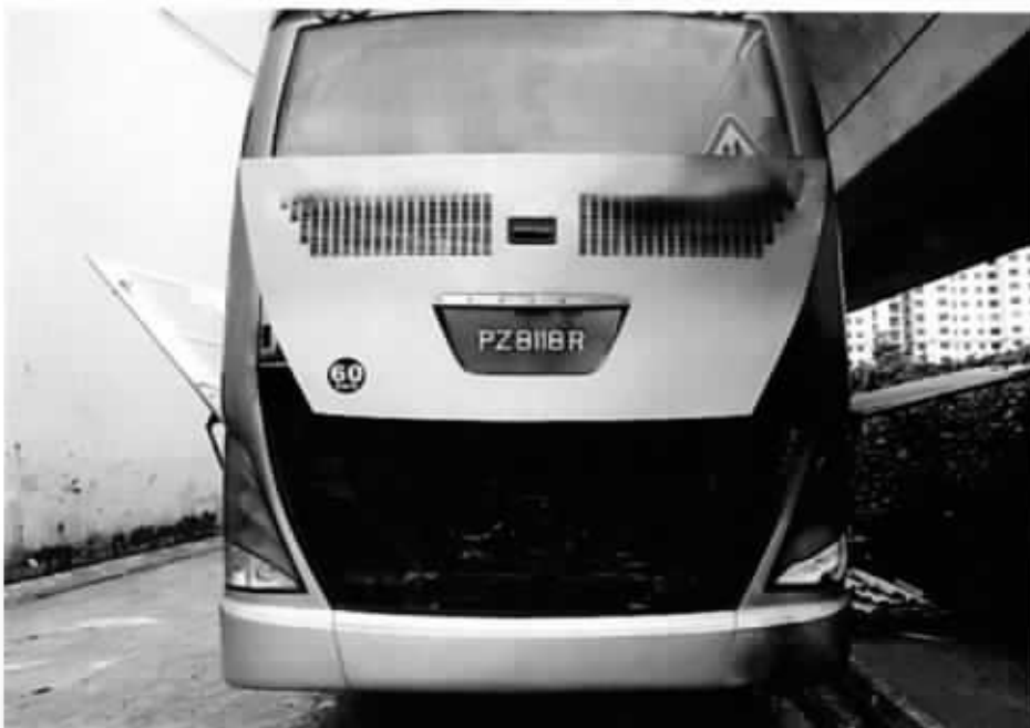
Photo 4 shows the general view of the rear portion of the Insured Vehicle at the time of our inspection. The Insured Vehicle had sustained fire damage at the rear portion. Affected parts had included the rear windscreen, engine panel, side panels, tail lights and rear bumper, amongst others.
