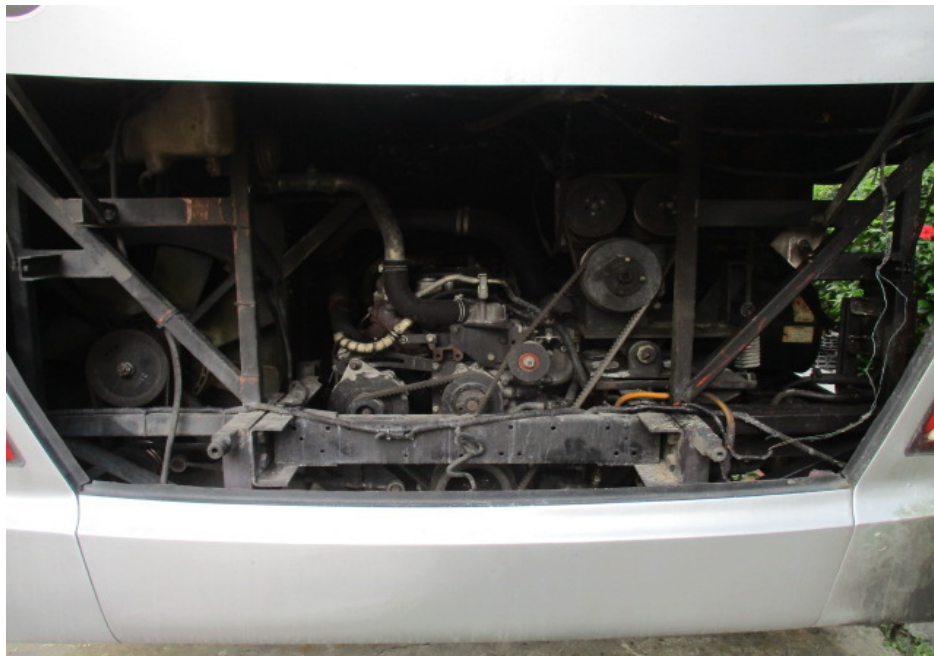
Photo 6 shows a general view of the engine compartment of the Insured Vehicle at the time of our inspection. The engine compartment of the Insured Vehicle was significantly affected by the fire. Most of the parts inside the engine compartment were found to be partially burnt and/or melted as a result of the fire.
