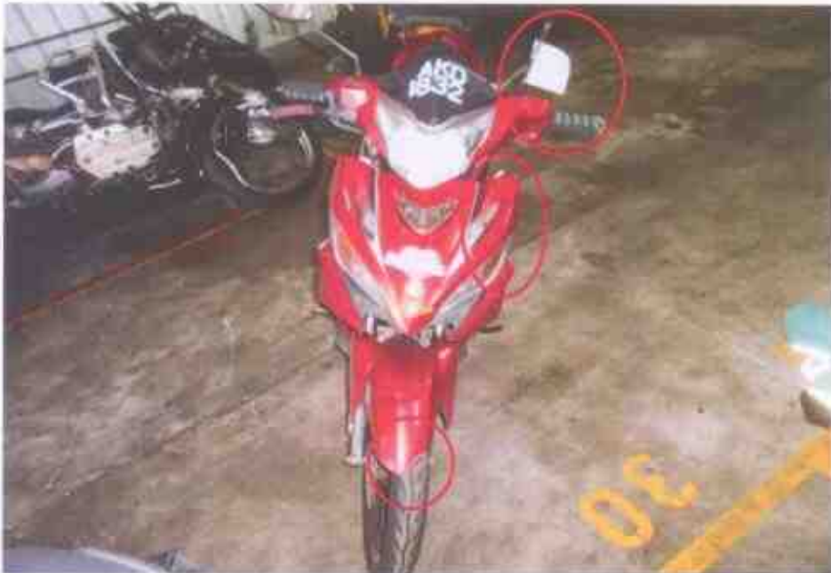
Photo 5 shows a general view of the front portion of the Motorcycle at the time of our inspection. The Motorcycle was observed to have sustained minor damages which include missing left wing mirror, slight bend handle bar, and bent foot rest amongst others as a result of the accident.
