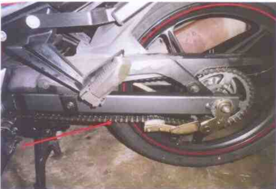
Photo 10 shows the general view of the gear train (arrowed) of the Motorcycle, which was observed to be intact with no misalignment. It was also adequately lubricated for operating purposes.
