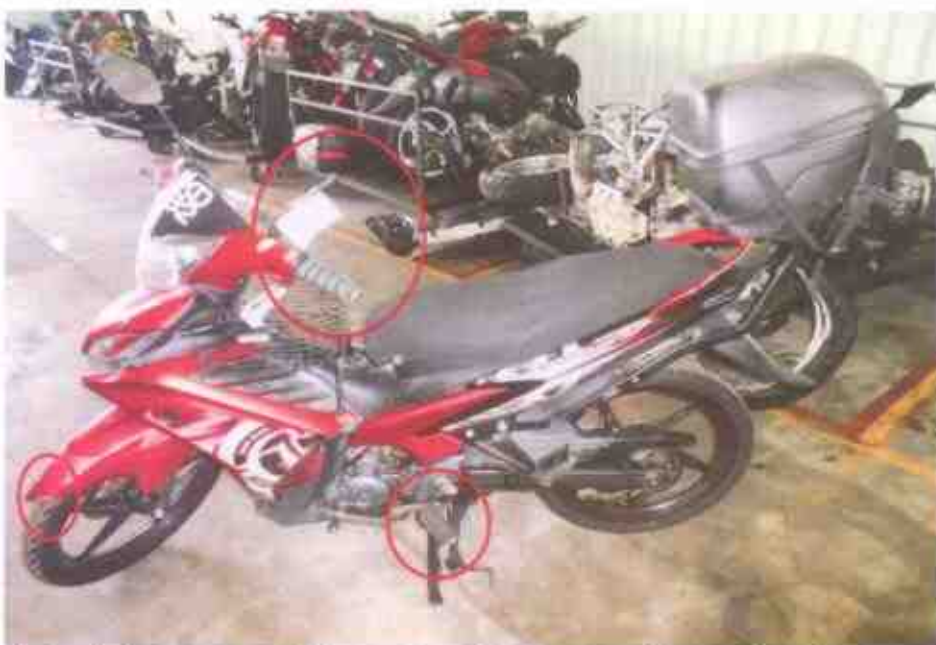
Photo 4 shows a general view of the left body of the Motorcycle at the time of our inspection. The Motorcycle was observed to have sustained minor damages which includes missing left wing mirror, slight bend handle bar, bent foot rest amongst others as a result of the accident.
