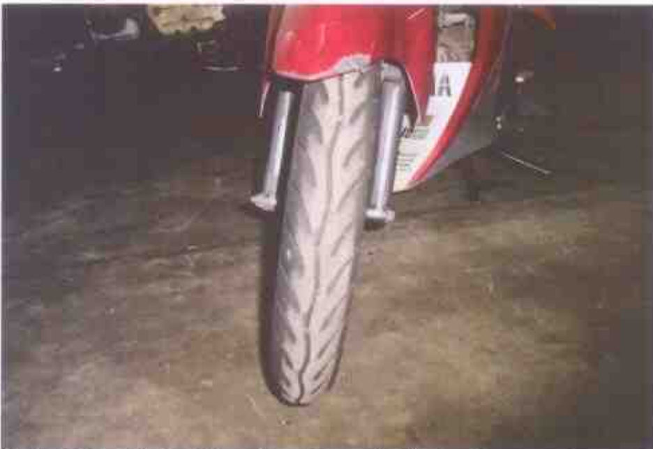
Photo 7 shows the front tyre of the Motorcycle. The front tyre was observed to be in serviceable condition with remaining tread depth of approximately 2mm. The tyre was also observed to be sufficiently inflated for vehicular operation.
