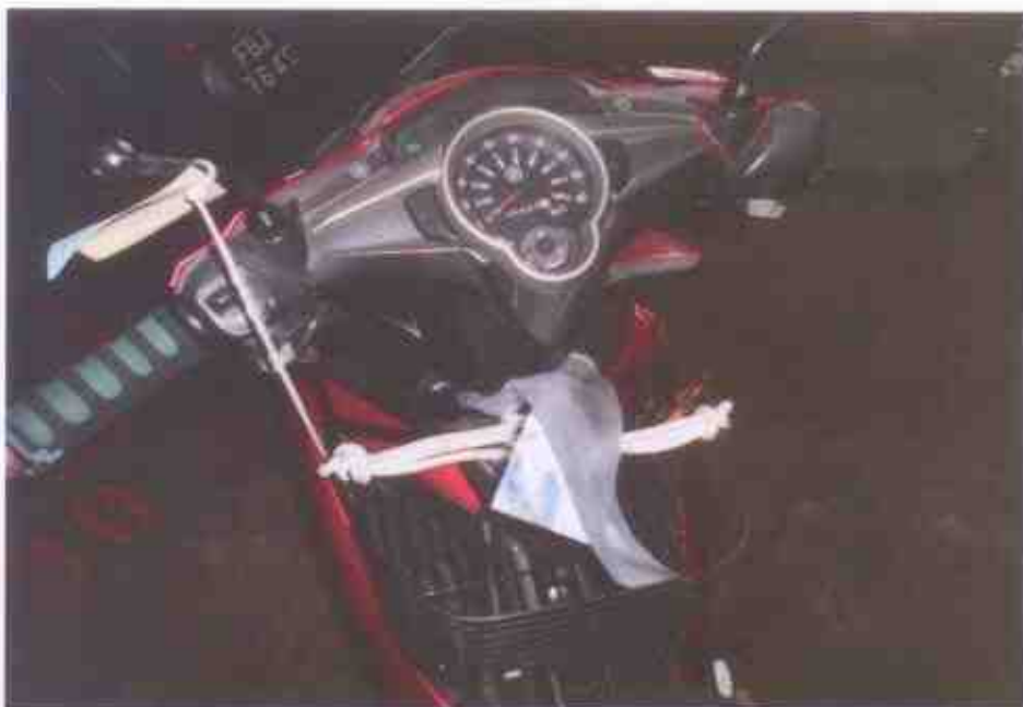
Photo 12 shows the steering system was observed to be in a serviceable condition. It was able to be steered to the full left & right at time of our inspection.
