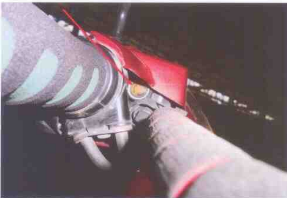
Photo 13 shows our checks on the brake fluid reservoir had also indicated that the brake fluid was of sufficient level for operational purposes, and without contamination.
