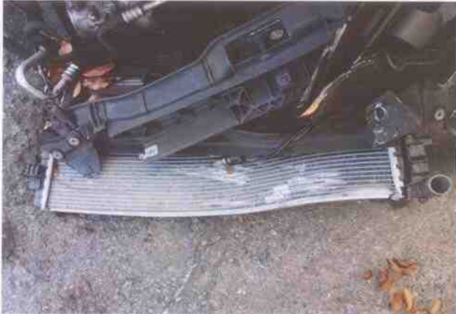
Photo 4 shows a closer view of the damage at the frontal portion of the Motor Car's engine. The impact force was significant, causing the various parts and components inside the engine compartment to be dislodged from its original installation.
