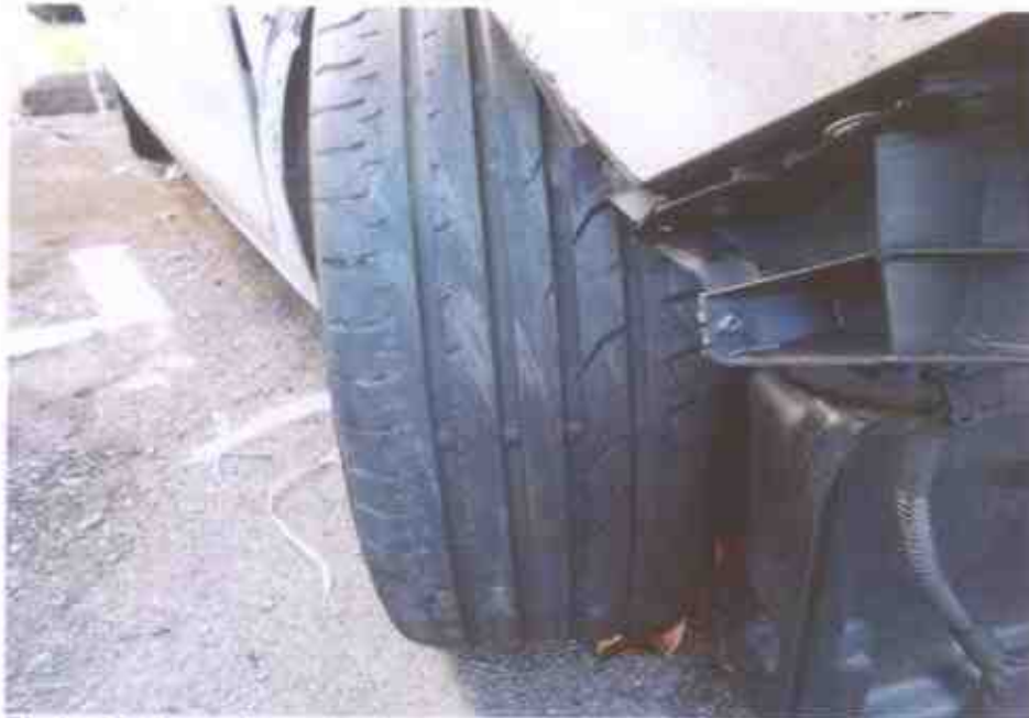
Photo 14 shows the condition of the front right portion of the Motor Car, which was observed to be in serviceable condition. We did not find any tear, cut or burst mark(s) on the outer and the inner sidewalls as well as across the tread of the 4 tyres. The 4 tyres were also observed to be sufficiently inflated for vehicular operation with remaining tread depth of approximately at 4mm.
