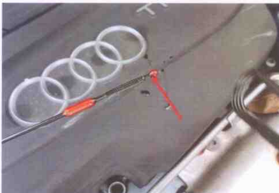
Photo 21 shows the close up view of the insufficient engine fluid due to the leakage as a result of the accident.
