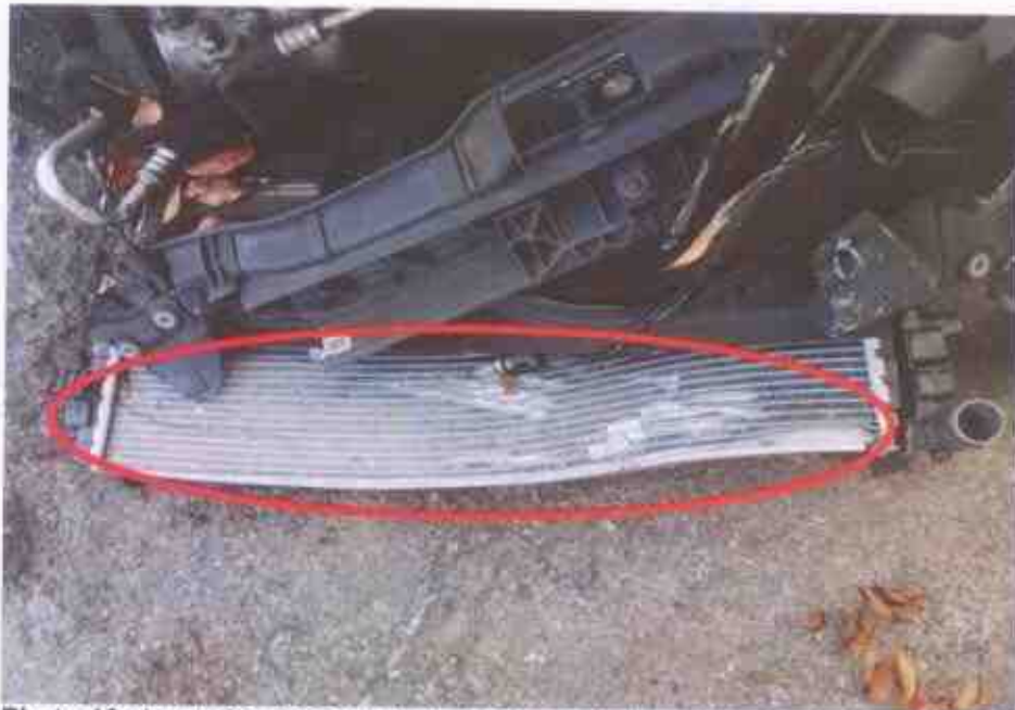
Photo 19 shows the close up view of the radiator's tank that was observed to be damaged likely due to the accident impact. Hence cause leakage to the coolant fluid.
