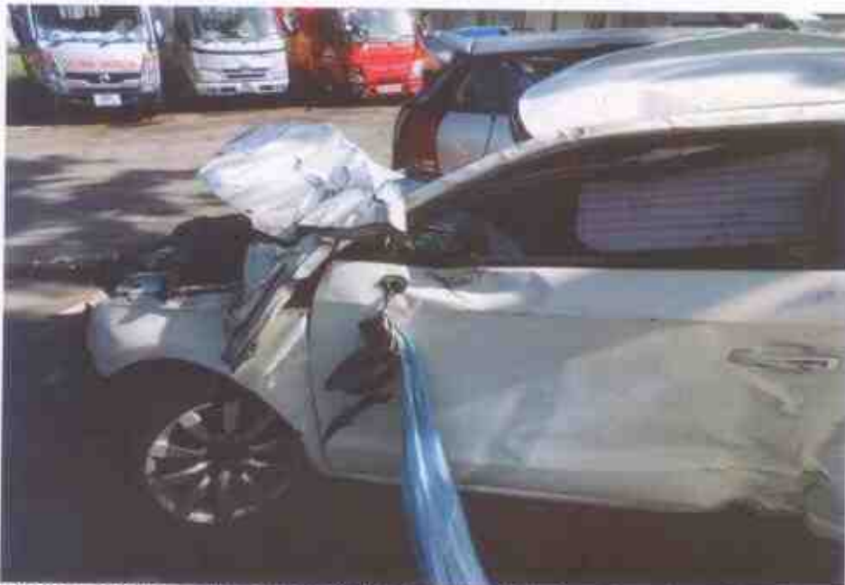
Photo 7 shows a closer view of the damage at the frontal portion of the Motor Car. The impact force was significant, causing the various parts and components inside the engine compartment to be pushed inwards, towards the rear of the Motor Car.
