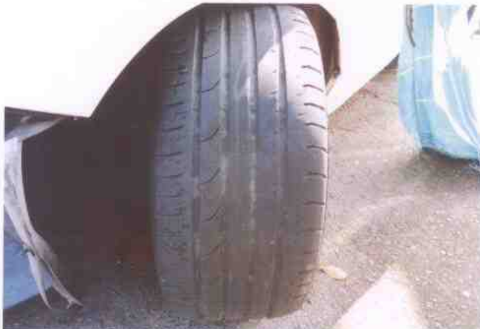
Photo 15 shows the condition of the front left tyre of the Motor Car, which was observed to be in serviceable condition. The 4 tyres were also observed to be sufficiently inflated for vehicular operation with remaining tread depth of approximately at 4mm.
