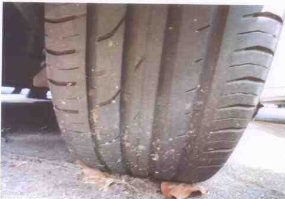
Photo 17 shows the condition of the rear right tyre of the Motor Car, which was observed to be in serviceable condition. The 4 tyres were also observed to be sufficiently inflated for vehicular operation with remaining tread depth of approximately at 4mm.
