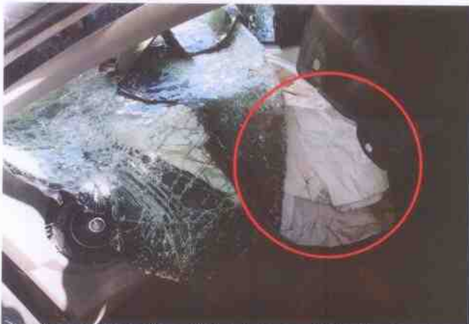
Photo 28 shows the Supplemental Restraint System (SRS) of the Motor Car was however likely to be in normal operating condition at the material time of the accident. The evidence of the deployed front passenger's airbag indicates that the impact sensors and control module of the Motor Car's SRS were all in serviceable condition at the material time of accident.
