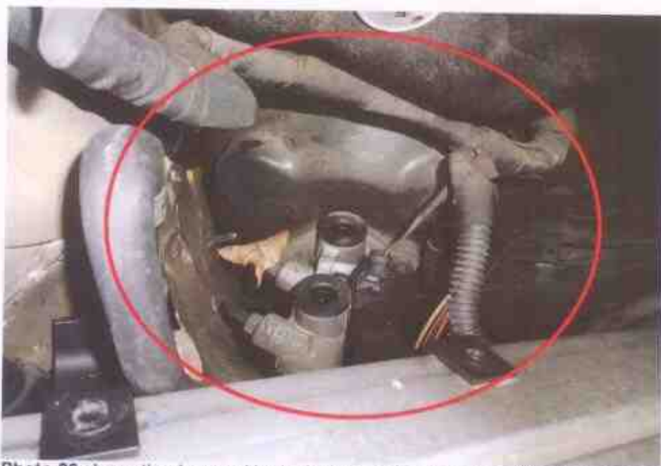
Photo 26 shows the damaged brake booster of the Motor Car. We observe signs of brake fluid leakage at the time of our inspection of the Motor Car.
