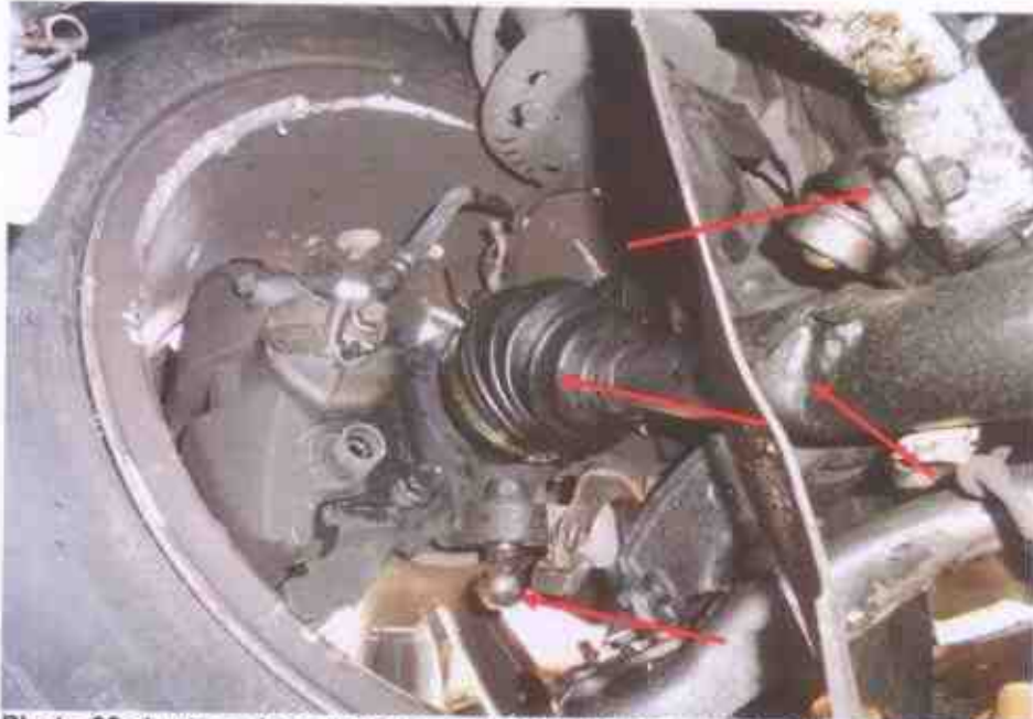
Photo 22 shows a close up view on the front left drive shaft of the Motor Car. We were not able to conduct any tests on the steering system of the Motor Car due to the damage to these components.
