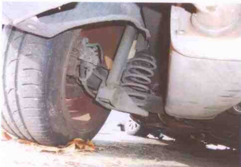
Photo 25 shows the braking & steering components at the rear left wheel of the Motor Car. We did not observe any leakage of brake fluid at the time of our inspection of the Motor Car.
