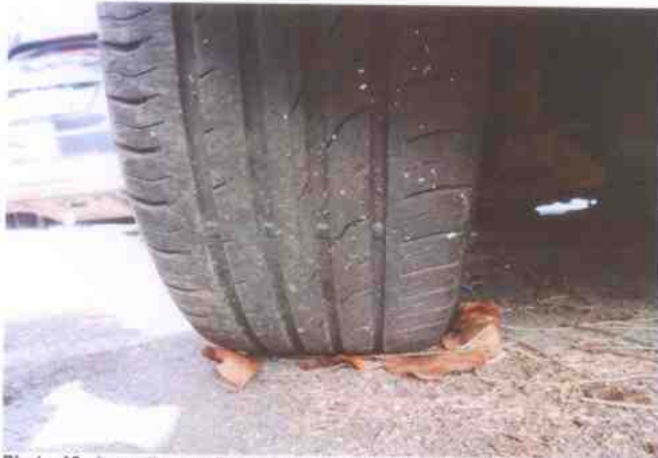
Photo 16 shows the condition of the rear left tyre of the Motor Car, which was observed to be in serviceable condition. The 4 tyres were also observed to be sufficiently inflated for vehicular operation with remaining tread depth of approximately at 4mm.
