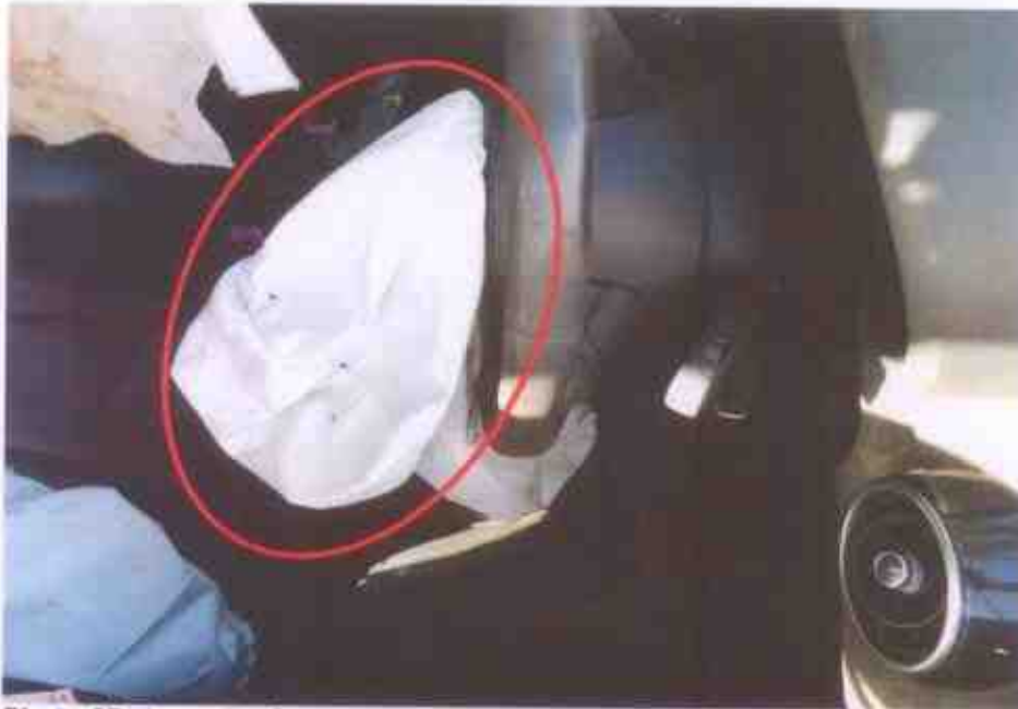
Photo 27 shows the Supplemental Restraint System (SRS) of the Motor Car was however likely to be in normal operating condition at the material time of the accident. The evidence of the deployed front driver's airbag indicates that the impact sensors and control module of the Motor Car's SRS were all in serviceable condition at the material time of accident.
