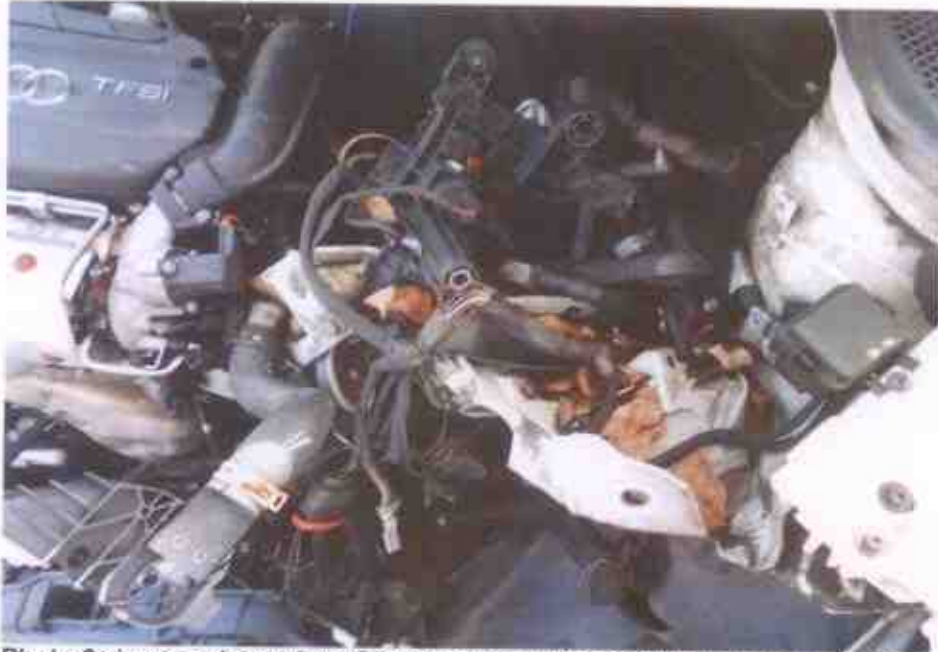
Photo 6 shows a closer view of the damage at the frontal left portion of the Motor Car. The impact force was significant, causing the various parts and components inside the engine compartment to be dislodged from its original installation.
