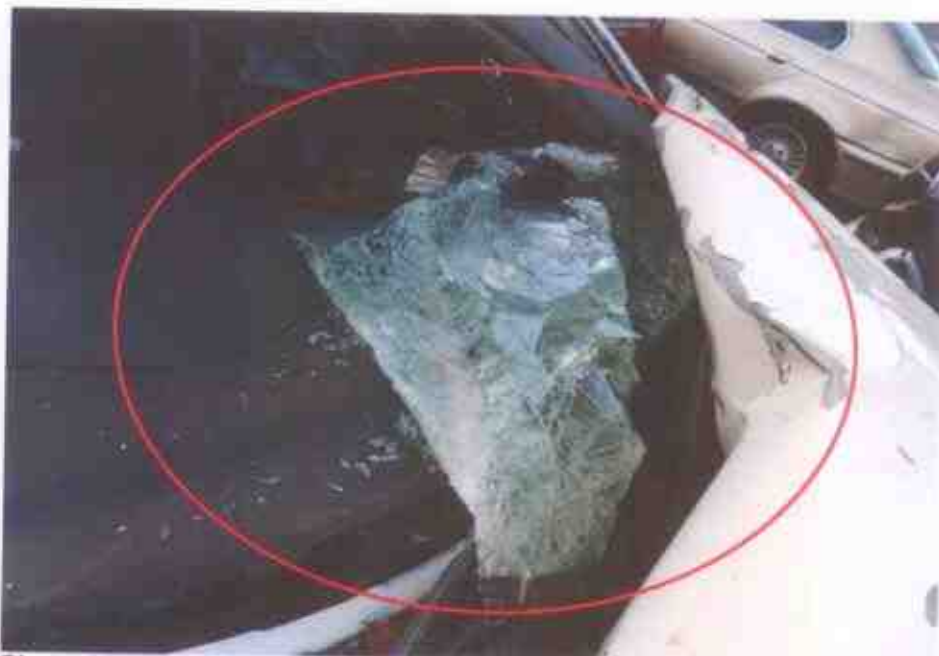
Photo 10 shows a closer view of the damage at the windscreen area of the Motor Car. The impact force was significant, causing the windscreen to sustain a shattering cracked.
