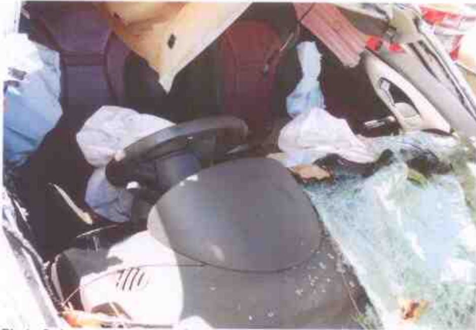
Photo 8 shows a closer view of the damage at the driver's seat of the Motor Car. The impact force was significant, causing the various parts and components inside the interior compartment to be pushed inwards, including its ignition system.
