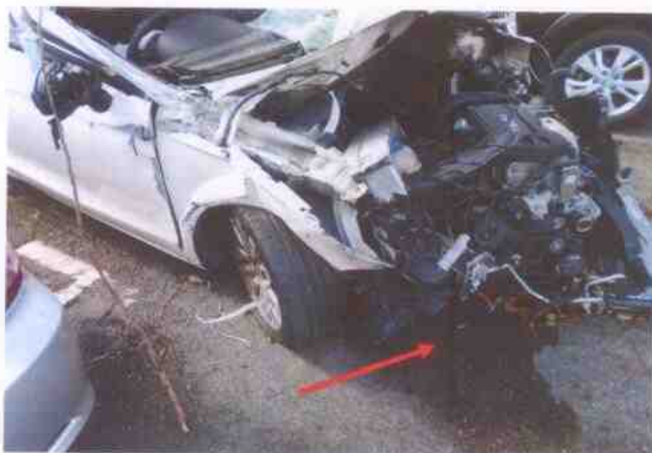
Photo 18 shows the semi-close up view of the dislodged engine of the Motor Car. Signs of fluid leakage stains were observed on the ground due to the accident's impact. Fluids such as brake fluid, steering fluid, engine fluid & coolant fluid were found to be leaking as a result of the accident.
