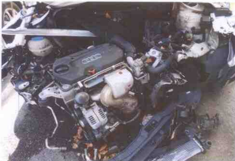
Photo 5 shows a closer view of the damage at the frontal right portion of the Motor Car. The impact force was significant, causing the various parts and components inside the engine compartment to be dislodged from its original installation.
