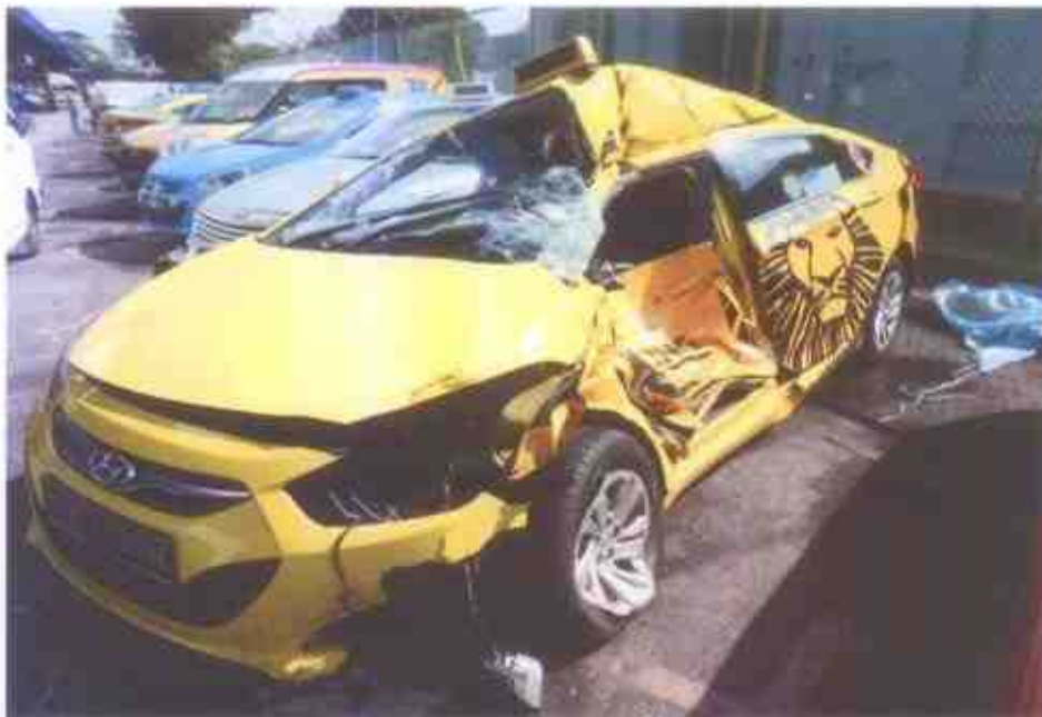
Photo 1 shows a general view of the frontal left portion of the Motor Taxi at the time of our inspection. The Motor Taxi was observed to have sustained extensive impact damage at its frontal, left & rear portion. The impact force was significant, causing the various parts and components to be damaged as a result of the accident.
