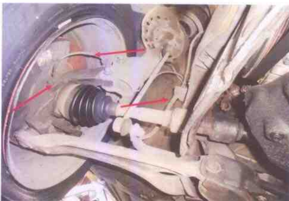
Photo 20 shows the braking components at the front right wheel of the Motor Taxi. We did not observe any leakage of brake fluid at the time of our inspection of the Motor Taxi.
