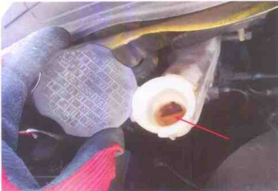
Photo 13 shows the close up view of the brake fluid that was seen with sufficient level not affected by the accident's impact.
