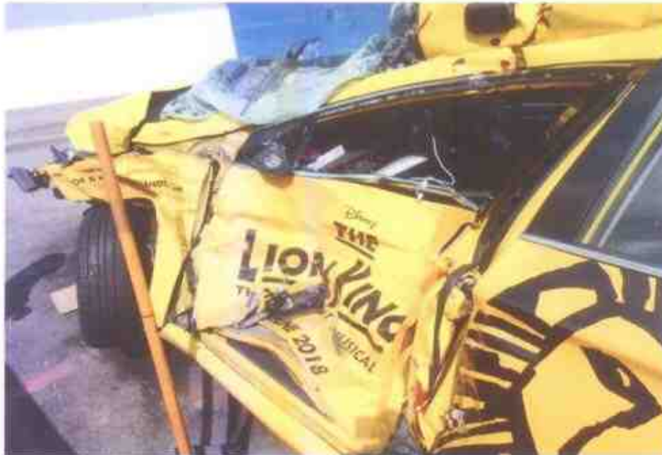
Photo 4 shows a closer view of the damage sustained on the left portion of the Motor Taxi. The impact force was significant, causing the left portion of the Motor Taxi to be pushed inwards, towards the right of the Motor Taxi.
