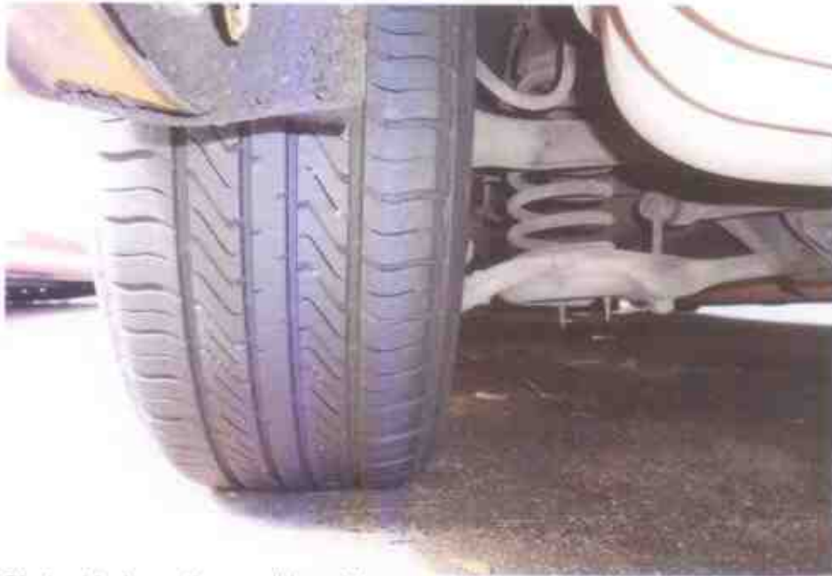
Photo 10 shows the condition of the rear left tyre of the Motor Taxi, which was observed to be in serviceable condition with remaining tread depth of approximately 4mm. There was also no tear, cut or burst mark(s) on the outer and the inner sidewalls as well as across the tread of this tyre.
