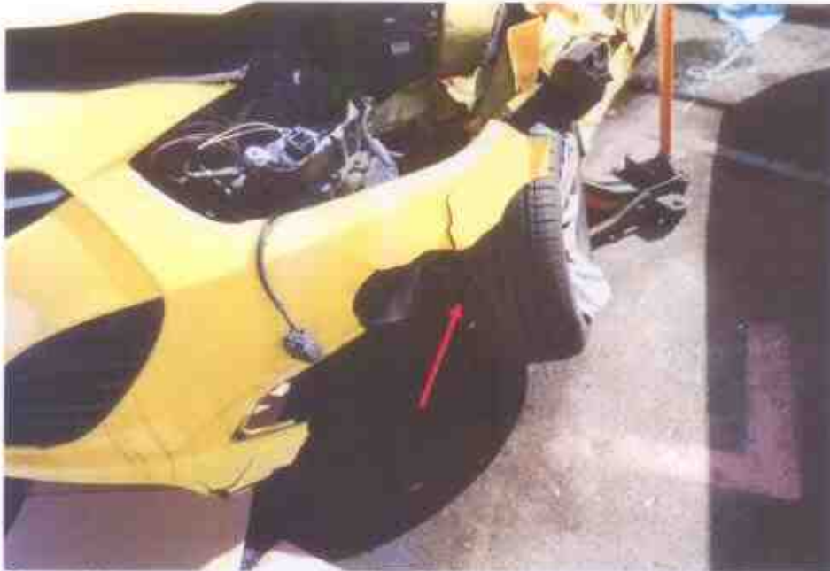
Photo 17 shows the misalignment of the front left wheel of the Motor Taxi.
