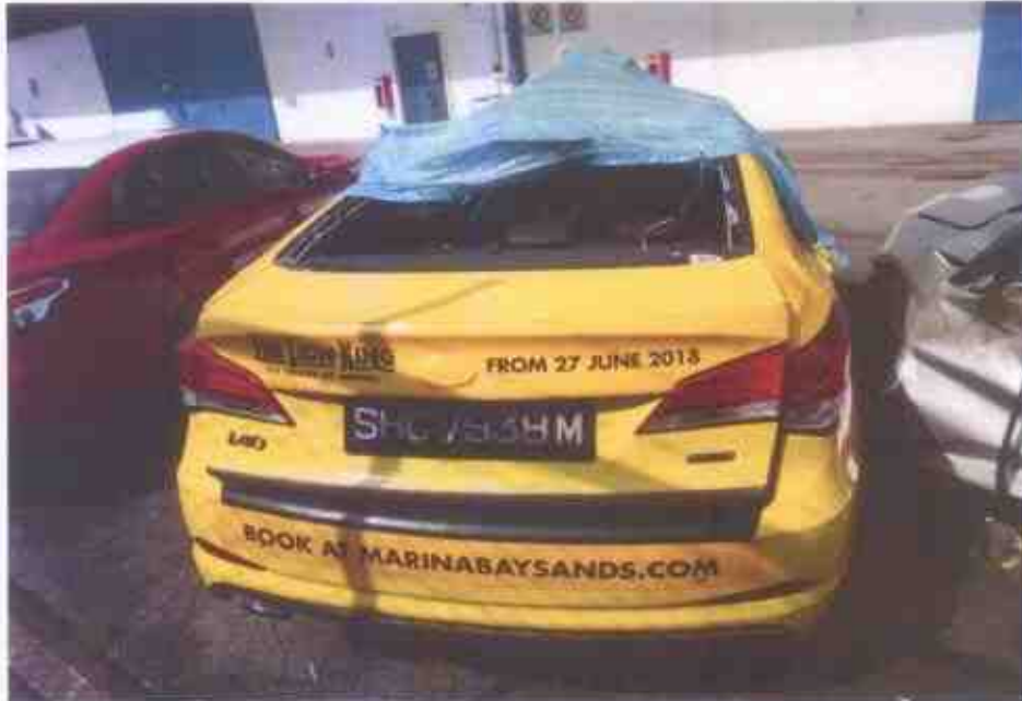
Photo 6 shows a closer view of the damaged rear boot lid. The impact force was significant, causing it to be misaligned due to the accident's impact.
