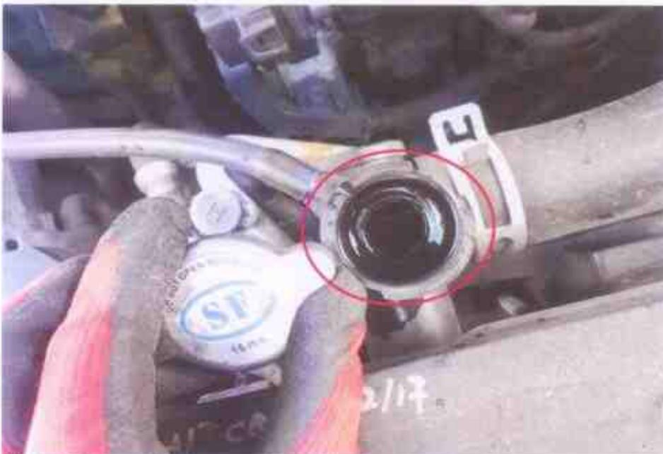
Photo 12 shows the close up view of the engine coolant that was seen empty affected by the accident's impact.
