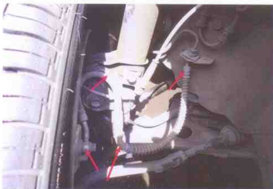
Photo 19 shows the braking components at the front left wheel of the Motor Taxi. We did not observe any leakage of brake fluid at the time of our inspection of the Motor Car.
