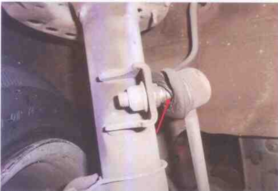
Photo 18 shows the damaged tie rod of the front right wheel of the Motor Taxi.
