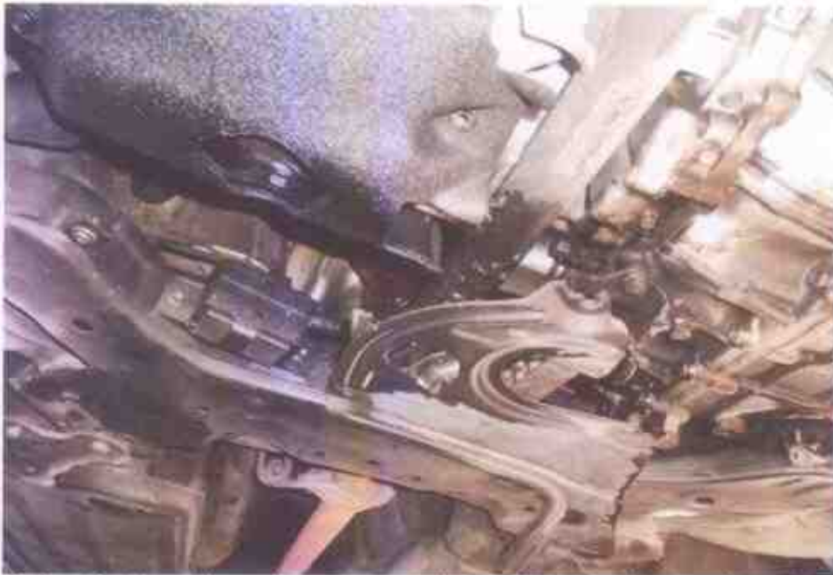
Photo 15 shows the undercarriage of the engine area. It was observed to sustained fluid leakage as a result of the accident.
