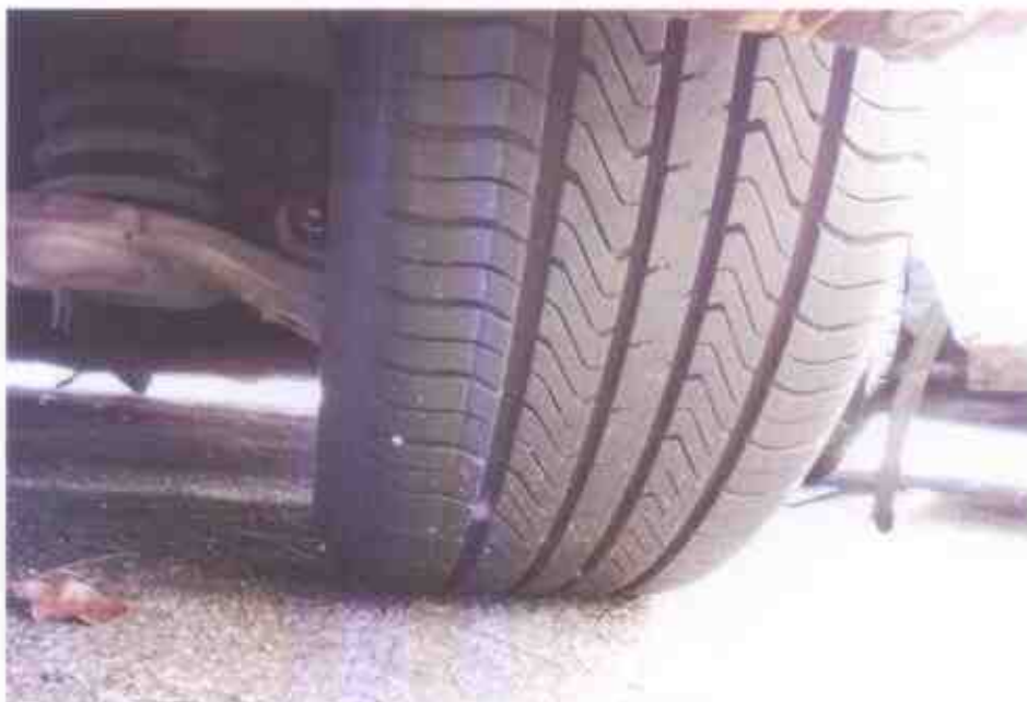
Photo 9 shows the condition of the rear right tyre of the Motor Taxi, which was observed to be in serviceable condition with remaining tread depth of approximately 4mm. There was also no tear, cut or burst mark(s) on the outer and the inner sidewalls as well as across the tread of this tyre.
