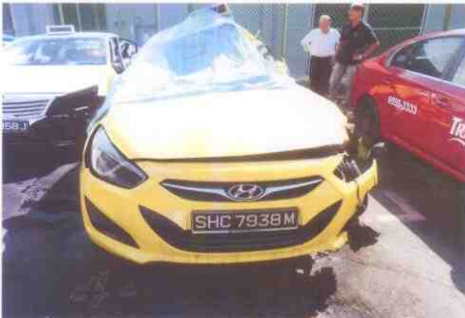
Photo 3 shows a general view of the front portion of the Motor Taxi at the time of our inspection. The Motor Taxi was observed to have sustained extensive impact damage at its front left & right portion.
