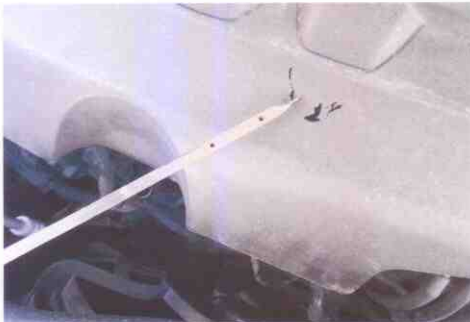
Photo 14 shows the engine oil dip stick of the Motor Taxi at the time of our inspection. The engine oil was observed to be insufficient level as a result of the accident.
