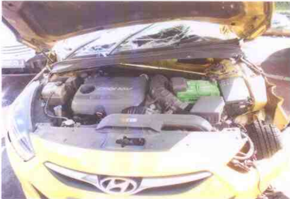
Photo 11 shows a general view of the Motor Car's engine compartment. Some of the various parts and components inside the engine compartment were observed to be affected by the accident. There were also sign(s) or indication(s) of fluid leakage and/or fluid stain within the engine compartment.
