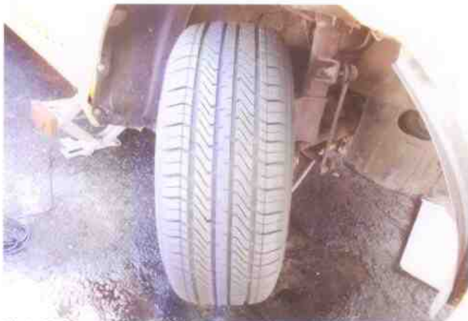
Photo 7 shows the condition of the front right tyre of the Motor Taxi, which was observed to be deflated with remaining tread depth of approximately 5mm. However, there was no tear, cut or burst mark(s) on the outer and the inner sidewalls as well as across the tread of this tyre.
