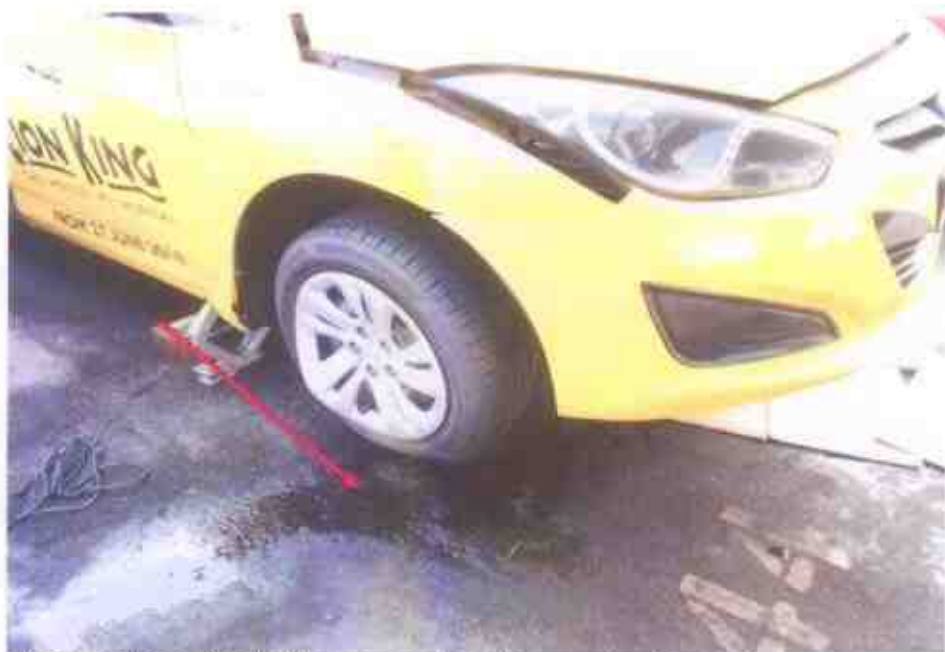
Photo 16 shows the fluid leakage spill on the ground surface.
