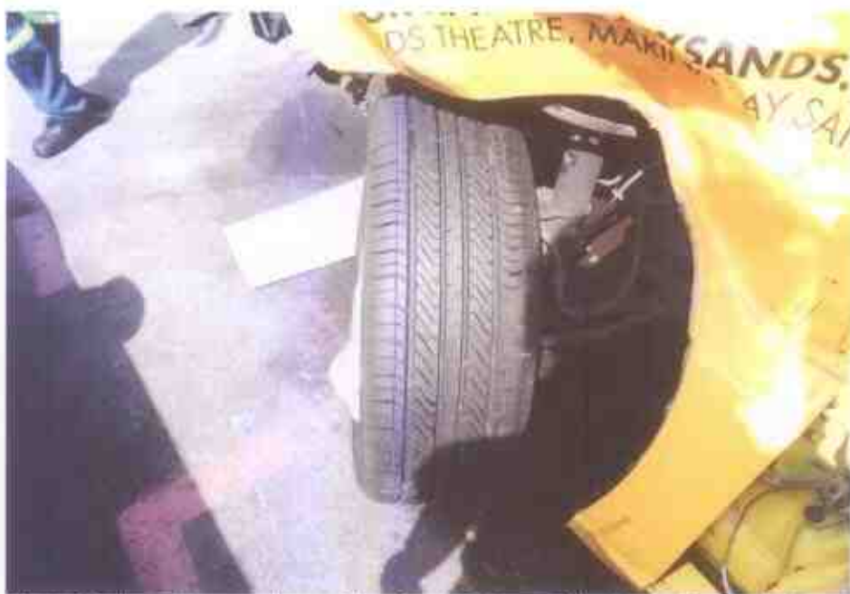
Photo 8 shows the condition of the front left tyre of the Motor Taxi, which was observed to be deflated with remaining tread depth of approximately 5mm. However, there was no tear, cut or burst mark(s) on the outer and the inner sidewalls as well as across the tread of this tyre.
