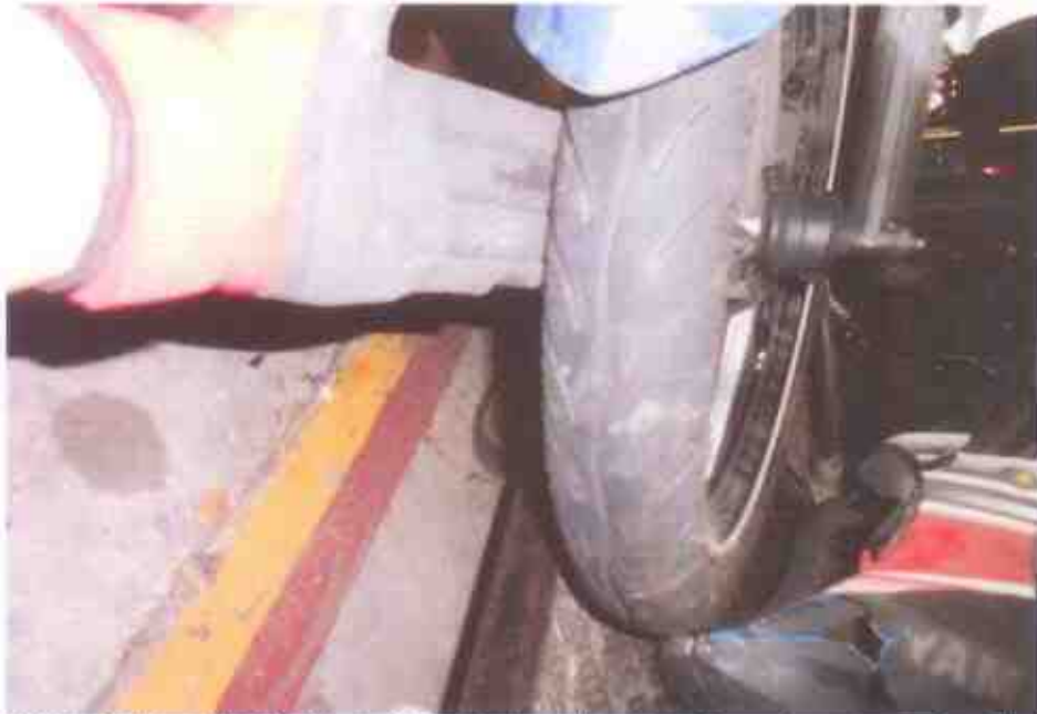
Photo 9 shows the front tyre of the Motorcycle at the time of our inspection. The pattern of the tread was clearly visible with remaining tread depth of approximately 4mm. There was no tear, burst mark(s) and/or punctured hole(s) on the sidewalls as well as across the tread of the front tyre. However, the wheel rim was observed to be broken as a result of the accident.
