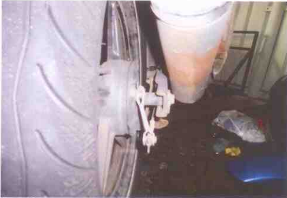
Photo 18 shows the rear brake drum spring & cable was observed to be in serviceable condition unaffected by the accident despite the damage sustained on the foot brake pedal.
