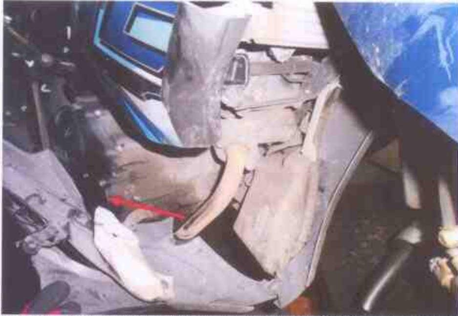
Photo 10 shows sign(s) or indication(s) of fluid leakage observed around the engine's underside area of the Motorcycle.
