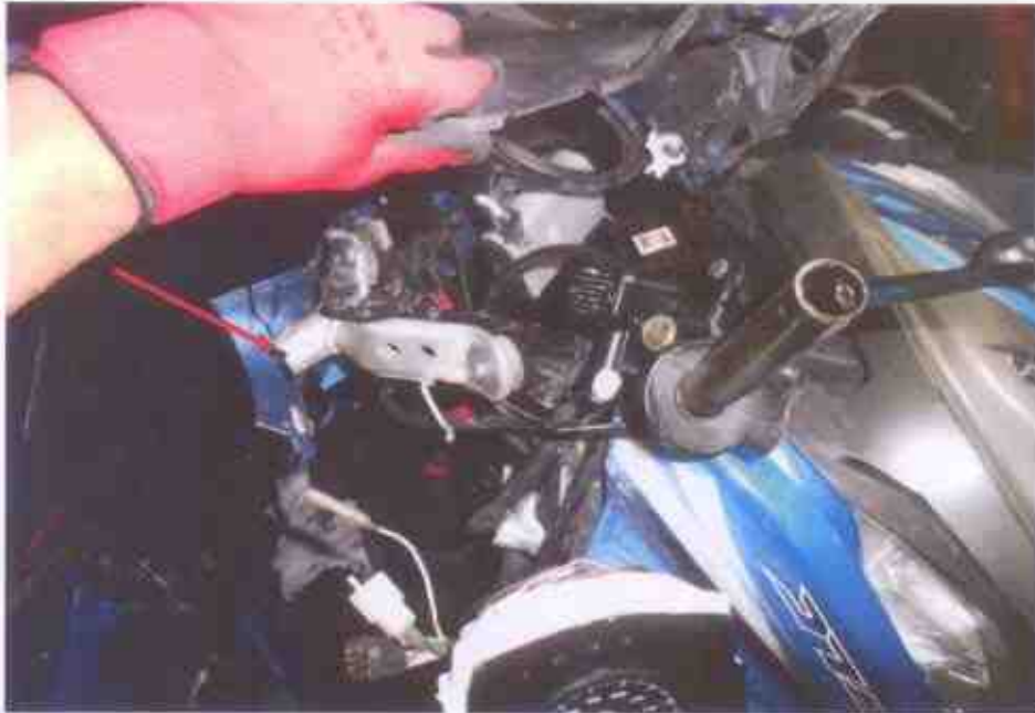
Photo 6 shows a close-up view of the dislodged handle bar. The Motorcycle was observed to have sustained relatively extensive impact including damages to the steering system to the accident collision.
