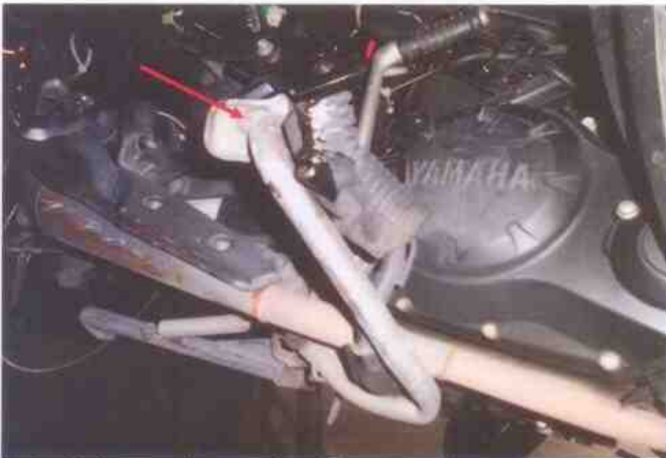
Photo 7 shows a close-up view of the damaged rear brake pedal. The Motorcycle was observed to have sustained relatively extensive impact including damages to the braking system to the accident collision.
