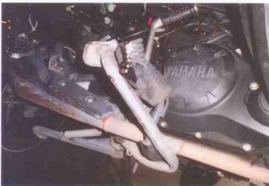
Photo 17 shows the rear brake pedal (arrowed) was observed to be in damaged due to the accident's impact collision.
