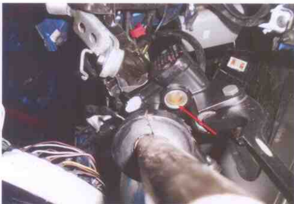
Photo 16 shows the front brake fluid was still at a sufficient level despite leakage observed at the connecting hose.
