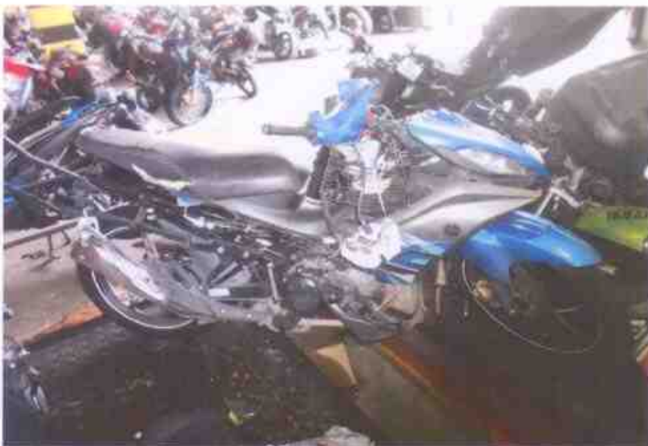
Photo 5 shows a general view of the right portion of the Motorcycle at the time of our inspection. The Motorcycle was observed to have sustained relatively extensive impact due to the accident collision.
