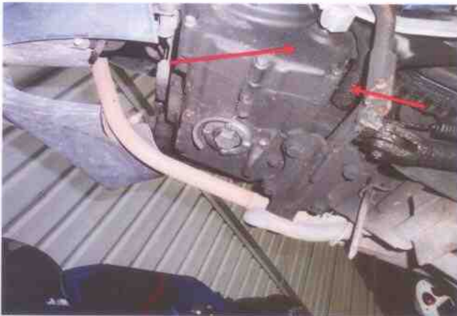
Photo 11 shows sign(s) or indication(s) of fluid leakage observed at the engine's undercarriage of the Motorcycle.
