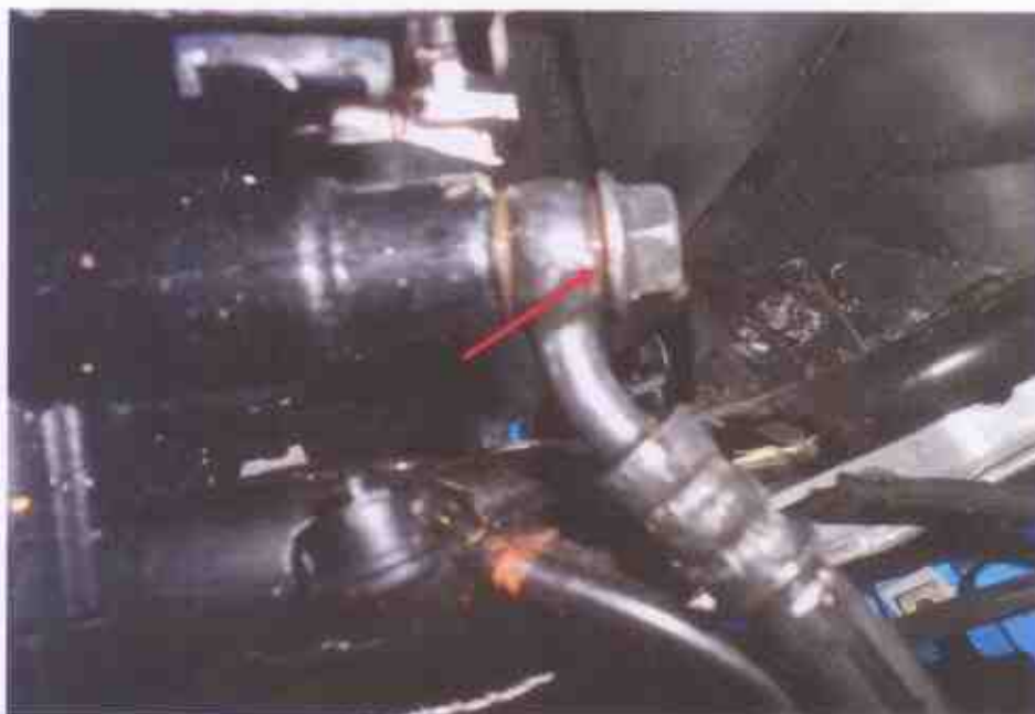
Photo 15 shows the front brake fluid leakage was observed to be caused by the accident. The brake fluid leakage was observed to be coming from the connecting hose when we grip the hand brake lever at the time of our inspection.
