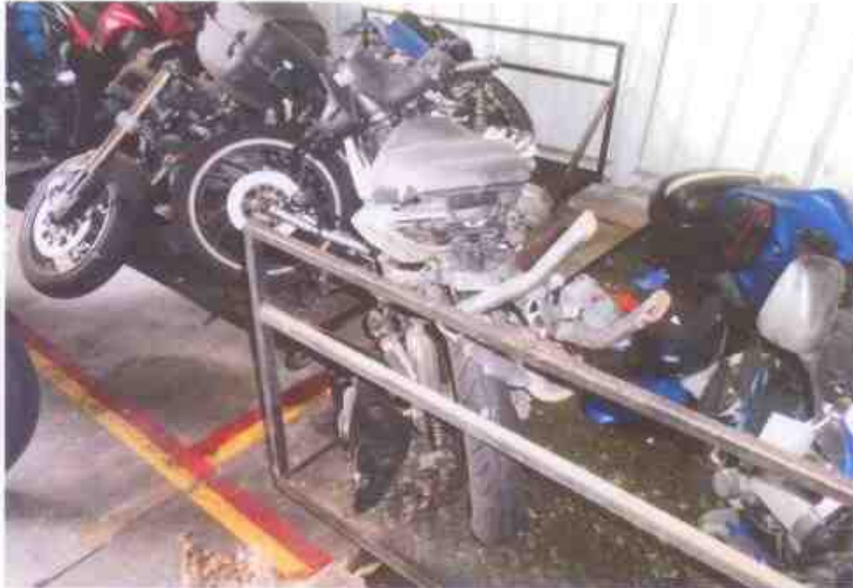
Photo 2 shows the Motorcycle rear portion that was observed to be severely damaged by the accident's impact collision. The rear parts that were observed to be damaged include its rear tail lamp, compartment rack, seat assembly and missing licence plate amongst others.
