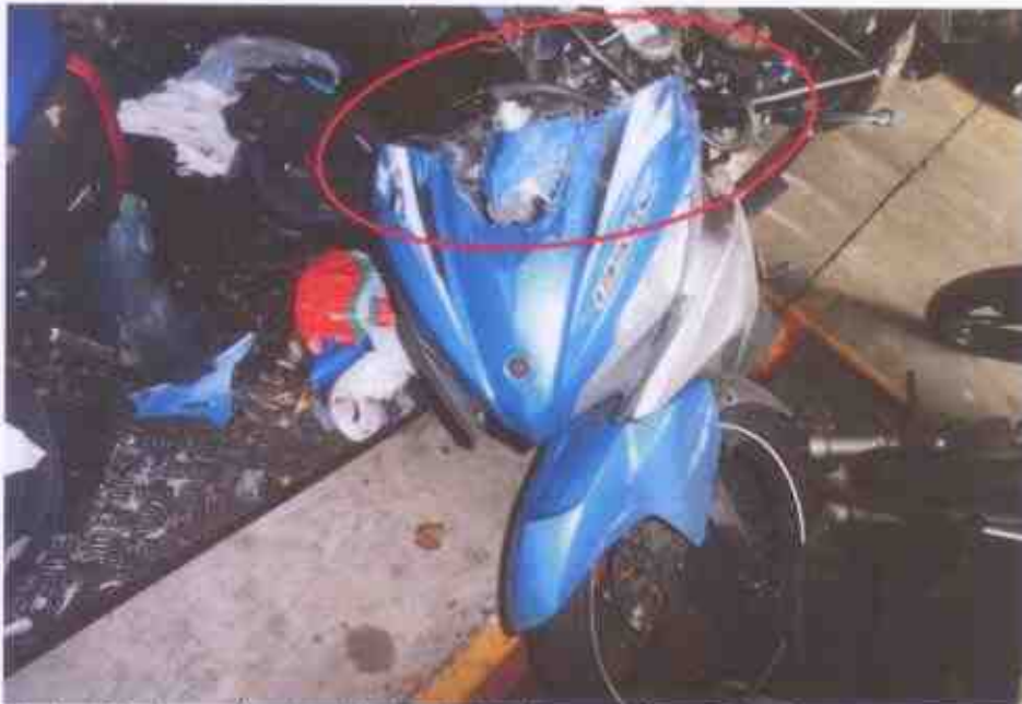
Photo 19 shows the handle bar (circled) was observed to be damaged as a result of the accident. Hence, we are unable to conduct any tests on the steering system of the Motorcycle.
