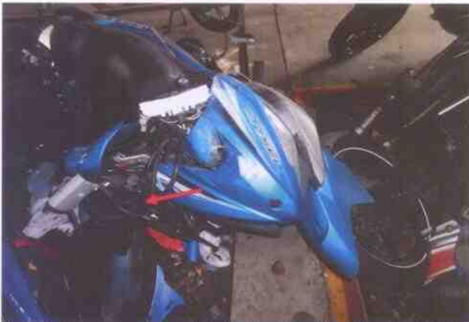
Photo 3 shows a close-up view of the frontal portion of the Motorcycle at the time of our inspection. The Motorcycle was observed to have sustained relatively extensive impact including damages to the steering system due to the accident collision.
