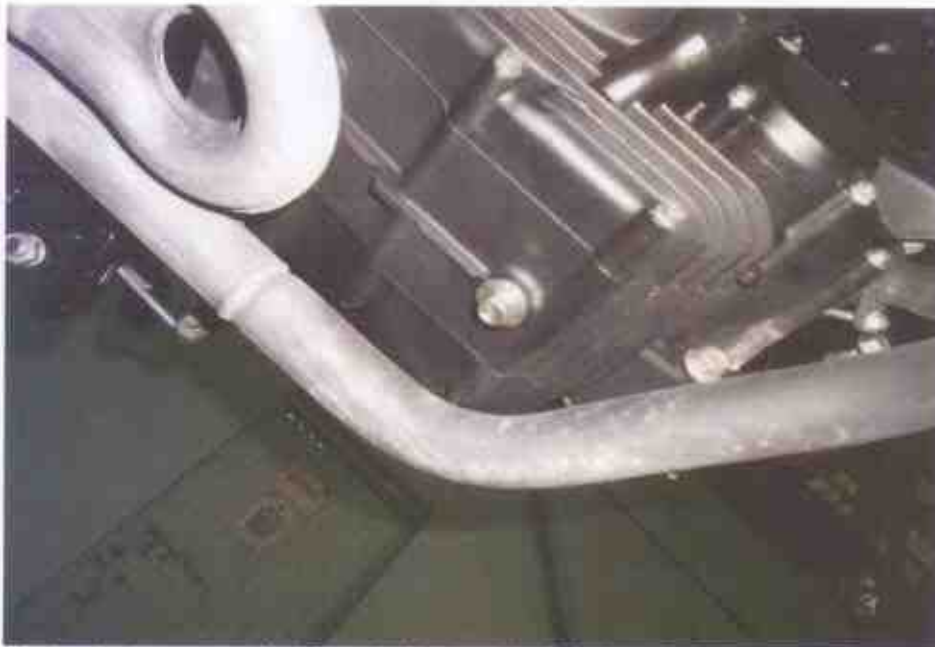
Photo 8 shows no sign(s) or indication(s) of fluid leak observed around the underside of the engine area of the Motorcycle.
