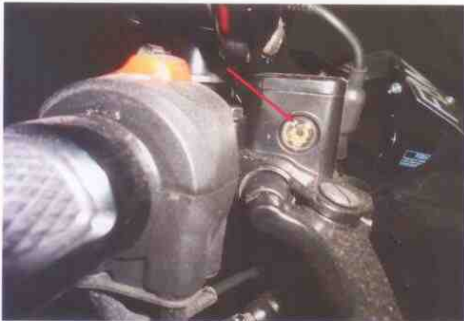
Photo 12 shows our checks on the brake fluid (front) reservoir had also indicated that the brake fluid was of sufficient level for operational purposes, and without contamination.
