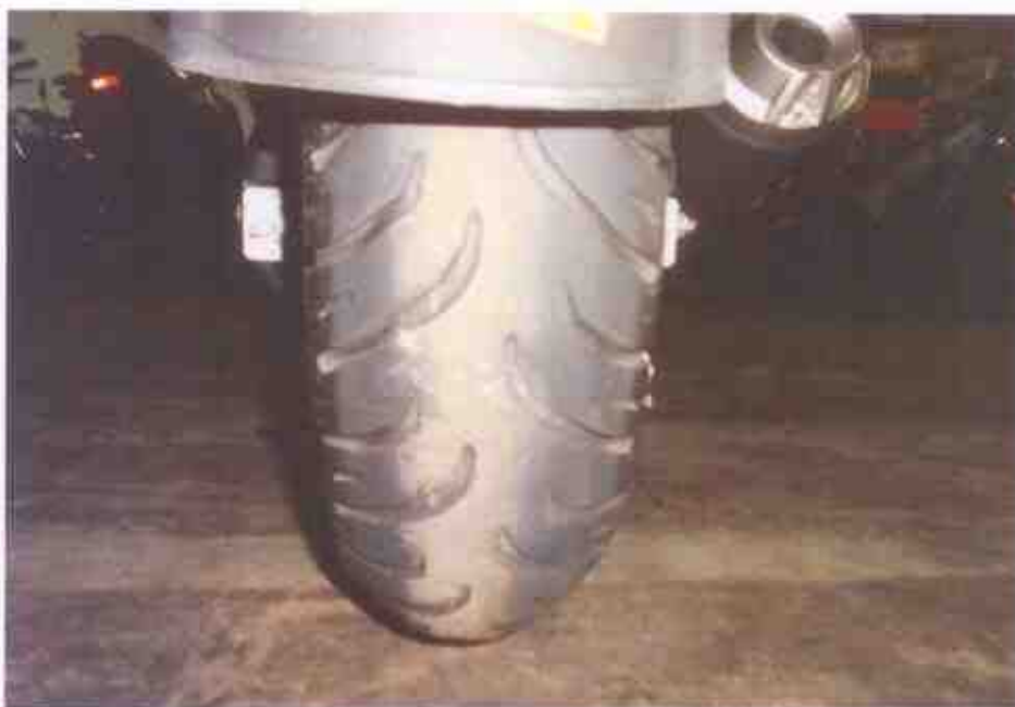
Photo 6 shows the rear tyre of the Motorcycle. The rear tyre was observed to be in serviceable condition with remaining tread depth of approximately 4mm. The tyre was also observed to be sufficiently inflated for vehicular operation.
