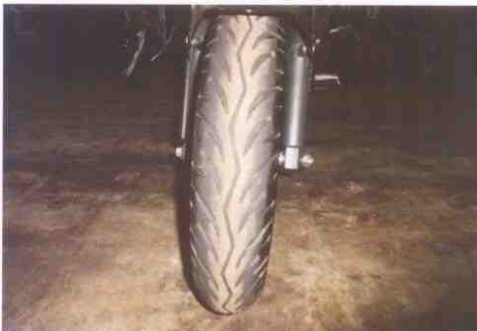
Photo 7 shows the front tyre of the Motorcycle. The front tyre was observed to be in serviceable condition with remaining tread depth of approximately 5mm. The tyre was also observed to be sufficiently inflated for vehicular operation.
