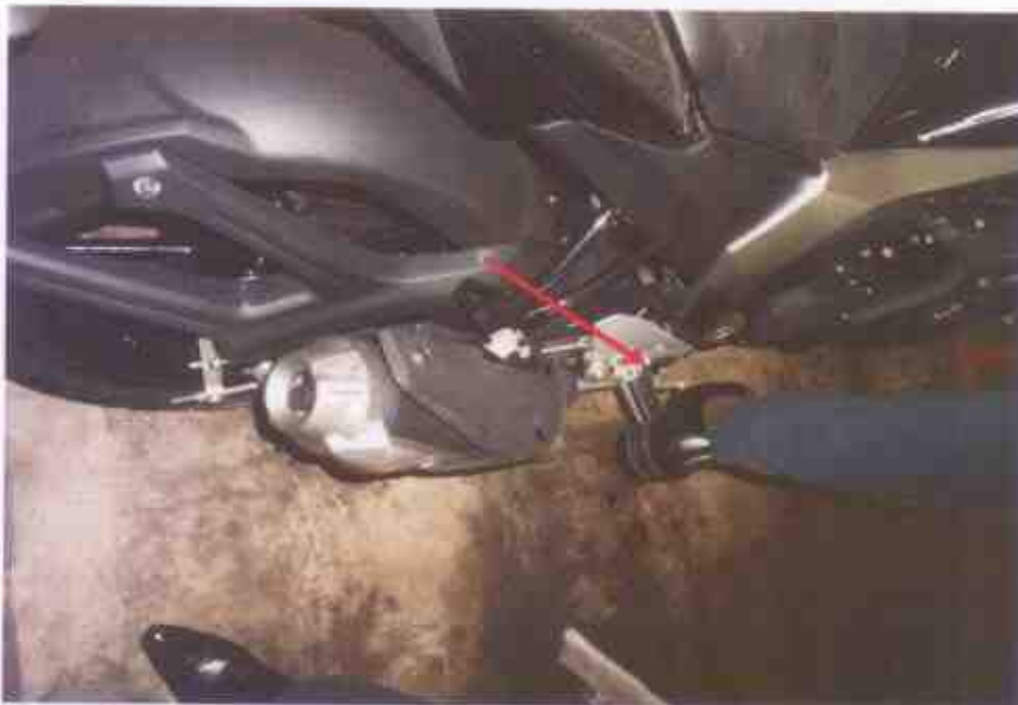
Photo 15 shows testing of the braking of the rear brake in progress. There was some resistance felt (spongy like feel) upon stepping on the brake pedal.
