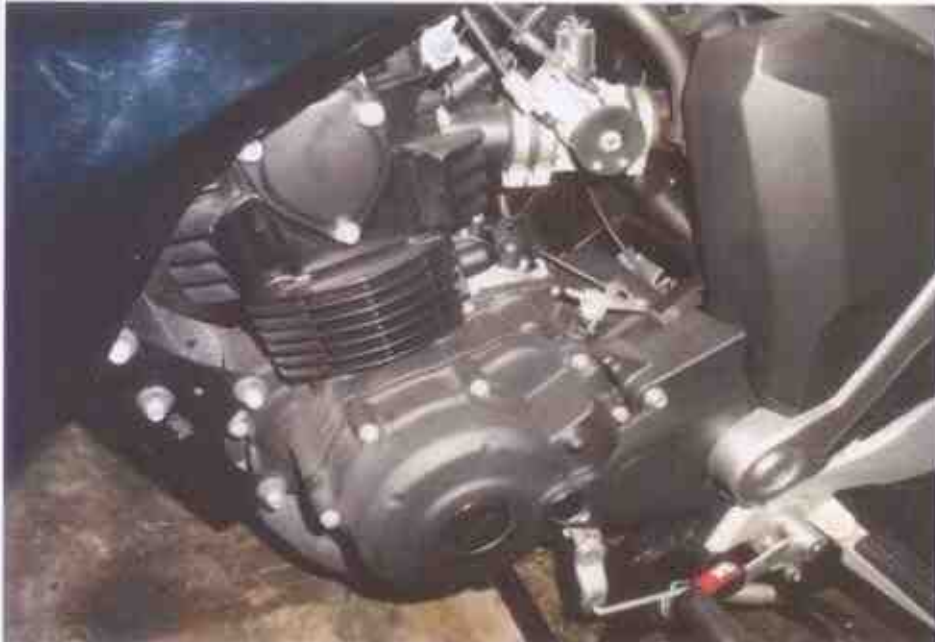
Photo 9 shows no sign(s) or indication(s) of fluid leakage stain observed around the engine area of the Motorcycle.
