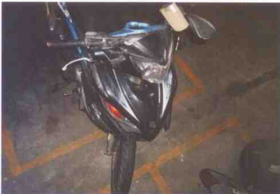
Photo 5 shows a semi close-up view of the frontal portion of the Motorcycle at the time of our inspection. The Motorcycle was observed to be sustained with relatively extensive impact due to the accident collision.
