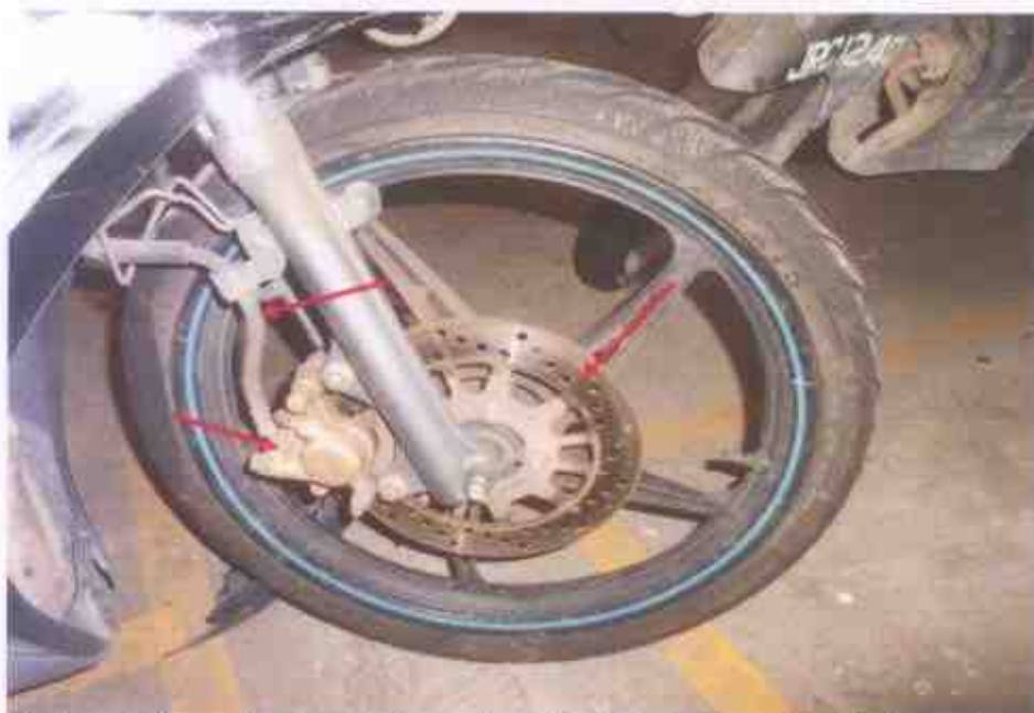
Photo 15 shows the front brake calliper, front brake disc, front brake pad and front brake hose of the Motorcycle, which are all part of the components in the front brake system of the Motorcycle. Our observation found that the front braking components were unaffected by the accident.
