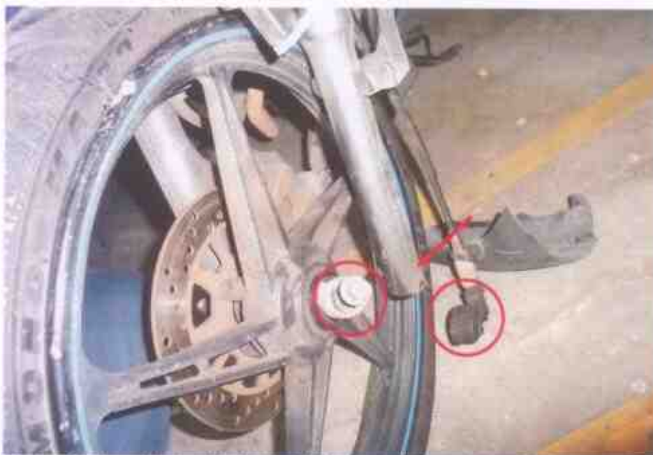
Photo 13 shows the front fork (circled & arrowed) was observed to be dislodged as a result of the accident. Hence, we are not able to conduct any tests on the steering system of the Motorcycle.
