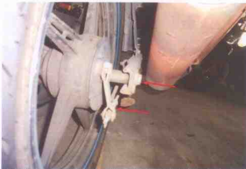
Photo 17 shows the rear brake cable and spring of the Motorcycle (arrowed), which are all part of the components in the rear brake system of the Motorcycle reveal all to be intact and without damage.
