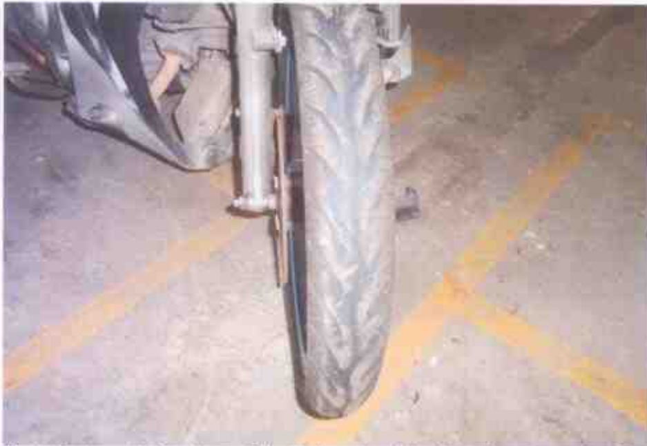
Photo 7 shows the front tyre of the Motorcycle at the time of our inspection. The front tyre was observed to be deflated with remaining tread depth of approximately 3mm as a result of the accident.
