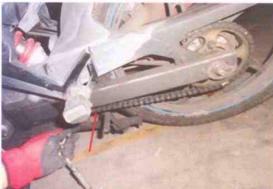
Photo 12 shows the general view of the gear train (arrowed) of the Motorcycle, which was observed to be intact with no misalignment. It was also adequately lubricated for operating purposes. Free play tension was also observed & found adequately acceptable.
