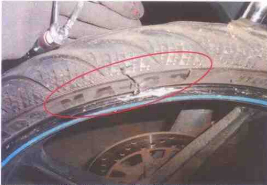
Photo 9 shows further observation on the front tyre that was deflated caused by torn mark at time of our inspection due to the accident's collision impact.
