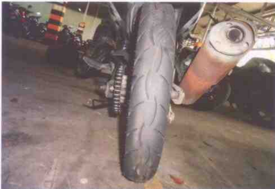
Photo 8 shows the rear tyre of the Motorcycle. The pattern of the tread was clearly visible with remaining tread depth of about 5mm. There was no tear, burst mark(s) and/or punctured hole(s) on the sidewalls as well as across the tread of the rear tyre unaffected by the accident's impact collision.
