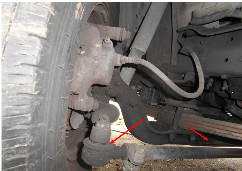
Photo 18 shows the undercarriage components at the front left wheel of the Motor Lorry. The various undercarriage components of the Motor Lorry were all observed to be intact and without any visible damage. This had included the steering rack (arrowed) of the Motor Lorry.
