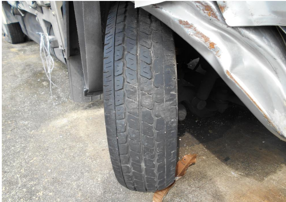
Photo 9 shows the condition of the front right tyre of the Motor Lorry. The front right tyre was observed to be in serviceable condition with remaining tread depth of approximately 5mm. There was also no tear, cut or burst mark(s) on the outer and the inner sidewalls as well as across the tread of this tyre.
