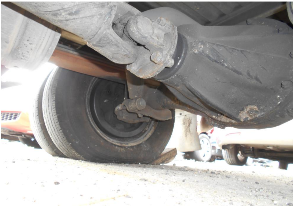
Photo 14 shows the condition of the rear right tyres (inner) of the Motor Lorry, which was observed to be unaffected by the accident's impact.
