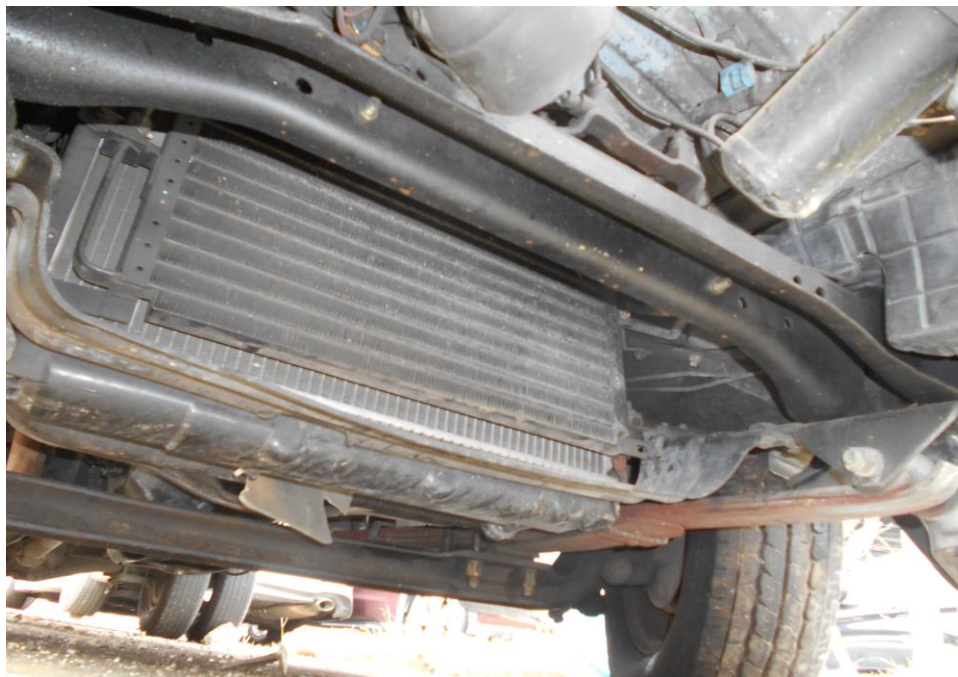
Photo 15 shows the underside of the Motor Lorry, at the area where the engine is located. We were not able to closely inspect the engine compartment of the Motor Lorry due to the extensive damage to its front cabin. Our visual checks from the underside had however appear to indicate that the engine assembly and transmission assembly were both intact and unaffected by the collision.
