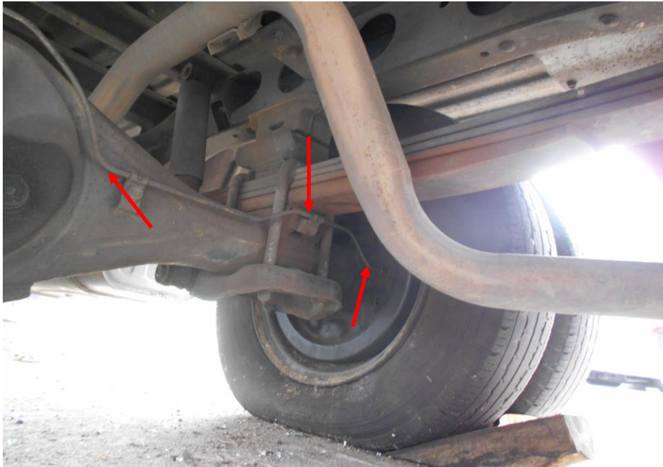
Photo 23 shows the brake hose (arrowed) at the rear wheels of the Motor Lorry. At the time of our inspection, we did not find any sign(s) of brake fluid leakage along the brake hoses and brake pipes.
