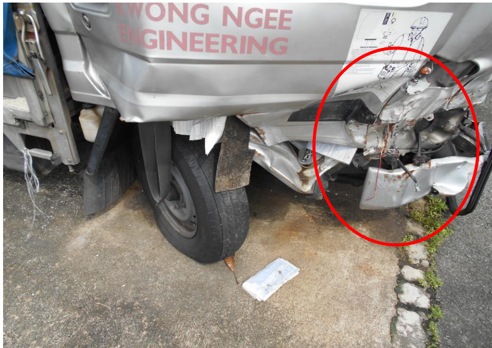
Photo 21 shows the undercarriage components at the front right lower portion of the Motor Lorry. The steering box was observed to be stuck into the buckled lower metal bumper as a result of the accident which disabling the normal operation of the steering system.
