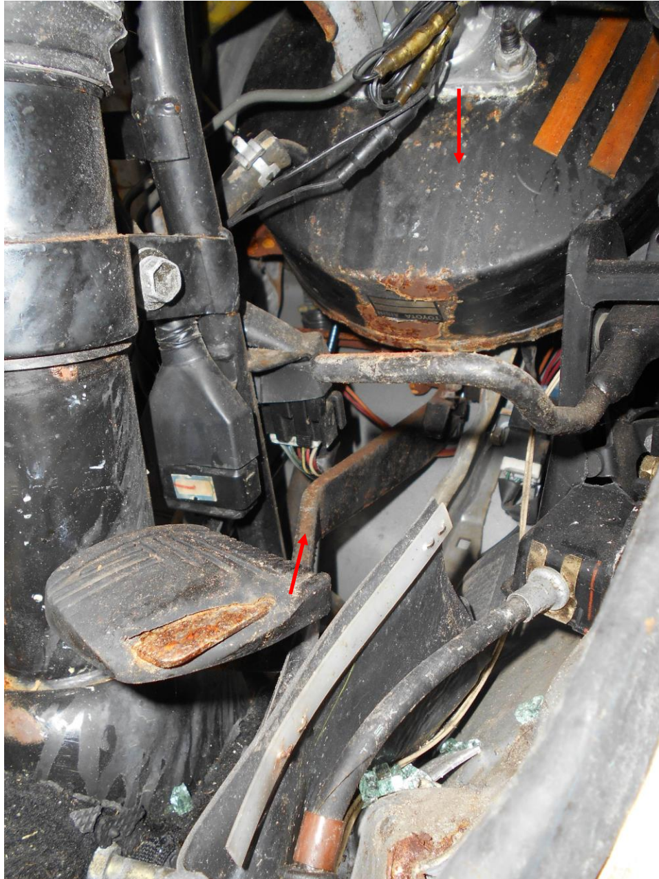
Photo 27 shows the brake booster & brake pedal of the Motor Lorry. At the time of our inspection, we did not find any sign(s) of brake fluid leakage around the Braking system components.
