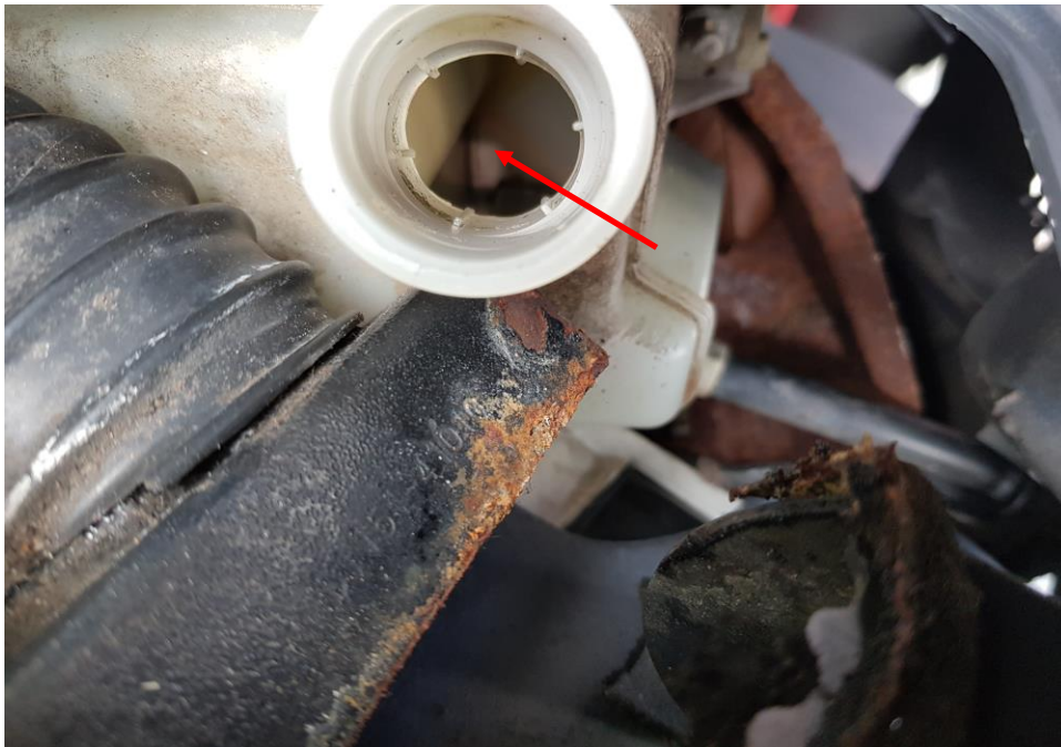
Photo 30 shows the internal view of the brake fluid reservoir tank which was observed to be below the minimum mark of the reservoir tank.
