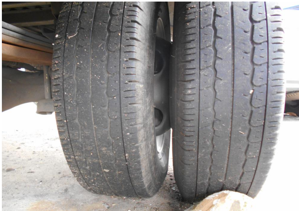
Photo 10 shows the condition of the rear left tyres of the Motor Lorry, which was observed to be in serviceable condition with remaining tread depth of approximately 8mm. There was no tear, cut or burst mark(s) on the outer and the inner sidewalls as well as across the tread of this 2 tyres.
