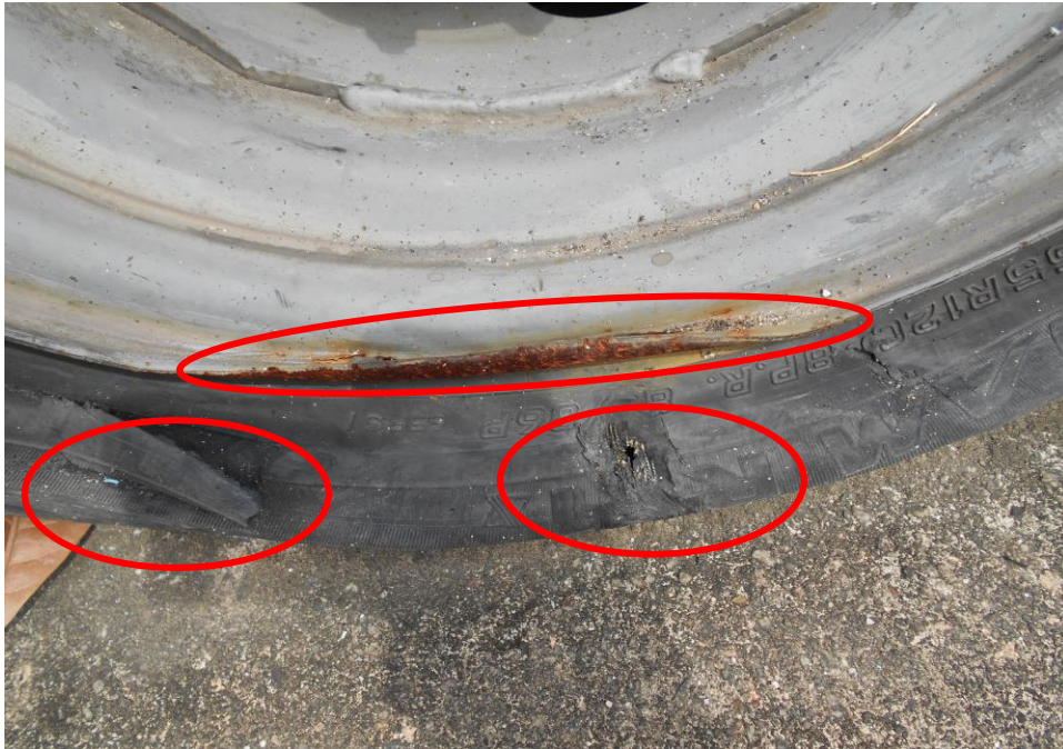
Photo 13 shows the condition of the rear right tyres (outer) of the Motor Lorry, which was observed to be deflated due to the dented rim & cut mark as a result of the accident.
