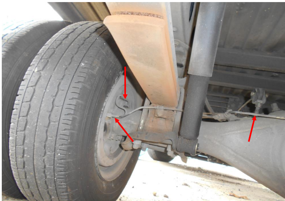
Photo 22 shows the brake hose (arrowed) at the rear wheels of the Motor Lorry. At the time of our inspection, we did not find any sign(s) of brake fluid leakage along the brake hoses and brake pipes.
