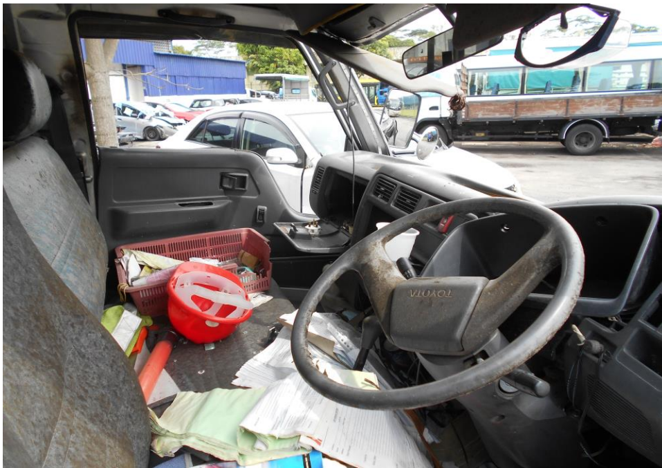
Photo 4 shows the interior of the front cabin. The dashboard, steering wheel, floor panel and braking system (pedal) inside the front cabin were all observed to be pushed/buckled inwards, towards the rear of the Motor Lorry. This is consistent to the nature of this accident where the direction of impact onto the Motor Lorry was from the front to rear direction.
