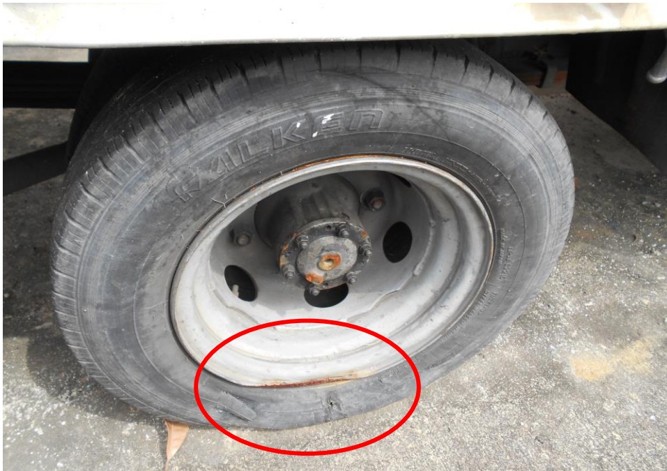
Photo 12 shows the condition of the rear right tyres (outer) of the Motor Lorry, which was observed to be deflated due to the dented rim & cut mark as a result of the accident.
