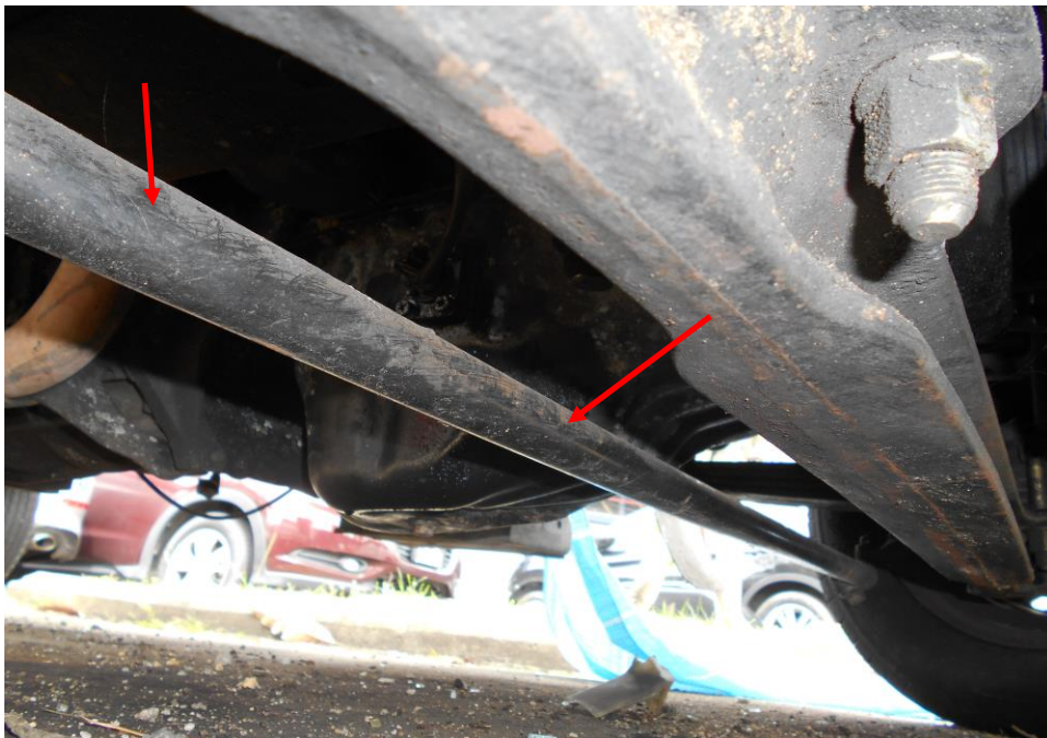
Photo 20 shows the undercarriage components at the centre portion of the Motor Lorry. The steering rod was observed to be intact and without any visible damage.
