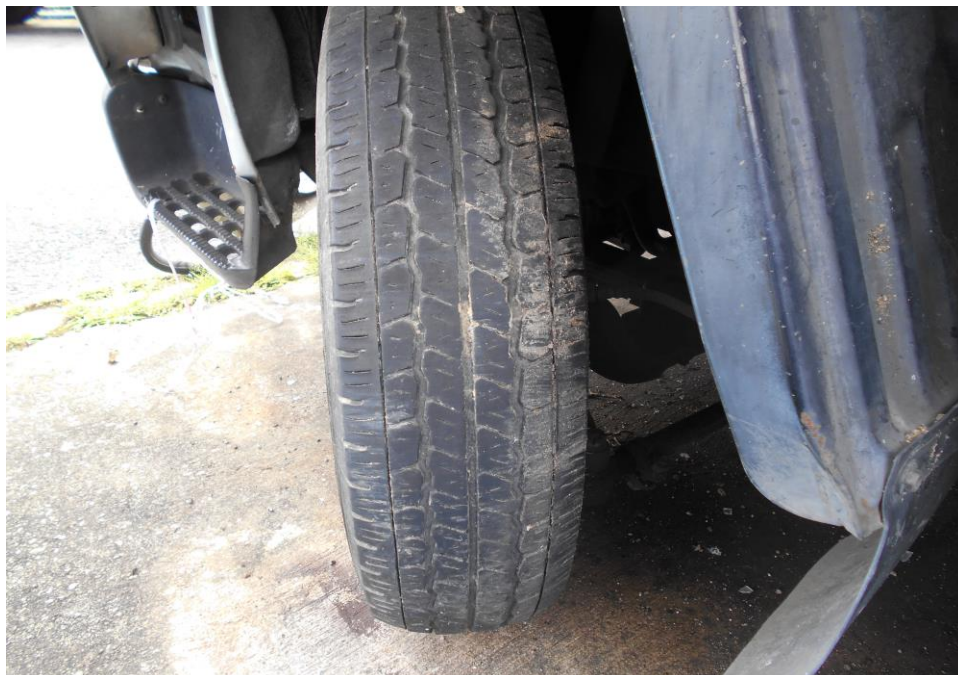
Photo 8 shows the condition of the front left tyre of the Motor Lorry, which was observed to be in serviceable condition with remaining tread depth of approximately 5mm. There was also no tear, cut or burst mark(s) on the outer and the inner sidewalls as well as across the tread of this tyre.
