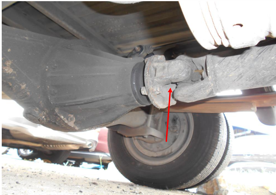
Photo 16 shows the transmission assembly (arrowed) of the Motor Lorry intact and unaffected by the collision.
