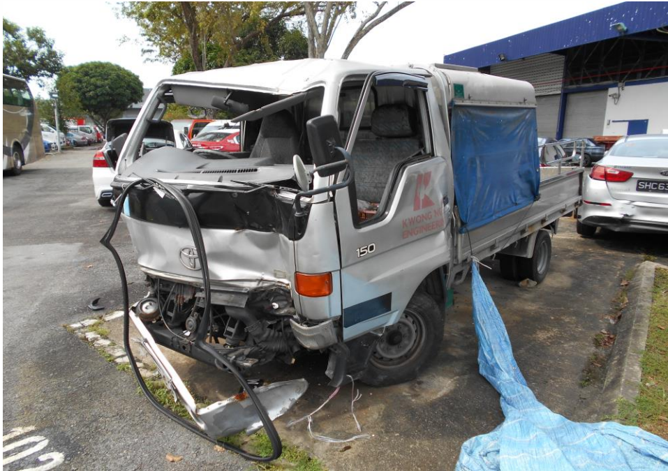
Photo 3 shows a general view of the front left portion of the Motor Lorry at the time of our inspection. The Motor Lorry was observed to have sustained extensive impact damage at its front left portion. The impact force was relatively significant, causing its entire front cabin to be pushed inwards and corrugated.
