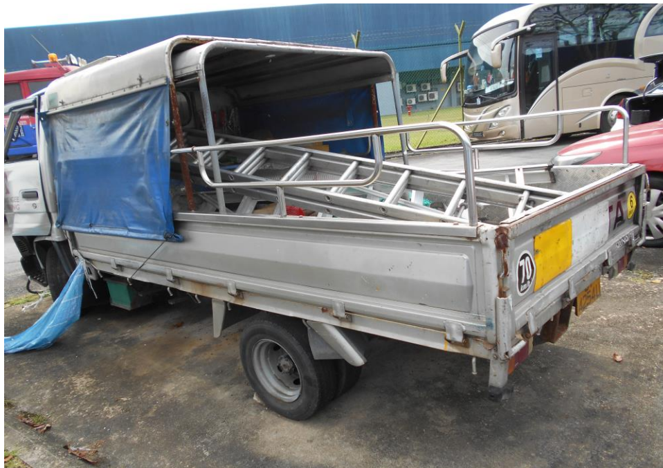
Photo 6 shows a general view of the rear right portion of the Motor Lorry at the time of our inspection. The rear portion was observed to be unaffected by the accident. The rear portion (deflated tyres & misalignment of tail lamp) was observed to be relatively affected by the accident.
