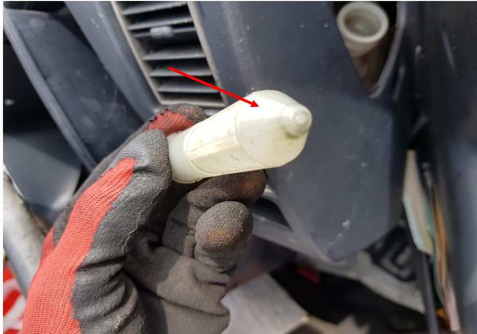
Photo 31 shows the brake fluid indicator from inside the brake reservoir. We note that it was dry at time of our examination & no brake fluid was observed touching the indicator.
