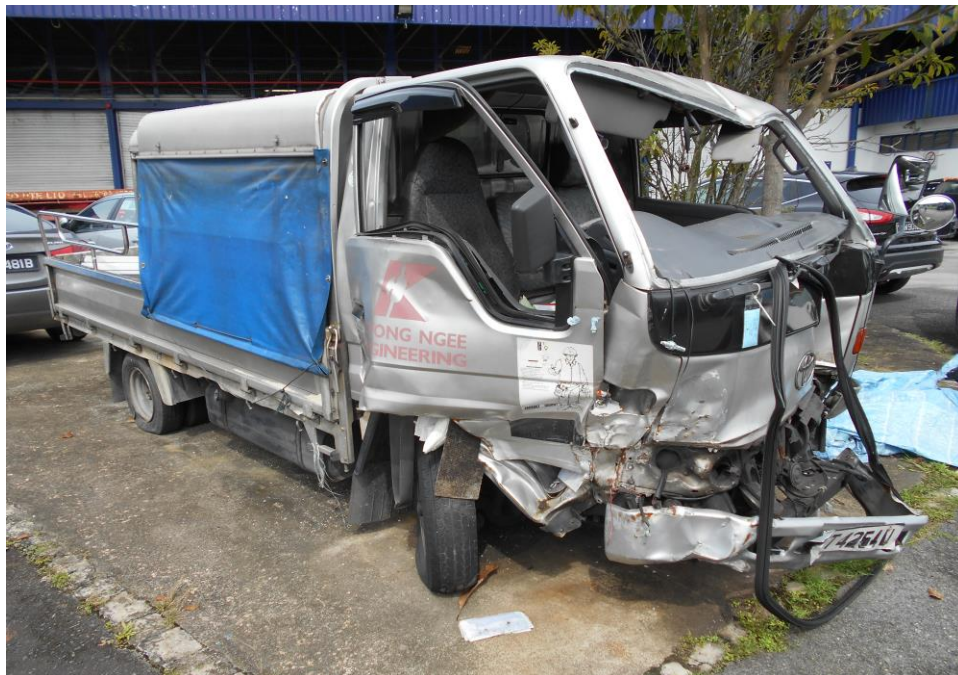
Photo 2 shows a general view of the frontal right portion of the Motor Lorry at the time of our inspection. A number of mechanical parts and components at the frontal portion were also severely damaged as a result of the accident.
