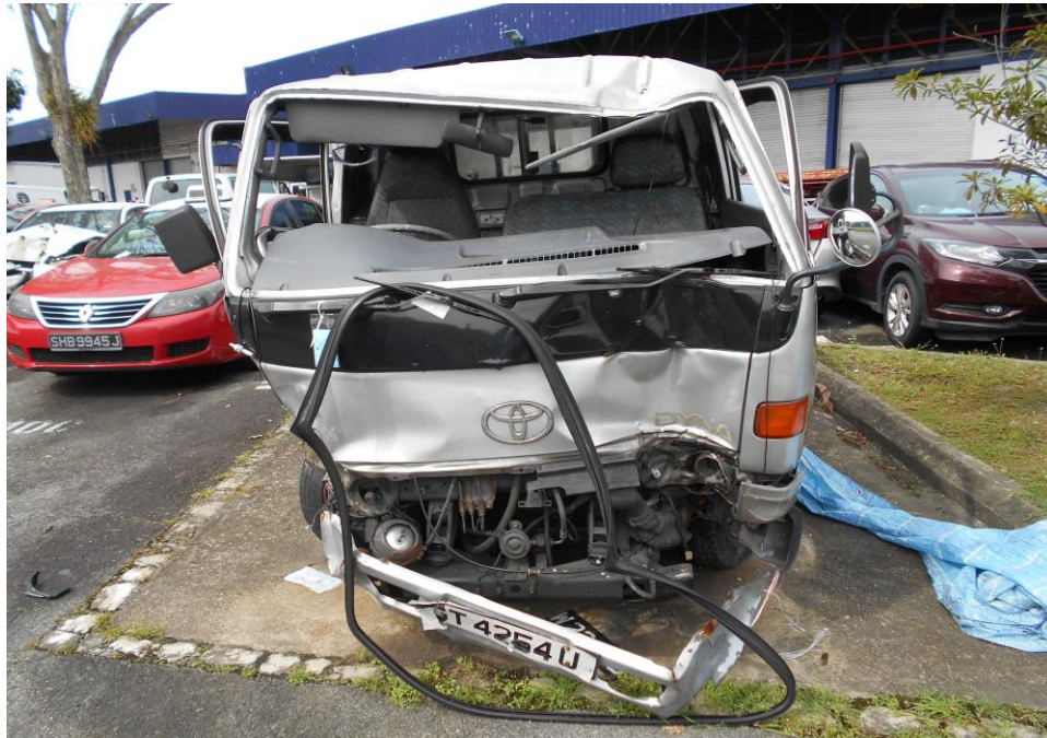
Photo 1 shows a general view of the frontal portion of the Motor Lorry at the time of our inspection. The Motor Lorry was observed to have sustained extensive impact damage at its frontal, left & right portion. The impact force was relatively significant, causing its entire front cabin to be pushed inwards and corrugated.
