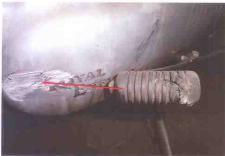
Photo 14 shows damaged engine pan due to the accident's impact collision.
