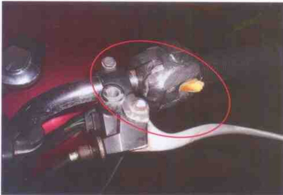
Photo 7 shows a closer view of the front left side handle bar of the Motorcycle at the time of our inspection. It was observed to be damage likely due to the accident. (Circled)
