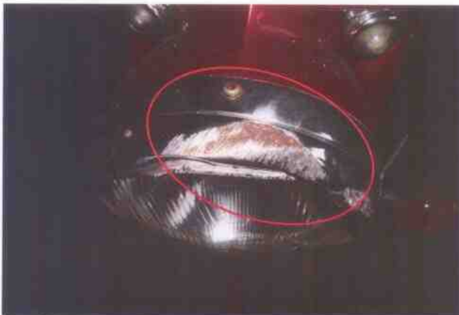
Photo 8 shows a closer view of the headlamp of the Motorcycle at the time of our inspection. It was observed to be damage likely due to the accident. (Circled)
