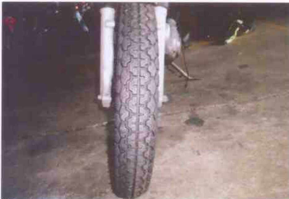
Photo 11 shows the front tyre of the Motorcycle. The front tyre was observed to be in serviceable condition with remaining tread depth of approximately 7mm. The tyre was also observed to be sufficiently inflated for vehicular operation.
