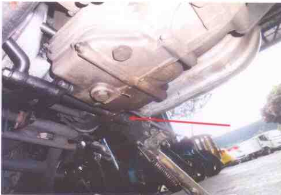
Photo 12 shows sign(s) or indication(s) of fluid leakage was observed around the underside of the engine area of the Motorcycle.
