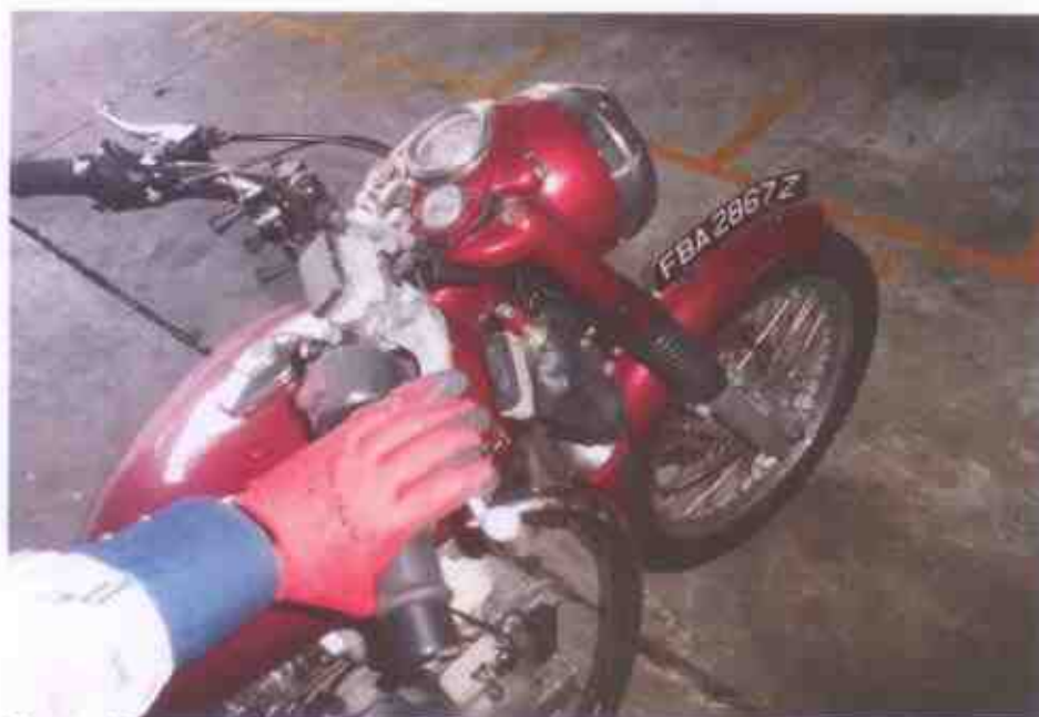
Photo 18 shows testing of the braking of the front brake in progress. There was some resistance felt (spongy like feel) upon pressing the brake lever.
