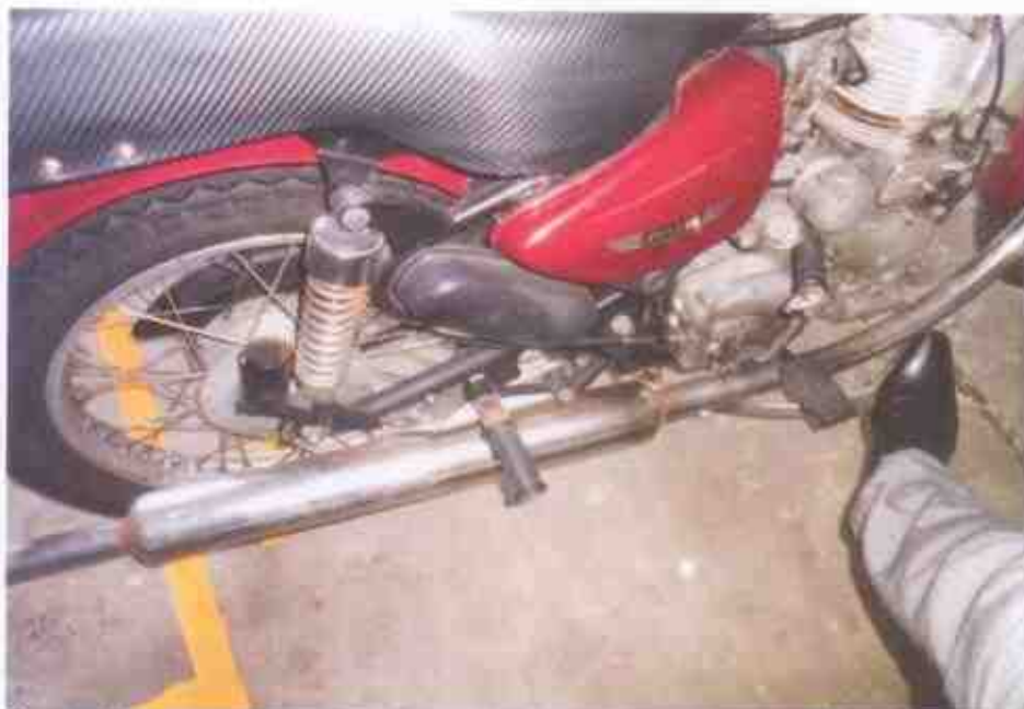
Photo 19 shows testing of the braking of the rear brake in progress. There was some resistance felt (spongy like feel) upon stepping on the brake pedal.
