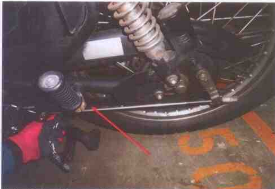
Photo 16 shows the general view of the gear train (arrowed) of the Motorcycle, which was observed to be intact with no misalignment. It was also adequately lubricated for operating purposes. Free play tension was also observed & found adequately acceptable.
