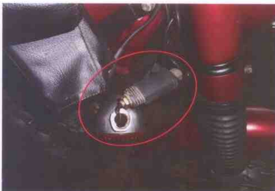
Photo 9 shows a closer view of the front right signal lamp of the Motorcycle at the time of our inspection. It was observed to be damage likely due to the accident. (Circled)
