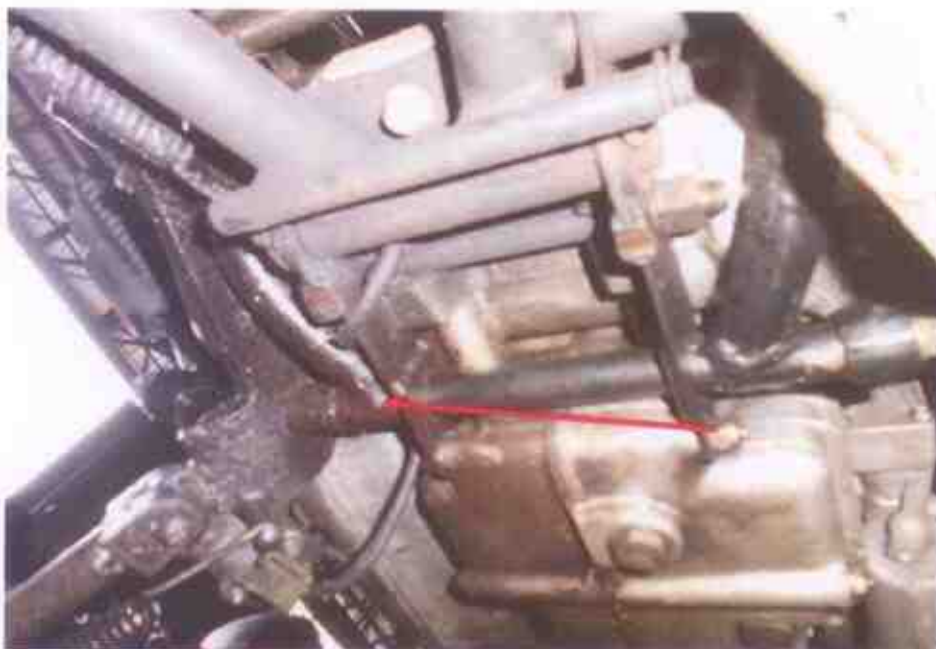
Photo 13 shows sign(s) or indication(s) of fluid leakage was observed around the underside of the engine area of the Motorcycle.
