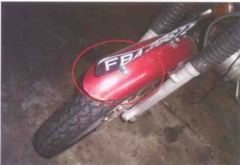
Photo 6 shows a closer view of the misaligned mudguard & dented licence plate of the Motorcycle at the time of our inspection. It was observed to have sustained with relatively minor damages due to the accident collision. (Circled)
