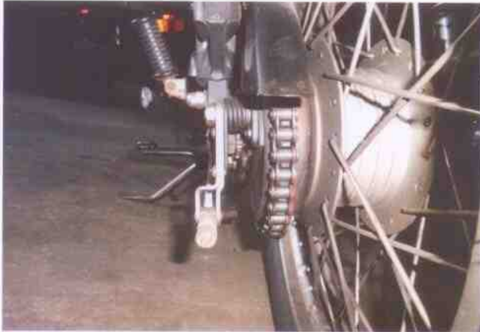
Photo 15 shows the general view of the gear train (arrowed) of the Motorcycle, which was observed to be intact with no misalignment. It was also adequately lubricated for operating purposes.
