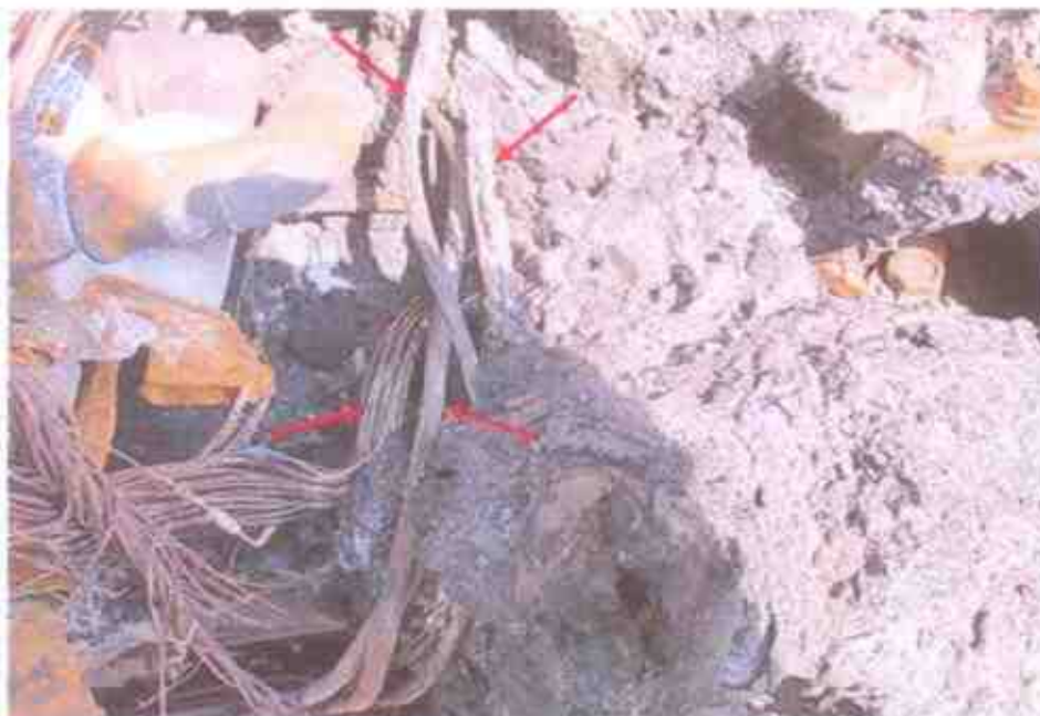
Photo 8 shows a closer view of the greenish residue found on some of the burnt stretches of original factory fitted wirings (arrowed). The presence of such greenish residue suggests occurrence of an electrical short circuit.
