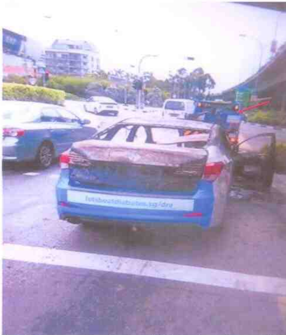
Photo 15 shows a rear view of the Insured Vehicle as it was being prepped to be towed away (arrowed). Our close examination of this photograph showed no unusual foreign material(s) and/or object(s) found on the ground in the immediate area of the slip road where the Insured Vehicle was positioned when the fire broke out.
