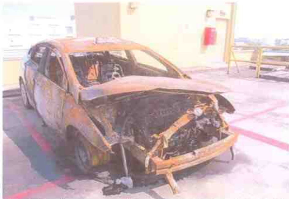
Photo 3 shows the general view of the right body of the Insured Vehicle at the time of our inspection. The Insured Vehicle was observed to have sustained extensive fire damage. Rust had accumulated all over the Insured Vehicle as a result of exposure to environmental condition for a period of time.
