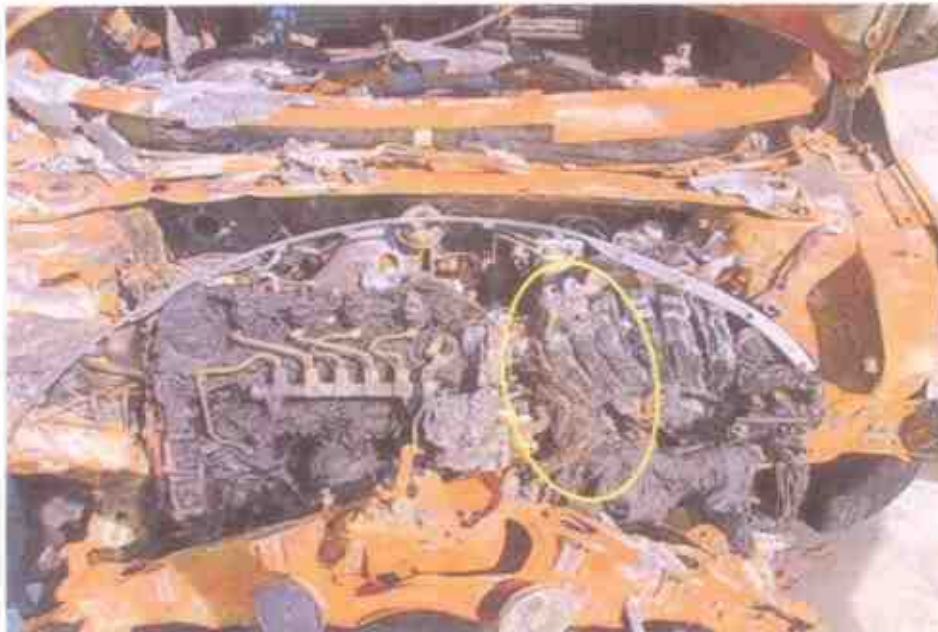
Photo 6 shows the original factory fitted wirings around the left portion of the engine compartment, which is in the immediate vicinity where the fire to the Insured Vehicle had likely started. We had found greenish residue on several burnt stretches of these wirings leading from the battery of the Insured Vehicle (circled). The presence of such greenish residue indicates internal heating of copper wires, a sign of an electrical short circuit occurring. The greenish residue is normally left behind from oxidation as a result of chemical reaction involving the copper wires.
