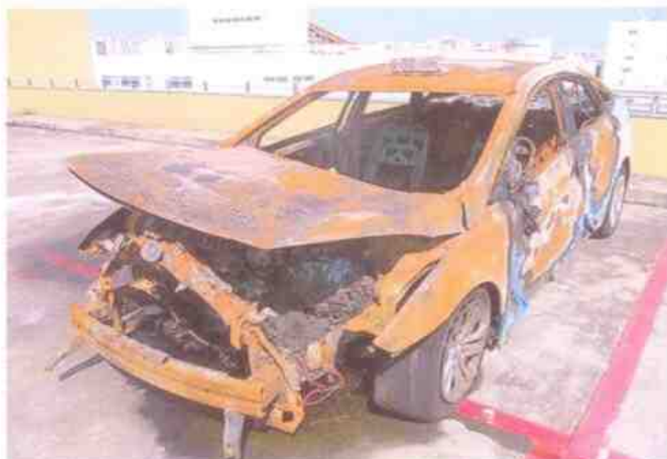
Photo 2 shows the general view of the left body of the Insured Vehicle at the time of our inspection. The Insured Vehicle was observed to have sustained extensive fire damage. Rust had accumulated all over the Insured Vehicle as a result of exposure to environmental condition for a period of time.
