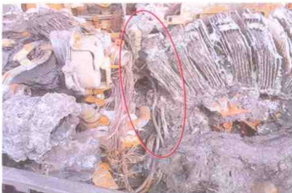
Photo 7 shows the greenish residue found on some of the burnt stretches of original factory fitted wirings (circled). The presence of such greenish residue suggests occurrence of an electrical short circuit.
