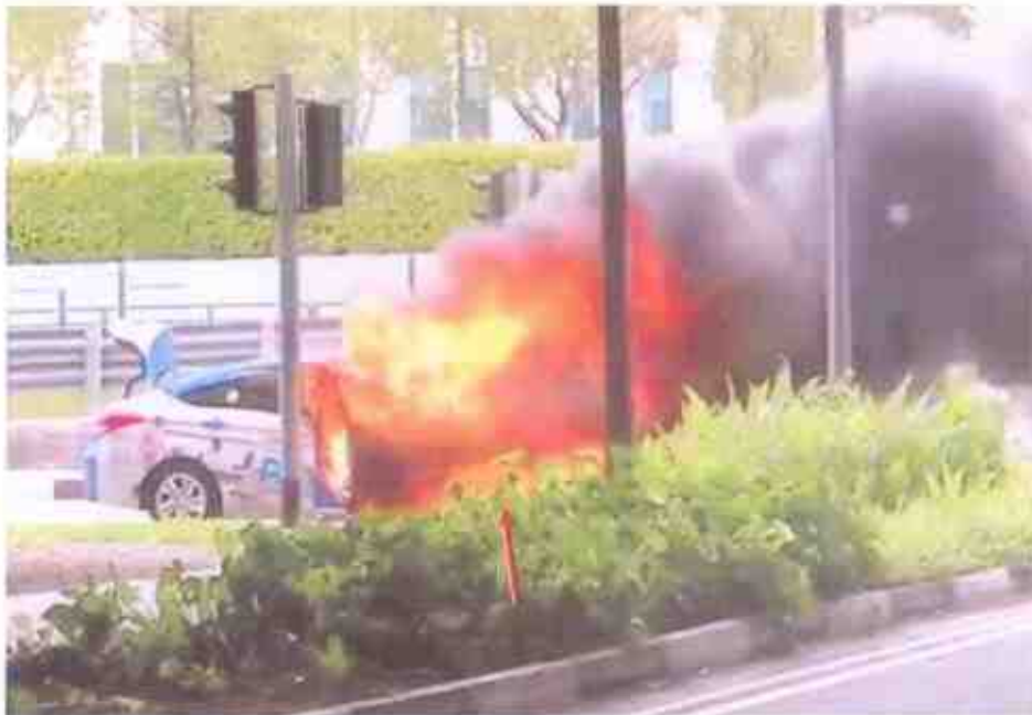
Photo 13 shows the Insured Vehicle engulfed in flames before the arrival of the SCDF. In general, the information that could be gathered from this photograph had corresponded to the events that were related to us by Mr Tay, which is the fire had started from the front portion of the Insured Vehicle (arrowed).
