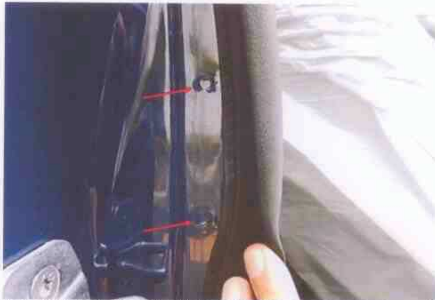
Photo 17 shows the rear right "B" pillar of the Motor Car. I did not find any weld marks other than original spot weld marks (arrowed) on the body panels of the Motor Car, indicating that there was no re-welding works carried out; and that the body panels of the Motor Car were originally fitted
