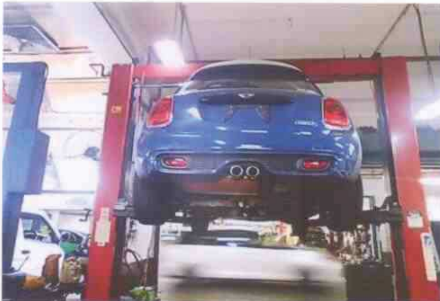
Photo 9 shows the Motor Car hoisted up for checks on its undercarriage. There was no sign(s) or indication(s) of fluid leakage and/or fluid stain(s). The undercarriage components of the Motor Car were also all observed to be intact and secured in an appropriate manner.
