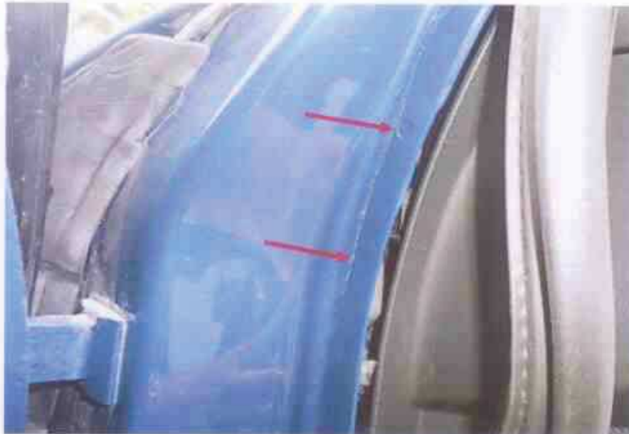
Photo 18 shows the front left "A" pillar of the Motor Car. I did not find any weld marks other than original spot weld marks (arrowed) on the body panels of the Motor Car, indicating that there was no re-welding works carried out; and that the body panels of the Motor Car were originally fitted.
