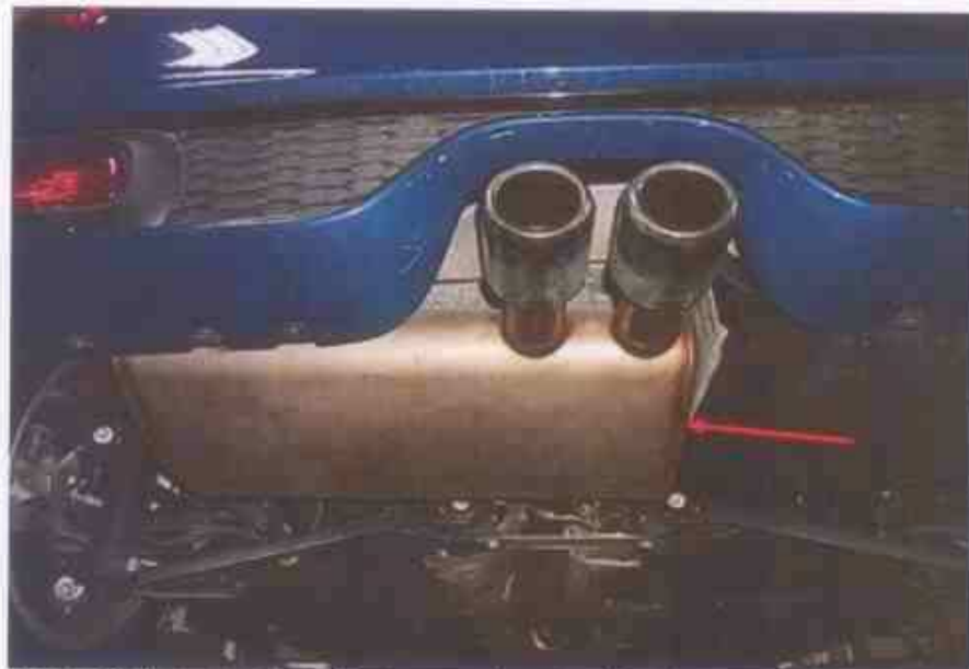
Photo 13 shows the Motor Car's rear exhaust muffler (arrowed). My examination of the Motor Car's exhaust system revealed no sign(s) or indication(s) of any cut or weld marks along its exhaust pipes and on its rear muffler.
