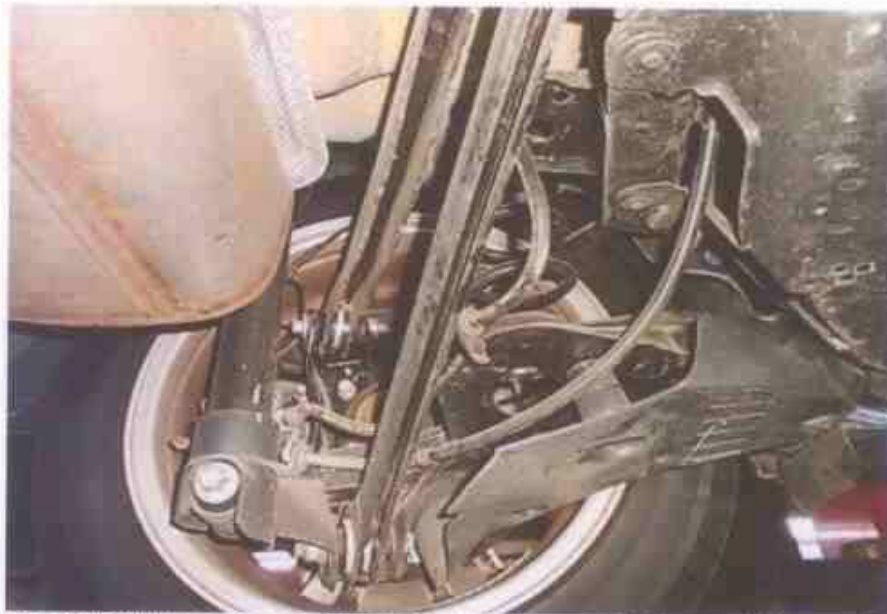
Photo 10 shows a general view of the control arms and linkages at the rear left wheel of the Motor Car. I did not observe any fluid leak and/or fluid stain on the underside of the Motor Car. All of the Motor Car's undercarriage components were observed to be intact and secured in an appropriate manner.
