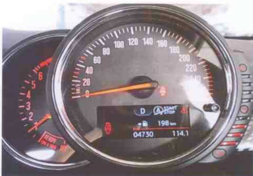
Photo 7 shows the respective warning lights no longer illuminated, indicating that there is no fault detected to the ABS, SRS, IAS, TPM and DSC lights of the Motor Car during the self-test. These electronic systems were hence in working condition at the time of my inspection.
