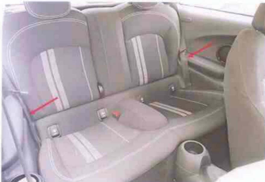
Photo 5 shows the rear seats of the Motor Car. All the seats of the Motor Car were fitted with a retractable seat belt reel (arrowed) and pre-tensioner. The seat belts were also able to be fastened to the pretension that were fitted on the side of each individual seat.
