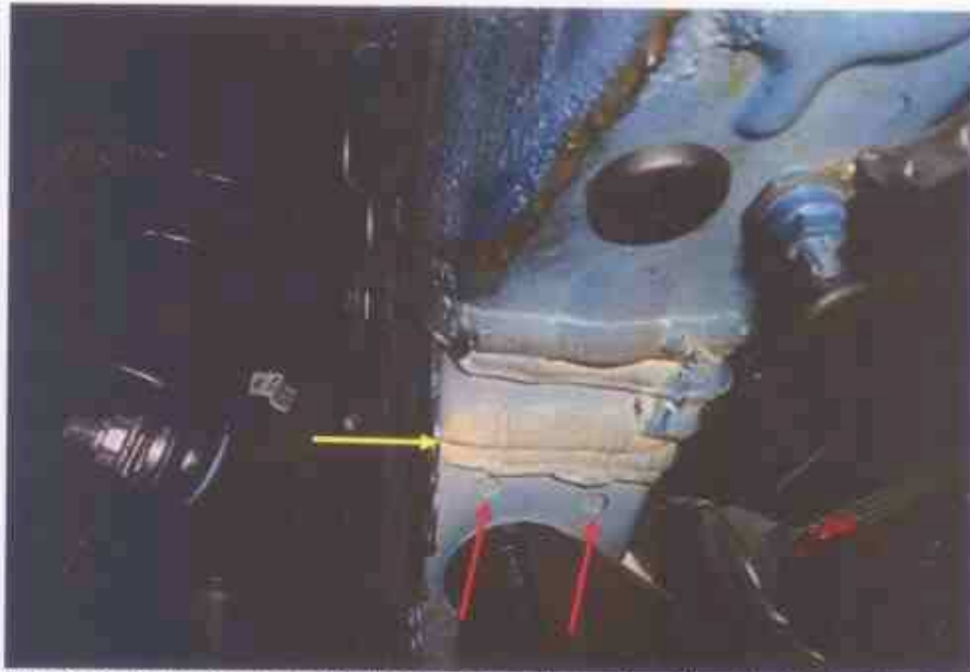
Photo 14 shows the front left chassis of the Motor Car. Visually, I did not find any weld marks other than original spot weld marks (red arrow) on the chassis body of the Motor Car. The original factory sealant (yellow arrow) at the joints along the chassis body was also untouched, indicating no work was done on the chassis body of the Motor Car and that the chassis body was originally fitted.
