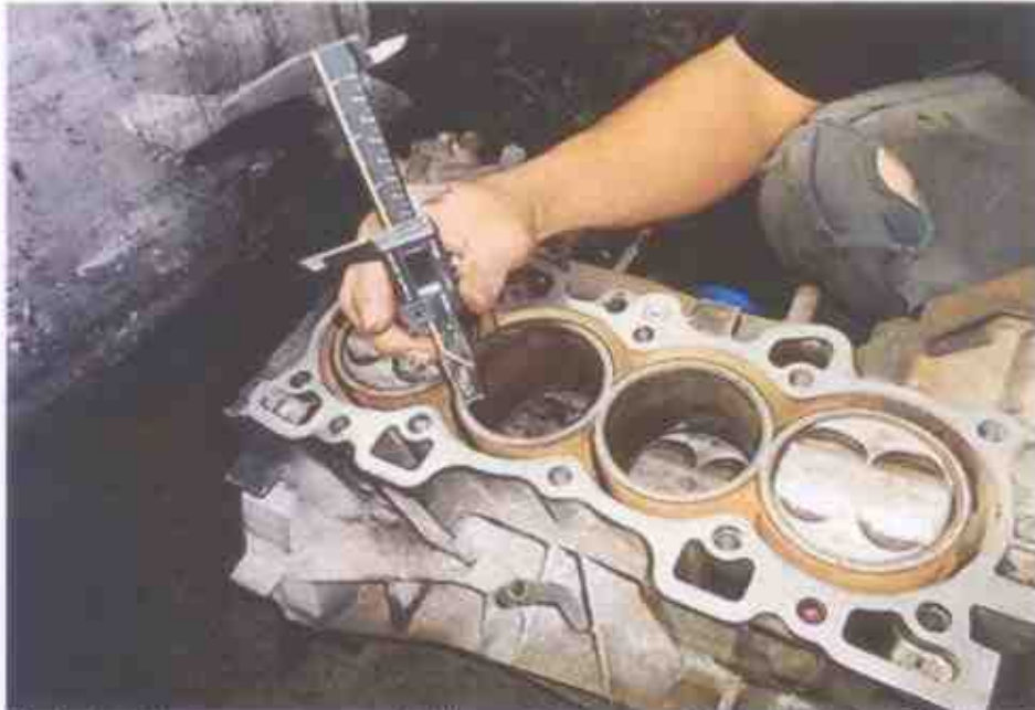
Photo 15 shows measurement of the stroke (arrowed) of cylinder 3 of the Honda engine that I had inspected. The bore and stroke measurements of the Honda engine were carried out using a digital Vernier Caliper that was calibrated before the start of measurements.
