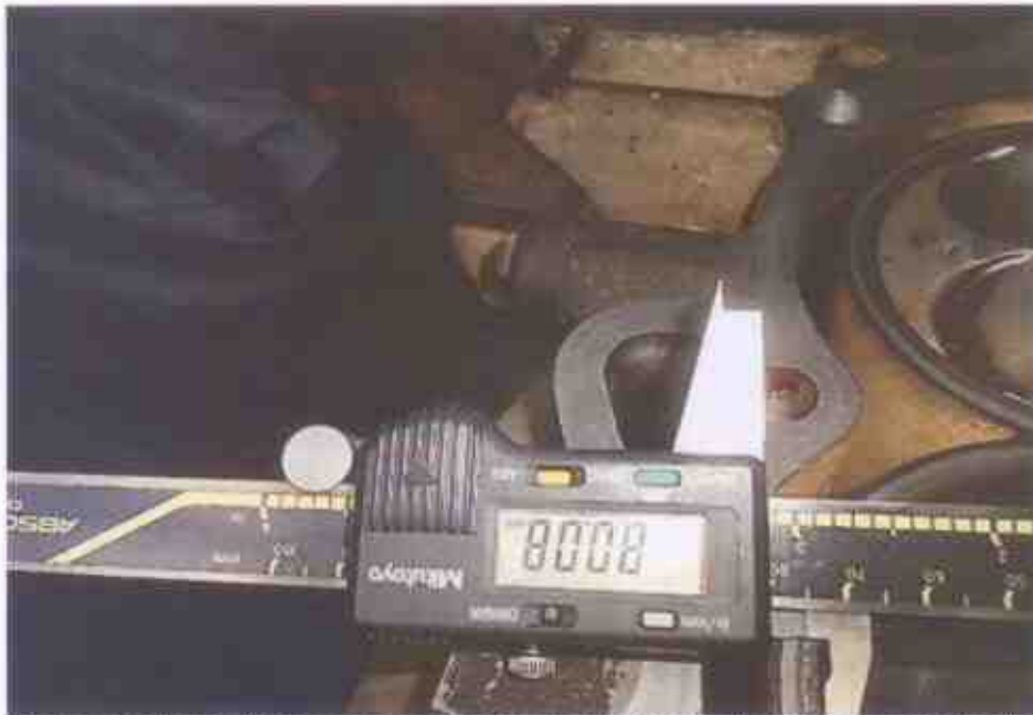
Photo 11 shows the bore measurement of cylinder 2, which was recorded to be 80.08mm.
