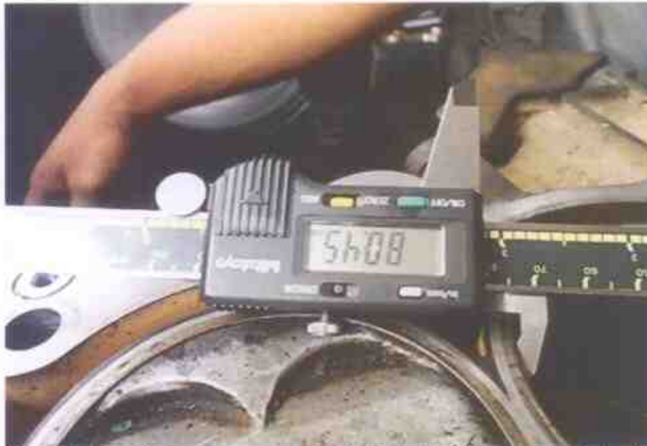
Photo 7 shows the bore measurement of cylinder 1, which was recorded to be 80.45mm.
