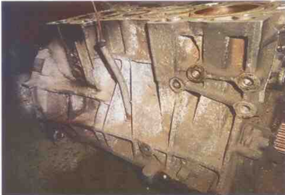
Photo 3 shows a general view of the Honda engine that I had inspected. My visual examination of the engine housing revealed the housing to be of serviceable/satisfactory condition. There was no crack and/or hole observed on the engine housing.
