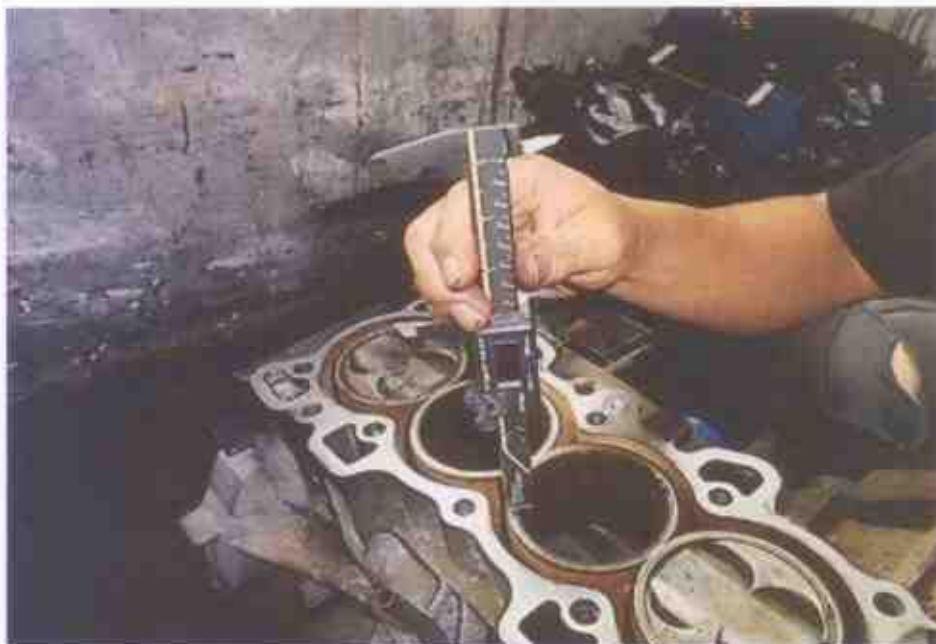
Photo 12 shows measurement of the stroke of cylinder 2 of the Honda engine that I had inspected. The bore and stroke measurements of the Honda engine were carried out using a digital Vernier Caliper, which was calibrated before the start of measurements.
