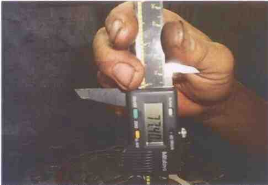
Photo 13 shows the stroke measurement of cylinder 2, which was recorded to be 77.40mm.
