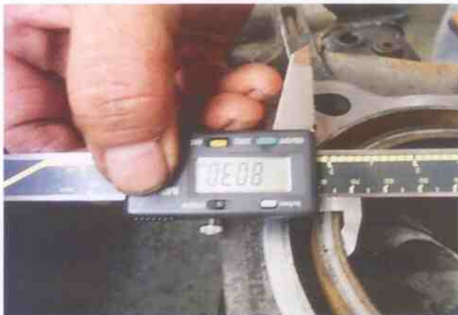
Photo 18 shows the bore measurement of cylinder 4, which was recorded to be 80.30mm.
