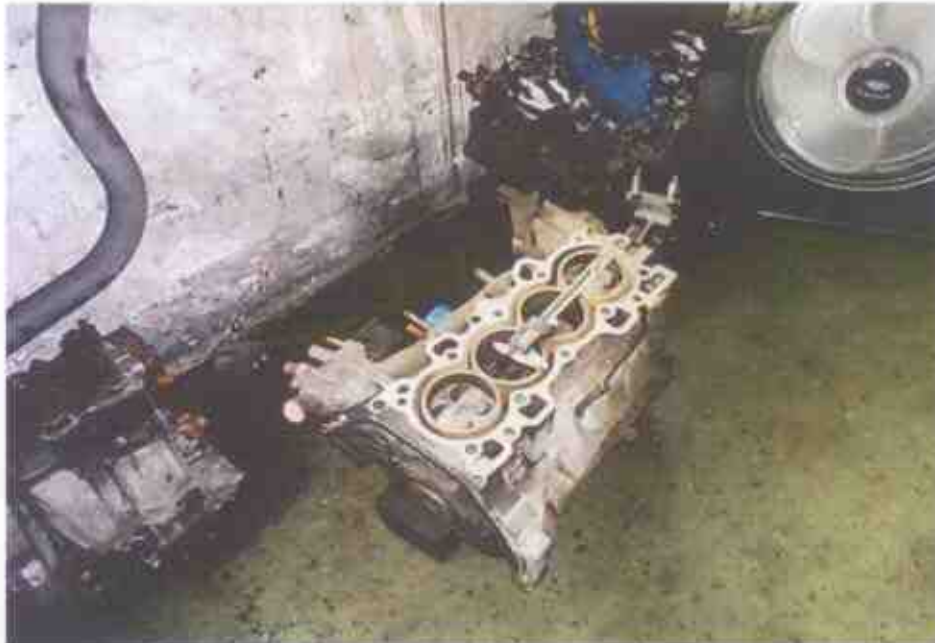
Photo 1 shows a general view of the Honda engine that I had inspected. The Honda engine was observed to be a used engine and was not fitted on any motor car. The top block of the Honda engine was separated from its bottom block. This was to enable me to carry out measurements of its cylinders, in particular the bore and stroke measurements of each cylinder, which typically can be used to determine the engine displacement or more commonly referred to as engine cc.
