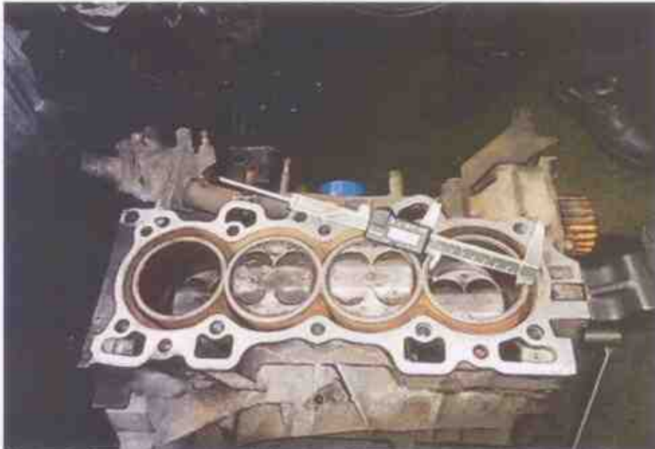
Photo 5 shows the bottom block of the Honda engine and the digital Vernier Caliper that was used to measure the bore and stroke of the Honda engine. The digital Vernier Caliper was calibrated before the start of the measurements.
