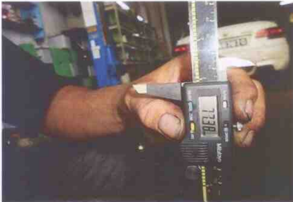
Photo 9 shows the stroke measurement of cylinder 1, which was recorded to be 77.38mm.
