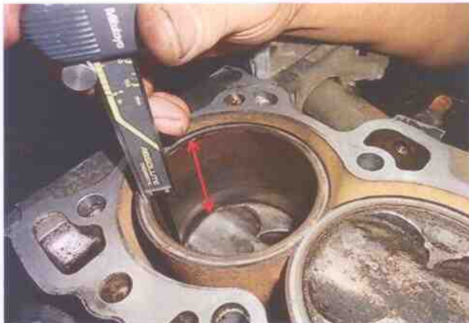
Photo 19 shows measurement being carried out to the stroke (arrowed) of cylinder 4 of the Honda engine. The bore and stroke measurements of the Honda engine were carried out using a digital Vernier Caliper that was calibrated before the start of measurements.
