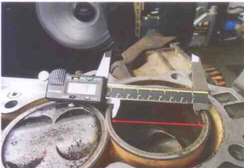
Photo 6 shows measurement being carried out to the bore (arrowed) of cylinder 1 of the Honda engine. The bore measurement of cylinder 1 was recorded to be 80.45mm.
