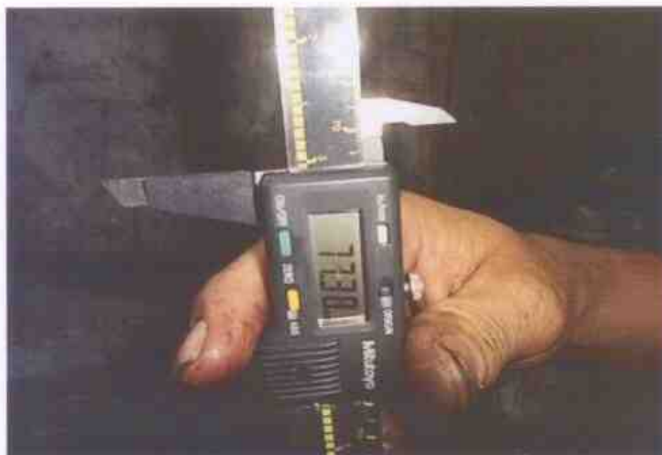
Photo 20 shows the stroke measurement of cylinder 4, which was recorded to be 77.38mm.
