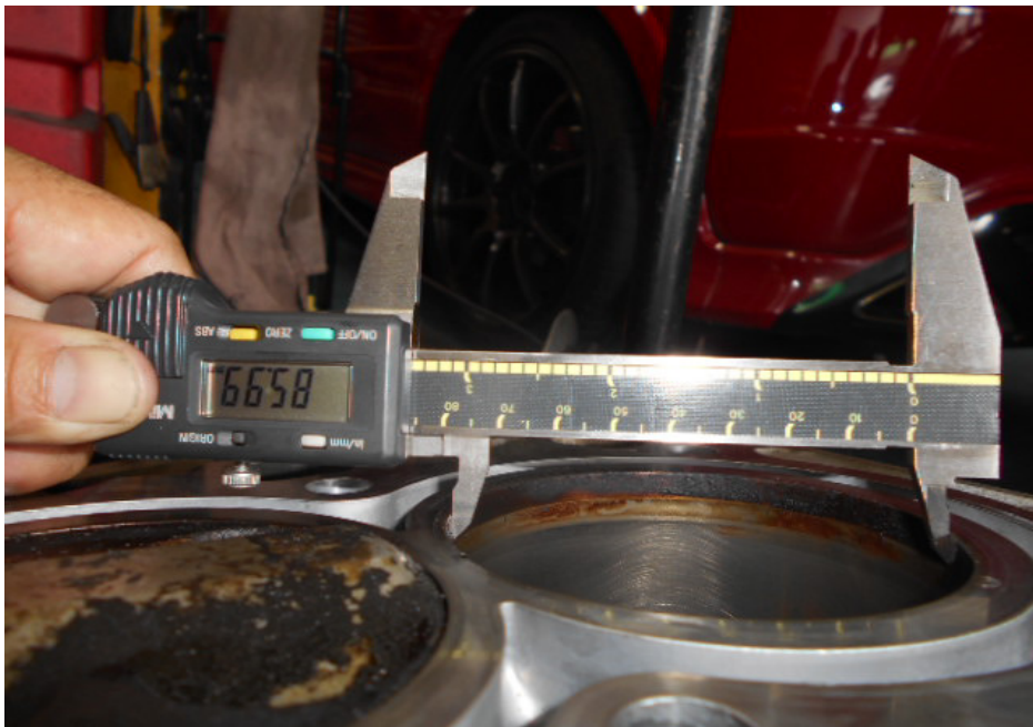
Photo 18 shows the bore measurement of cylinder 4, which was recorded to be 85.99mm.
