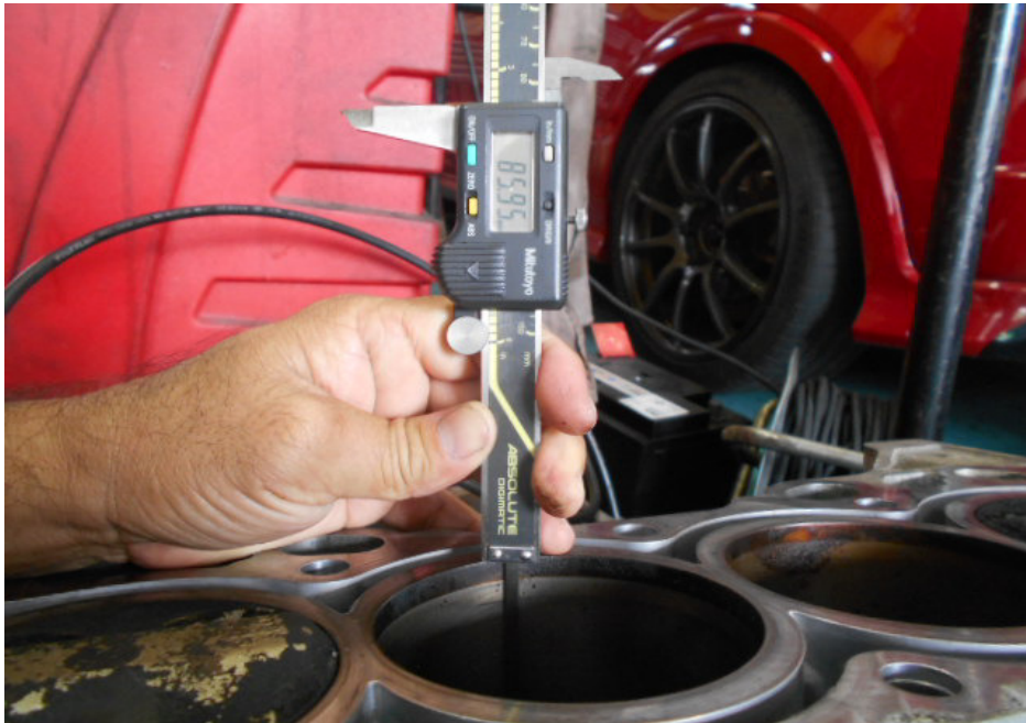
Photo 13 shows the stroke measurement of cylinder 2, which was recorded to be 85.95mm.
