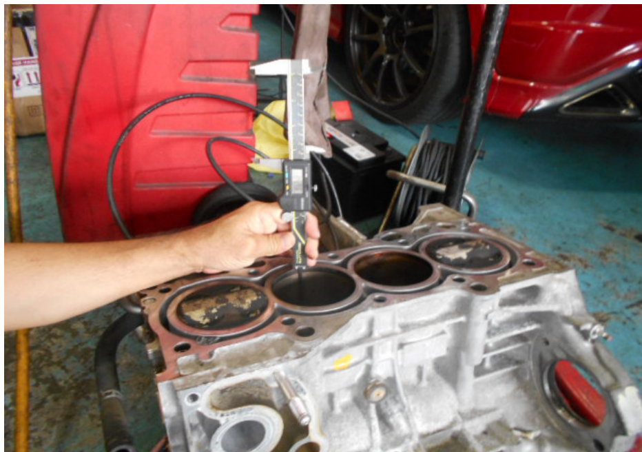
Photo 12 shows measurement of the stroke for cylinder 2 of the Honda engine that I had inspected. The measurement was carried out using a digital Vernier Caliper that was calibrated at the start of the measurements.
