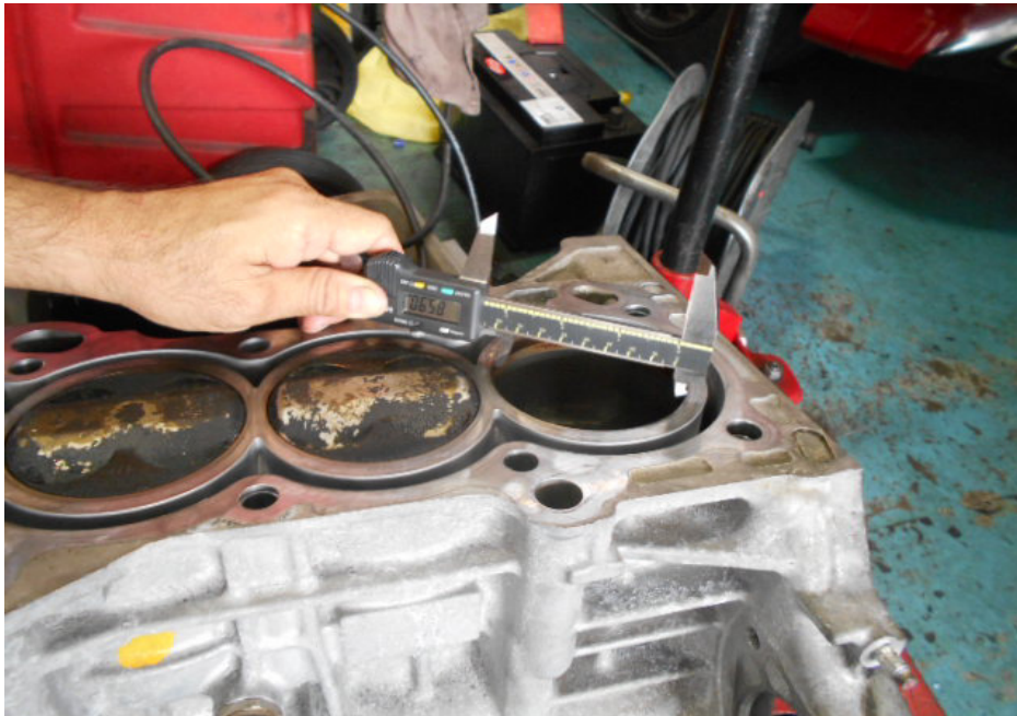
Photo 17 shows measurement being carried out to the bore of cylinder 4 of the Honda engine. The bore and stroke measurements of the Honda engine were carried out using a digital Vernier Caliper that was calibrated at the start of the measurements.
