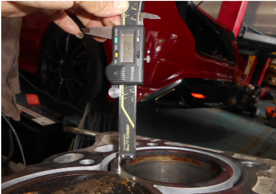
Photo 19 shows measurement being carried out to the stroke of cylinder 4 of the Honda engine. The bore and stroke measurements of the Honda engine were carried out using a digital Vernier Caliper.
