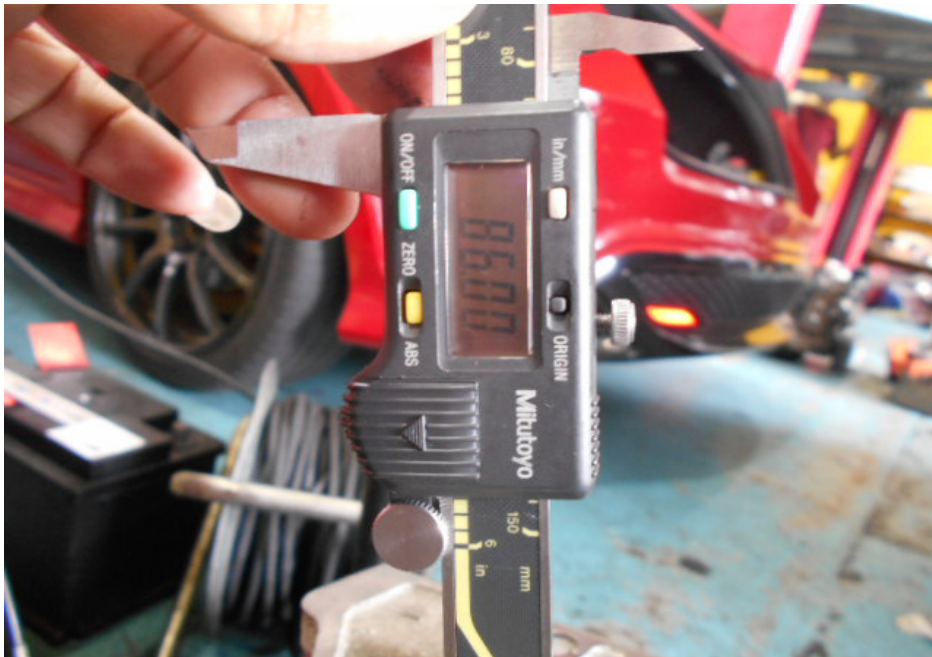
Photo 20 shows the stroke measurement of cylinder 4, which was recorded to be 86.00mm.
