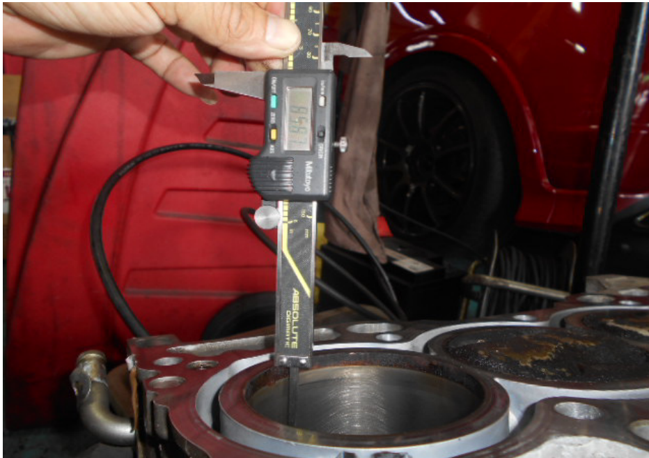
Photo 7 shows measurement being carried out to the stroke of cylinder 1 of the Honda engine. The bore and stroke measurements of the Honda engine were carried out using a digital Vernier Caliper.
