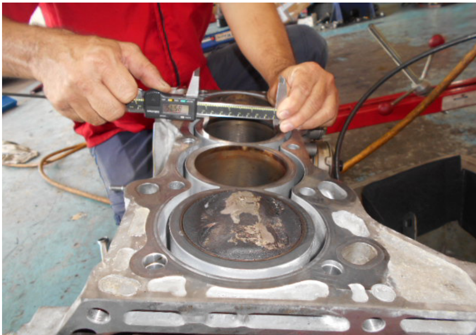
Photo 10 shows measurement being carried out to the bore of cylinder 2 of the Honda engine. The bore and stroke measurements of the Honda engine were carried out using a digital Vernier Caliper.
