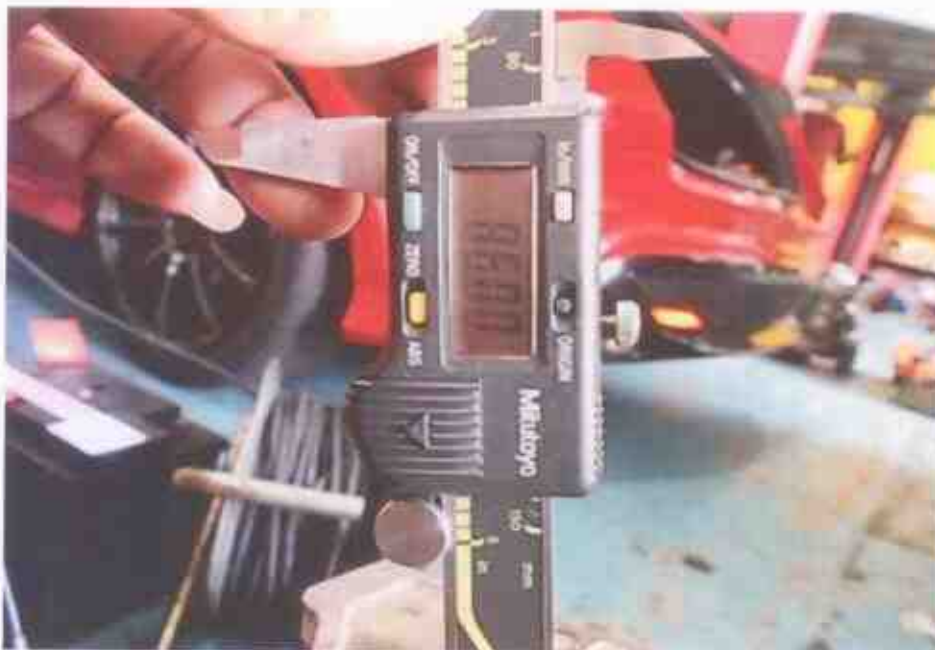
Photo 20 shows the stroke measurement of cylinder 4, which was recorded to be 85.00mm.
