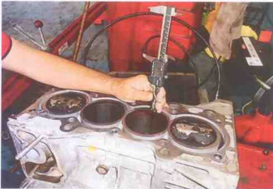
Photo 15 shows measurement of the stroke for cylinder 3 of the Honda engine that I had inspected. The measurement was carried out using a digital Vernier Caliper that was calibrated at the start of the measurements.
