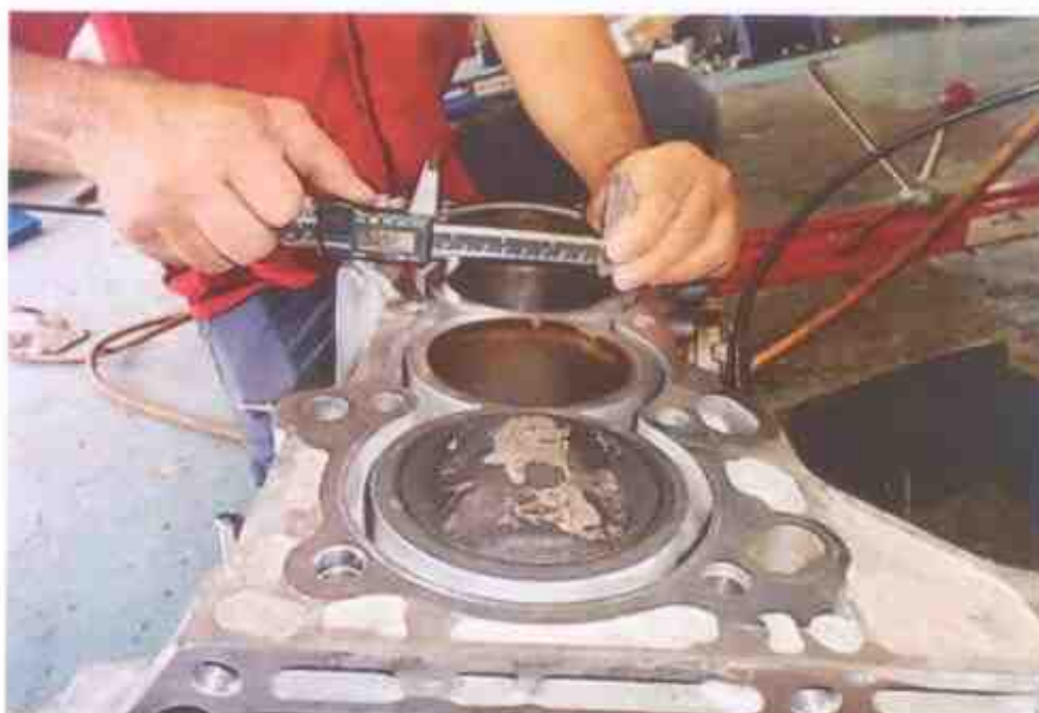
Photo 10 shows measurement being carried out to the bore of cylinder 2 of the Honda engine. The bore and stroke measurements of the Honda engine were carried out using a digital Vernier Caliper.
