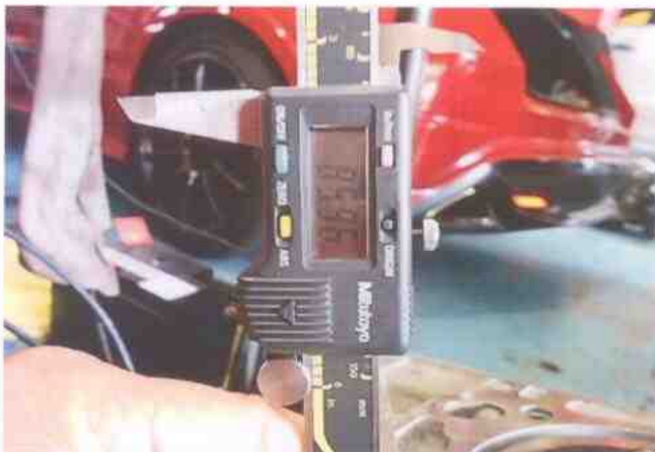
Photo 16 shows the stroke measurement of cylinder 3, which was recorded to be 85.96mm.
