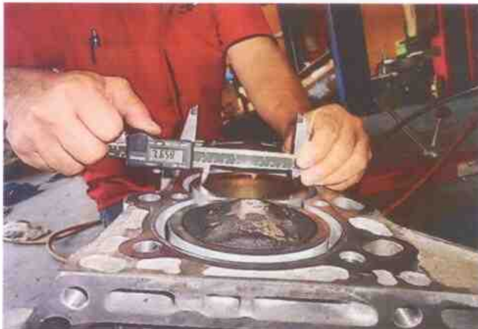
Photo 14 shows measurement being carried out to the bore of cylinder 3 of the Honda engine. The bore and stroke measurements of the Honda engine were carried out using a digital Vernier Caliper. The bore measurement of cylinder 3, which was recorded to be 85.97mm.
