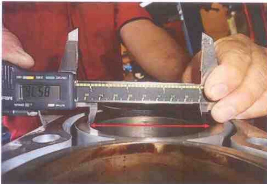
Photo 11 shows the bore measurement of cylinder 2, which was recorded to be 85.76mm.
