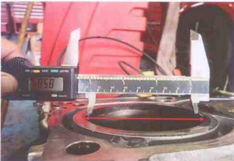
Photo 6 shows measurement being carried out to the bore of cylinder 1 of the Honda engine. The bore and stroke measurements of the Honda engine were carried out using a digital Vernier Caliper. The bore measurement of cylinder 1 was recorded to be 85.84mm.
