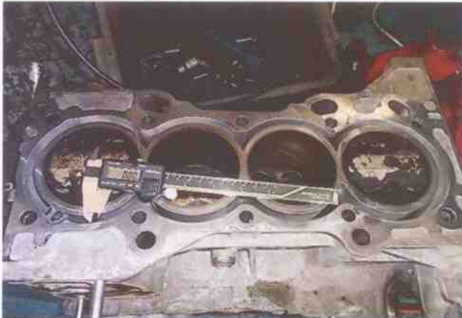
Photo 5 shows the bottom block of the Honda engine with its top block removed for me to carry out measurements of its cylinders, in particular the bore and stroke measurements of each cylinder, which typically can be used to determine the engine displacement or more commonly referred to as engine cc. The measurements were carried out using a digital Vernier Caliper that was calibrated at the start of the measurements.
