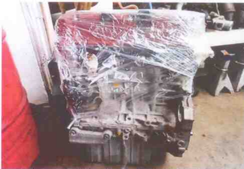
Photo 1 shows a general view of the Honda engine that I had inspected. The Honda engine was observed to be a used engine and was not fitted on any motor car. It was also observed to be a complete assembly with all mechanical parts still intact, within the engine housing. There was no crack and/or hole observed on the engine housing.
