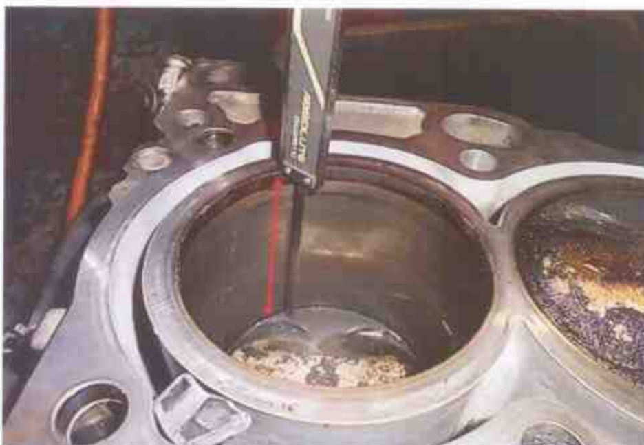
Photo 8 shows measurement being carried out to the stroke of cylinder 1 of the Honda engine. The bore and stroke measurements of the Honda engine were carried out using a digital Vernier Caliper that was calibrated at the start of the measurements.
