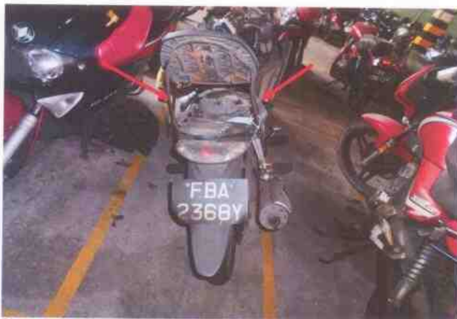
Photo 3 shows a general view of the rear left body of the Motorcycle at the time of our inspection. The Motorcycle was observed to have sustained minor damages at the rear portion which includes bent rear box rack as a result of the accident.
