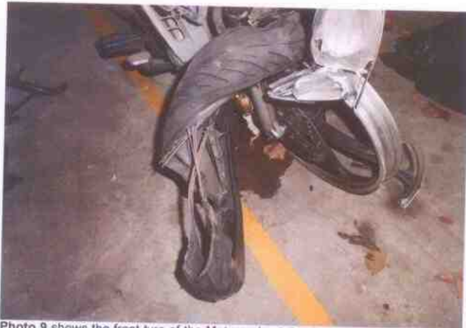
Photo 9 shows the front tyre of the Motorcycle at the time of our inspection. The front tyre was observed to be dislodged from the broken wheel rim & deflated due to the accident's impact collision. However, the tread pattern of the front tyre was clearly visible. We did observe that the front tyre was torn as a result of the accident.
