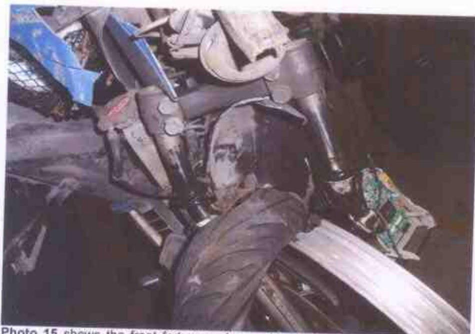
Photo 15 shows the front fork was observed to be buckled as a result of the accident. Hence, we are not able to conduct any tests on the steering system of the Motorcycle.
