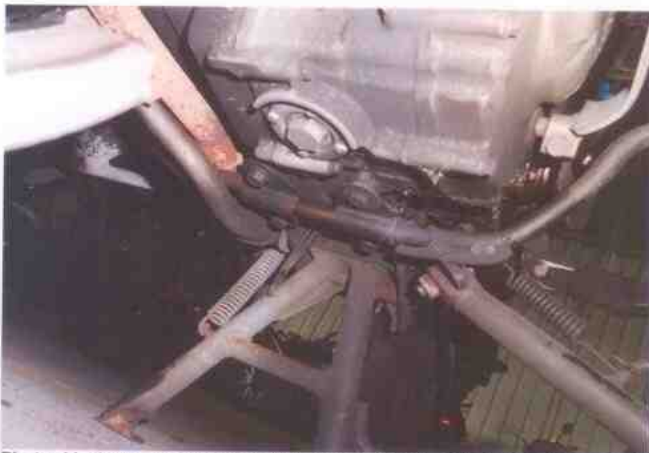
Photo 11 shows no sign(s) or indication(s) of fluid leak observed around the engine area of the Motorcycle.
