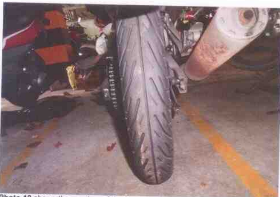
Photo 10 shows the rear tyre of the Motorcycle at the time of our inspection. The rear tyre was observed to be in serviceable condition with remaining tread depth of approximately 3mm. It was also sufficiently inflated for vehicular operation.
