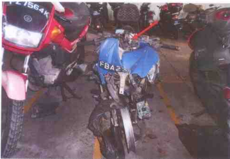
Photo 2 shows a general view of the front body of the Motorcycle at the time of our inspection. The Motorcycle was observed to be sustained with relatively extensive impact due to the accident collision. Amongst the body parts damaged was its handle bar (arrowed), which was observed to be dislodged.
