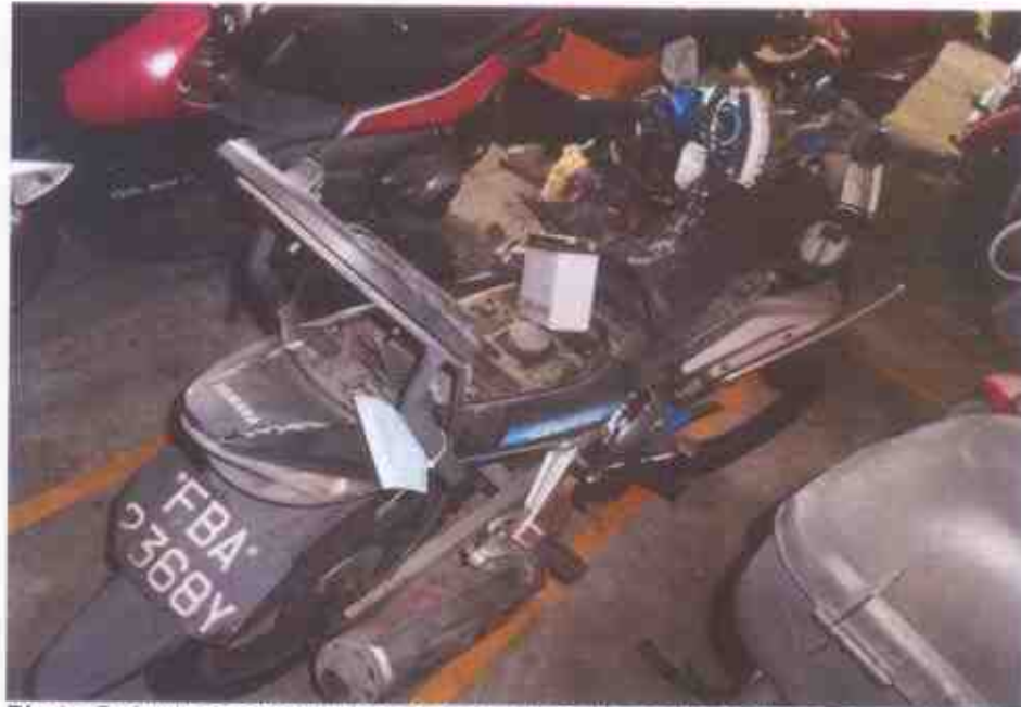
Photo 5 shows a general view of the frontal right portion of the Motorcycle at the time of our inspection. The Motorcycle was observed to be sustained relatively extensive impact which includes dislodged seat assembly due to the accident collision.
