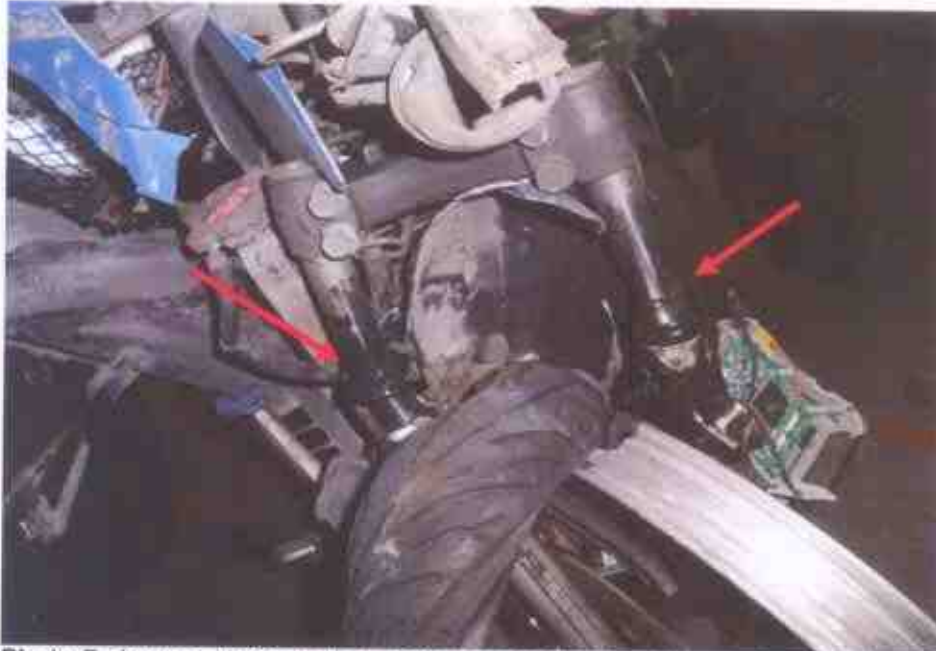
Photo 7 shows a close-up view of the front fork of the Motorcycle at the time of our inspection. It was observed to have sustained with relatively extensive impact due to the accident collision.
