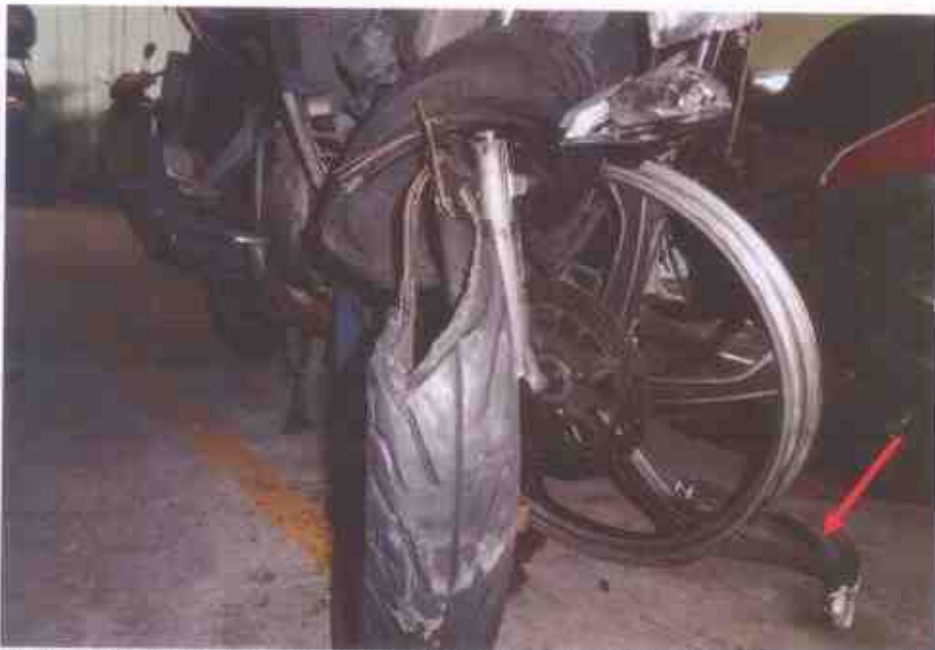
Photo 8 shows a close-up view of the broken alloy rim of the Motorcycle at the time of our inspection. The Motorcycle alloy rim was observed to be broken due to the accident collision.
