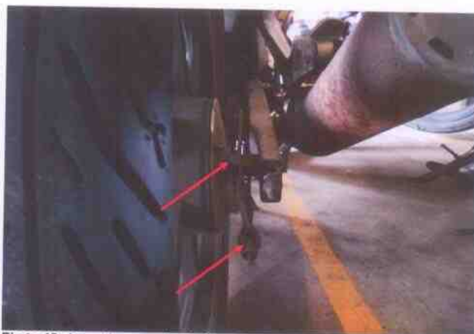
Photo 18 shows the rear wheel of the Motorcycle. The type of brake system for the rear wheel was of mechanical type, controlled by the brake foot pedal of the Motorcycle. Our checks of the cable (arrowed), spring and drum, which are all part of the components in the rear brake system of the Motorcycle reveal all to be intact and without damage.
