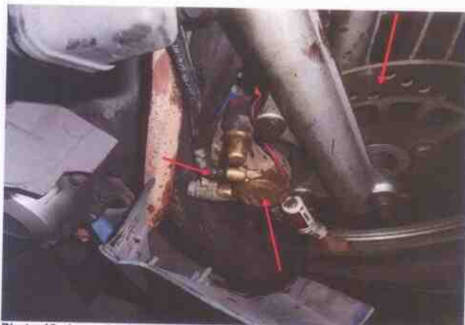
Photo 16 shows the front brake calliper, front brake disc and brake pad of the Motorcycle (arrowed), which are all part of the components in the front brake system of the Motorcycle. Our visual checks of these various components had revealed that there's brake fluid leakage as a result of the accident.
