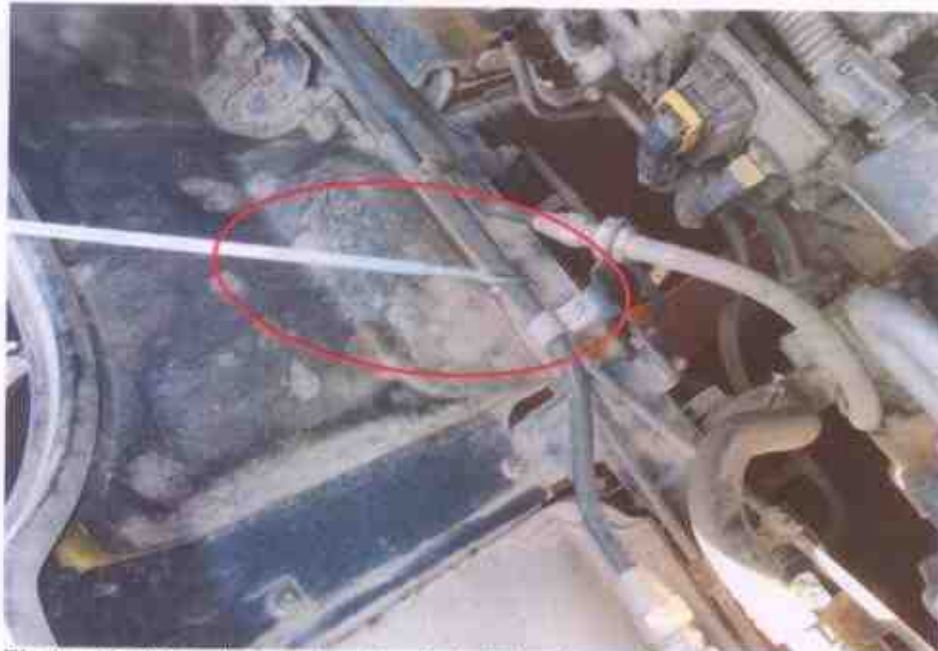
Photo 16 shows the engine dip stick of the Tipper Truck at the time of our inspection. The engine oil was observed to be of sufficient level and without any visible contamination (circled).
