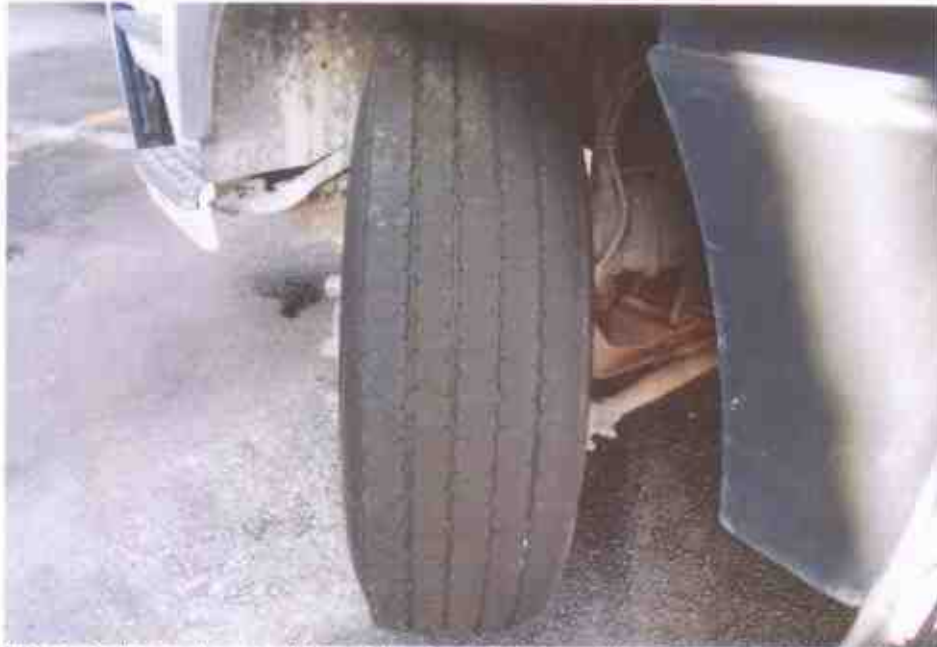
Photo 7 shows the condition of the front left tyre of the Tipper Truck, which was observed to be in serviceable condition with remaining tread depth of approximately 6mm. The tyre, which was wrapped around standard alloy wheel rim, was also observed to be sufficiently inflated for vehicular operation.
