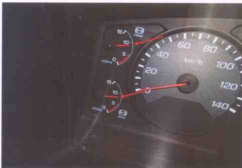
Photo 19 shows the compressed air meters for braking system. This shows that there's no dropped of pressure. Hence, revealed that no air leakage at the time of our inspection.
