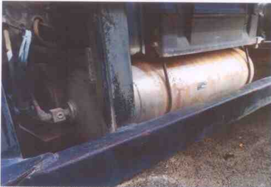
Photo 22 shows the air pressure tank of the Tipper Truck. It was observed to be unaffected by the accident. No air leakage was found at time of our inspection.
