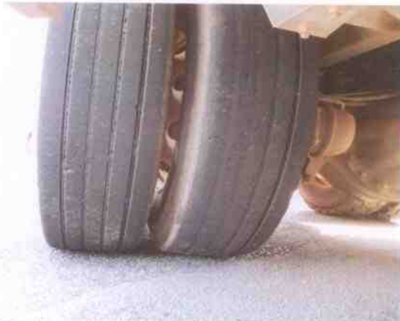
Photo 10 shows the condition of the centre right tyres of the Tipper Truck, which were observed to be in serviceable condition with remaining tread depth of approximately 4mm.
