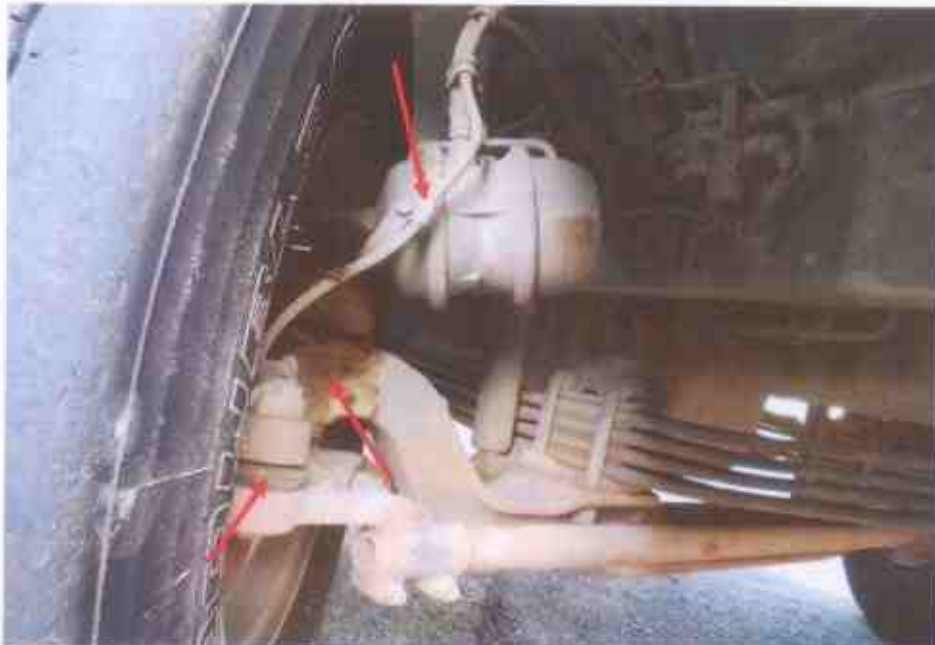
Photo 17 shows the various undercarriage components at the front left wheel of the Tipper Truck, in particular the steering tie rod end (arrowed). The various undercarriage components of the Tipper Truck were all found to be intact without any visible damage. There was also no sign of fluid stain(s) observed on the various undercarriage components.
