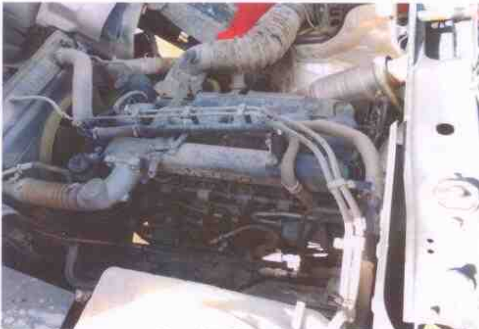
Photo 13 shows a general view of the Tipper Truck's engine compartment, which was accessed by lifting the front cabin of the Tipper Truck. The various parts and components inside the engine compartment were unaffected by the accident. There was also no sign(s) or indication(s) of fresh fluid leakage and/or fluid stain within the engine.
