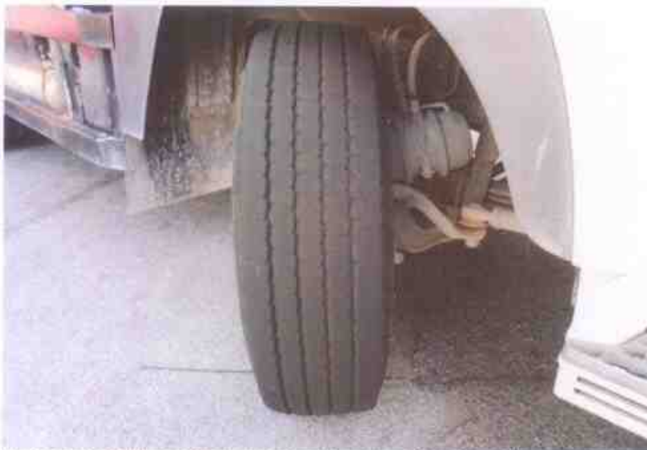
Photo 8 shows the condition of the front right tyre of the Tipper Truck, which was observed to be in serviceable condition with remaining tread depth of approximately 7mm. The tyre, which was wrapped around standard alloy wheel rim, was also observed to be sufficiently inflated for vehicular operation.
