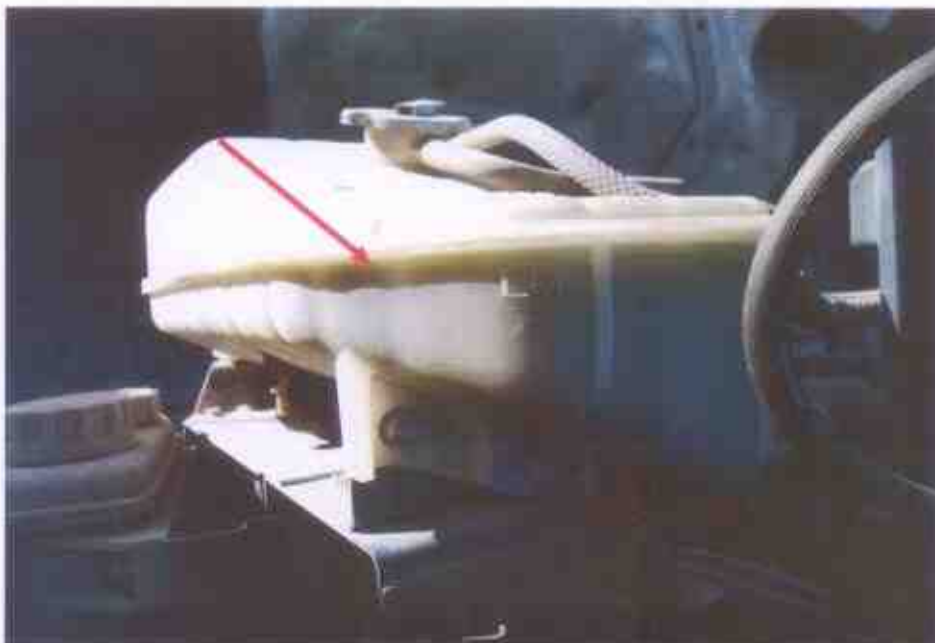
Photo 15 shows the engine coolant reservoir of the Tipper Truck at the time of our inspection. The engine coolant was observed to be of sufficient level and without any visible contamination (arrowed).
