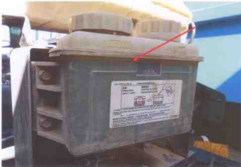
Photo 14 shows the power steering fluid reservoir of the Tipper Truck at the time of our inspection. It was observed to be of sufficient level and without any visible contamination (arrowed).
