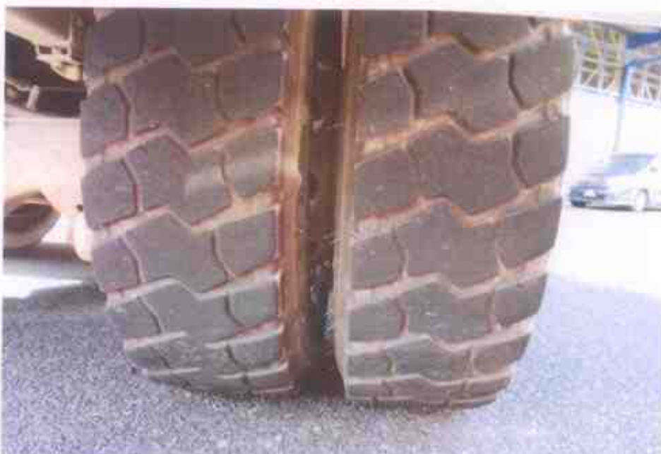
Photo 12 shows the condition of the rear right tyres of the Tipper Truck, which were observed to be in serviceable condition with remaining tread depth of approximately 8mm.
