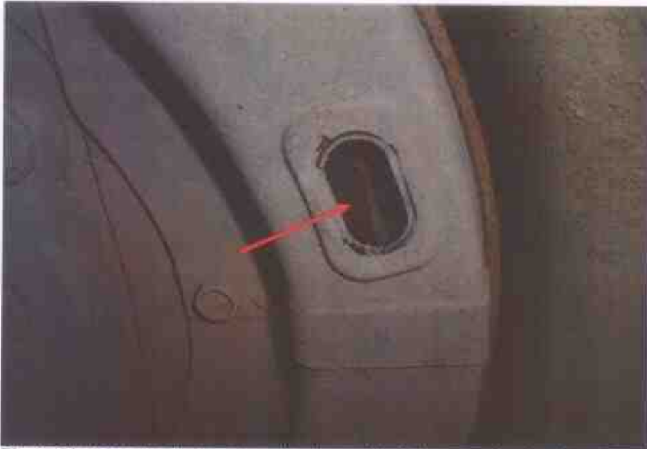
Photo 21 shows the brake shoes (brake pads) at the rear wheels of the Tipper Truck revealed that the brake shoes (brake pads) were in serviceable condition with sufficient frictional material for operational purposes.
