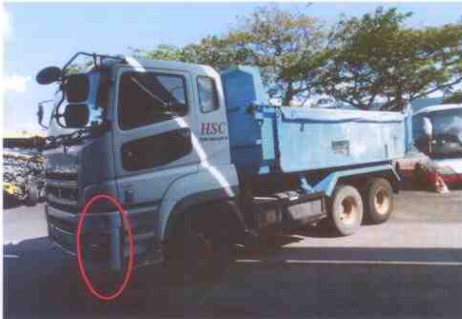
Photo 3 shows a general view of the front portion of the Tipper Truck at the time of our inspection. The Tipper Truck was observed to have sustained minor impact at its front left bumper. Only stain marks was observed on the front left bumper as a result of the accident.
