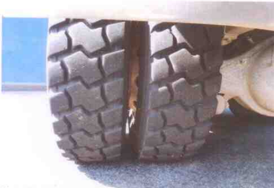
Photo 11 shows the condition of the rear left tyres of the Tipper Truck, which was observed to be in serviceable condition with remaining tread depth of approximately 9mm. The tyres, which were wrapped around standard alloy wheel rim, were also observed to be sufficiently inflated for vehicular operation.
