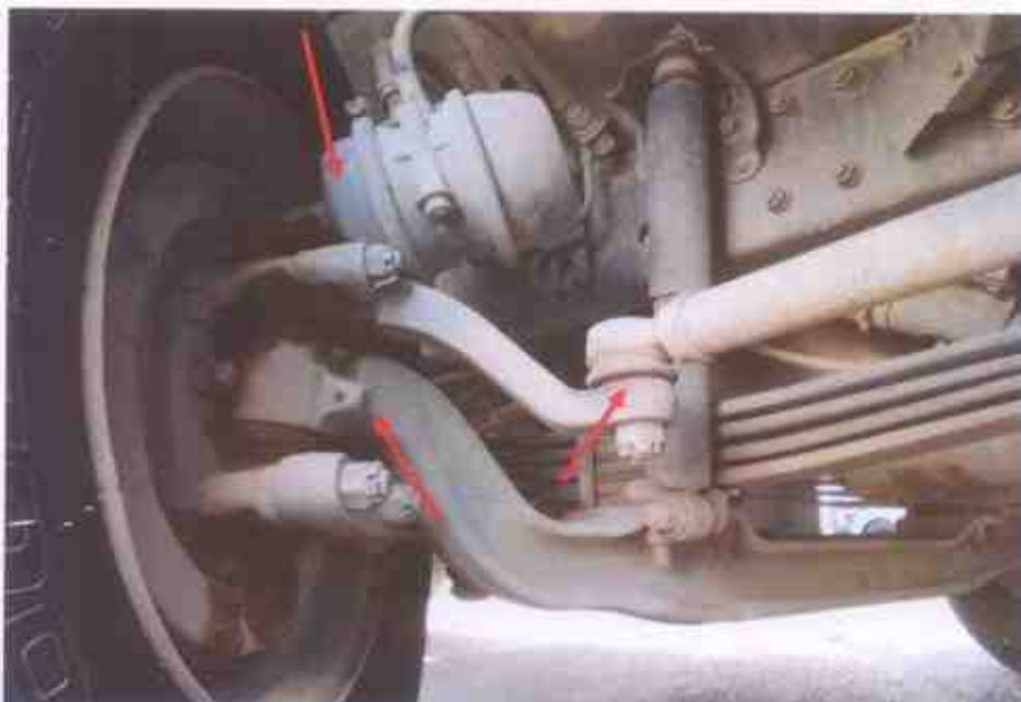
Photo 18 shows the various undercarriage components at the front right wheel of the Tipper Truck, in particular the steering tie rod end (arrowed). The various undercarriage components of the Tipper Truck were all found to be intact without any visible damage. There was also no sign of fluid stain(s) observed on the various undercarriage components.
