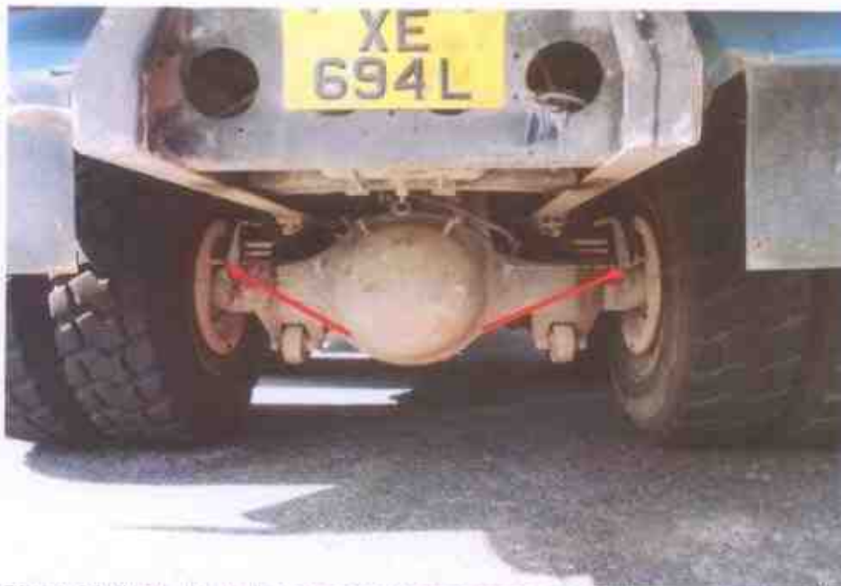
Photo 20 shows the various undercarriage components at the rear wheels of the Tipper Truck. There was no sign(s) of brake fluid leakage along the brake hoses and brake pipes.
