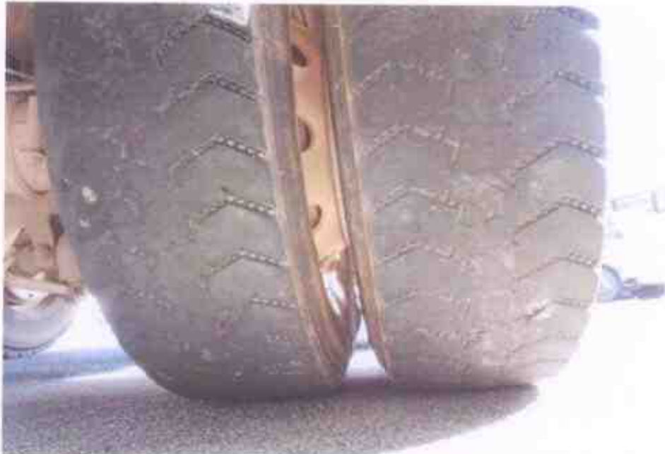
Photo 9 shows the condition of the centre left tyres of the Tipper Truck, which was observed to be in serviceable condition with remaining tread depth of approximately 3mm. The tyres, which were wrapped around standard alloy wheel rim, were also observed to be sufficiently inflated for vehicular operation.
