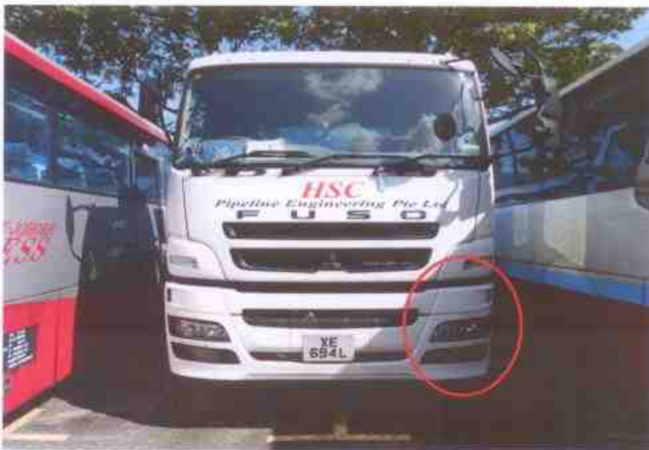
Photo 2 shows a general view of the front portion of the Tipper Truck at the time of our inspection. The Tipper Truck was observed to have sustained minor impact at its front left bumper. Only stain marks was observed on the front left bumper as a result of the accident.
