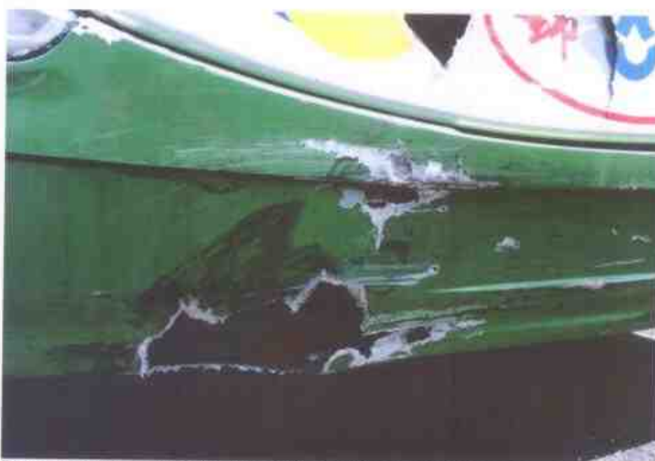
Photo 4 shows a close-up view of the front body of the Motor Bus at the time of our inspection. The Motor Bus front lower bumper was observed to sustained damages due to the accident's impact.
