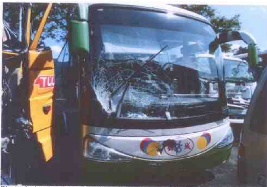
Photo 2 shows a general view of the front body of the Motor Bus at the time of our inspection. The Motor Bus was observed to have sustained damages at its front portion as a result of the accident's collision.
