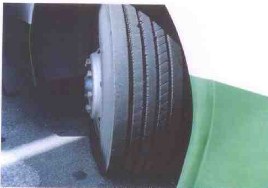
Photo 8 shows the condition of the front left tyre of the Motor Bus, which was observed to be in serviceable condition with remaining tread depth of approximately 8mm. The tyre was also observed to be sufficiently inflated for vehicular operation.
