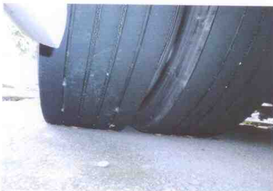
Photo 9 shows the condition of the rear right tyres of the Motor Bus, which were observed to be in serviceable condition with remaining tread depth of approximately 5mm. The tyres, which were wrapped around standard alloy wheels rims, were also observed to be sufficiently inflated for vehicular operation.
