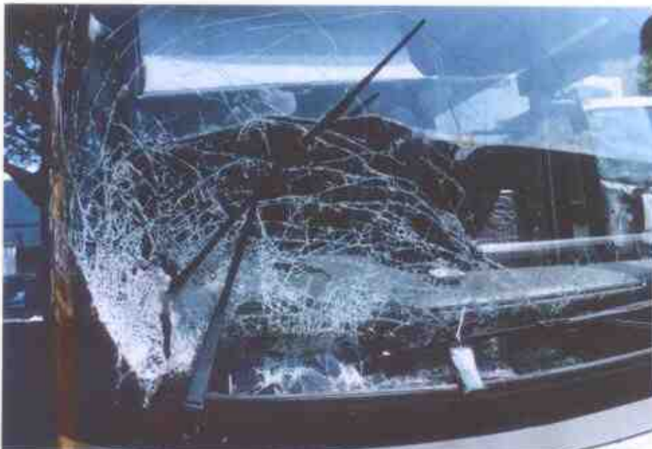
Photo 6 shows a close-up view of the cracked front windshield of the Motor Bus.
