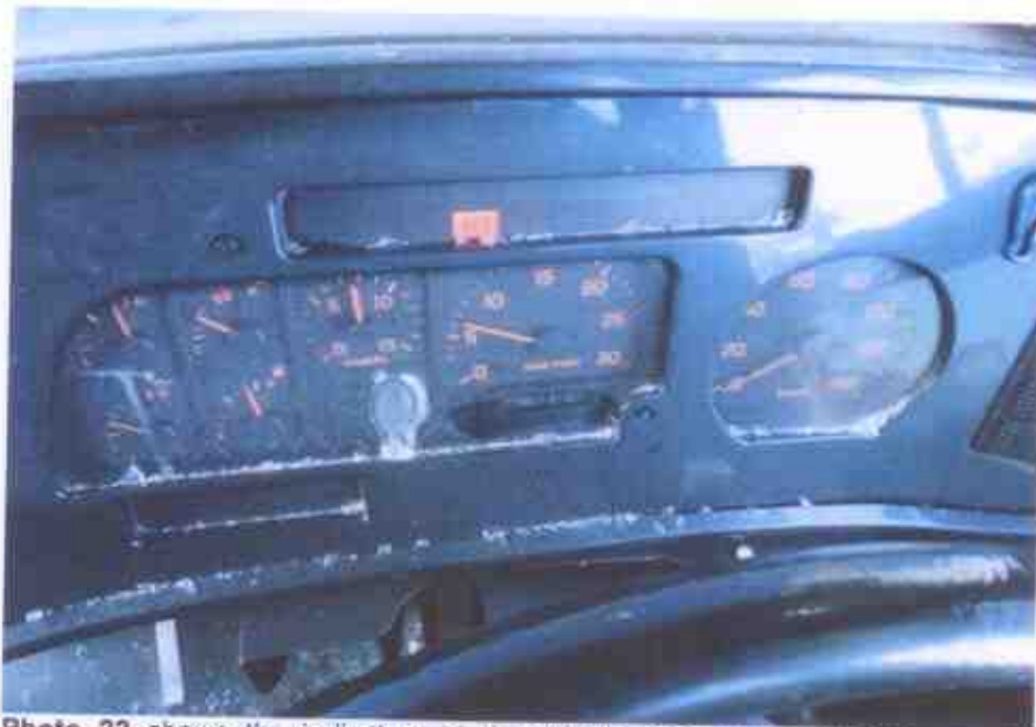
Photo 22 shows the indicators at the driver's seat, these systems were in working condition. This can be established from the warning lights disappearing from the instrument panel after the self-test.
