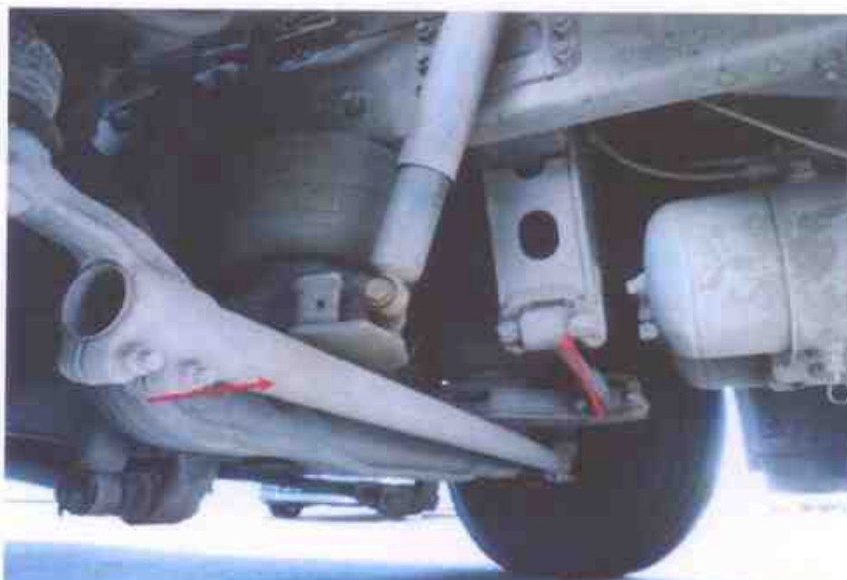
Photo 16 shows some of the mechanical components (arrowed) of the Motor Bus's steering system. Our visual check on the various mechanical components of the steering system revealed all to be intact and in good condition. The steering system of the Motor Bus likely to be in serviceable condition at the time of accident.
