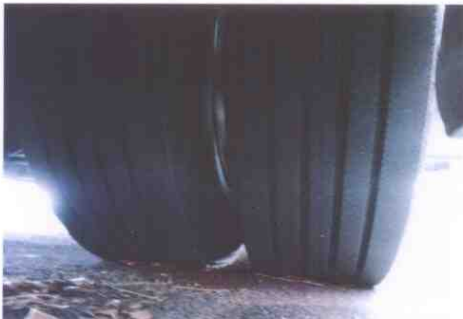
Photo 10 shows the condition of the rear left tyres of the Motor Bus, which were observed to be in serviceable condition with remaining tread depth of approximately 7mm. The tyres, which were wrapped around standard alloy wheel rims, were also observed to be sufficiently inflated for vehicular operation.
