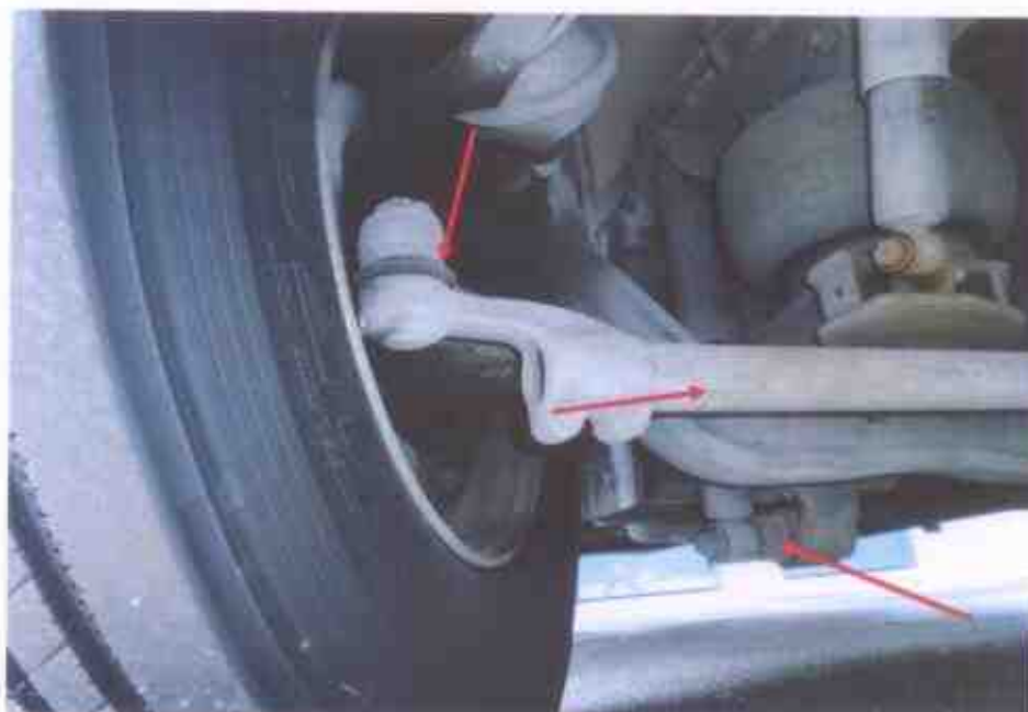
Photo 17 shows the front left wheel components of the front steering system of the Motor Bus. The various undercarriage components of the Motor Bus were all observed to be intact and without any visible damage. This had included the steering rack and steering ball joints (arrowed) of the Motor Bus, which were observed to be securely attached to the front left wheel and front right wheel.
