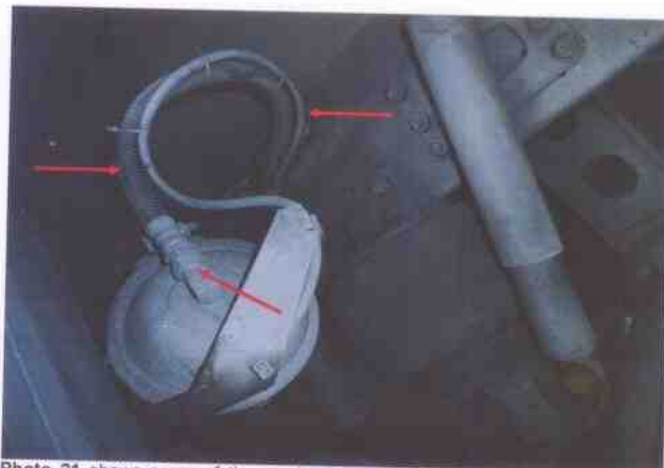
Photo 21 shows some of the mechanical components (arrowed) of the Motor Bus's braking system (including hoses). Our visual check on the various mechanical components reveals all to be intact and in good condition. It was in serviceable condition at the time of accident.
