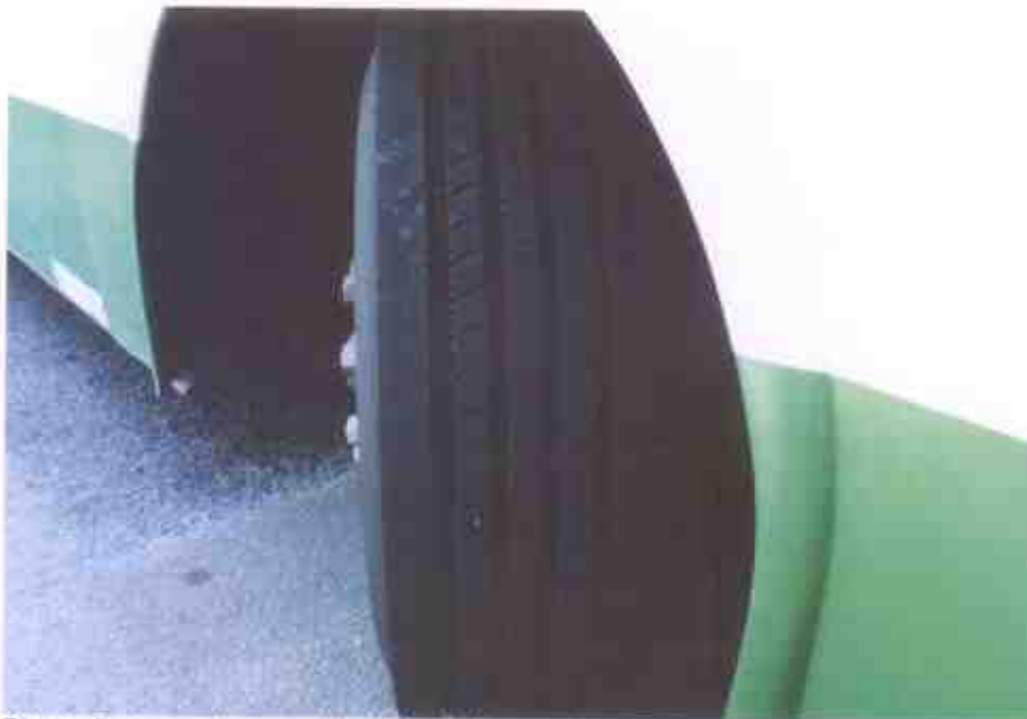
Photo 7 shows the condition of the front right tyre of the Motor Bus, which was observed to be in serviceable condition with remaining tread depth of approximately 8mm. The tyre was also observed to be sufficiently inflated for vehicular operation.
