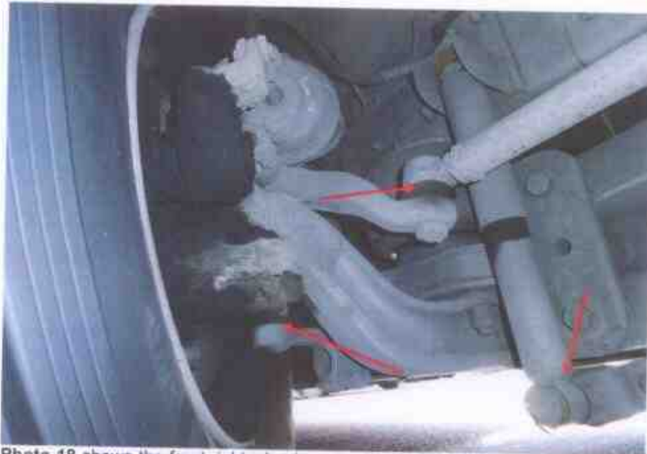
Photo 18 shows the front right wheel components of the front steering system of the Motor Bus. The various undercarriage components of the Motor Bus were all observed to be intact and without any visible damage. This had included the steering rack and steering ball joints (arrowed) of the Motor Bus, which were observed to be securely attached to the front left wheel and front right wheel.
