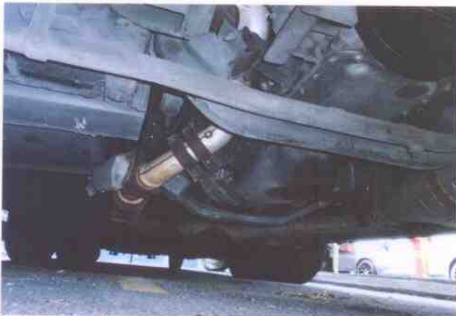
Photo 12 shows the engine undercarriage of the Motor Bus. Some pre-existed fluid was observed at time of our inspection.
