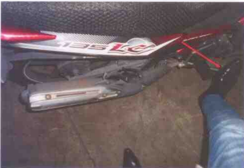
Photo 17 shows testing of the braking of the rear brake in progress. There was some resistance felt (spongy like feel) upon stepping on the brake pedal.
