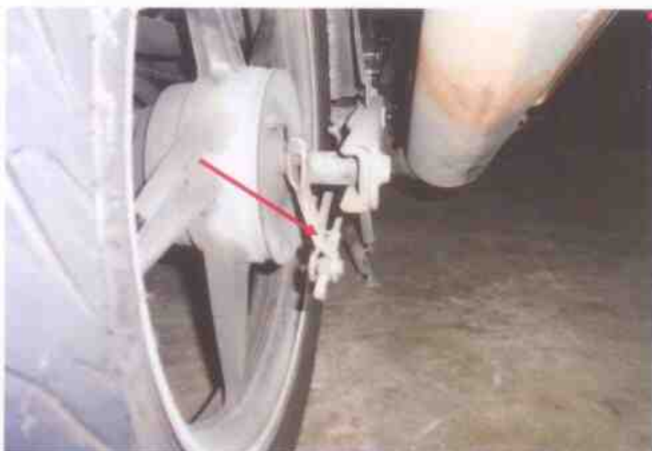
Photo 15 shows our checks on the rear brake mechanical components had also indicated that the rear brake was fit for operational purposes, without abnormalities unaffected by the accident.
