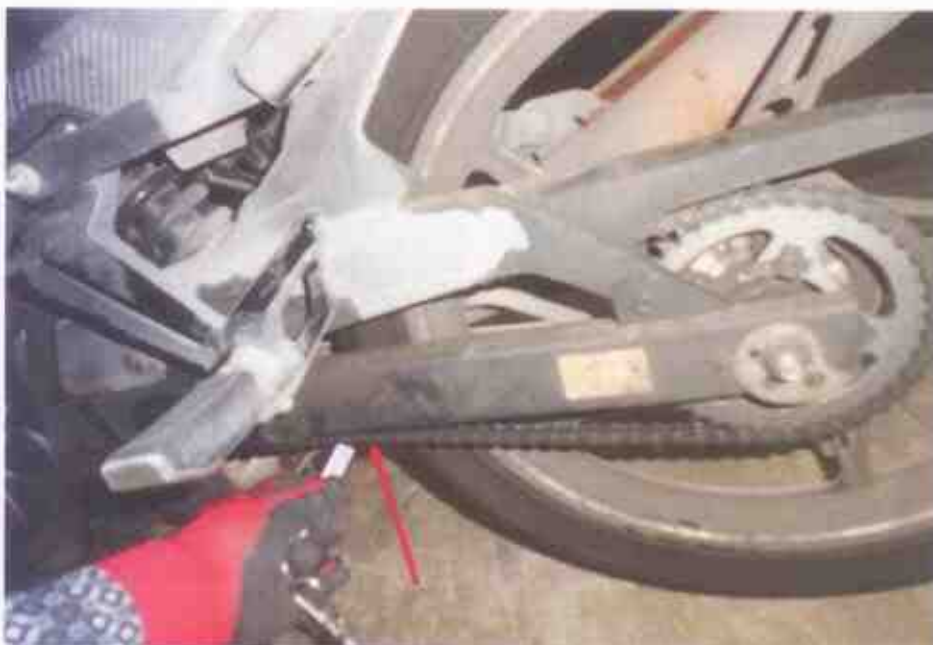
Photo 13 shows the general view of the gear train (arrowed) of the Motorcycle, which was observed to be intact with no misalignment. It was also adequately lubricated for operating purposes. Free play tension was also observed & found adequately acceptable.
