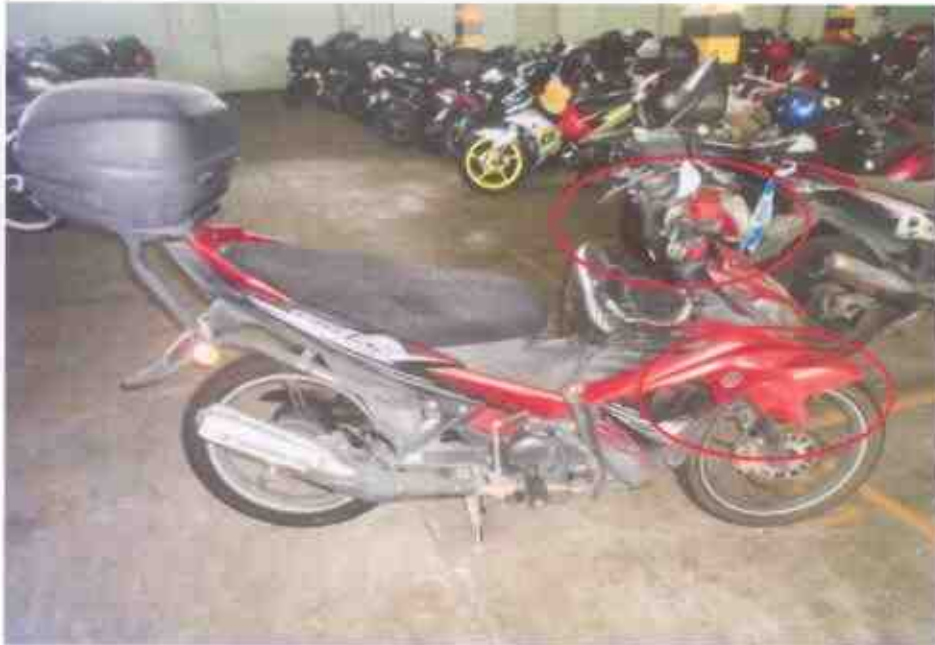
Photo 3 shows a general view of the right body of the Motorcycle at the time of our inspection. The Motorcycle was observed to have sustained relatively minor damages on the right side fairing, handle, mud guard & brake lever at time of our inspection.
