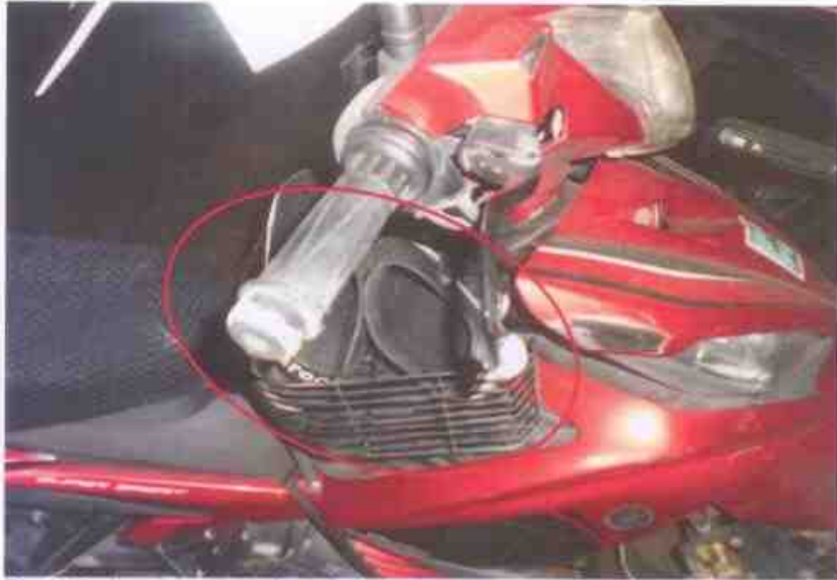
Photo 7 shows a closer view of the right handle & brake lever of the Motorcycle at the time of our inspection. The Motorcycle was observed to have sustained with relatively minor damages due to the accident collision. (Circled)
