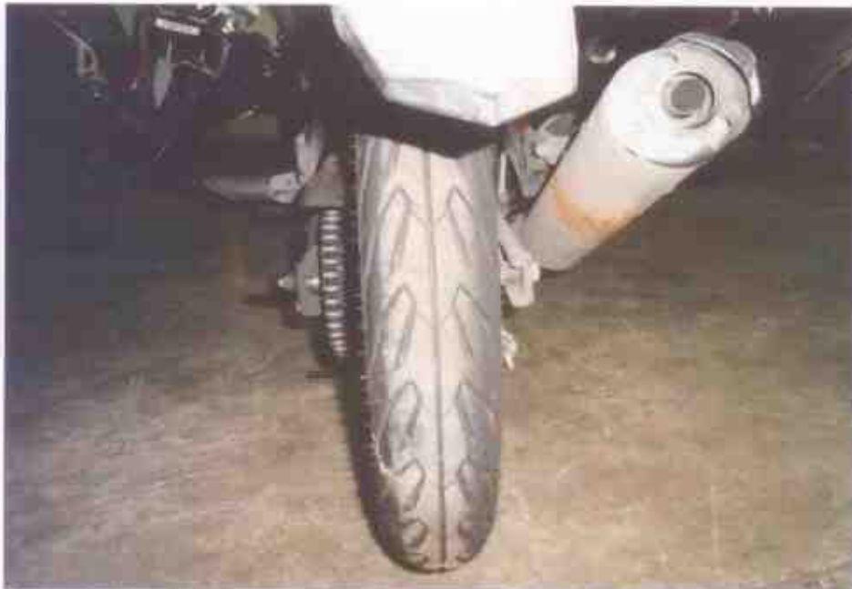
Photo 8 shows the rear tyre of the Motorcycle. The rear tyre was observed to be in serviceable condition with remaining tread depth of approximately 3mm. The tyre was also observed to be sufficiently inflated for vehicular operation.
