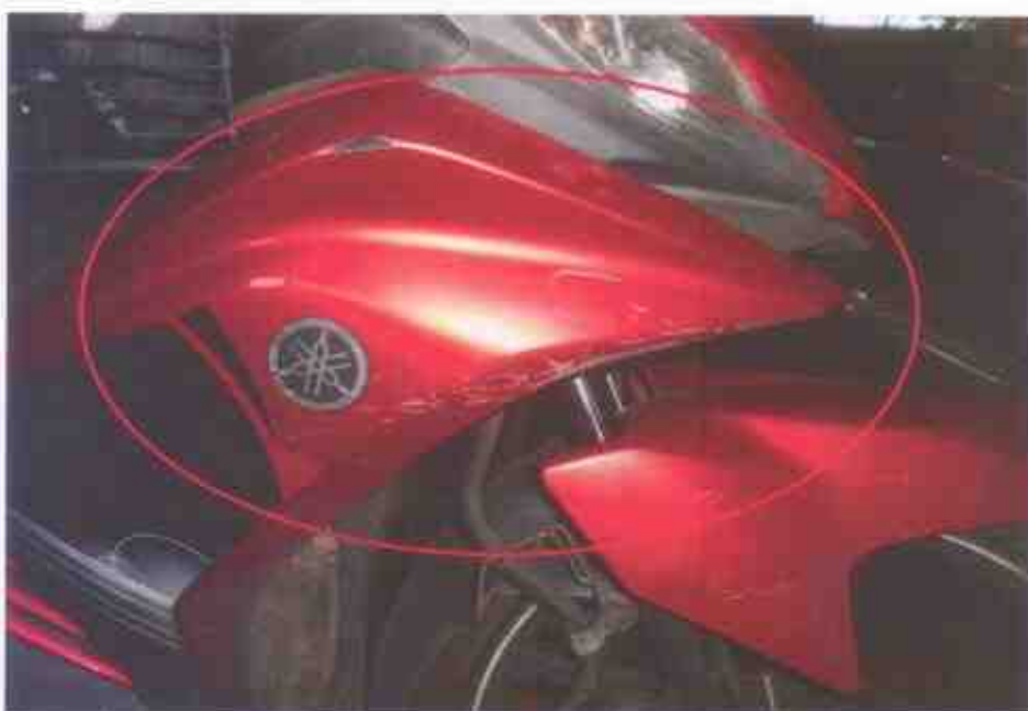
Photo 6 shows a closer view of the right fairing of the Motorcycle at the time of our inspection. The Motorcycle was observed to have sustained with relatively minor damages due to the accident collision. (Circled)
