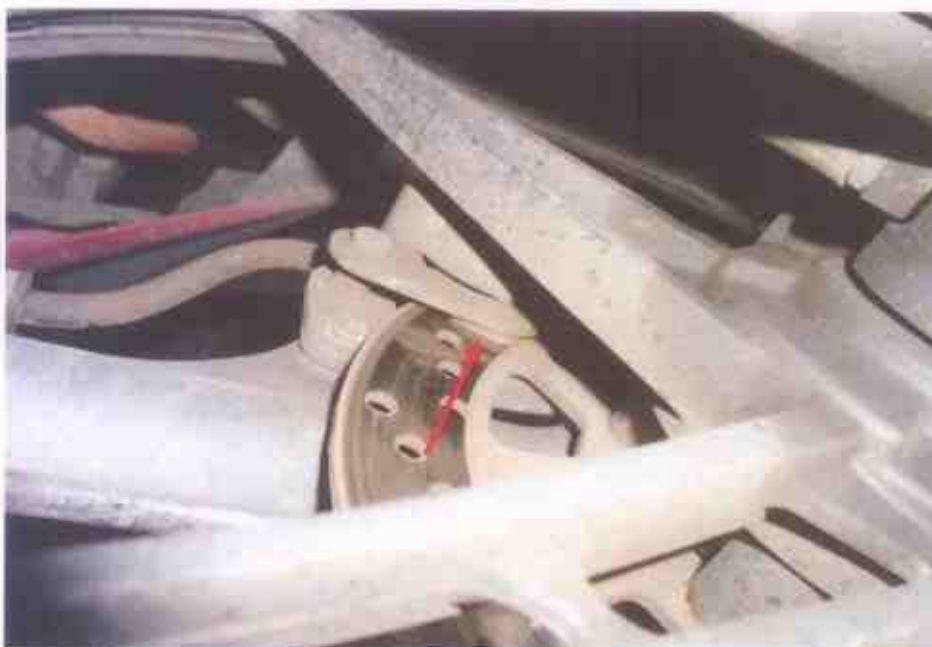
Photo 18 shows the front brake pad at time of our inspection. The frictional material was observed to be sufficient for operational purposes.
