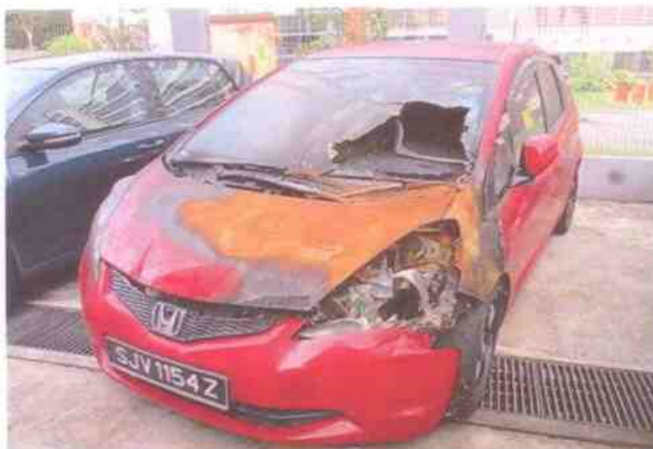
Photo 3 shows the general view of the left portion of the Insured Vehicle at the time of our inspection. The exterior body of the Insured Vehicle had sustained visible fire damage. This included its windscreen, front bonnet, left headlight, front bumper, left side panel, left front rim and left front tyre.
