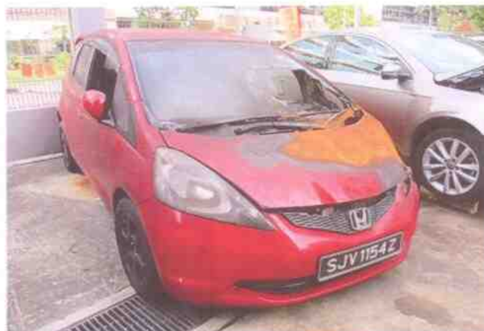
Photo 2 shows the general view of the right portion of the Insured Vehicle at the time of our inspection. The exterior body of the Insured Vehicle had sustained visible fire damage. This included its windscreen, front bonnet, front bumper and right headlight.
