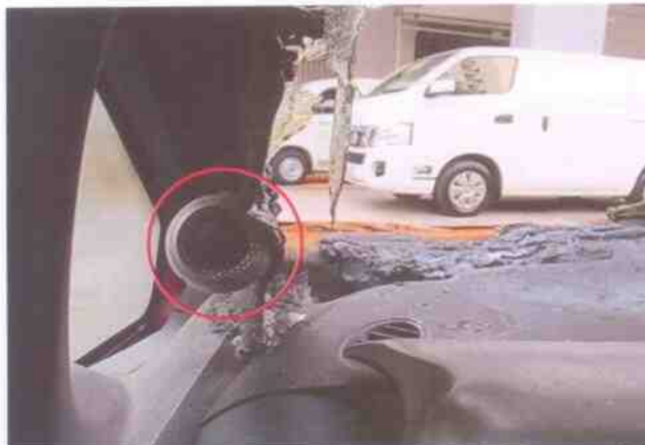
Photo 9 shows the 2nd aftermarket twitter fitted onto the left corner of the dashboard of the Insured Vehicle upon our inspection which had sustained serious fire damage (circled).
