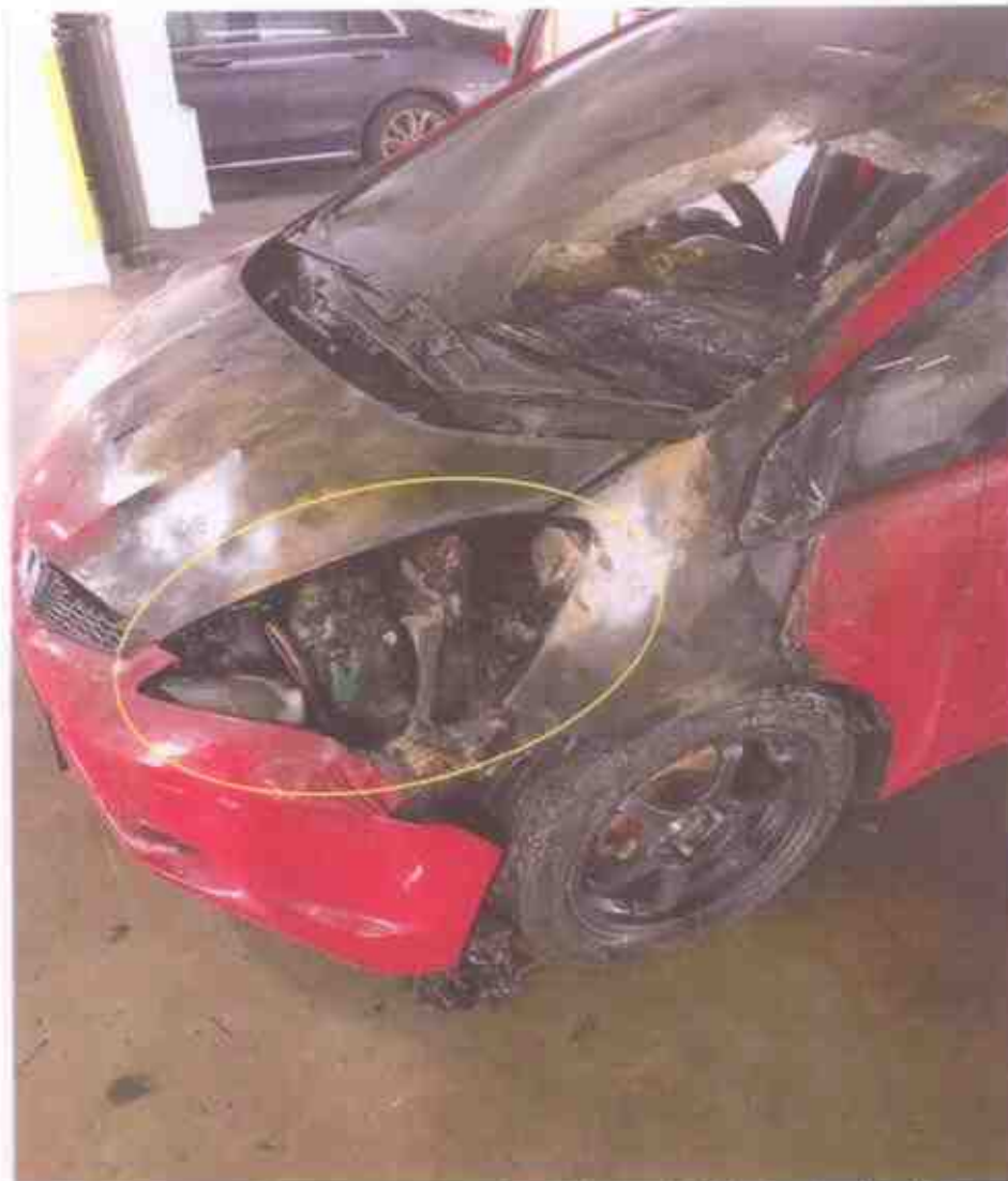
Photo 23 shows the left side view of the Insured Vehicle after the fire was extinguished. The extensive damages sustained to the left front portion of the Insured Vehicle indicate that the fire had started from the left portion of the engine compartment (circled).
