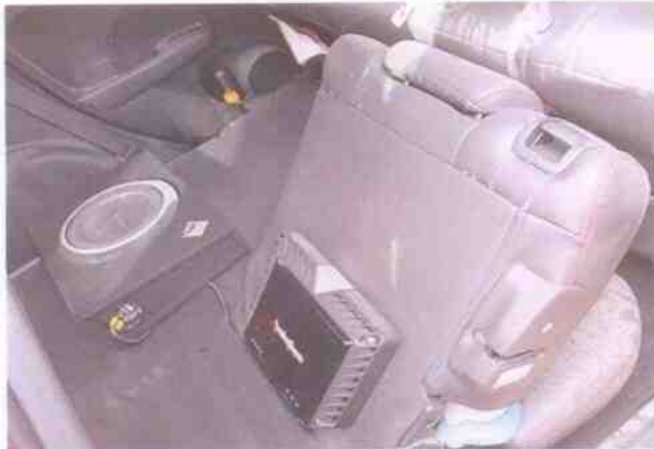
Photo 10 shows the aftermarket amplifier and subwoofer fitted behind the rear passenger seats of the Insured Vehicle upon our inspection.
