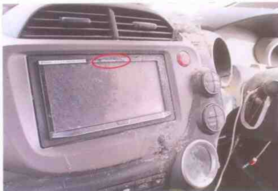
Photo 13 shows the in-car DVD player that was fitted at the centre portion of the front dashboard of the Insured Vehicle which had sustained serious fire damage. The brand of the in-car DVD player was 'PIONEER' (circled).
