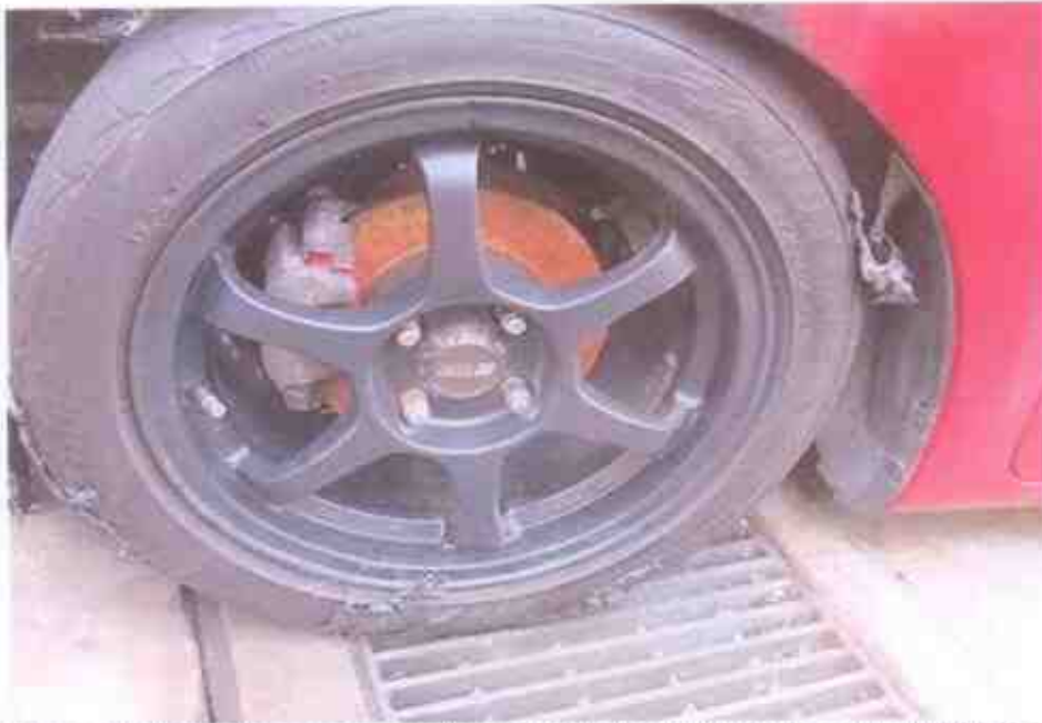
Photo 16 shows the non-standard rim found to be fitted on the Insured Vehicle at the time of our inspection. The 15- inch alloy rims fitted on the Insured Vehicle were not the standard type for the Insured Vehicle.
