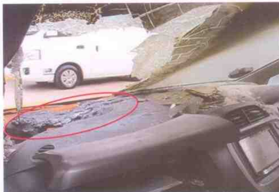
Photo 6 shows a closer view of the the interior compartment of the Insured Vehicle which was observed to be severely affected by the fire, in particular the left portion of the dashboard (circled).
