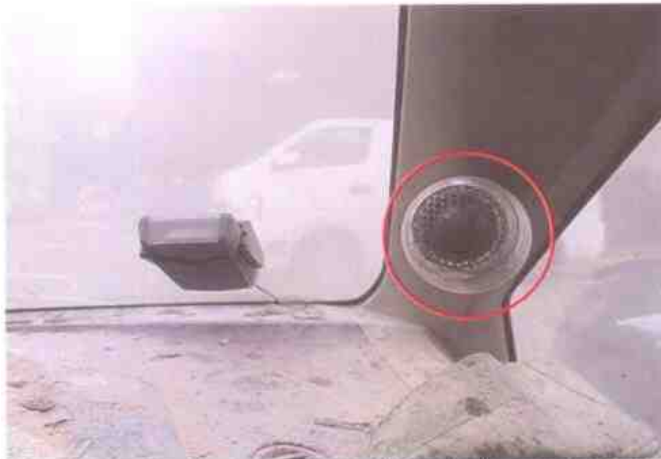
Photo 8 shows the 1st aftermarket twitter fitted onto the right corner of the dashboard of the Insured Vehicle upon our inspection which had sustained minor fire damage (circled).
