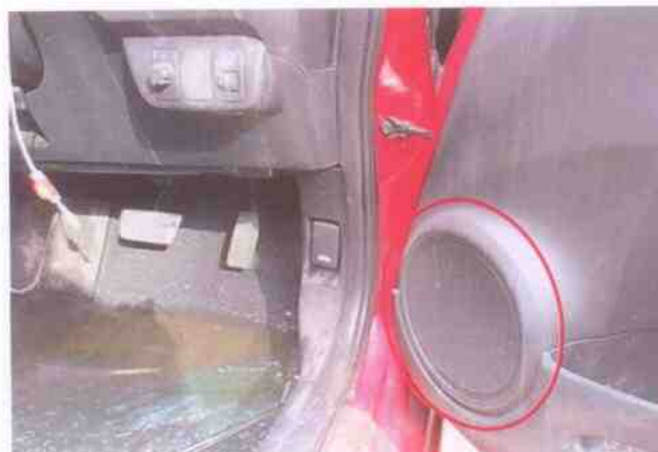
Photo 15 shows the 2nd aftermarket speaker fitted at the driver door panel (circled).
