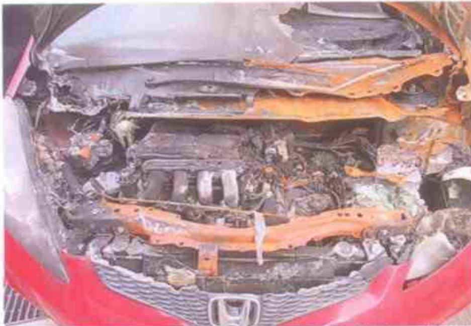
Photo 7 shows a general view of the engine compartment of the Insured Vehicle at the time of our inspection. Most of the components inside the engine compartment were found to be severely burnt and/or melted as a result of the fire.
