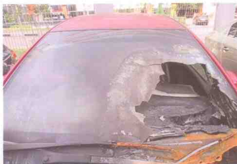
Photo 4 shows a closer view of the windscreen of the Insured Vehicle at the time of our inspection. The windscreen had sustained extensive fire damage.
