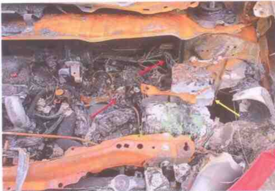
Photo 17 shows the wirings around the left rear portion of the engine compartment, which is in the immediate vicinity where the fire to the Insured Vehicle had likely started. Greenish residue was found on the wirings (red arrows) leading to the Engine Control Module (ECM) (yellow arrow). The presence of such greenish residue suggests occurrence of an electrical short circuit.
