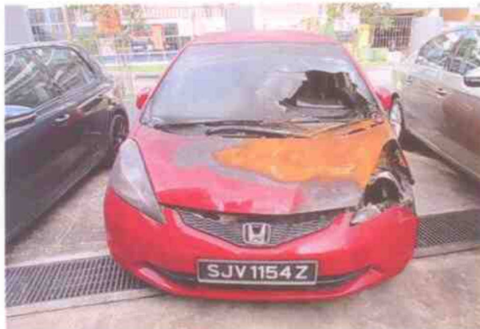
Photo 1 shows the general view of the front portion of the Insured Vehicle at the time of our inspection. The exterior body of the Insured Vehicle had sustained visible fire damage. This included its windscreen, front bonnet, headlights, front bumper, side panels, front rims and front tyres.
