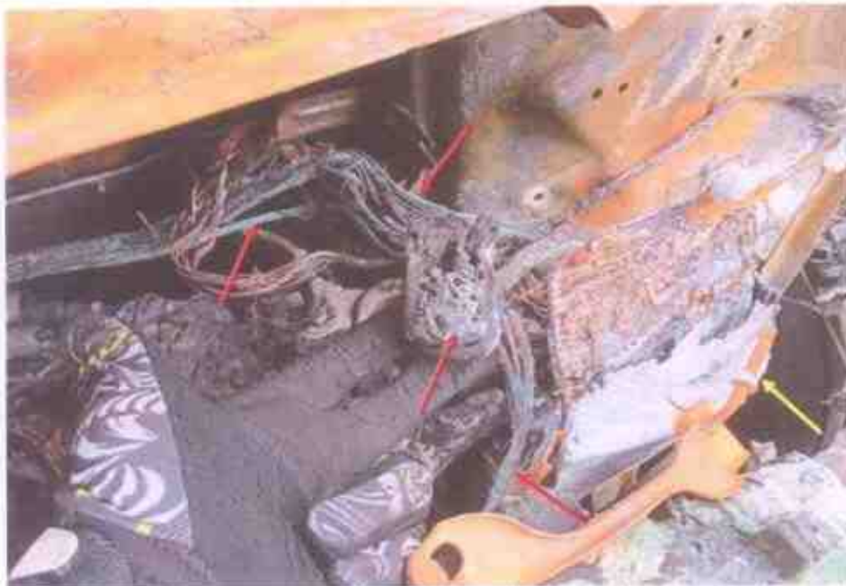
Photo 19 shows a closer view of the wirings with greenish residue (red arrows) leading to the Engine Control Module (ECM) (yellow arrow). The presence of such greenish residue suggest occurrence of an electrical short circuit.
