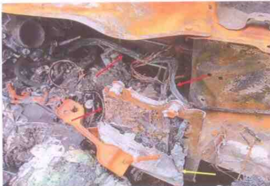
Photo 18 shows a closer view of the wirings with greenish residue (red arrows) leading to the Engine Control Module (ECM) (yellow arrow). The presence of such greenish residue suggest occurrence of an electrical short circuit.
