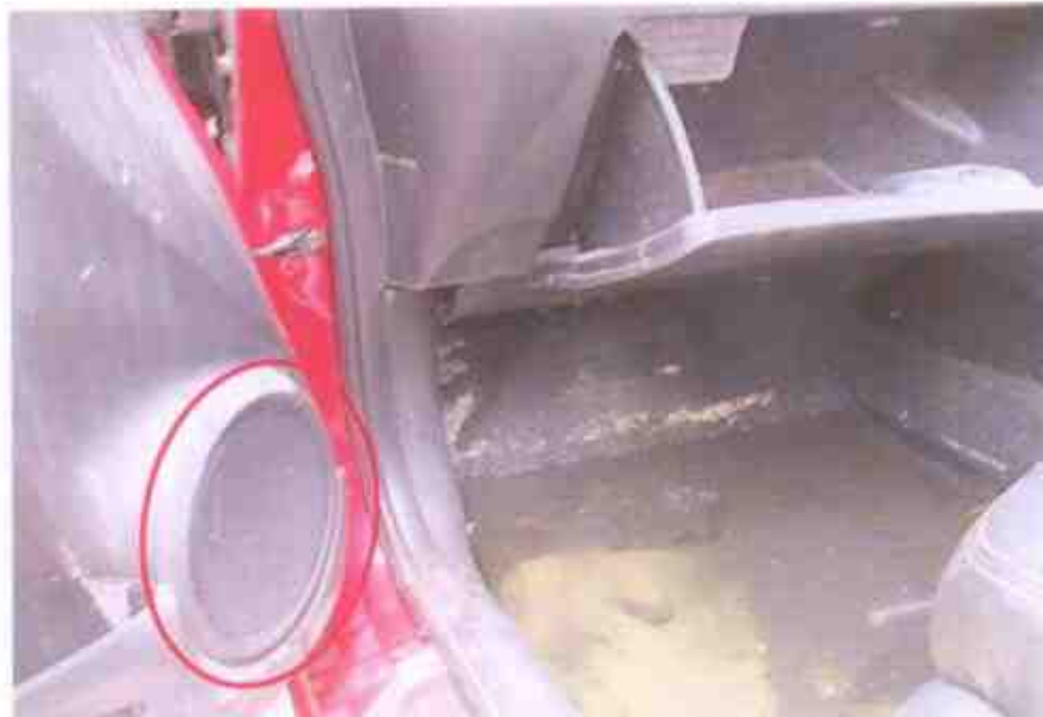
Photo 14 shows the 1st aftermarket speaker fitted at the front passenger door panel (circled).
