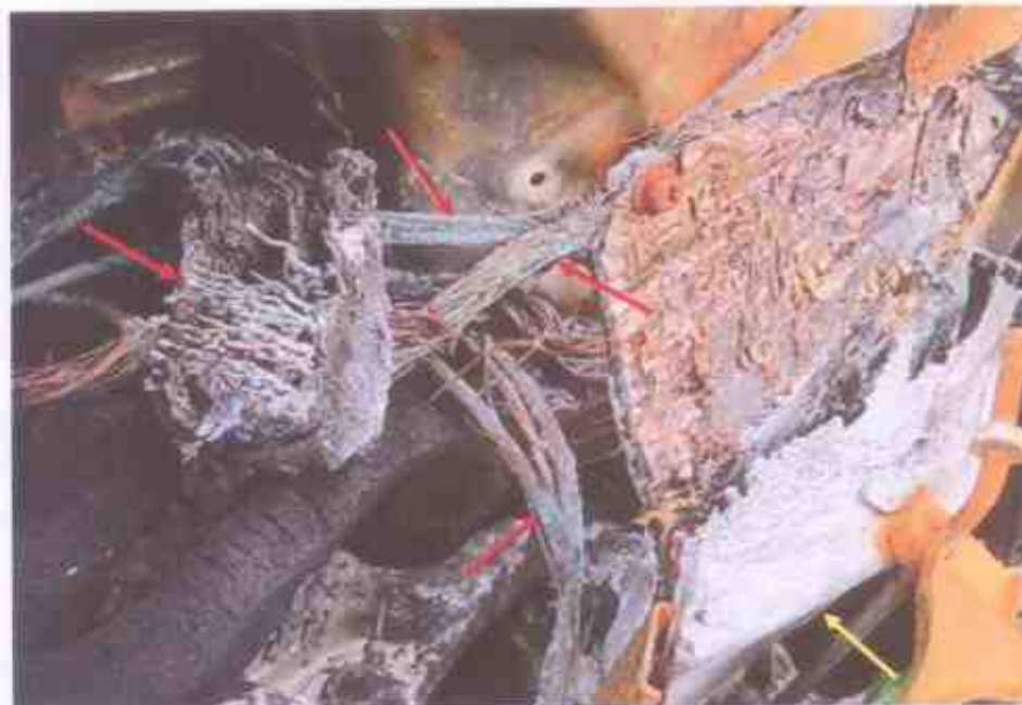
Photo 20 shows a close up view of the wirings with greenish residue (red arrows) leading to the Engine Control Module (ECM) (yellow arrow). The presence of such greenish residue suggest occurrence of an electrical short circuit.
