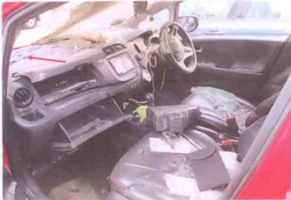
Photo 5 shows the interior compartment of the Insured Vehicle at the time of our inspection. The interior compartment of the Insured Vehicle was observed to be severely affected by the fire, in particular the left portion of the dashboard (arrowed).
