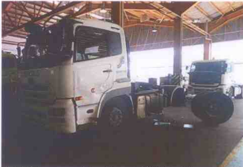
Photo 10 shows a general view of Exemplar Vehicle 2, a Nissan model prime mover that was fitted with a full air-brake system, the same type that was fitted on the Motor Lorry. The rear left brake drums were removed for my checks on the condition of the brake drums.
