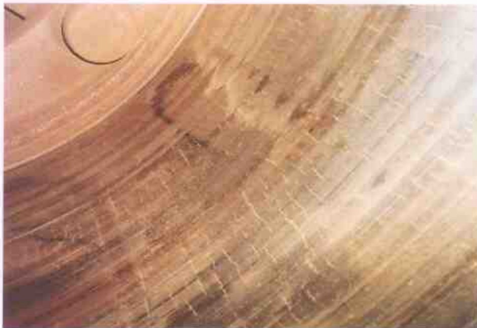
Photo 15 shows a close-up view of the same type of marks that were referred to as "cracks" in Koays Report (refer to the photographs seen in page 14 to page 16 of Koays Report). These marks were found on the rear right brake drum of Exemplar Vehicle 2.
