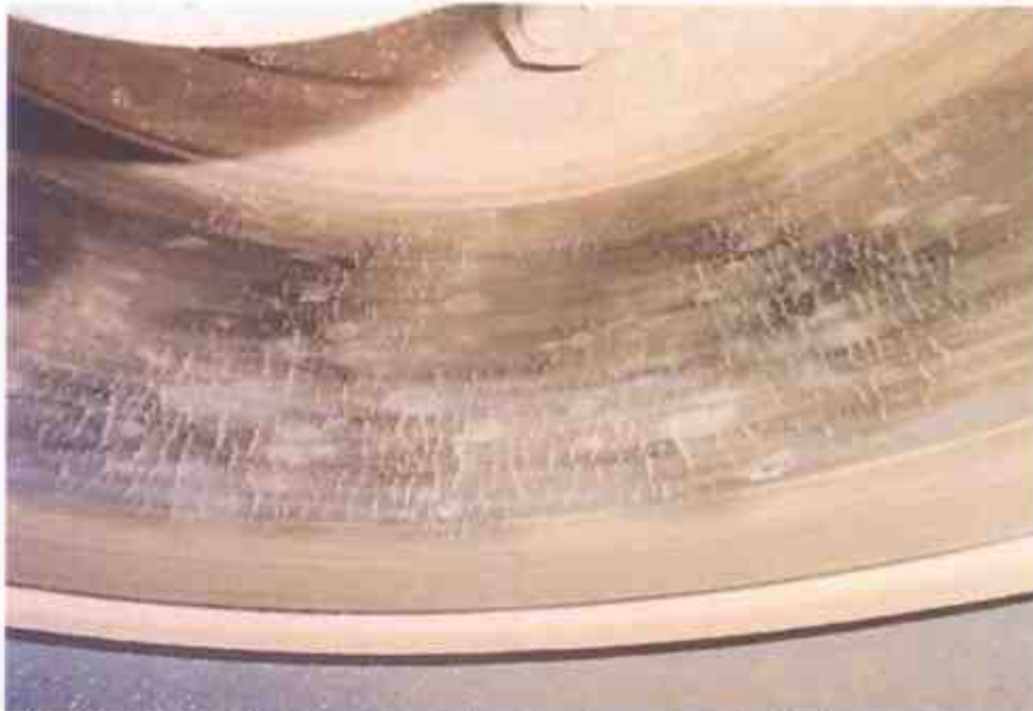
Photo 6 shows a close-up view of the same type of marks that were referred to as "cracks" in Koays Report (refer to the photographs seen in page 14 to page 16 of Koays Report). These marks were found on the front left brake drum of Exemplar Vehicle 1.
