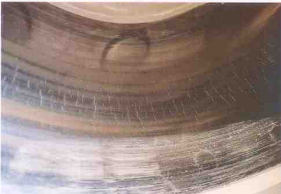
Photo 17 shows a close-up view of the same type of marks that were referred to as "cracks" in Koays Report (refer to the photographs seen in page 14 to page 16 of Koays Report). These marks were found on the front right brake drum of Exemplar Vehicle 2.
