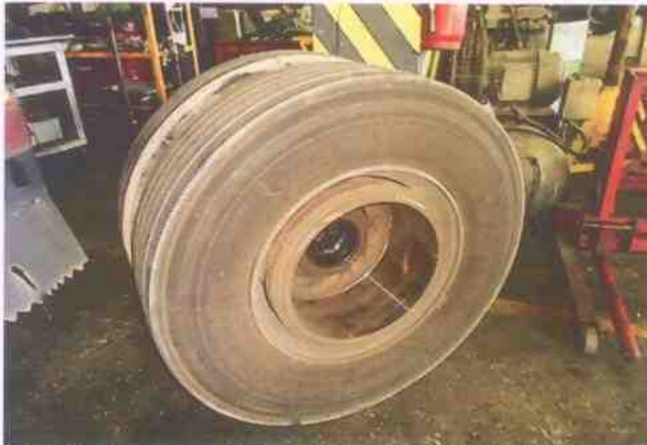
Photo 14 shows a general view of the removed rear right brake drum of Exemplar Vehicle 2. I had found the same type of marks, which were referred to as "cracks" in Koays Report. These marks were observed to be around the entire circumference of the brake drum.
