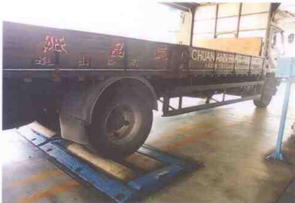
Photo 7 shows Exemplar Vehicle 1 going through the roller brake test at STA Inspection Centre with the brake drums condition as seen in photograph 3 and photograph 6 above. There were 2 tests carried out to ensure the accuracy of the result.
