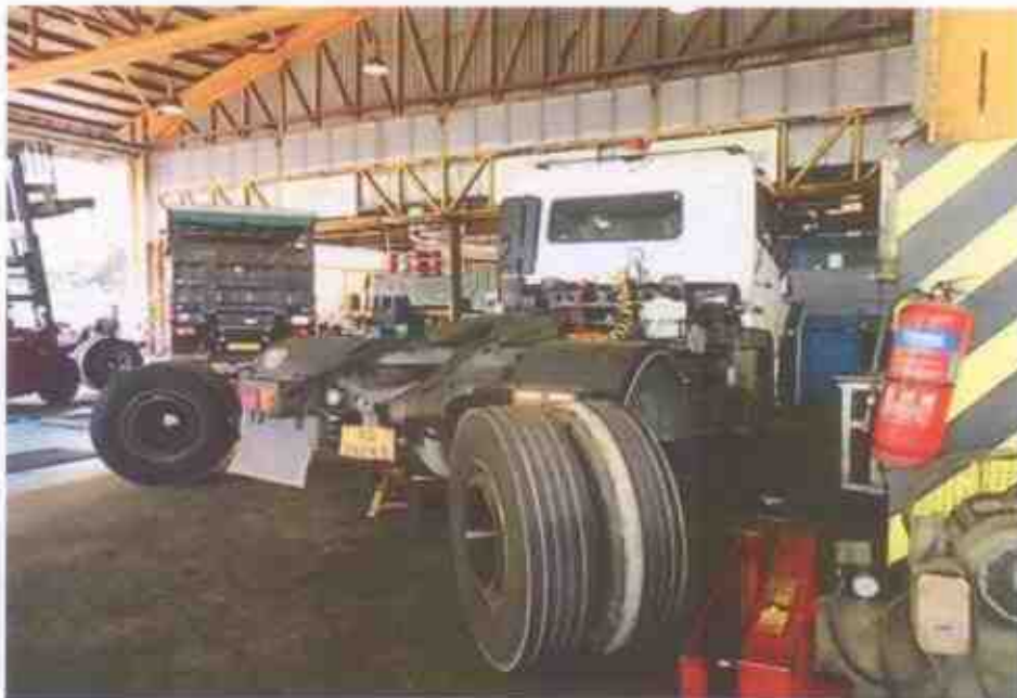
Photo 13 shows a general view of Exemplar Vehicle 2 with its rear right brake drums removed for my checks on the condition of the brake drums.
