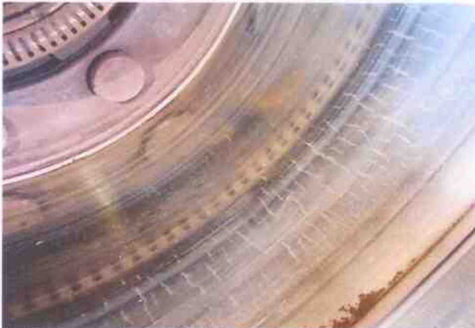
Photo 12 shows a close-up view of the same type of marks that were referred to as "cracks" in Koays Report (refer to the photographs seen in page 14 to page 16 of Koays Report). These marks were found on the rear left brake drum of Exemplar Vehicle 2.
