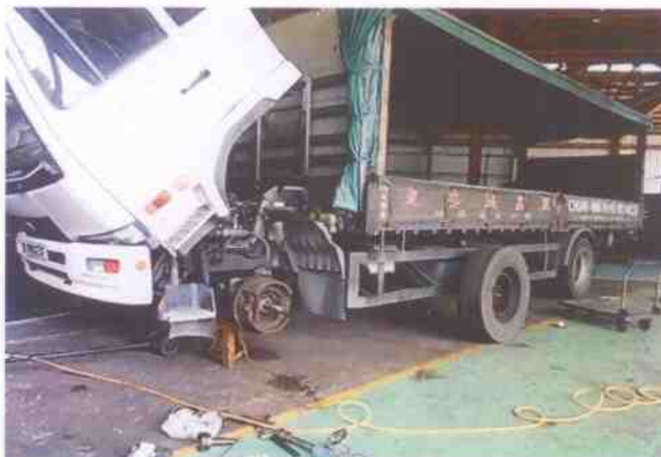
Photo 4 shows the front left brake drum of Exemplar Vehicle 1, removed for checks on the condition of the front left brake drum. Exemplar Vehicle 1 was an exact same model as the Motor Lorry.
