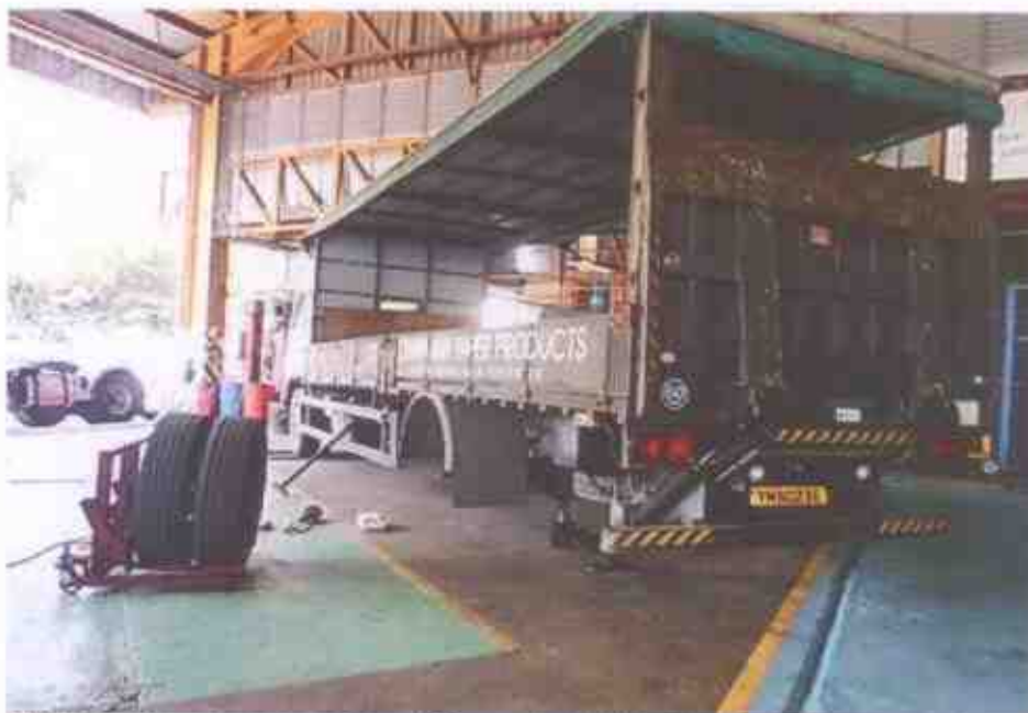
Photo 1 shows a general view of Exemplar Vehicle 1, which was an exact same model as the Motor Lorry. The rear left brake drums were removed for my checks on the condition of the brake drums.
