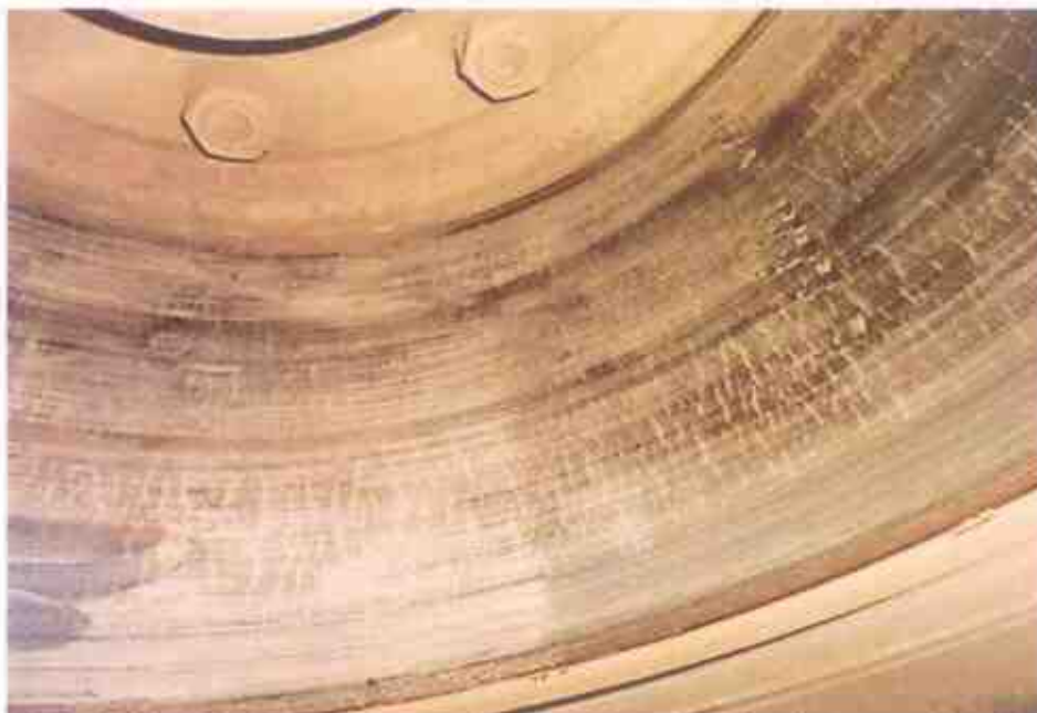
Photo 3 shows a close-up view of the same type of marks that were referred to as "cracks" in Koays Report (refer to the photographs seen in page 14 to page 16 of Koays Report). These marks were found on the rear left brake drum of Exemplar Vehicle 1.
