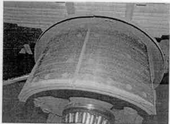
Photo 50: Brake linings appear faded due to overheating and need replacement.
