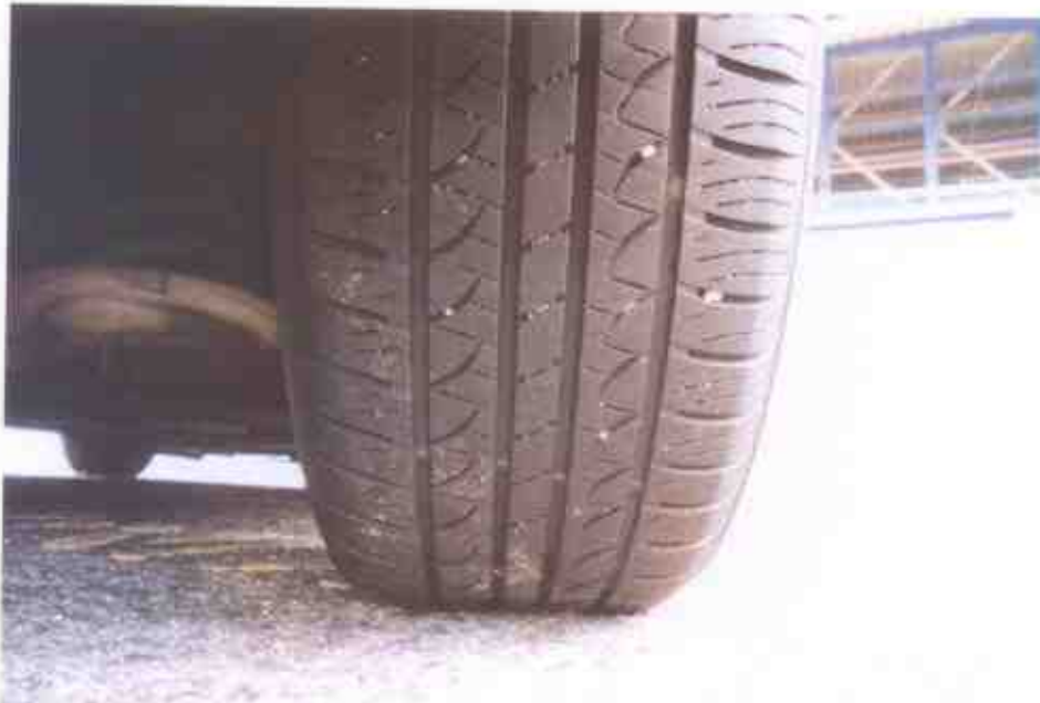
Photo 11 shows the condition of the rear right tyre of the Motor Taxi, which was observed to be in serviceable condition with remaining tread depth of approximately 5mm.
