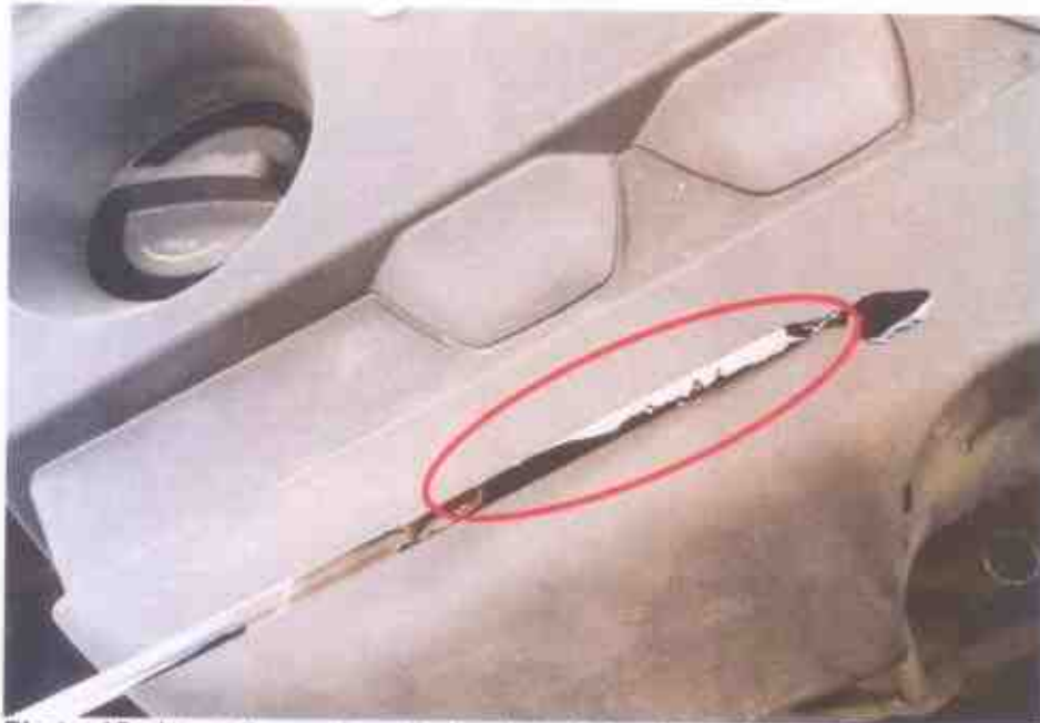
Photo 15 shows the engine oil dip stick of the Motor Taxi at the time of our inspection. The engine oil was observed to be of sufficient level and without any visible contamination.
