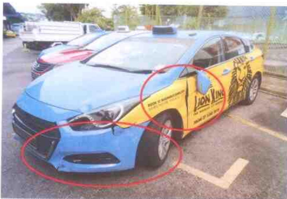
Photo 3 shows a general view of the front left body of the Motor Taxi at the time of our inspection. The Motor Taxi was observed to have sustained minor impact damages that were confined to its frontal left & right portion.
