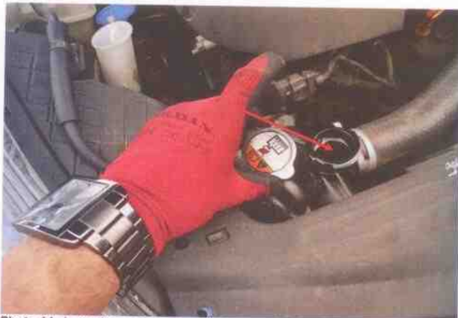
Photo 14 shows the engine coolant fluid reservoir of the Motor Taxi at the time of our inspection. The engine coolant fluid was observed to be of sufficient level and without any visible contamination.
