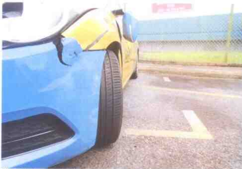
Photo 7 shows a close up view of the front left portion of the Motor Taxi at the time of our inspection. The Motor Taxi had sustained damages at the front right lower bumper, headlamp, side fender, passenger's door & left side mirror likely due to the accident.
