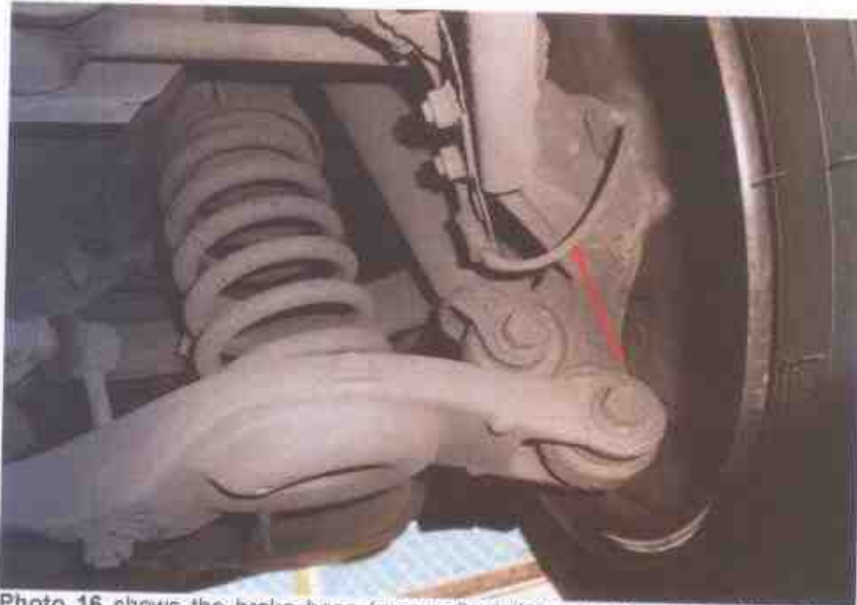
Photo 16 shows the brake hose (arrowed) at the rear left wheel of the Motor Taxi. We did not observe any leakage of brake fluid at the time of our inspection of the Motor Taxi. Our visual inspection of the various mechanical components of the Motor Taxi's braking system revealed all to be intact without visible damage.
