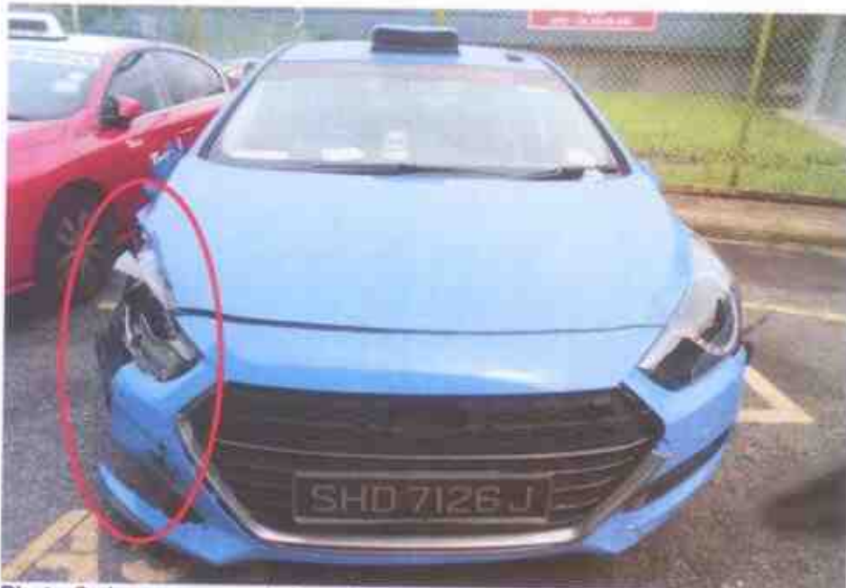
Photo 2 shows a general view of the front body of the Motor Taxi at the time of our inspection. The Motor Taxi was observed to have sustained impact damages that were confined to its frontal left & right portion. Its front right lower bumper was observed to be damaged likely due to the accident's collision impact.
