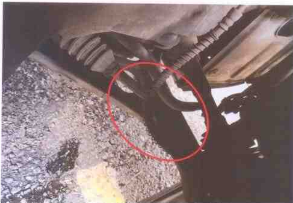
Photo 18 shows the various undercarriage components at the front right wheel of the Motor Taxi, in particular the steering rod (circled). It was observed to be bent as a result of the accident.
