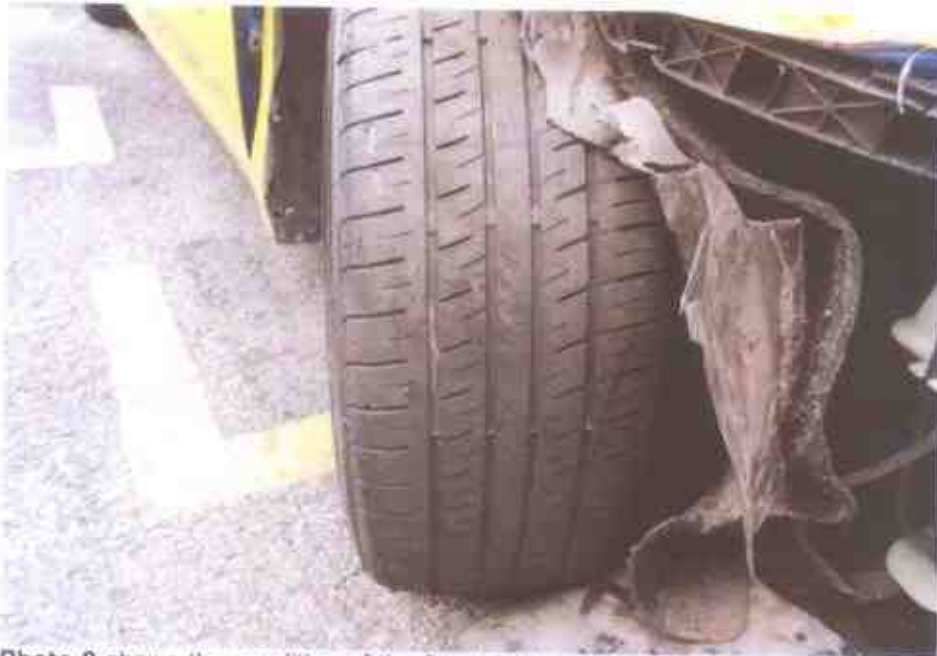
Photo 8 shows the condition of the front right tyre of the Motor Taxi, which was observed to be in serviceable condition with remaining tread depth of approximately 4mm.
