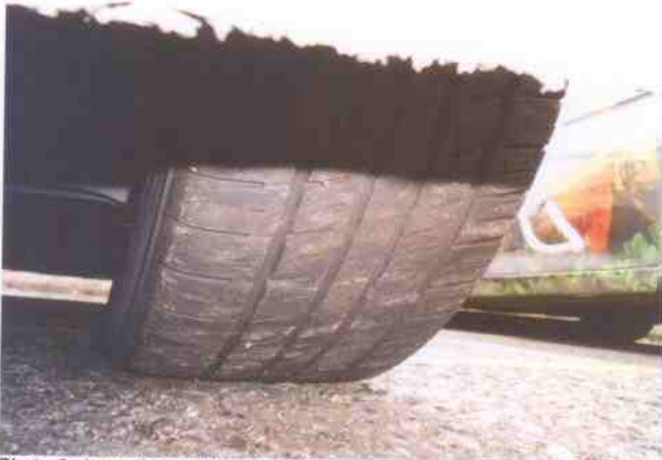
Photo 9 shows the condition of the front left tyre of the Motor Taxi, which was observed to be in serviceable condition with remaining tread depth of approximately 3mm.
