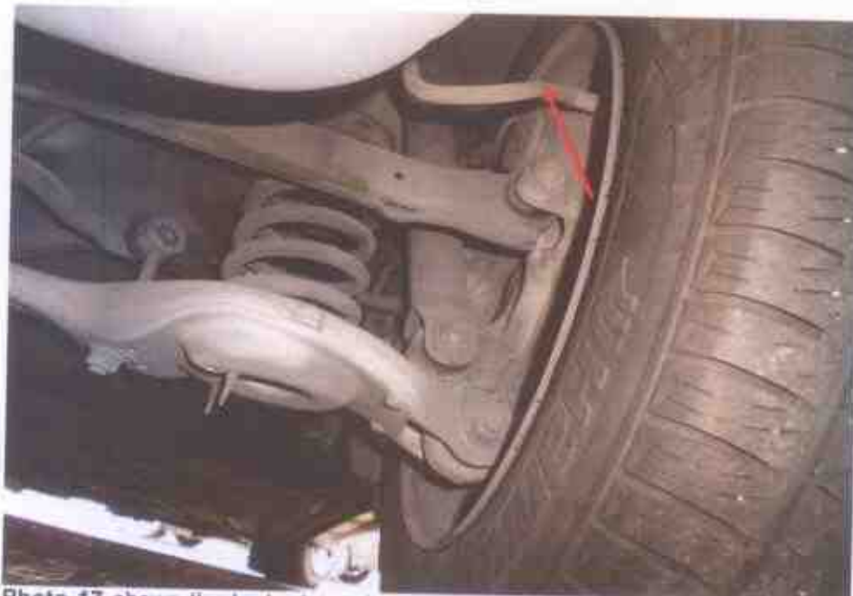
Photo 17 shows the brake hose (arrowed) at the rear right wheel of the Motor Taxi. We did not observe any leakage of brake fluid at the time of our inspection of the Motor Taxi. Our visual inspection of the various mechanical components of the Motor Taxi's braking system revealed all to be intact without visible damage.
