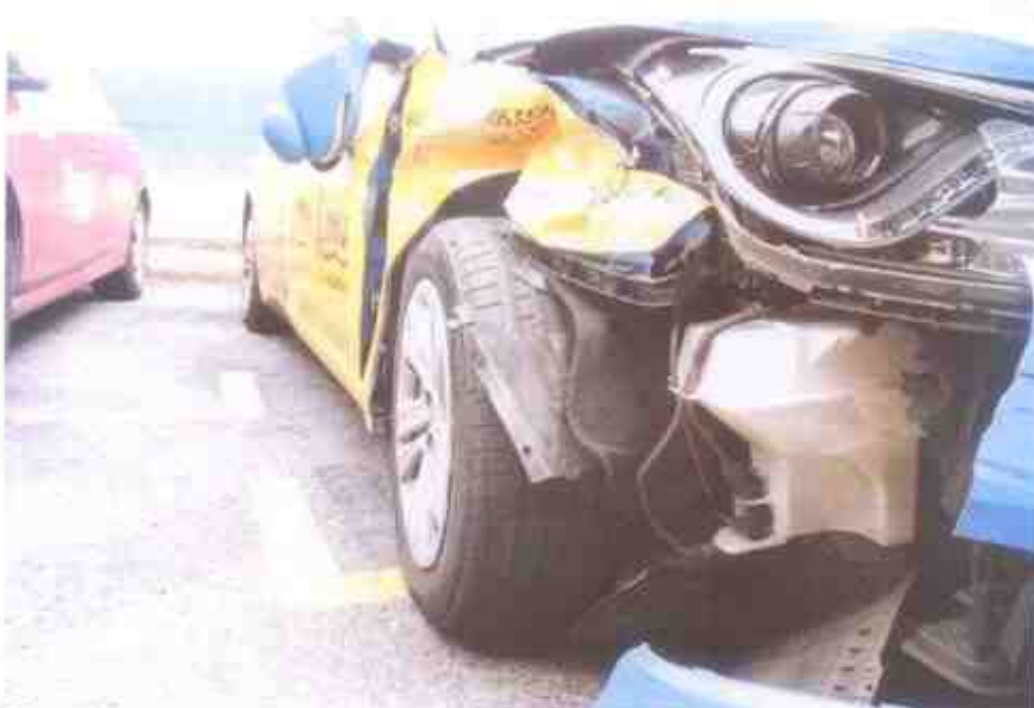
Photo 6 shows a semi close up view of the front right portion of the Motor Taxi at the time of our inspection. The Motor Taxi had sustained damages at the front right lower bumper, headlamp, side fender, driver door & right side mirror likely due to the accident.
