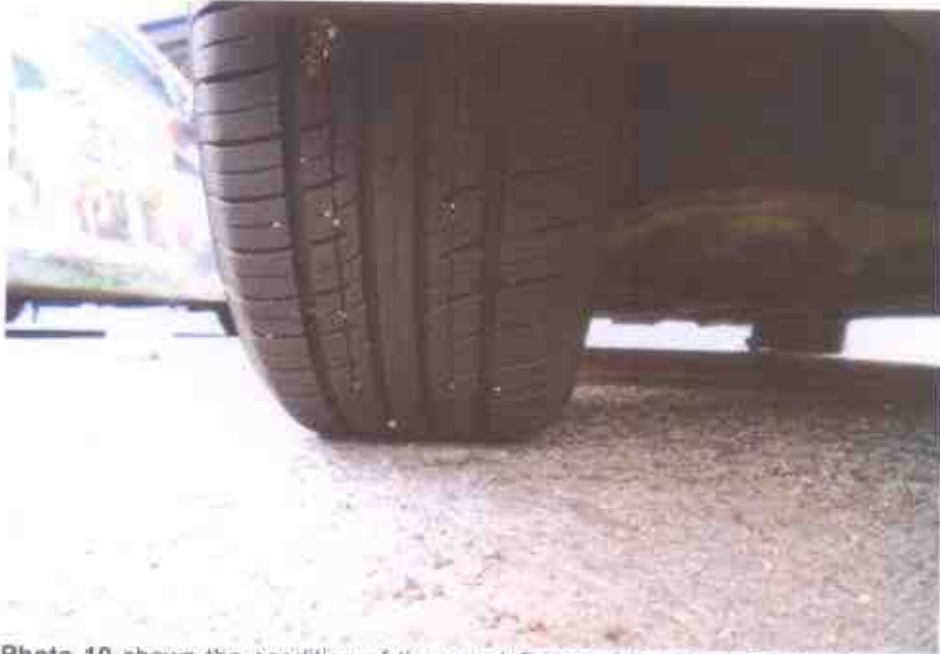
Photo 10 shows the condition of the rear left tyre of the Motor Taxi, which was observed to be in serviceable condition with remaining tread depth of approximately 5mm.
