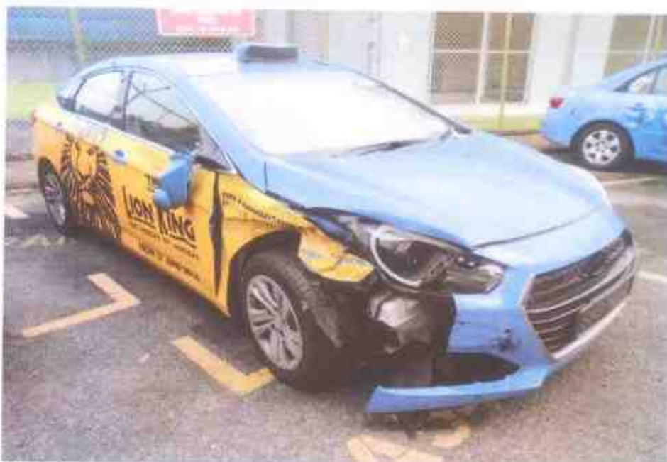
Photo 4 shows a general view of the front right body of the Motor Taxi at the time of our inspection. The Motor Taxi was observed to have sustained impact damages that were confined to its frontal left & right portion.
