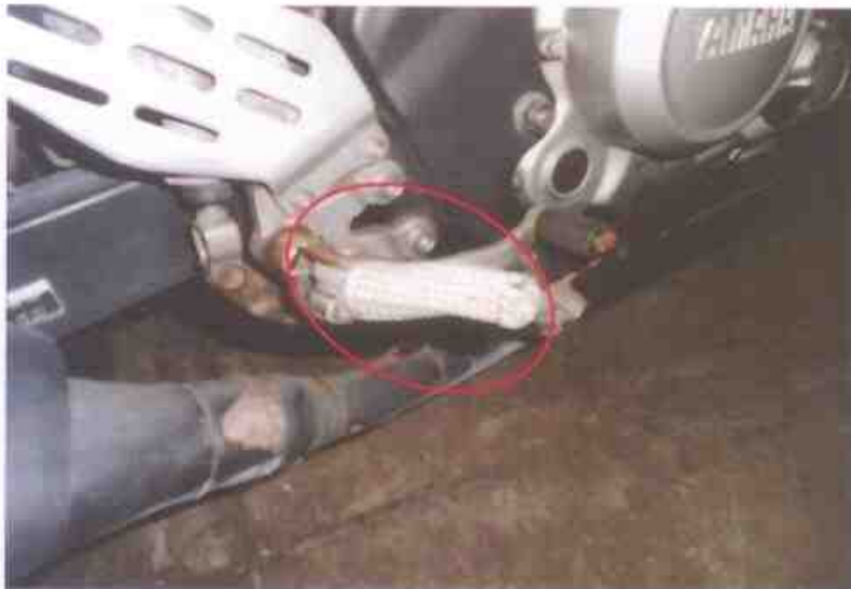
Photo 9 shows a closer view of the right foot rest of the Motorcycle at the time of our inspection. The Motorcycle was observed to have sustained with relatively minor damages due to the accident collision. (Circled)
