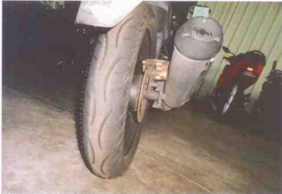
Photo 10 shows the rear tyre of the Motorcycle. The rear tyre was observed to be in serviceable condition with remaining tread depth of approximately 5mm. The tyre was also observed to be sufficiently inflated for vehicular operation.
