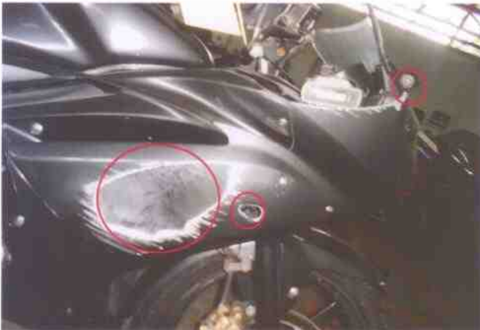
Photo 6 shows a closer view of the missing front right signal lamp, scratched portion of the side fairing & missing wing mirror of the Motorcycle at the time of our inspection. The Motorcycle was observed to have sustained with relatively minor damages due to the accident collision. (Circled)
