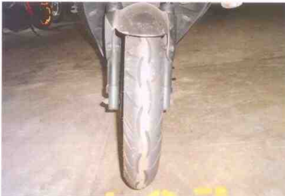
Photo 11 shows the front tyre of the Motorcycle. The front tyre was observed to be in serviceable condition with remaining tread depth of approximately 5mm. The tyre was also observed to be sufficiently inflated for vehicular operation.
