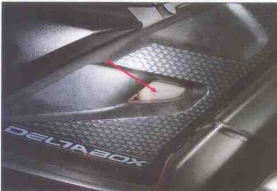
Photo 17 shows our checks on the brake fluid (rear) reservoir had also indicated that the brake fluid was of sufficient level for operational purposes, and without contamination.
