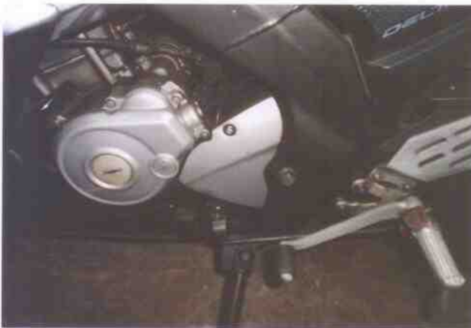
Photo 13 shows no sign(s) or indication(s) of fluid leakage stain observed around the engine area of the Motorcycle.
