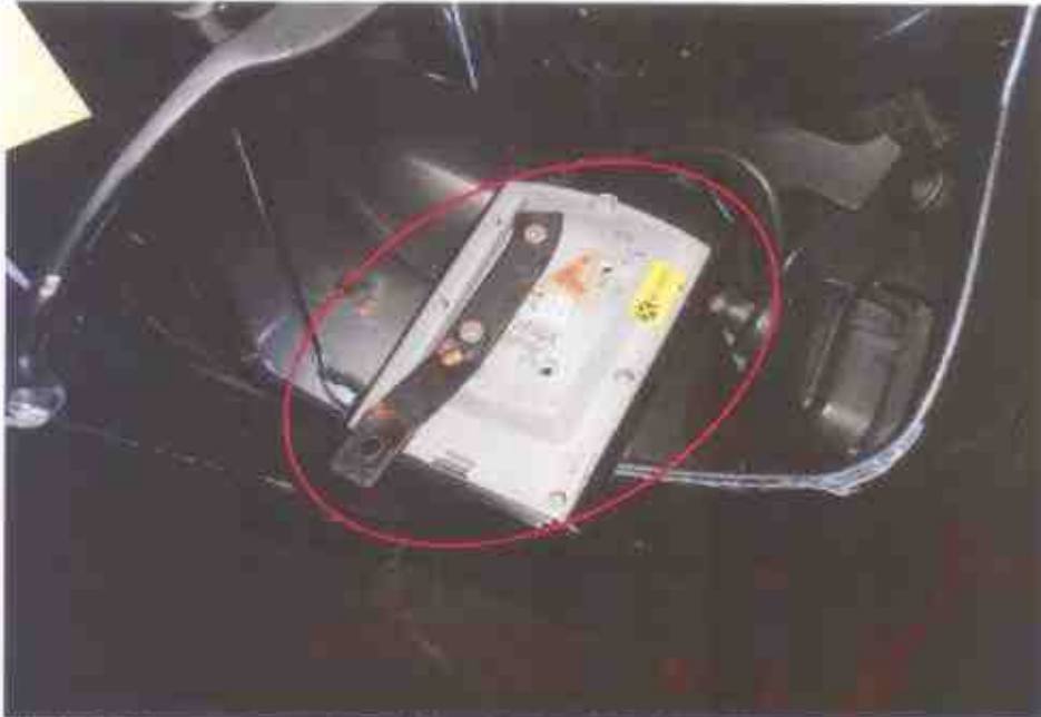
Photo 7 shows a closer view of the dislodged UI of the Motorcycle at the time of our inspection. It was observed to be dislodged due to the accident collision. (Circled)
