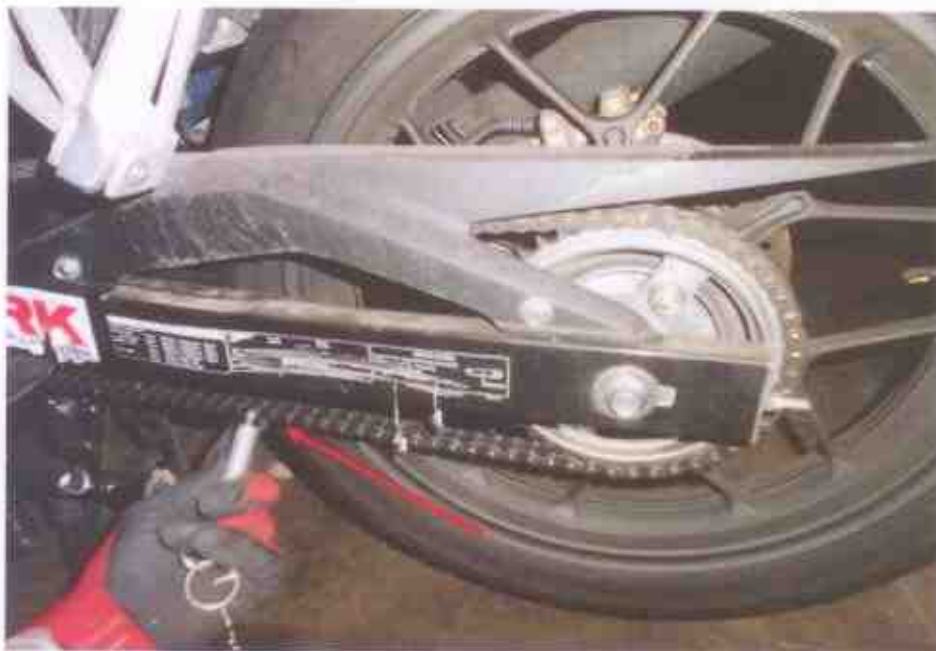
Photo 14 shows the general view of the gear train (arrowed) of the Motorcycle, which was observed to be intact with no misalignment. It was also adequately lubricated for operating purposes. However, free play tension test was unable to be conducted due to the stuck foot rest in between the gear chain due to the accident.
