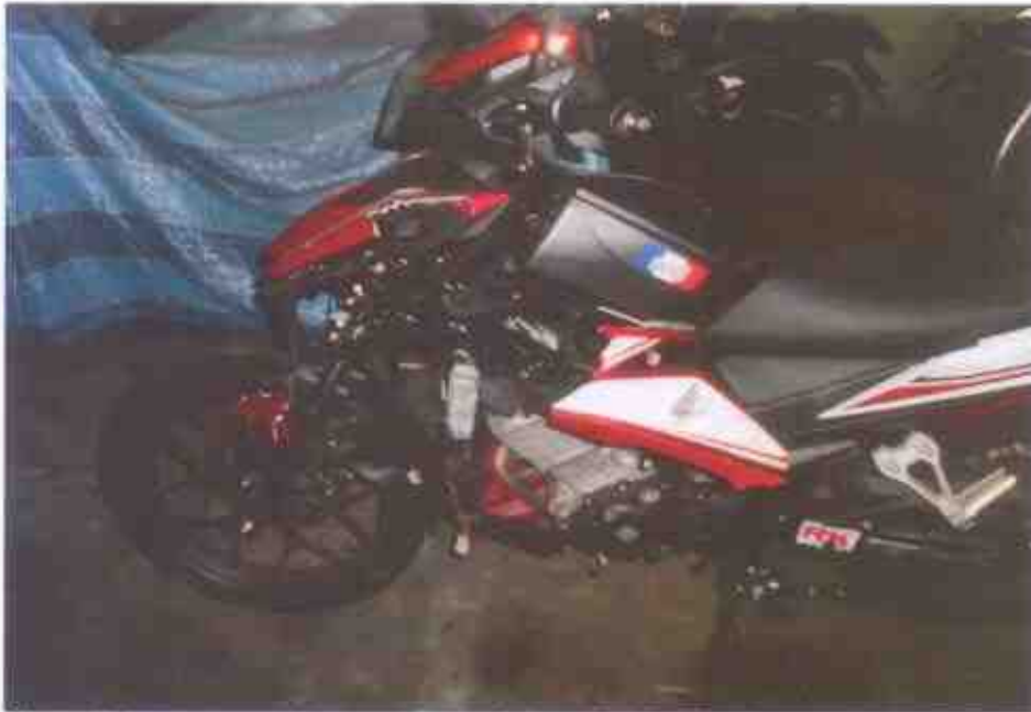
Photo 5 shows a semi close-up view of the left side of the Motorcycle at the time of our inspection. It was observed to have sustained with extensive damages on the ignition system, left-side fairing, left signal lamp & shift gear pedal/ foot rest due to the accident collision.
