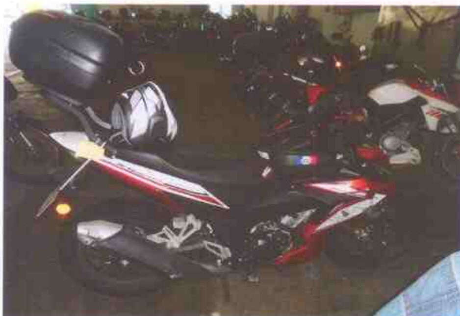
Photo 4 shows a general view of the right side portion of the Motorcycle at the time of our inspection. The Motorcycle was observed to be sustained relatively minor impact on the right side portion likely due to the accident collision.
