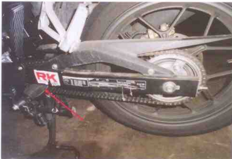
Photo 13 shows the general view of the gear train (arrowed) of the Motorcycle, which was observed to be intact with no misalignment. However, free play tension test was unable to be conducted due to the stuck foot rest in between the gear chain.
