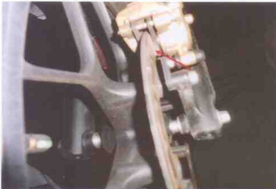
Photo 19 shows the front brake pad at time of our inspection. The frictional material was observed to be at a sufficient level for operational purposes.
