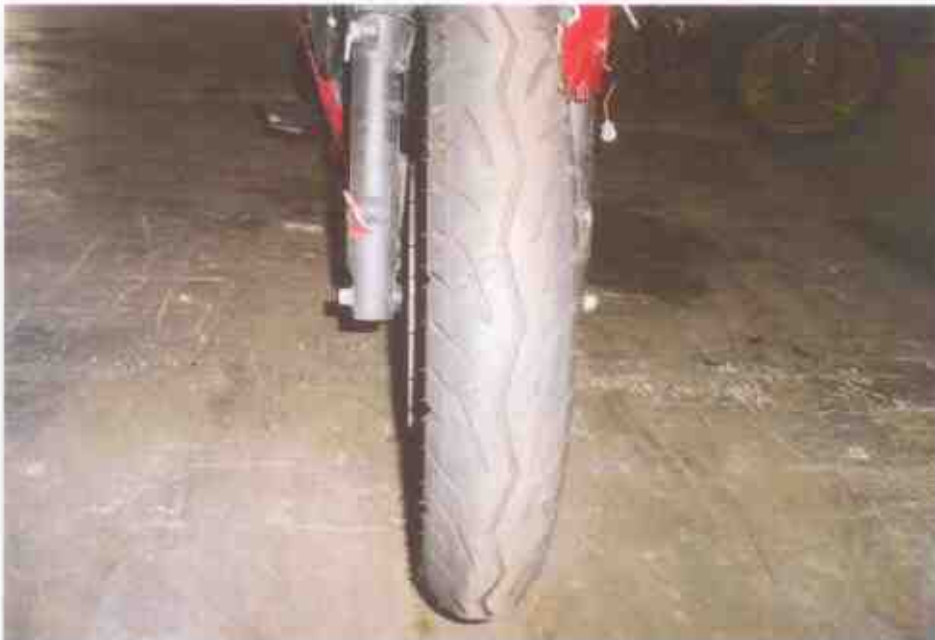
Photo 10 shows the front tyre of the Motorcycle. The pattern of the tread was clearly visible. There was no tear, burst mark(s) and/or punctured hole(s) on the sidewalls as well as across the tread of the front tyre.
