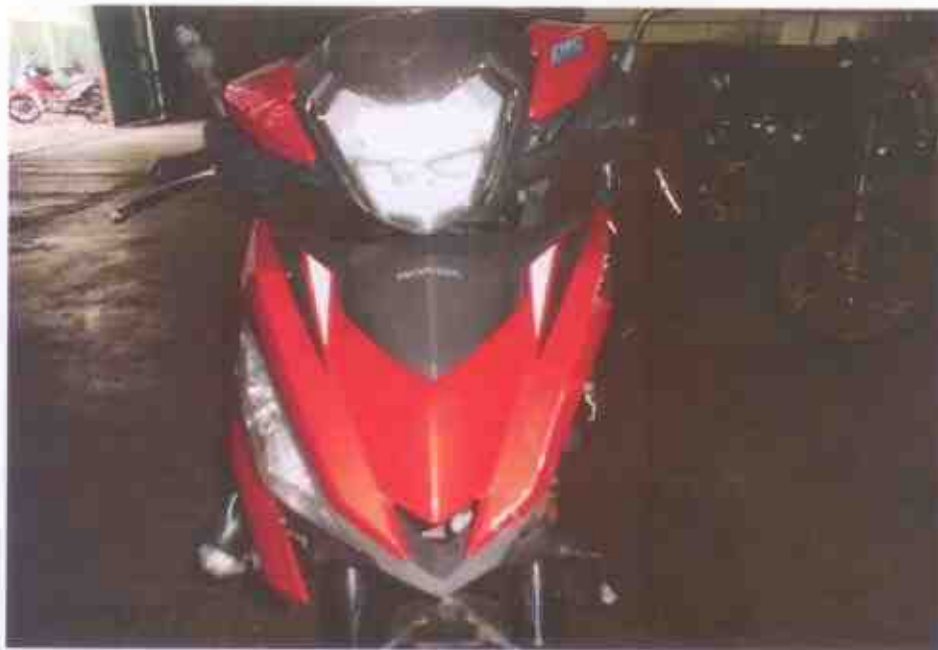
Photo 15 shows the handle bar was observed to be misaligned as a result of the accident. Hence, we are not able to conduct any tests on the steering system of the Motorcycle.
