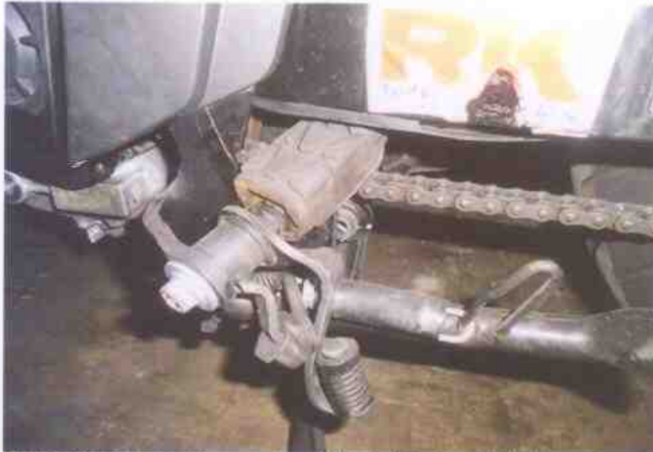
Photo 16 shows the close-up view of the stuck foot rest in between the gear chain as a result of the accident.
