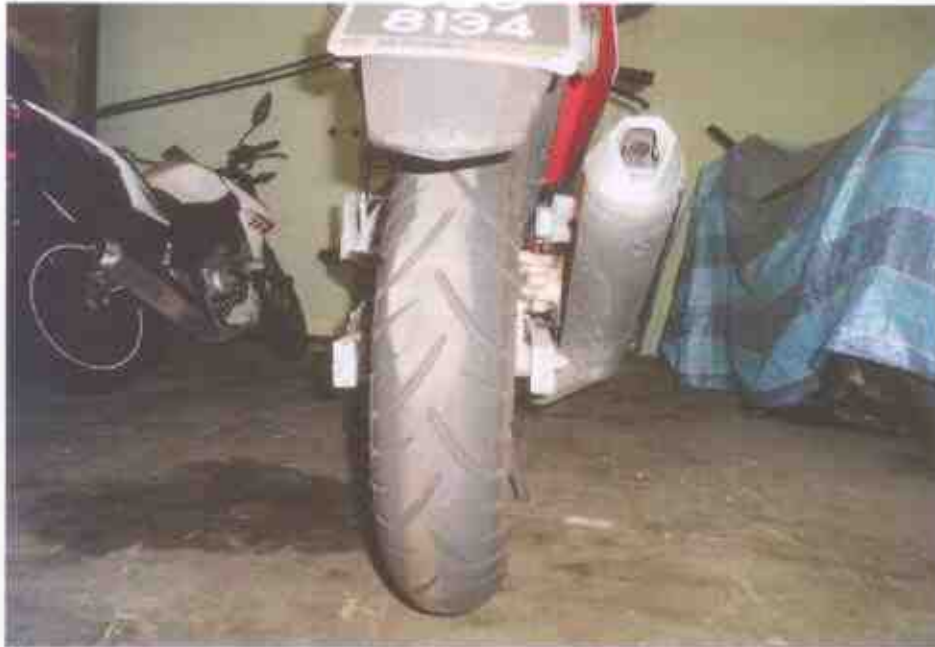
Photo 9 shows the rear tyre of the Motorcycle at the time of our inspection. The rear tyre was observed to be in serviceable condition with remaining tread depth of approximately 4mm. The tyre was also observed to be sufficiently inflated for vehicular operation. There was no significant damage observed on the rear wheel rim & tyre.
