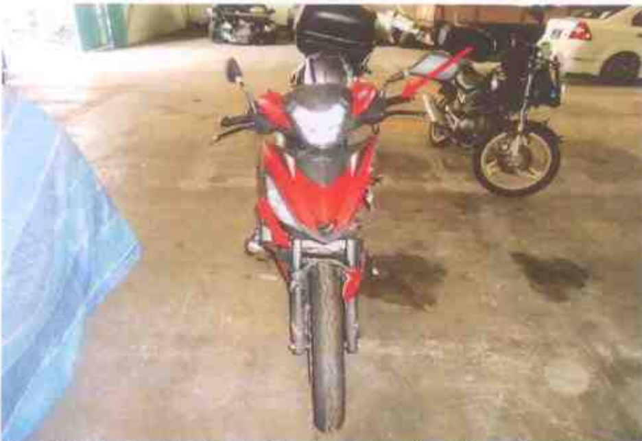
Photo 2 shows a general view of the front body of the Motorcycle at the time of our inspection. The Motorcycle was observed to be sustained with relatively extensive impact due to the accident collision. Amongst the body parts damaged was its handle bar (arrowed), which was observed to be misaligned.
