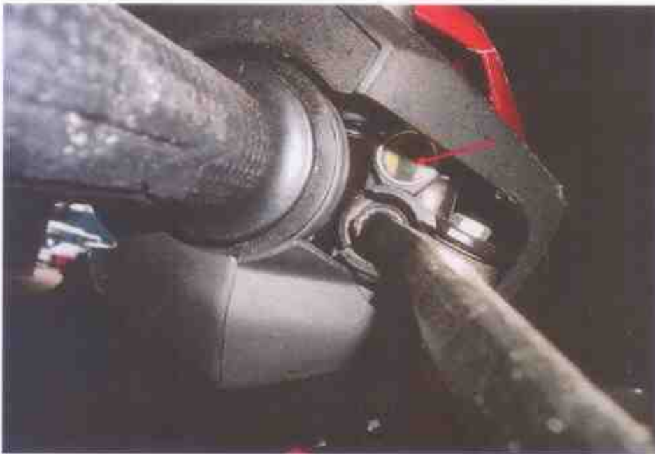
Photo 18 shows the front brake fluid reservoir at time of our inspection. It was observed to be at a sufficient level without any contamination.
