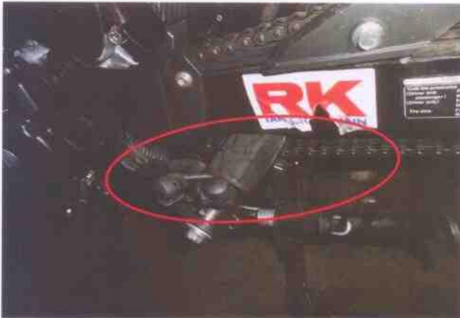
Photo 12 shows the free play tension test was unable to be conducted due to the stuck foot rest in between the gear chain likely due to the accident's collision impact.
