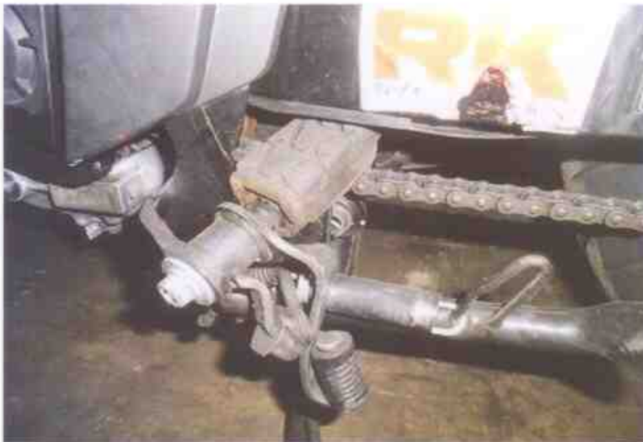
Photo 8 shows a close-up view of the stuck foot pedal in between the gear chain of the Motorcycle at the time of our inspection. It was likely due to the accident collision.
