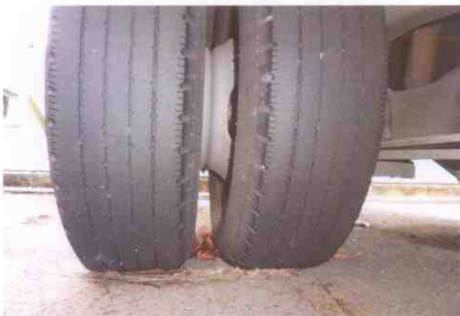
Photo 12 shows the condition of the rear right tyres of the Motor Lorry, which were observed to be in serviceable condition with remaining tread depth of approximately 2mm.
