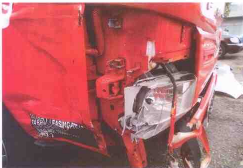
Photo 3 shows a damaged headlamp, lower bumper and right door likely due to the accident's impact.
