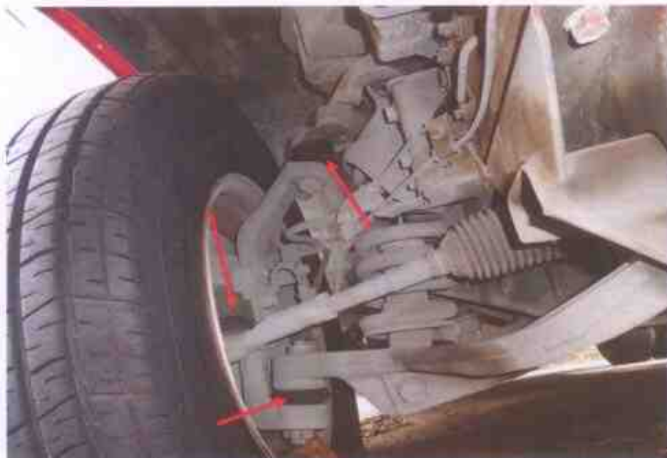
Photo 18 shows the various undercarriage components at the front right wheel of the Motor Lorry, in particular the steering tie rod end (arrowed). The various undercarriage components of the Motor Lorry were all found to be intact without any visible damage. There was also no sign of fluid stain(s) observed on the various undercarriage components.
