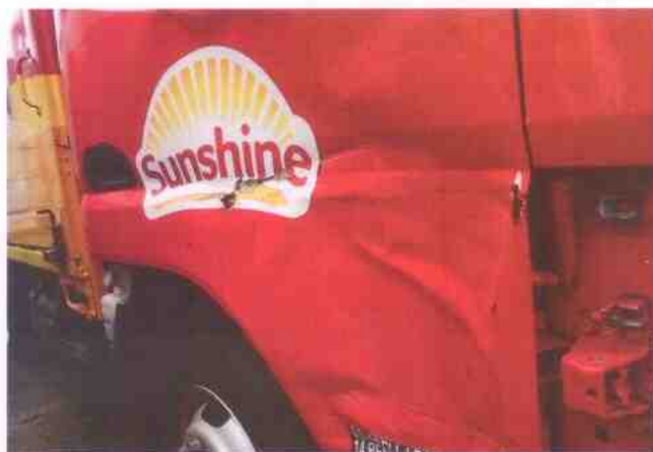
Photo 4 shows the close-up view of the damaged right door of the Motor Lorry. It was observed to have sustained damages as a result of the accidents.
