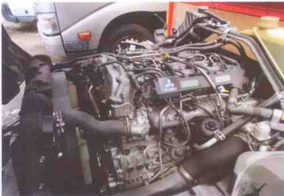
Photo 13 shows a general view of the Motor Lorry's engine compartment, which was accessed by lifting the front cabin of the Motor Lorry. The various parts and components inside the engine compartment were unaffected by the accident. There was also no sign(s) or indication(s) of fresh fluid leakage and/or fluid stain within the engine.
