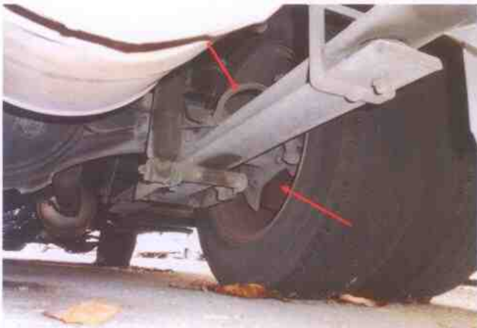
Photo 19 shows the various undercarriage components at the rear right wheels of the Motor Lorry. There was no sign(s) of brake fluid leakage along the brake hoses and brake pipes.
