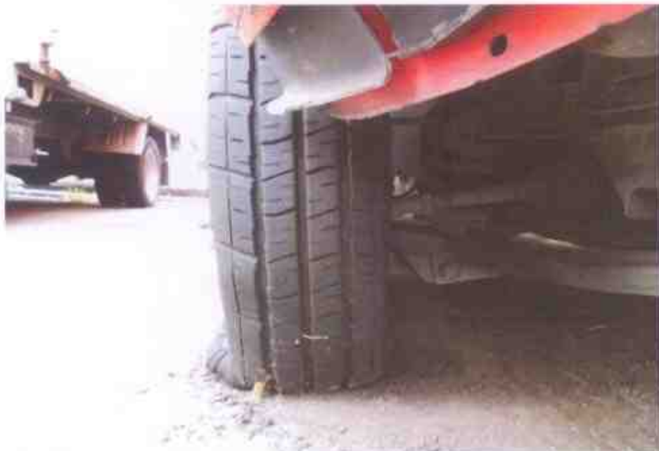
Photo 8 shows the condition of the front right tyre of the Motor Lorry, which was observed to be deflated & torn at the outer sidewall as a result of the accident. The remaining tread depth was measured at approximately 6mm.
