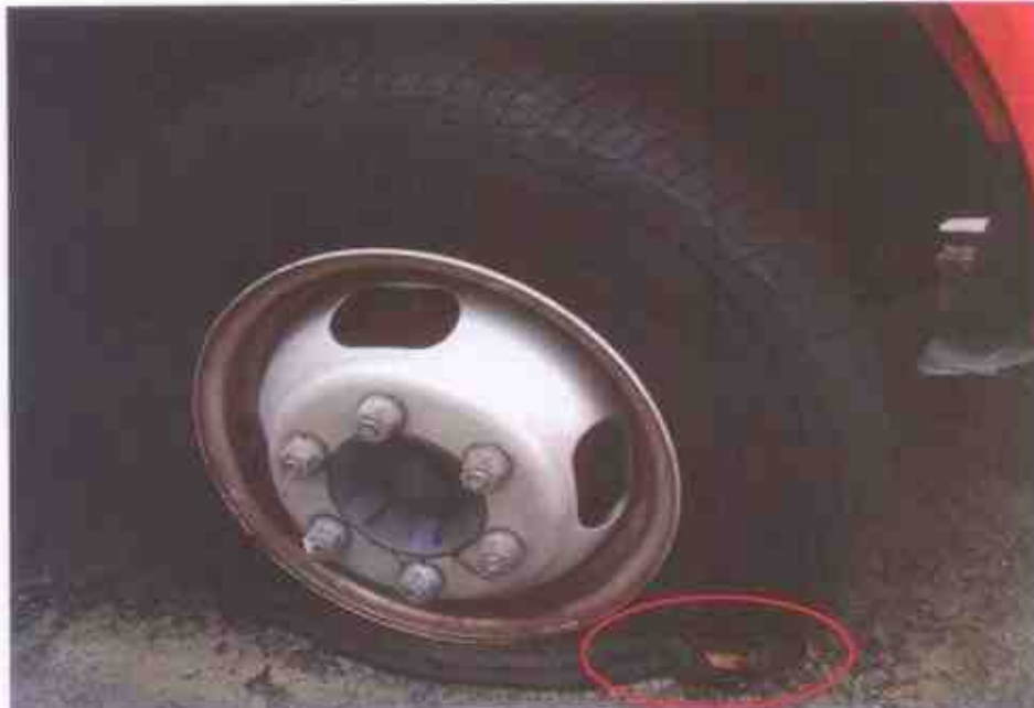
Photo 9 shows the condition of the front right tyre of the Motor Lorry, which was observed to be deflated & torn at the outer sidewall as a result of the accident. The remaining tread depth was measured at approximately 6mm.
