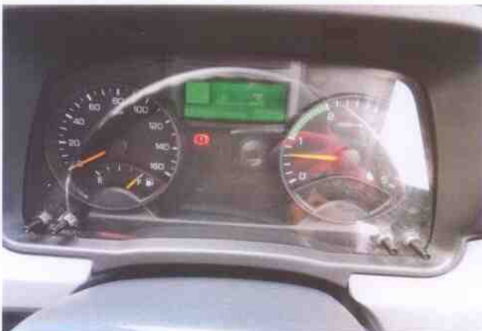
Photo 22 shows no warning lights illuminated on the instrument panel of the Motor Van after the engine was cranked. This would suggest that there was no abnormality to the various electronic operating systems of the Motor Car.
