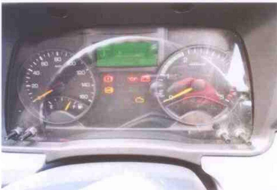
Photo 21 shows the warning lights for the various electronic operating systems of the Motor Car appearing on its instrument panel during the self-test when the engine was cranked.
