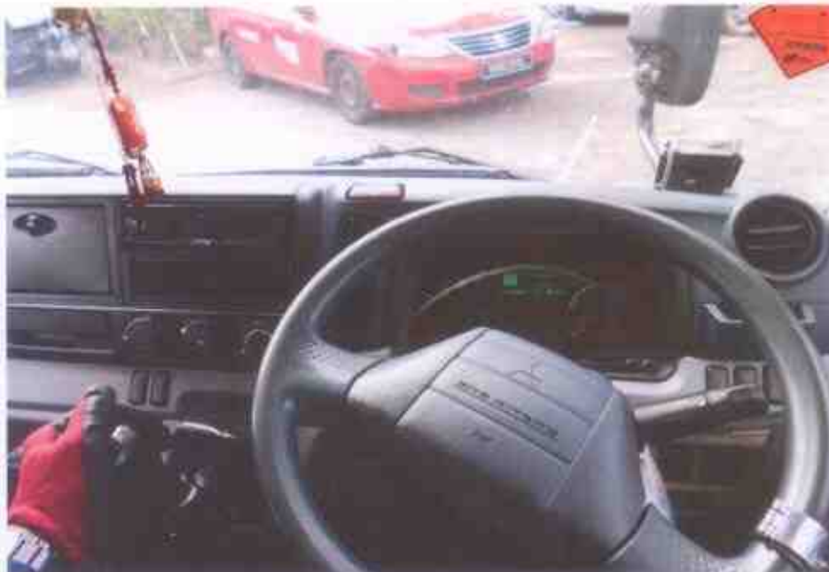
Photo 24 shows the operational test on the Motor Lorry. It was observed to be in serviceable condition. Operational test such as moving forward, reverse, turn left & right and also braking test on the Motor Lorry was conducted successfully.
