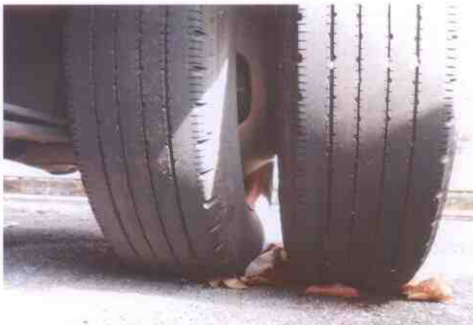
Photo 11 shows the condition of the rear left tyres of the Motor Lorry, which was observed to be in serviceable condition with remaining tread depth of approximately 3mm. The tyres, which were wrapped around standard alloy wheel rim, were also observed to be sufficiently inflated for vehicular operation.
