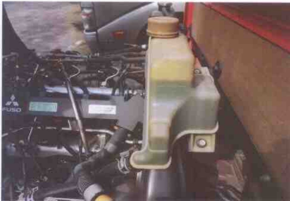
Photo 16 shows the power steering fluid of the Motor Lorry at the time of our inspection. The fluid was observed to be of sufficient level and without any visible contamination.
