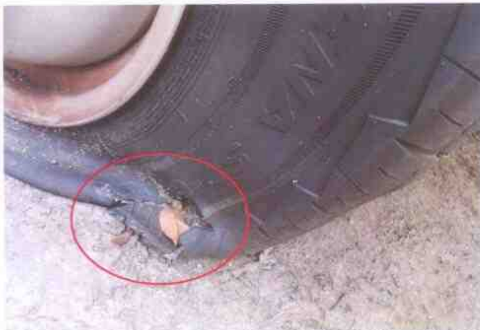
Photo 10 shows the close-up view condition of the front right tyre of the Motor Lorry, which was observed to be deflated & torn at the outer sidewall as a result of the accident. The remaining tread depth was measured at approximately 6mm.
