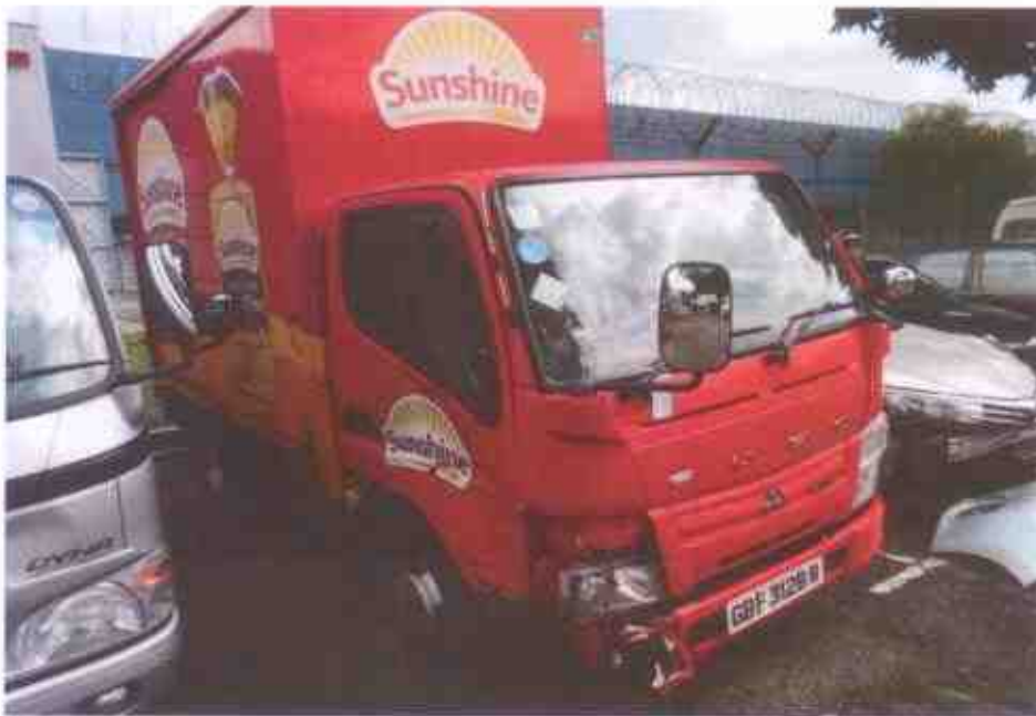
Photo 2 shows a general view of the front portion of the Motor Lorry at the time of our inspection. The Motor Lorry was observed to have sustained minor damages at its front right headlamp, front right lower bumper and its right driver door were amongst the body parts that were damaged as a result of the accident.
