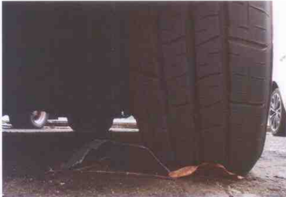
Photo 7 shows the condition of the front left tyre of the Motor Lorry, which was observed to be in serviceable condition with remaining tread depth of approximately 5mm. The tyre, which was wrapped around standard alloy wheel rim, was also observed to be sufficiently inflated for vehicular operation.
