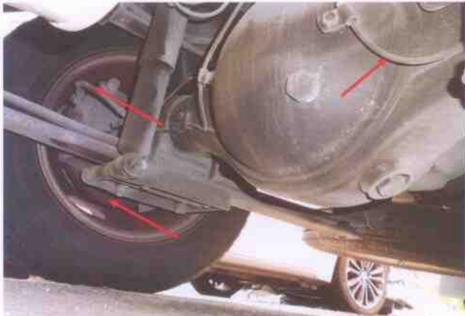
Photo 20 shows the various undercarriage components at the rear left wheels of the Motor Lorry. There was no sign(s) of brake fluid leakage along the brake hoses and brake pipes.
