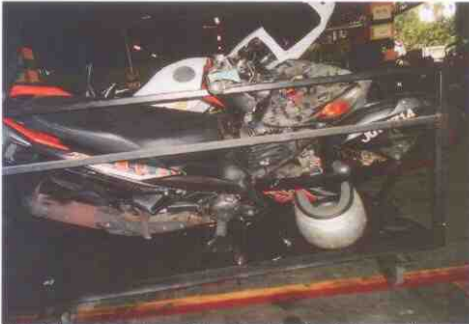
Photo 6 shows a general view of the right portion of the Motorcycle at the time of our inspection. The Motorcycle was observed to have sustained relatively extensive impact including damages to the steering system as a result of the accident collision.
