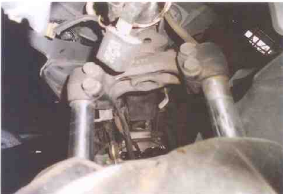
Photo 5 shows a close-up view of the front fork of the Motorcycle at the time of our inspection. It was observed to be bent due to the accident collision.
