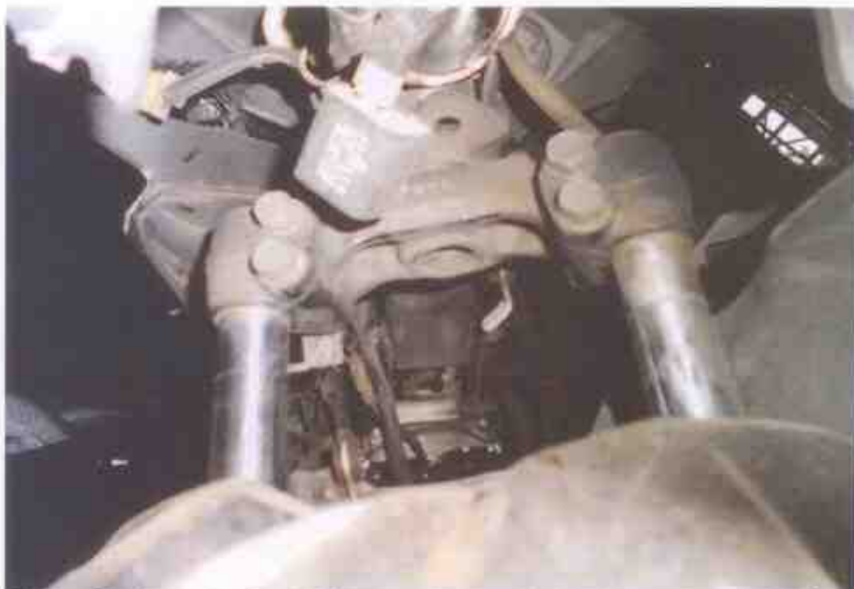
Photo 18 shows the front fork was observed to be bent as a result of the accident. Hence, we are unable to conduct any tests on the steering system of the Motorcycle.
