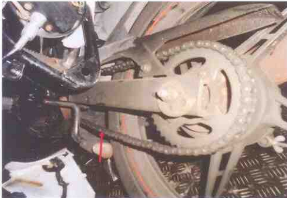
Photo 12 shows the general view of the gear train (arrowed) of the Motorcycle, which was observed to be intact with no misalignment. It was also adequately lubricated for operating purposes.
