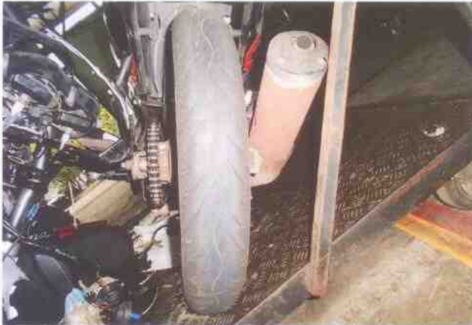
Photo 7 shows the rear tyre of the Motorcycle at the time of our inspection. The rear tyre was observed to be in serviceable condition with remaining tread depth of approximately 3mm. The tyre was also observed to be sufficiently inflated for vehicular operation. There was no significant damage observed on the rear wheel rim & tyre.
