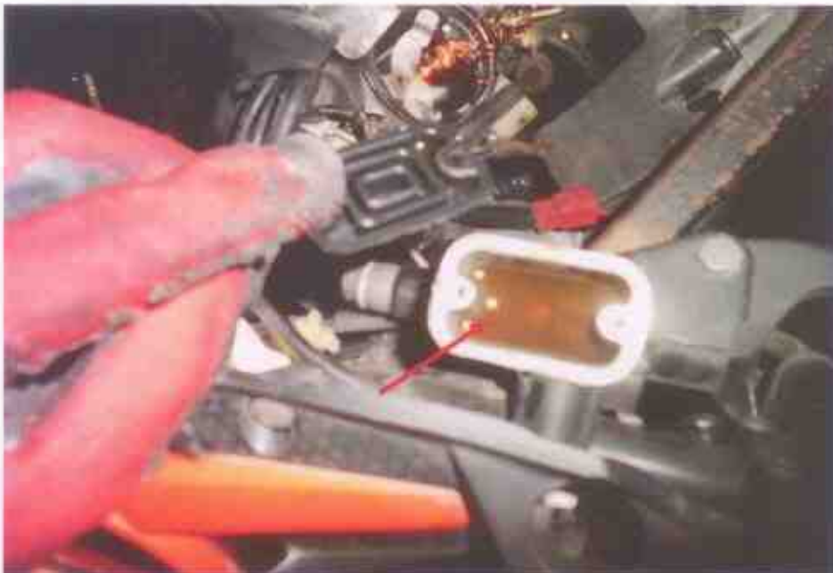
Photo 15 shows the front brake fluid reservoir (arrowed) was observed to be unaffected by the accident. It was observed to be of sufficient level & not contaminated at the time of our inspection.
