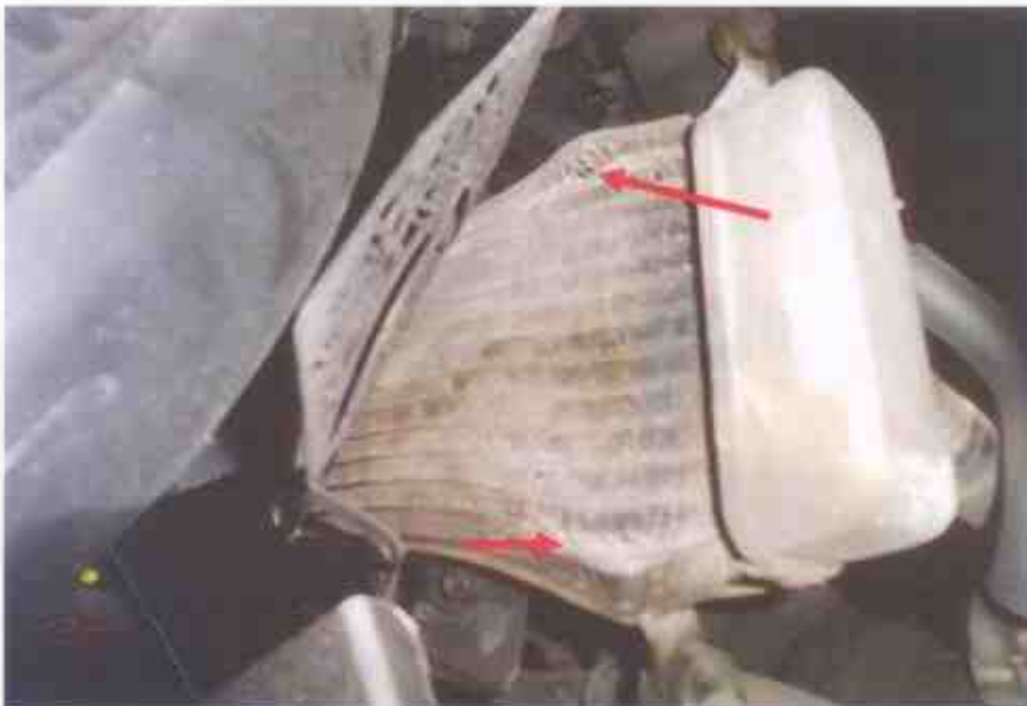
Photo 11 shows the close-up view of the corrugated radiator as a result of the accident's impact collision.
