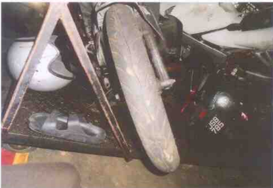
Photo 8 shows the front tyre of the Motorcycle at the time of our inspection. The pattern of the tread was clearly visible with remaining tread depth of approximately 3mm. There was no tear, burst mark(s) and/or punctured hole(s) on the sidewalls as well as across the tread of the front tyre.
