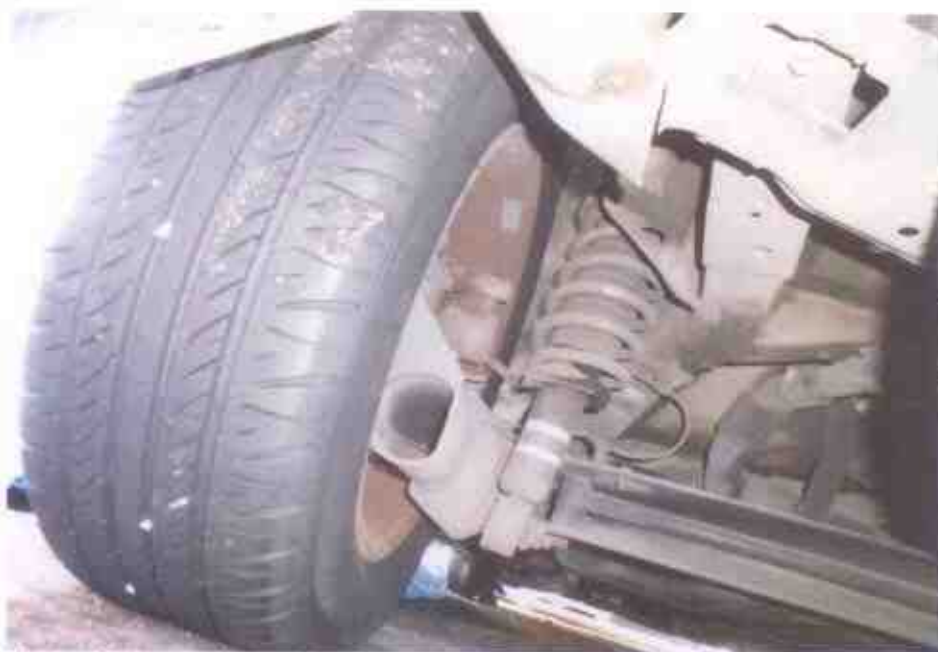
Photo 22 shows the braking & steering components at the left right wheel of the Motor Car. We did not observe any leakage of brake fluid at the time of our inspection of the Motor Car.
