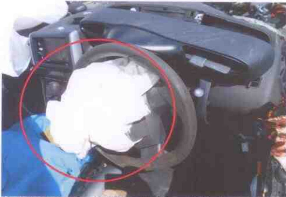
Photo 23 shows the Supplemental Restraint System (SRS) of the Motor Car was however likely to be in normal operating condition at the material time of the accident. The evidence of the deployed driver's airbag indicates that the impact sensors and control module of the Motor Car's SRS were all in serviceable condition at the material time of accident.
