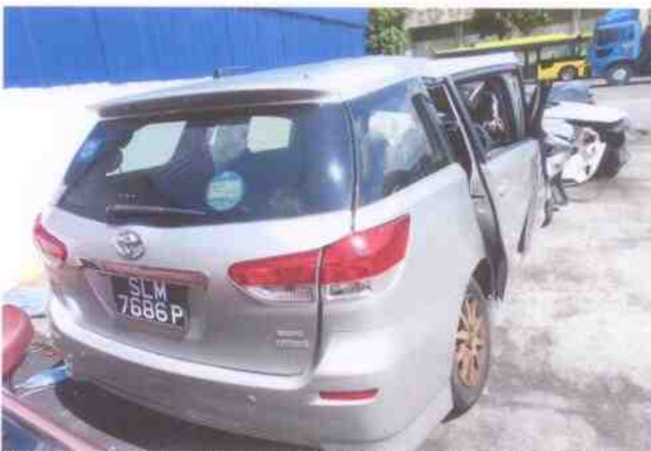
Photo 9 shows a general view of the rear right portion of the Motor Car. The rear portion was observed to be in good condition, no damages found on the Motor Car's body at time of our inspection. However, we found that the rear boot lid sustained minor misalignment due to the accident.
