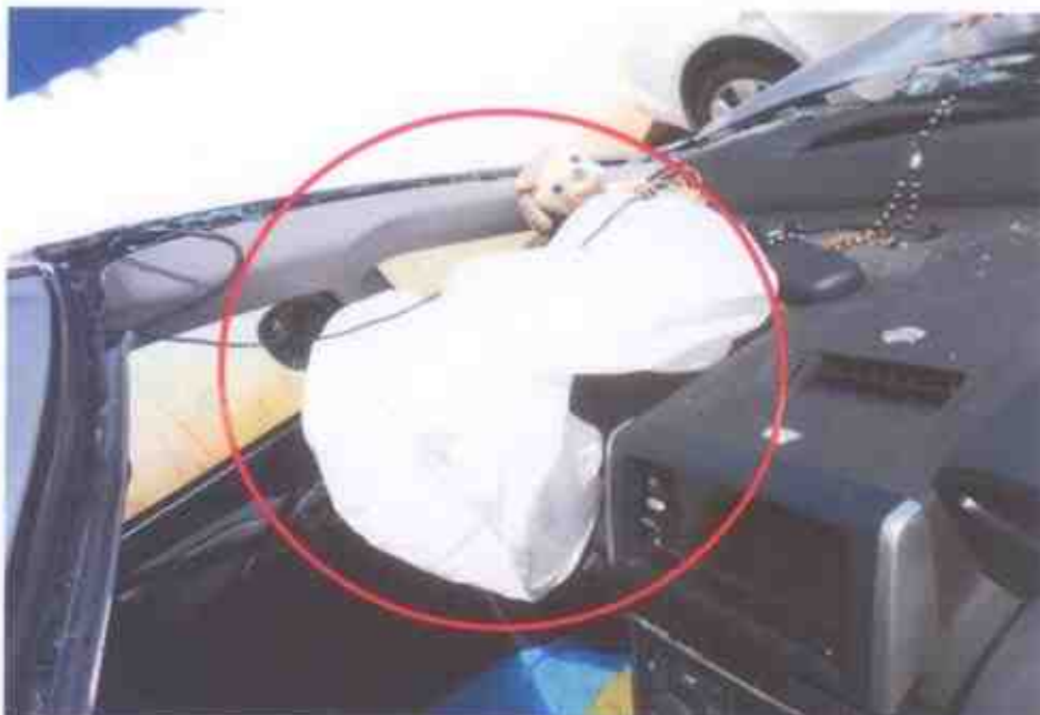
Photo 24 shows the Supplemental Restraint System (SRS) of the Motor Car was however likely to be in normal operating condition at the material time of the accident. The evidence of the deployed passenger's airbag indicates that the impact sensors and control module of the Motor Car's SRS were all in serviceable condition at the material time of accident.
