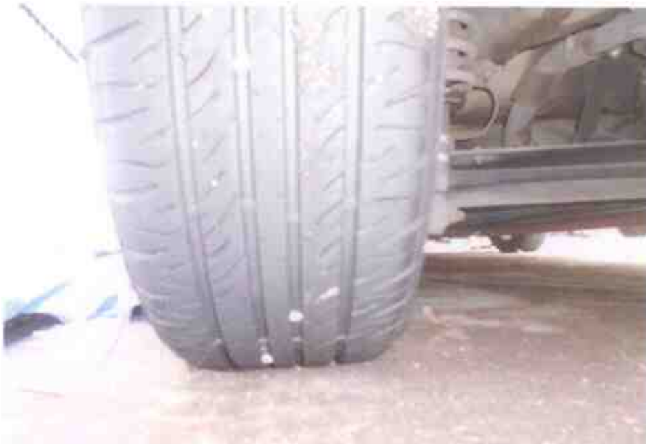
Photo 13 shows the condition of the rear left tyre of the Motor Car, which was observed to be in serviceable condition. The tyre was also observed to be sufficiently inflated for vehicular operation. The remaining tread depth of the front left tyre was approximately 5mm.
