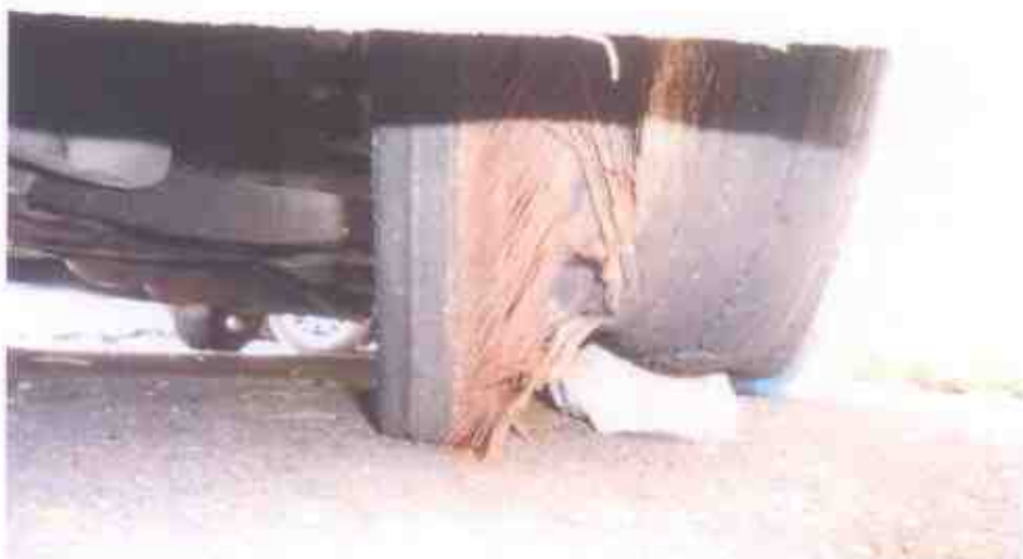
Photo 11 shows the condition of the front left tyre of the Motor Car, which was observed to be torn due to the accident's impact.
