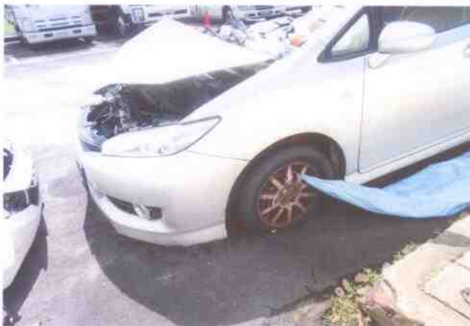
Photo 10 shows the general view condition of the front left tyre of the Motor Car. It was observed to be deflated as a result of the accident.
