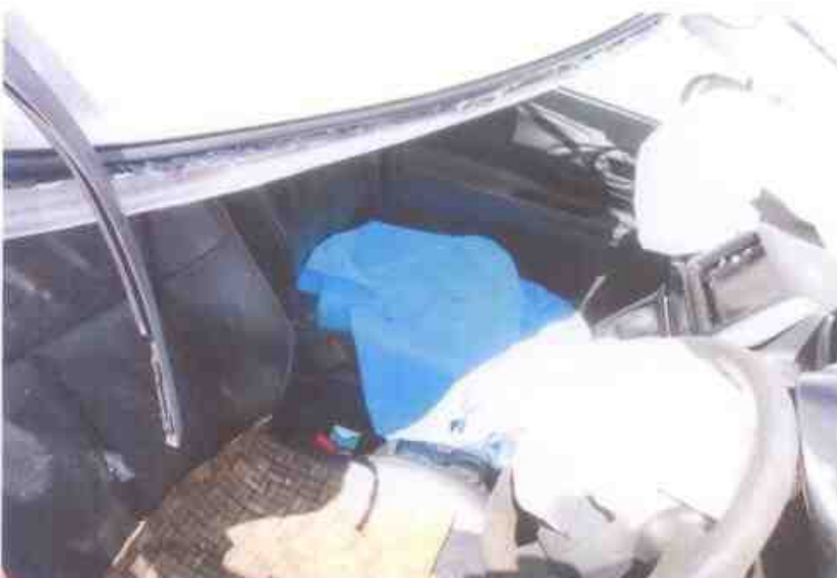
Photo 7 shows a closer view of the interior cabin of the Motor Car. The impact force caused damages to the interior cabin and also activated both driver's & passenger's airbag at time of impact.
