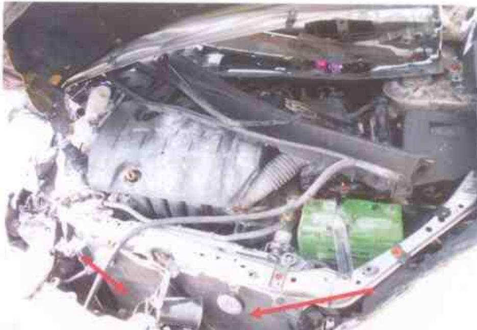
Photo 15 shows the close up view of the radiator's tank that was observed to be damaged likely due to the accident impact.
