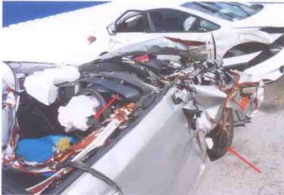
Photo 20 shows the damaged on the steering system of the Motor Car. We were not able to conduct any tests on the steering system of the Motor Car due to the damage to these components. It was observed to be misaligned from its original alignment as a result of the accident.
