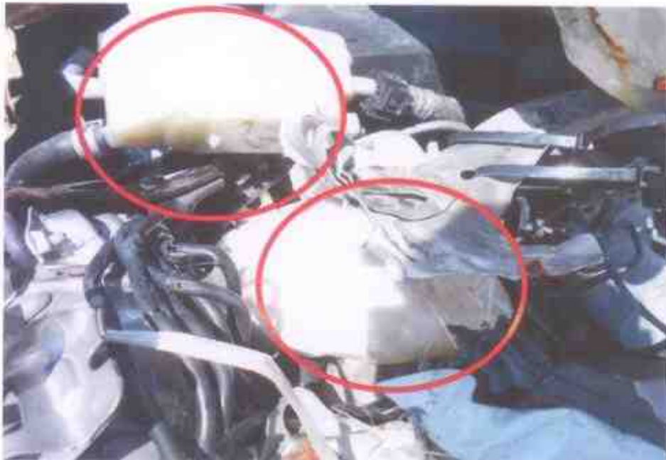
Photo 17 shows the close up view of the engine coolant fluid reservoir & brake fluid reservoir damages due to the accident impact.
