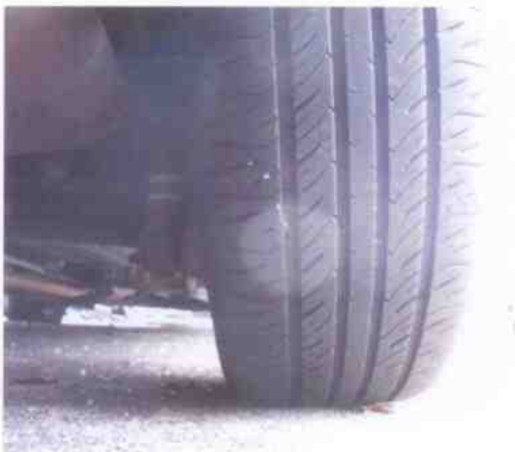
Photo 14 shows the condition of the rear right tyre of the Motor Car, which was observed to be in serviceable condition. The tyre was also observed to be sufficiently inflated for vehicular operation. The remaining tread depth of the front left tyre was approximately 5mm.
