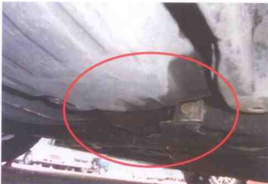
Photo 18 shows the close up view of the fluid leakage at the undercarriage area likely due to the accident impact.
