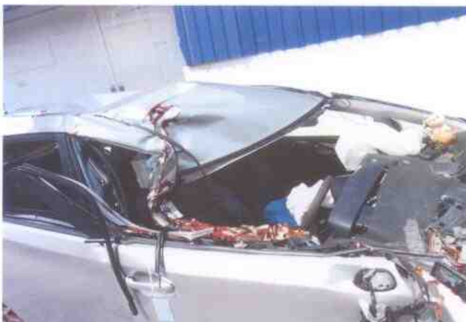
Photo 6 shows a closer view of the damage at the frontal portion of the Motor Car. The impact force was significant, causing extensive damage to the windshield & rooftop amongst others due to the accident.
