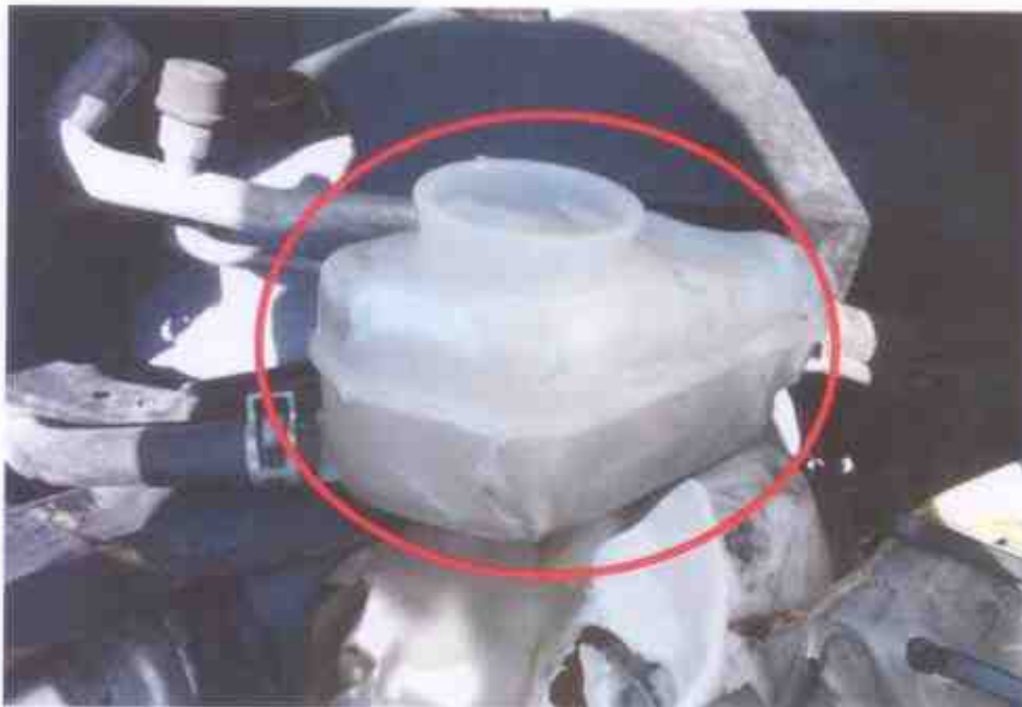
Photo 16 shows the close up view of the brake fluid reservoir that was broken likely due to the accident impact.
