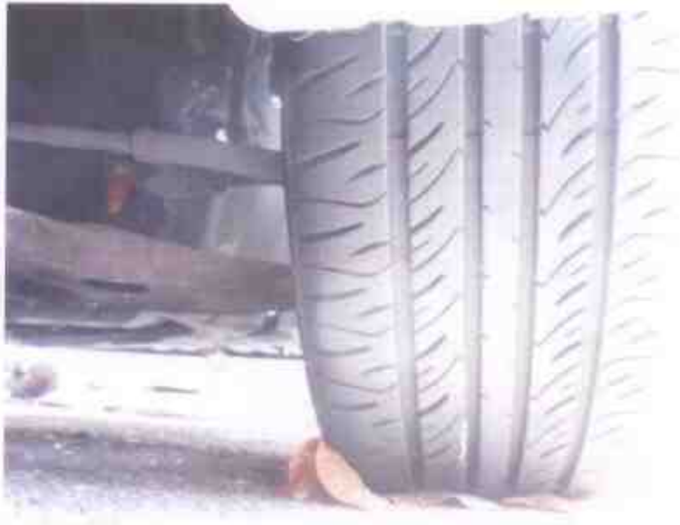
Photo 12 shows the condition of the front right tyre of the Motor Car, which was observed to be in serviceable condition. The tyre was also observed to be sufficiently inflated for vehicular operation. The remaining tread depth of the front left tyre was approximately 6mm.
