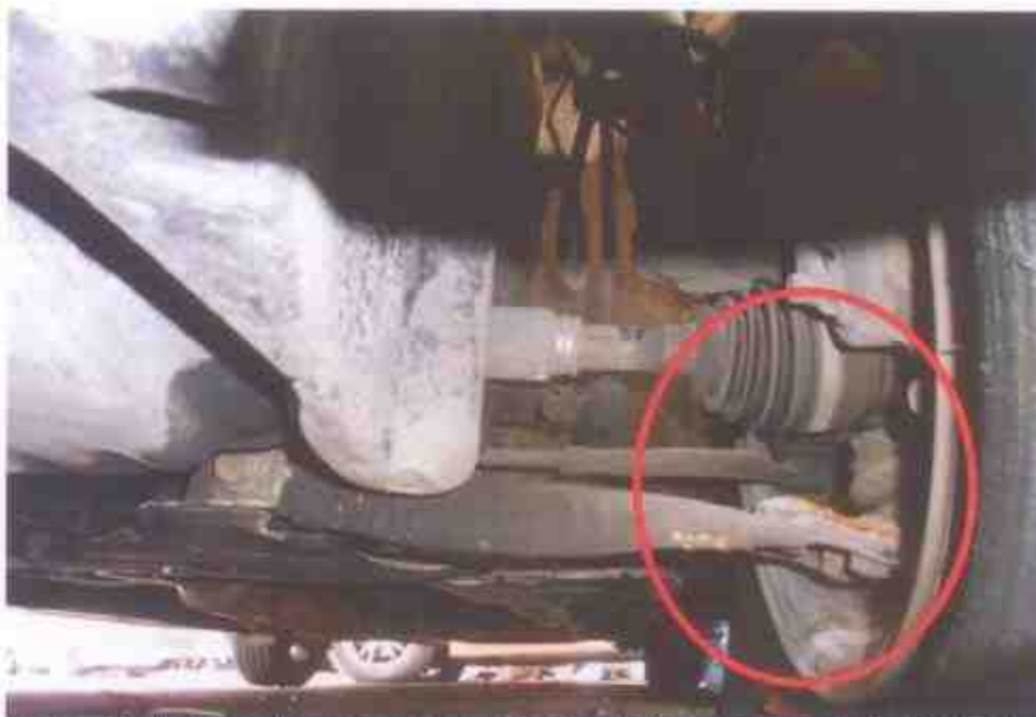
Photo 19 shows a close up view on the front left lower arm of the Motor Car steering system. We were not able to conduct any tests on the steering system of the Motor Car due to the damage to these components as a result of the accident.
