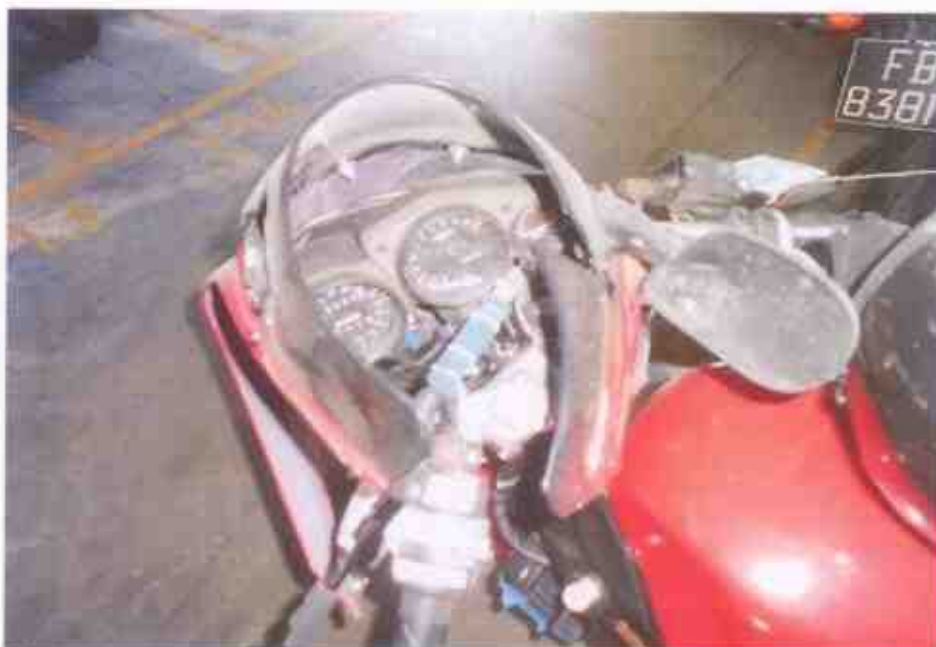
Photo 16 shows the front handle bar was observed to be dislocated as a result of the accident. Hence, we are not able to conduct any tests on the steering system of the Motorcycle.
