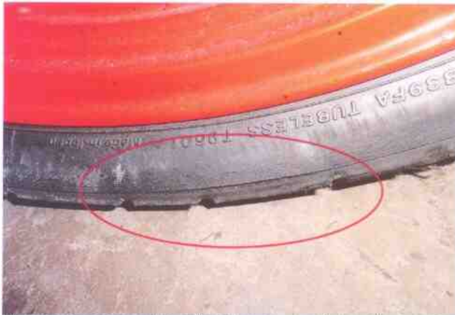
Photo 10 shows the front tyre of the Motorcycle was deflated at the time of our inspection. It was found to have sustained torn mark on the outer sidewall likely due to the accident's impact collision. However, the tread pattern was clearly visible.
