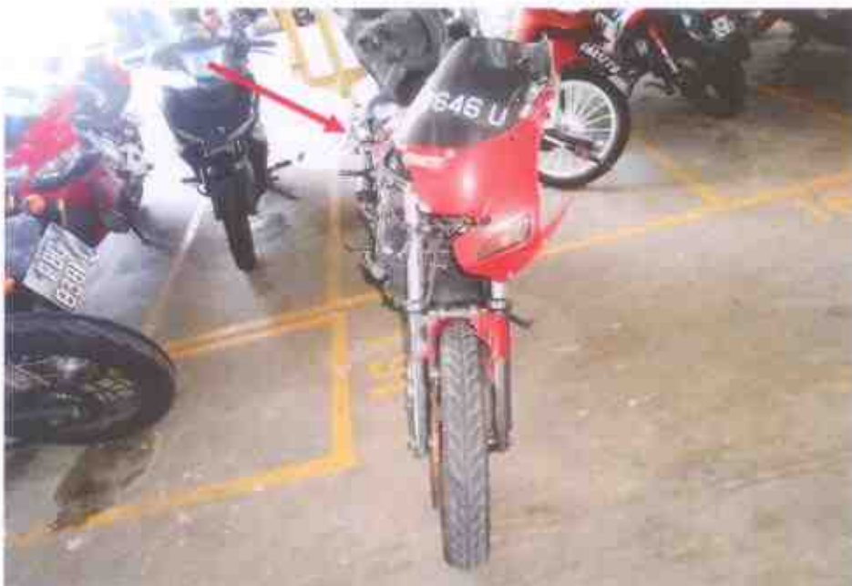
Photo 2 shows a general view of the front body of the Motorcycle at the time of our inspection. The Motorcycle was observed to be sustained with relatively extensive impact due to the accident collision. Amongst the body parts damaged was its handle bar (arrowed), which was observed to be dislocated.
