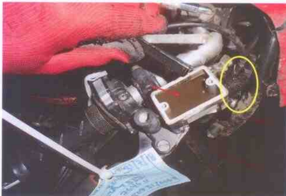
Photo 18 shows the front brake fluid observed to be sufficient at time of our inspection. However, fluid leakage was observed came from the connecting hoses right after the brake fluid reservoir. (Circled)
