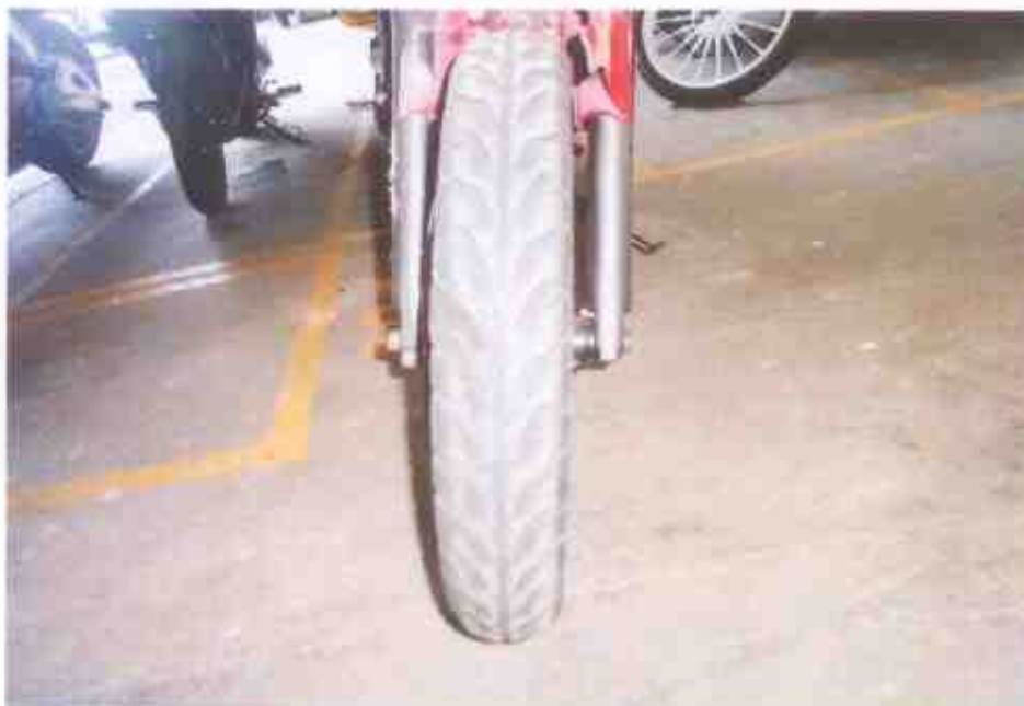
Photo 9 shows the front tyre of the Motorcycle at the time of our inspection. It was found to have sustained torn mark on the outer sidewall likely due to the accident's impact collision. However, the tread pattern was clearly visible.
