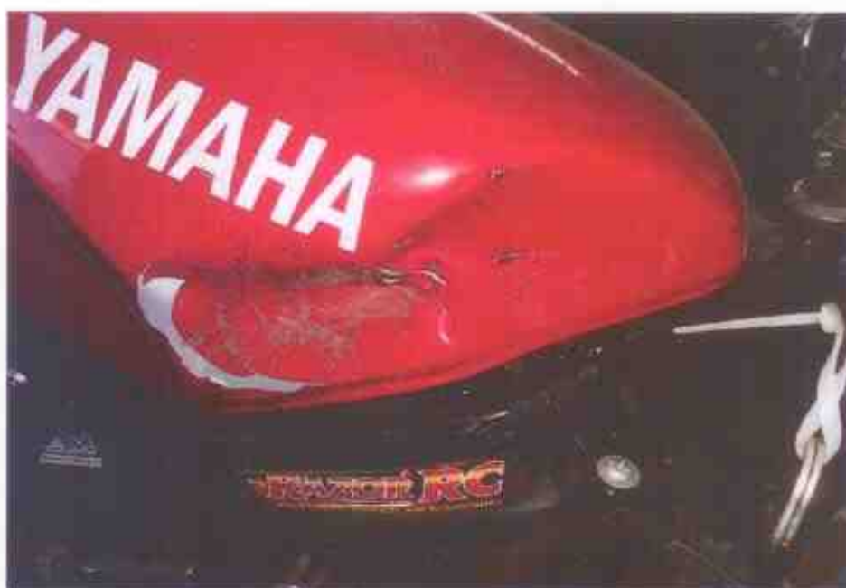
Photo 7 shows a close-up view of the fuel tank of the Motorcycle at the time of our inspection. It was observed to be dented due to the accident collision.
