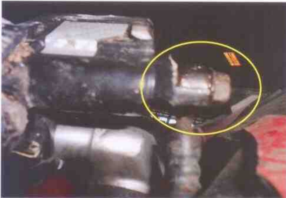
Photo 19 shows the front brake fluid observed to be sufficient at time of our inspection. However, fluid leakage was observed came from the connecting hoses right after the brake fluid reservoir. (Circled)
