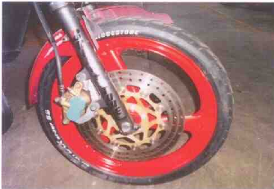
Photo 12 shows the front tyre was wrapped around alloy wheel rim that was found to be without any significant damage.
