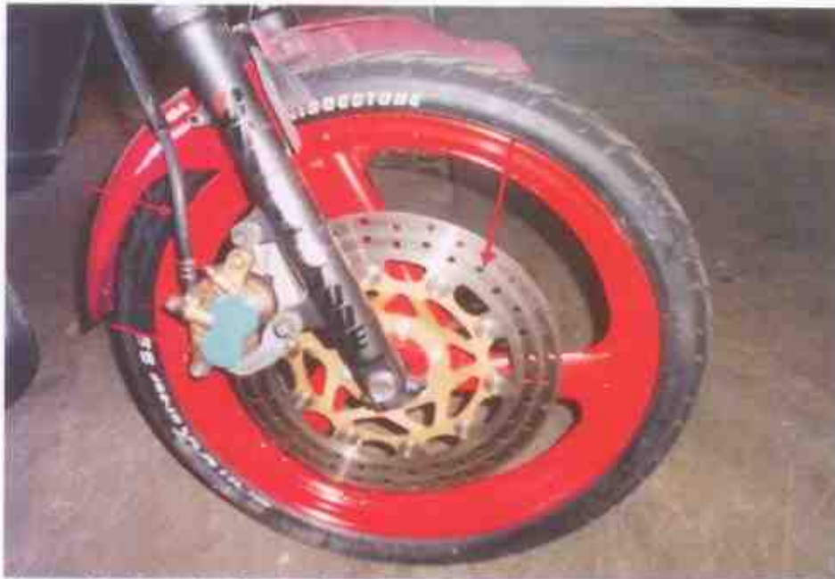
Photo 17 shows the front brake calliper, front brake disc and brake pad of the Motorcycle (arrowed), which are all part of the components in the front brake system of the Motorcycle. Our visual checks of these various components had revealed all to be intact with no visible damage.
