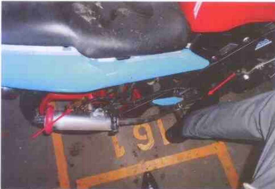
Photo 22 shows a static brake test performed on the rear brake. It was found to be in a serviceable condition.
