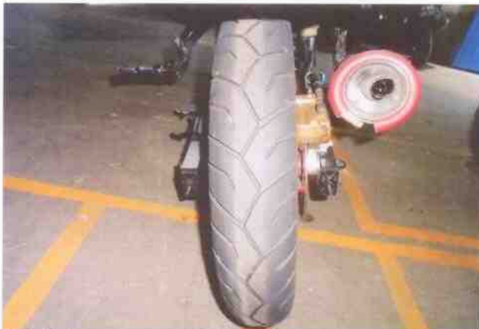
Photo 11 shows the rear tyre of the Motorcycle at the time of our inspection. The rear tyre was observed to be in serviceable condition with remaining tread depth of approximately 4mm. It was also sufficiently inflated for vehicular operation.
