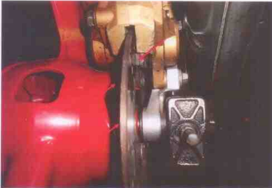
Photo 21 shows the rear brake pad of the Motorcycle (arrowed), which are still with sufficient frictional material for operational purposes.
