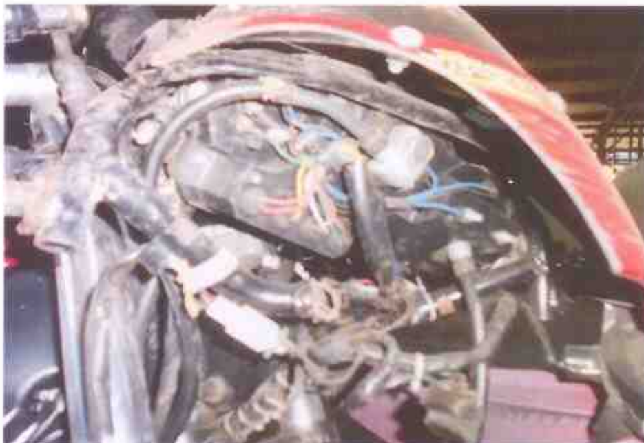
Photo 6 shows a close-up view of the damaged steering system & ignition system of the Motorcycle at the time of our inspection. The Motorcycle was observed to be sustained relatively extensive impact due to the accident collision.
