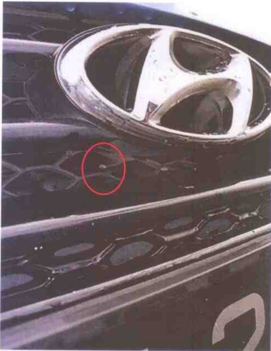
Photo 2 shows a general view of the cracked (circled) radiator grille of the Motor Taxi. This was directly at the centre of the Motor Taxi's frontal portion, above the front number plate. Apart from this cracked radiator grille, all other body parts at the frontal portion of the Motor Taxi were undamaged and re-usable as indicated in the Vehicle Damage Inspection Report of the Motor Taxi dated 13 January 2017.
