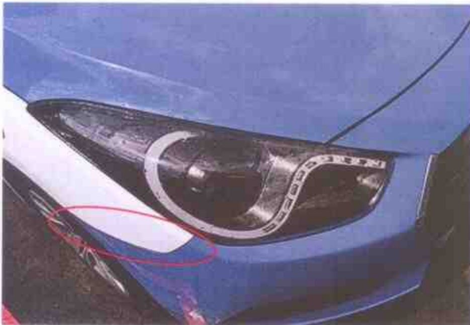
Photo 5 shows no obvious misalignment at the corner edges of the Motor Taxi's front bumper, adjacent to its front right fender (circled). This would indicate that the impact onto the frontal portion of the Motor Taxi was relatively light/minor.
