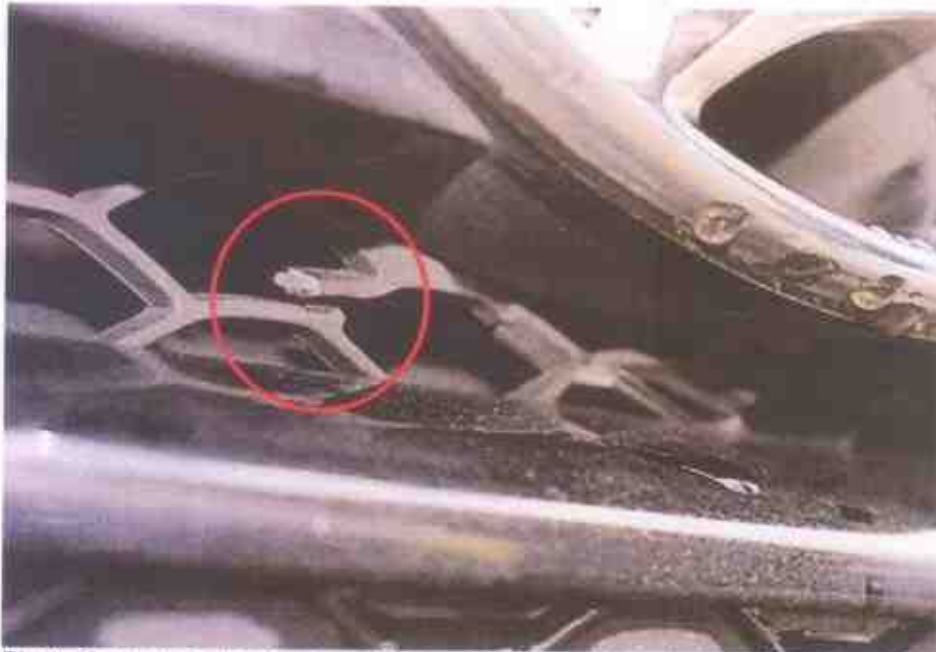
Photo 3 shows a closer view of the cracked (circled) radiator grille of the Motor Taxi. Apart from this cracked radiator grille, all other body parts at the frontal portion of the Motor Taxi were undamaged and re-usable as indicated in the Vehicle Damage Inspection Report of the Motor Taxi dated 13 January 2017.
