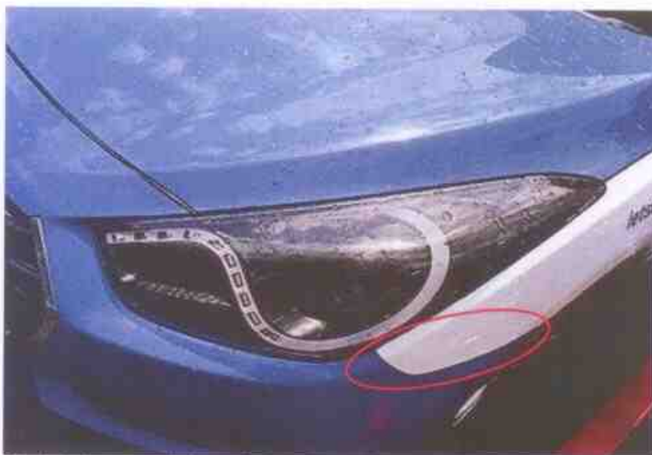
Photo 6 shows no obvious misalignment at the corner edges of the Motor Taxi's front bumper, adjacent to its front right fender (circled). This would indicate that the impact onto the frontal portion of the Motor Taxi was relatively light/minor.
