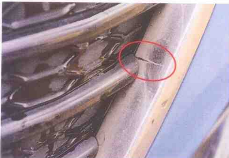
Photo 4 shows the cracked (circled) radiator grille chrome moulding of the Motor Taxi. This was towards the left of the Motor Taxi's frontal portion. This damage was indicated as old damage in the Vehicle Damage Inspection Report of the Motor Taxi dated 13 January 2017.
