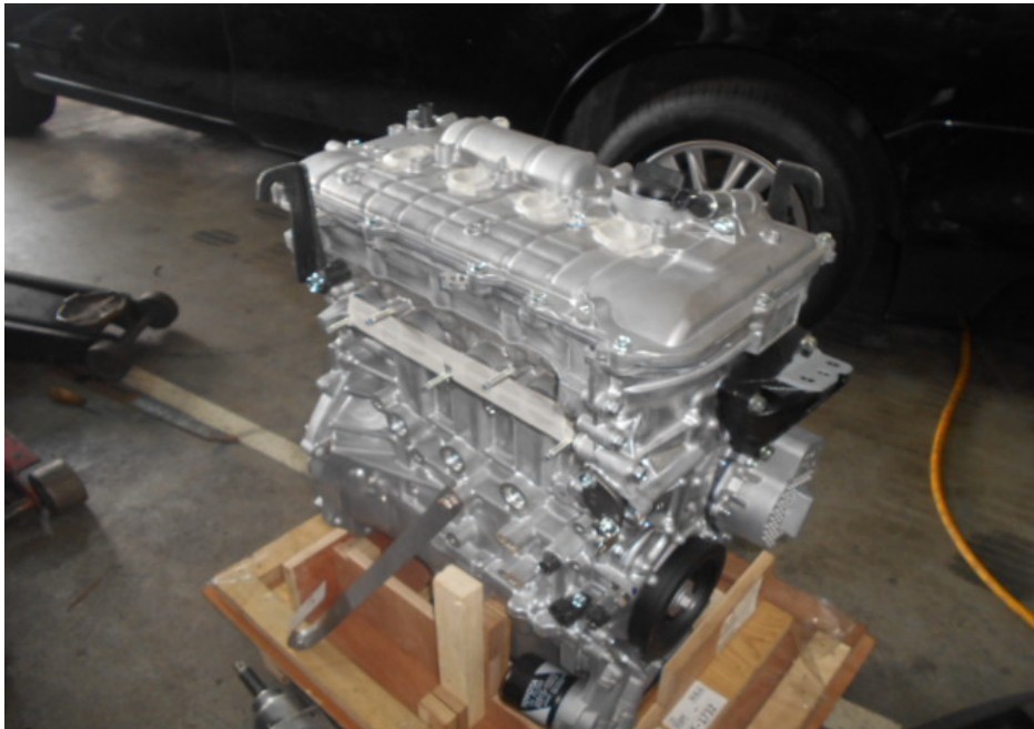
Photo 1 shows a general view of the Toyota engine that I had inspected. The Toyota engine was observed to be a new engine and was not fitted on any motor car. My visual examination of the engine housing revealed no crack and/or hole on the engine housing.
