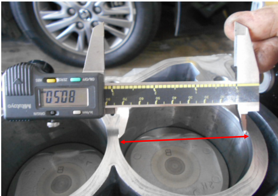
Photo 6 shows measurement being carried out to the bore (arrowed) of cylinder 1 of the Toyota engine. The bore measurement of cylinder 1 was recorded to be 80.50mm.
