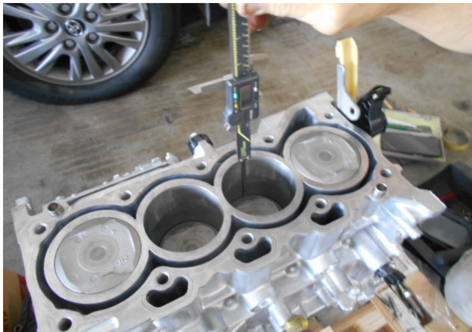
Photo 10 shows measurement of the stroke of cylinder 2 of the Toyota engine that I had inspected. The bore and stroke measurements of the Toyota engine were carried out using a digital Vernier Caliper, which was calibrated before the start of measurements.
