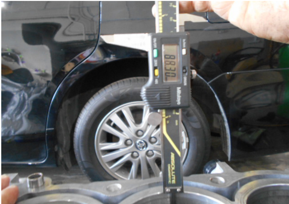
Photo 15 shows the stroke measurement of cylinder 3, which was recorded to be 88.30mm.
