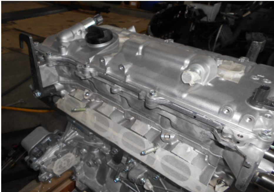
Photo 2 shows a general view of the Toyota engine that I had inspected. My visual examination of the engine housing revealed the housing to be of good condition. There was no crack and/or hole observed on the engine housing.
