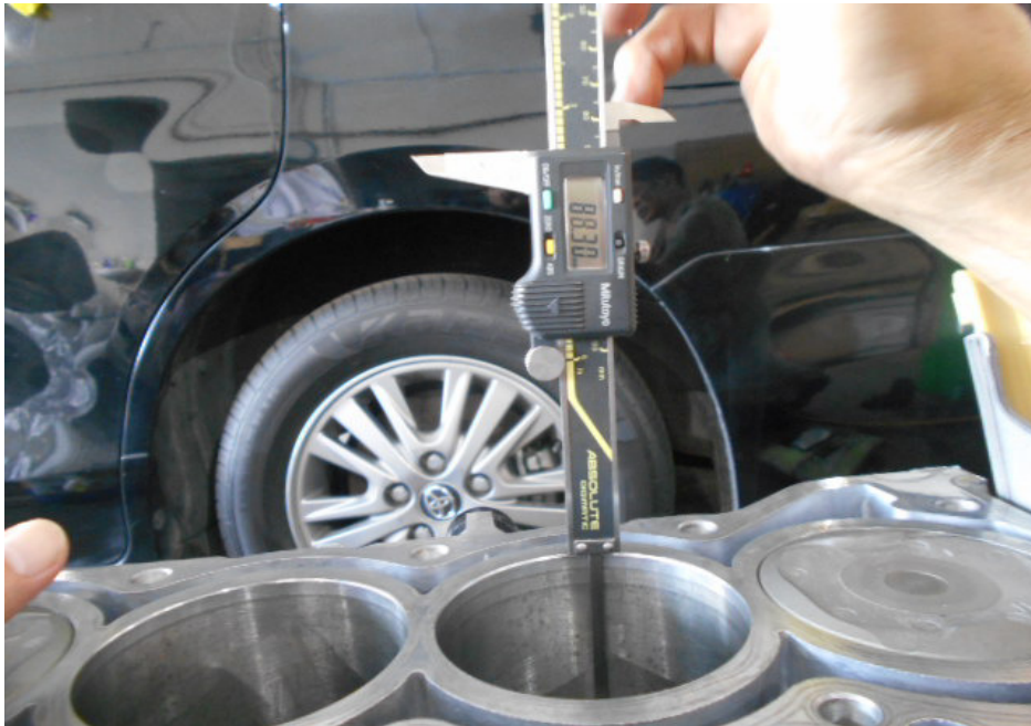
Photo 11 shows the stroke measurement of cylinder 2, which was recorded to be 88.30mm.
