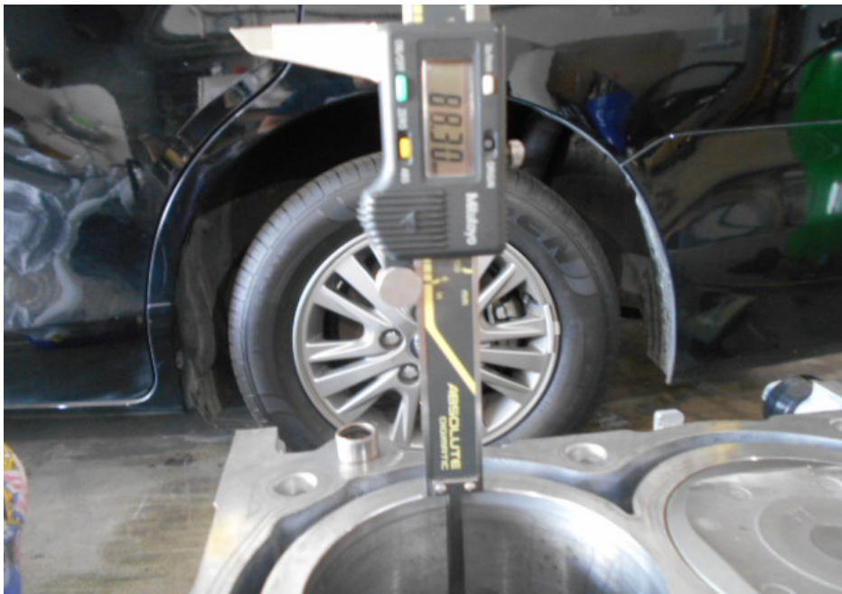
Photo 18 shows the stroke measurement of cylinder 4, which was recorded to be 88.30mm.
