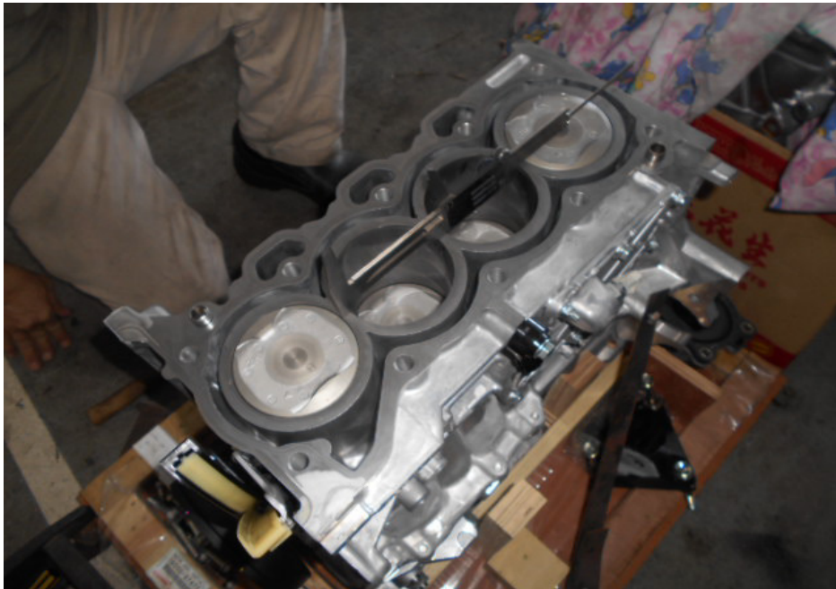
Photo 5 shows the bottom block of the Toyota engine. The top block was separated from the bottom block to facilitate my measurements of the bore and stroke of the Toyota engine. The measurements were carried out using a digital Vernier Caliper that was calibrated before the start of the measurements.
