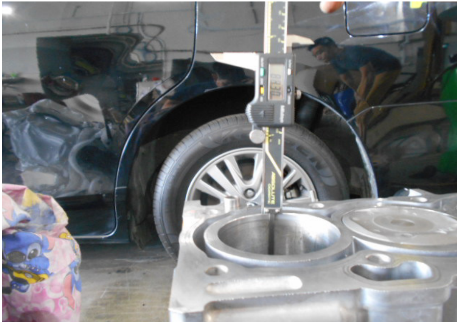
Photo 17 shows measurement being carried out to the stroke of cylinder 4 of the Toyota engine. The bore and stroke measurements of the Toyota engine were carried out using a digital Vernier Caliper that was calibrated before the start of measurements.
