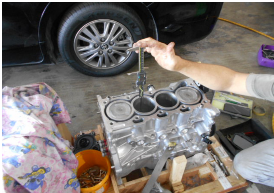
Photo 14 shows measurement of the stroke (arrowed) of cylinder 3 of the Toyota engine that I had inspected. The bore and stroke measurements of the Toyota engine were carried out using a digital Vernier Caliper that was calibrated before the start of measurements.
