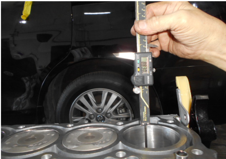
Photo 8 shows the stroke measurement of cylinder 1, which was recorded to be 88.30mm.
