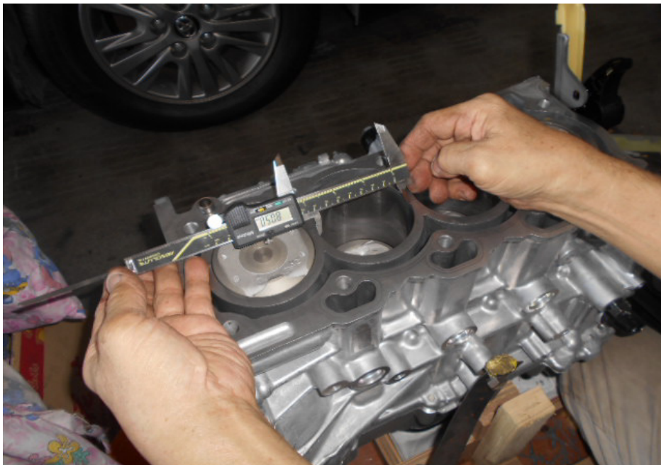
Photo 12 shows measurement being carried out to the bore of cylinder 3 of the Toyota engine. The bore and stroke measurements of the Toyota engine were carried out using a digital Vernier Caliper. The bore measurement of cylinder 3 was recorded to be 80.50mm.
