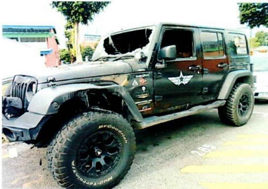
Photo 2 shows a general view of the fire damage at the front left body of the Insured Vehicle. The body panels that were found to have been burnt, include the front left fender and front left wheel arc. The front left door window and front windscreen were also observed to have been broken.
