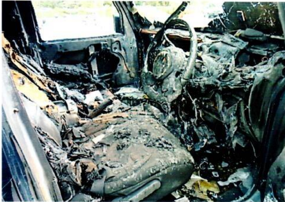
Photo 3 shows the interior compartment of the Insured Vehicle. The seats, roof upholstery, carpet, dashboard and various plastic trims were all burnt and/or melted as a result of the fire.
