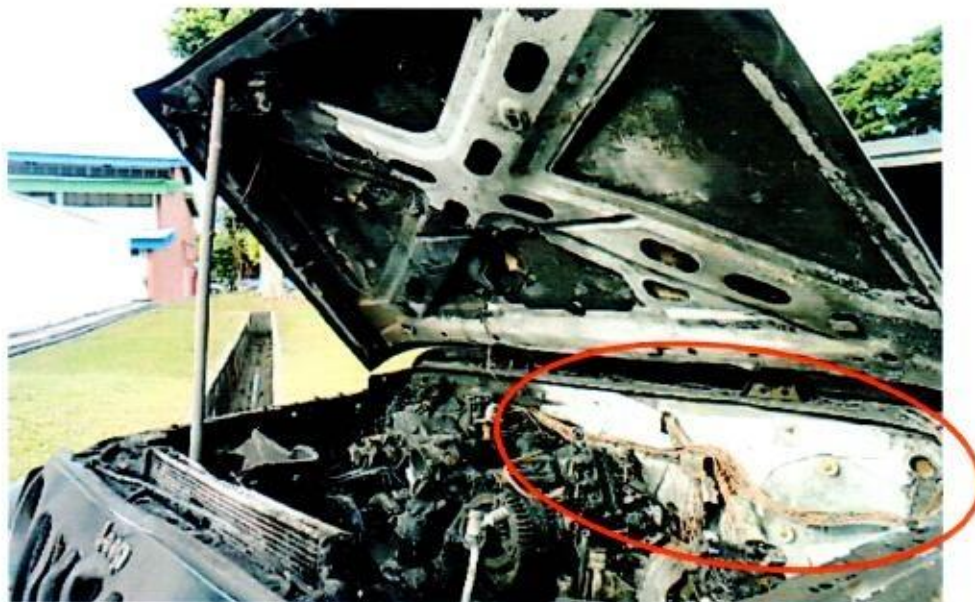
Photo 12 shows the intense burn marks (circled) observed on the firewall panel, at the left rear area of the Insured Vehicle's engine compartment.
