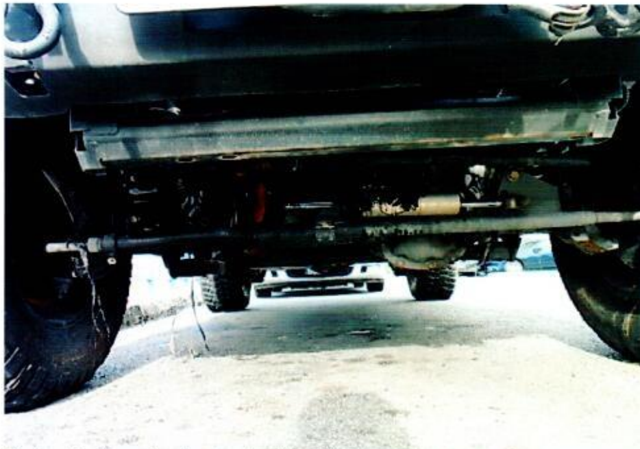
Photo 11 shows the front underside of the Insured Vehicle. Unlike in a normal saloon motor car, the engine area of the Insured Vehicle was not located within an enclosed/covered area. The engine area was relatively "open" from the underside of the Insured Vehicle, with no engine undercover covering the engine area. Heat generated from engine operation would have been easily dissipated out whilst the Insured Vehicle was moving.
