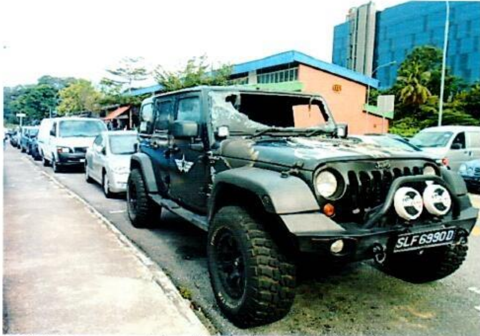
Photo 1 shows a general view of the front right body of the Insured Vehicle at the time of inspection. The Insured Vehicle was observed to have sustained relatively extensive fire damage at its frontal portion. The body panels at the frontal portion like the front right fender, front right wheel arc and front windscreen were found to have been burnt.
