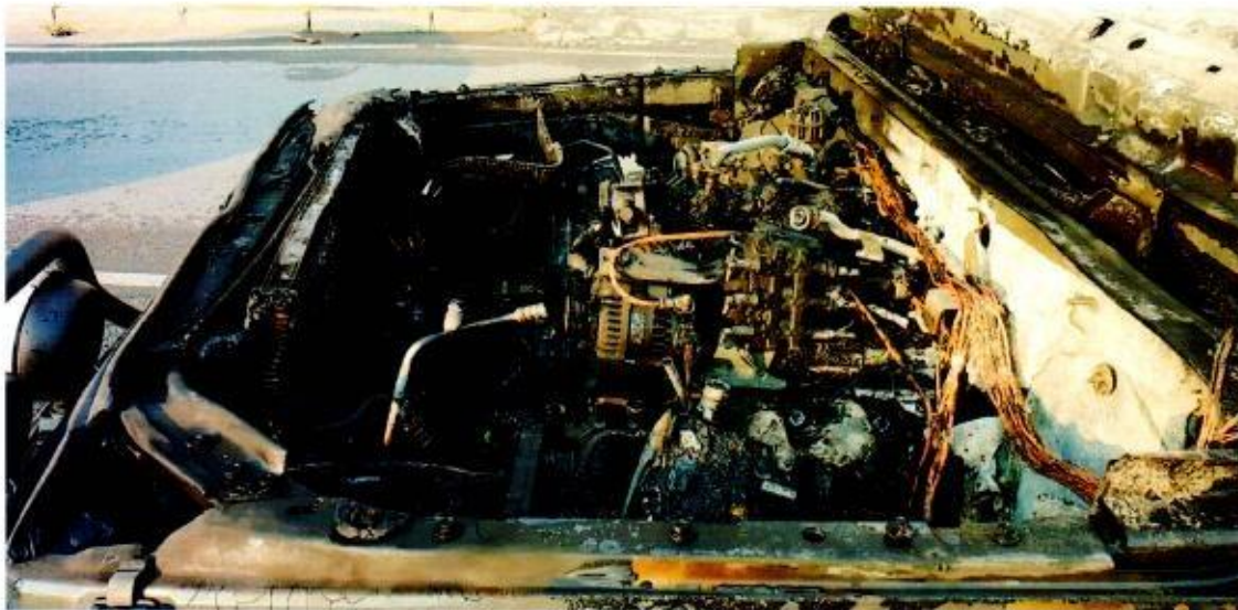
Photo 8 shows a general view of the engine compartment of the Insured Vehicle after the fire was extinguished. The damage of fire nature to the engine compartment, as seen from the photograph provided, was observed to be similar to what I had observed during my inspection of the Insured Vehicle.
