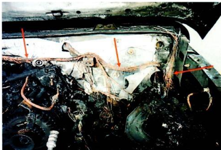
Photo 14 shows the stretch of wirings (arrowed) that were completely burned to its bare copper state. Such condition normally indicates internal heating of copper wires, which is a sign of an electrical short circuit occurring. This then indicates that the cause of fire to the Insured Vehicle was of electrical nature.
