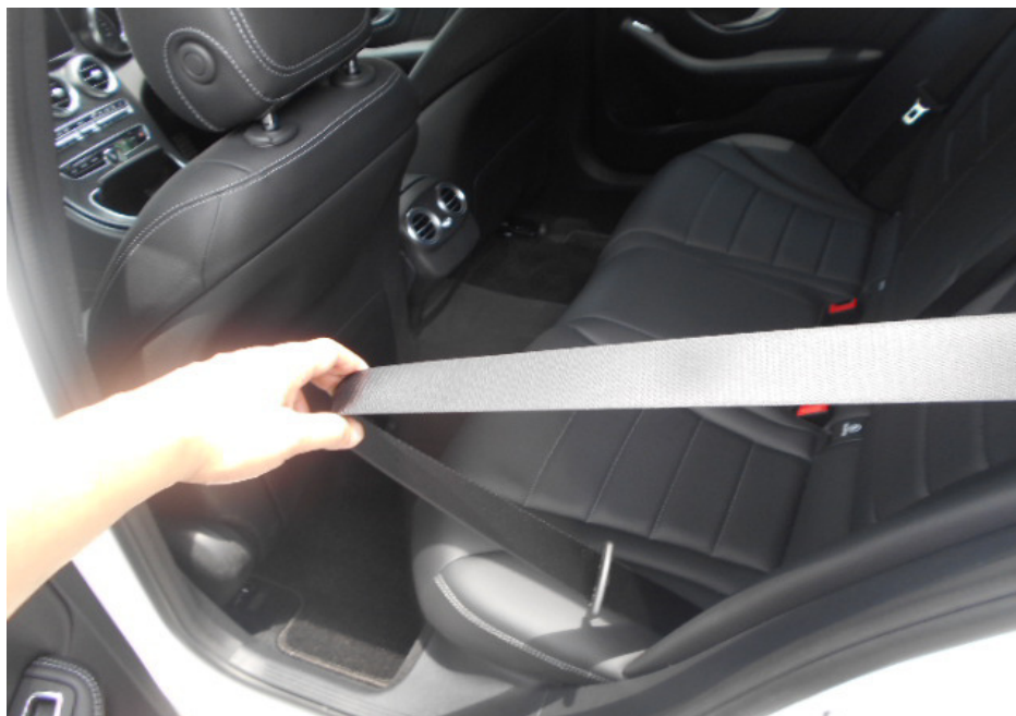
Photo 5 shows the rear seats of the Motor Car. All the seats were secured via seat rails to the floor board. The seats were also fitted with a retractable seat belt reel and pre-tensioner. The seat belts were tested and able to be fastened to the pretensioners that were fitted on the side of each individual seat.
