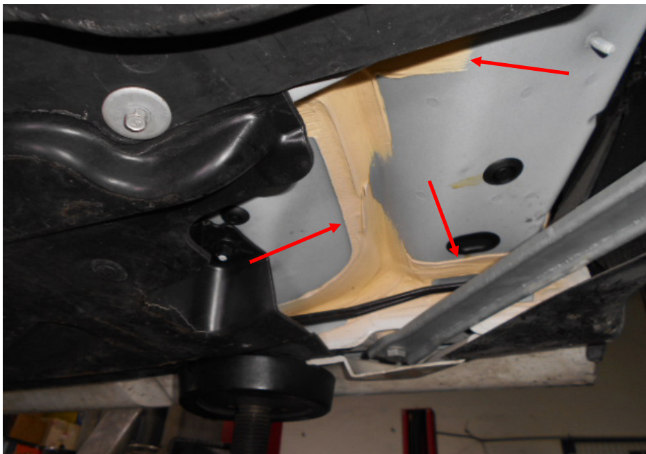
Photo 14 shows the structural body at the centre left of the Motor Car. Visually, I did not find any weld marks other than original spot weld marks on the chassis of the Motor Car. The joints (arrowed) along the chassis body was also untouched, indicating no work was done on the chassis body of the Motor Car and that the chassis body was originally fitted.
