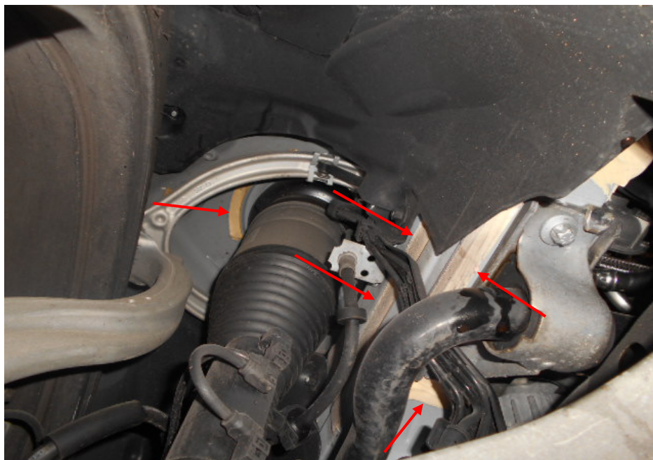
Photo 15 shows the structural body and wheel house panel at the front right of the Motor Car. The joints (arrowed) along the chassis body was untouched, indicating no work was done on the chassis body of the Motor Car and that the chassis body was originally fitted.
