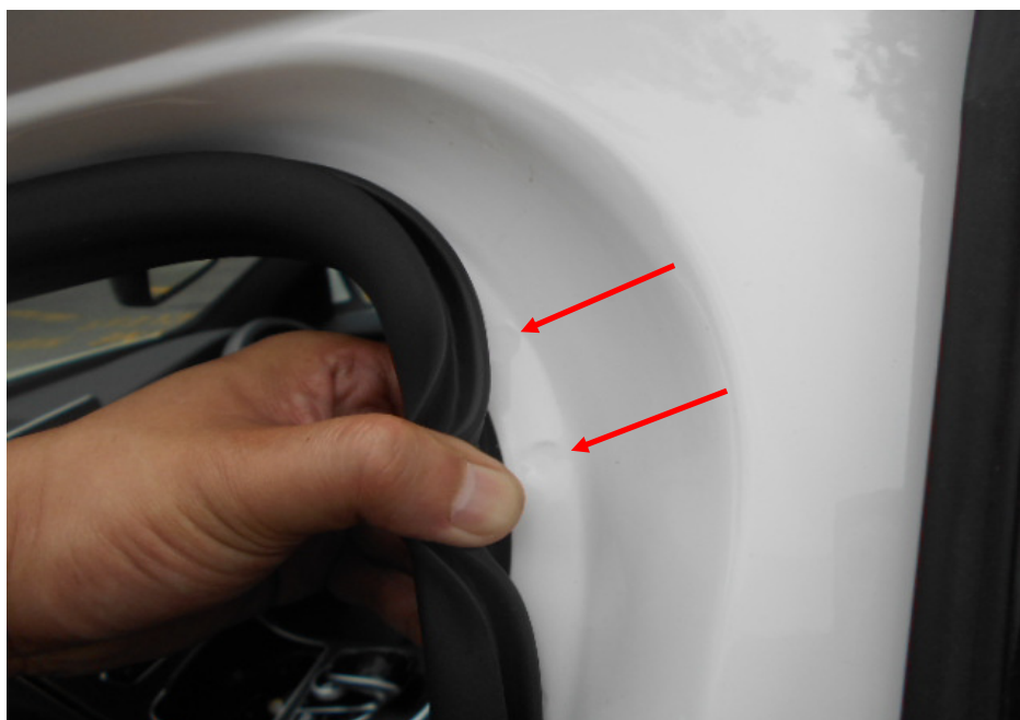
Photo 16 shows the left "B" pillar of the Motor Car. I did not find any weld marks other than original spot weld marks (arrowed) on the body panels of the Motor Car, indicating that there was no re-welding works carried out; and that the body panels of the Motor Car were originally fitted.
