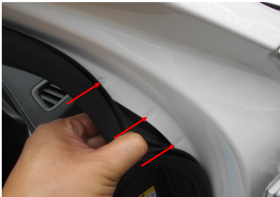
Photo 17 shows the front right “A” pillar of the Motor Car. I did not find any weld marks other than original spot weld marks (arrowed) on the body panels of the Motor Car, indicating that there was no re-welding works carried out; and that the body panels of the Motor Car were originally fitted.
