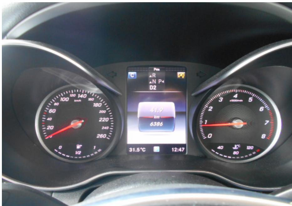
Photo 7 shows the respective warning lights no longer illuminated, indicating that there is no fault detected to the ABS, SRS, PSA and TCS systems of the Motor Car during the self-test. These electronic systems were hence in working condition at the time of my inspection.
