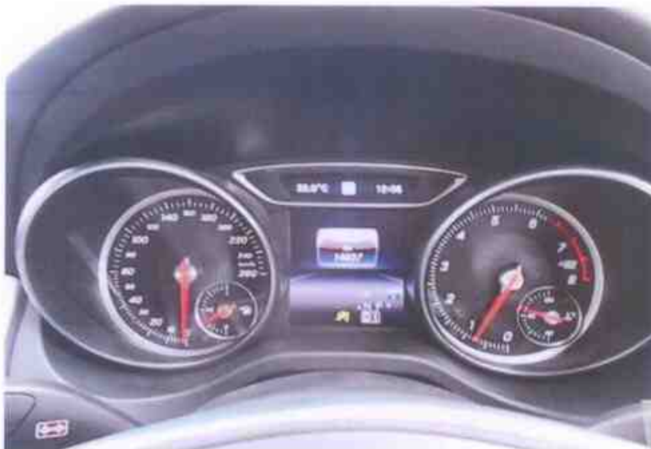
Photo 7 shows the respective warning lights no longer illuminated, indicating that there is no fault detected to the ABS, SRS and TC systems of the Motor Car during the self-test. These electronic systems were hence in working condition at the time of my inspection.
