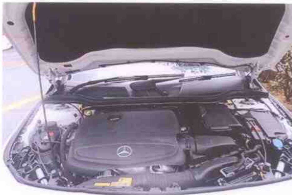
Photo 4 shows a general view of the engine compartment of the Motor Car at the time of my inspection. The various parts and components inside the engine compartment were all observed to be intact and properly fitted. There was also no sign(s) or indication(s) of fluid leak and/or fluid stain found inside the engine compartment. The engine oil, brake fluid and engine coolant were all found to be of sufficient level for operating purposes. Visually, there was also no contamination found to these fluids.
