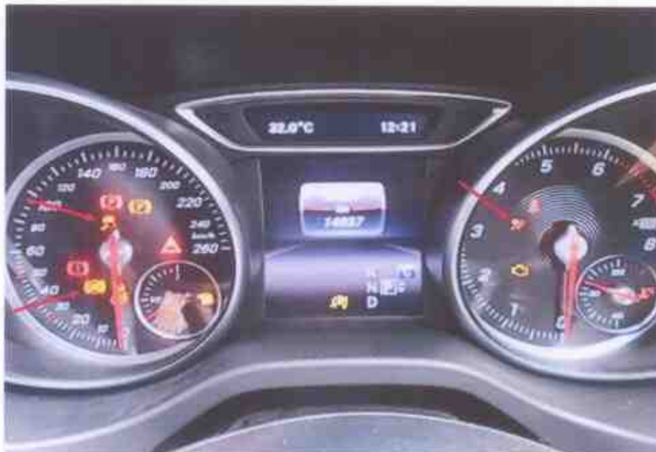
Photo 6 shows the warning lights for the various electronic safety features appearing on the instrument panel of the Motor Car during its self-test when the engine is cranked, in particular the ABS, SRS and TC lights (arrowed).
