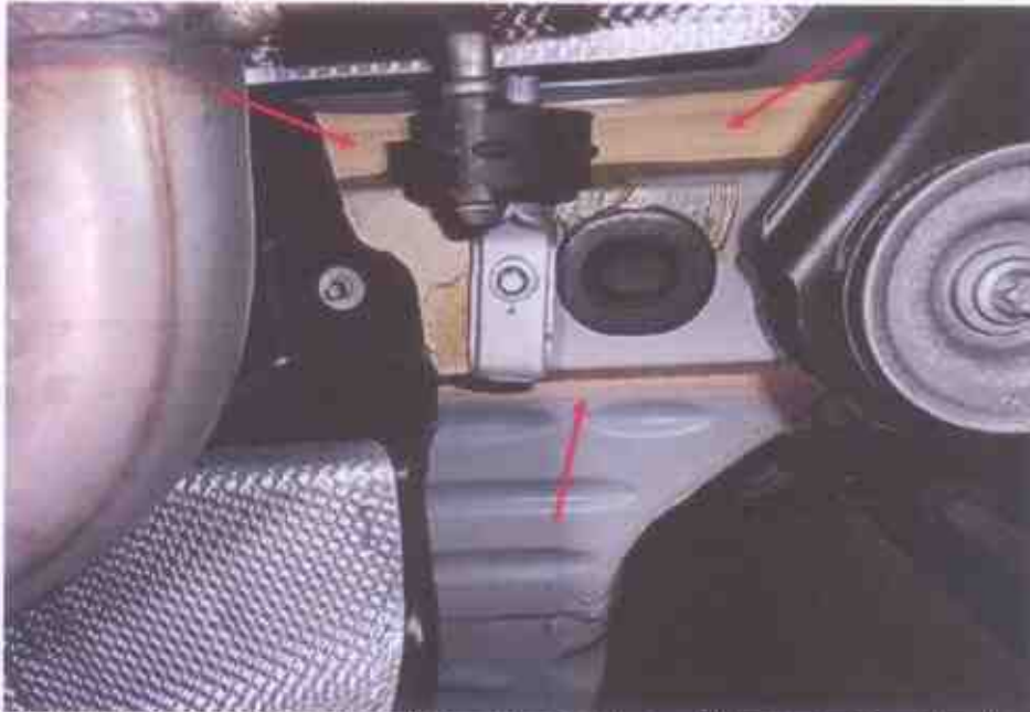
Photo 13 shows the structural body at the right rear of the Motor Car. Visually, I did not find any weld marks other than original spot weld marks on the chassis body of the Motor Car. The joints (arrowed) along the chassis body was also untouched, indicating no work was done on the chassis body of the Motor Car and that the chassis body was originally fitted.
