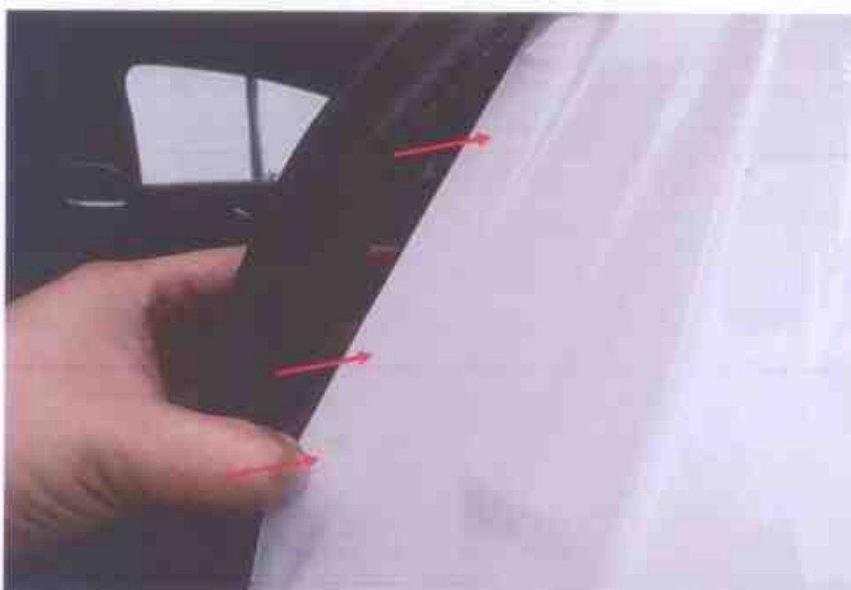
Photo 16 shows the rear left body panel of the Motor Car. I did not find any weld marks other than original spot weld marks (arrowed) on the body panels of the Motor Car, indicating that there was no re-welding works carried out; and that the body panels of the Motor Car were originally fitted.
