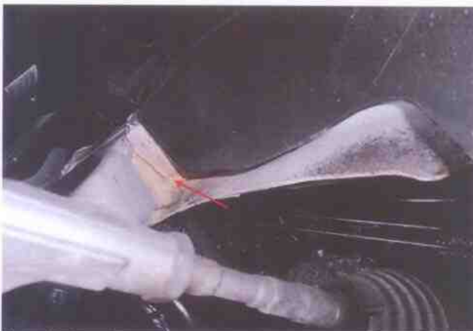
Photo 15 shows the structural body at the front left of the Motor Car. The joints (arrowed) along the chassis body was untouched, indicating no work was done on the chassis body of the Motor Car and that the chassis body was originally fitted.
