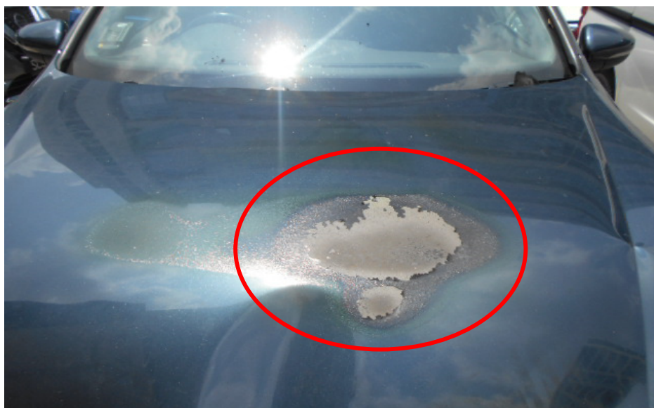
Photo 7 shows the intense burn marks (circled) that were found on the centre of the Insured Vehicle's front bonnet. Such marks are normally formed on steel/metal material body parts that had been exposed to prolong high heat intensity and can usually determine the origin of the fire.
