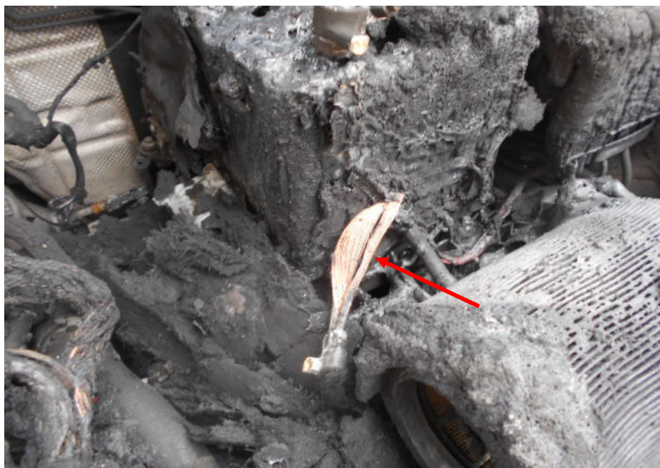
Photo 9 shows the completely burned to copper wire cable (arrowed) for the battery of the Insured Vehicle. This wire cable is an original factory fitted wire cable and is located at the centre area of the engine compartment, which was where the fire had originated. The bright reddish colour of the copper wires suggest that the wirings were exposed to high heat. Such condition normally indicates internal heating of copper wires, which is a sign of an electrical short circuit occurring.
