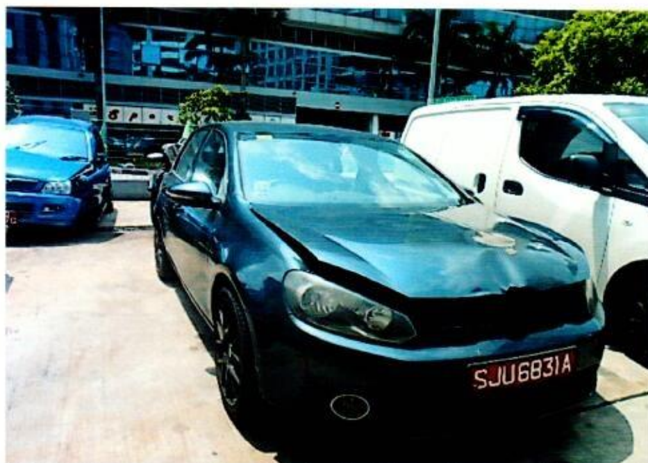
Photo 1 shows a general view of the front right body of the Insured Vehicle at the time of inspection. The Insured Vehicle was observed to have sustained fire damage that was confined to its frontal body. Its front bonnet, front radiator grille, front right headlamp and front right fender were amongst the body parts that were found to have been burnt as a result of the fire.
