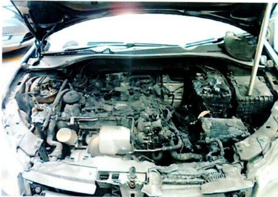
Photo 3 shows the engine compartment of the Insured Vehicle at the time of inspection. Almost all the parts inside the engine compartment were observed to have been burnt and/or melted as a result of the fire. These parts had included its radiator, air condenser, cooling fan, intake manifold, fuse box, battery, air duct, rubber hoses and pipes amongst others.
