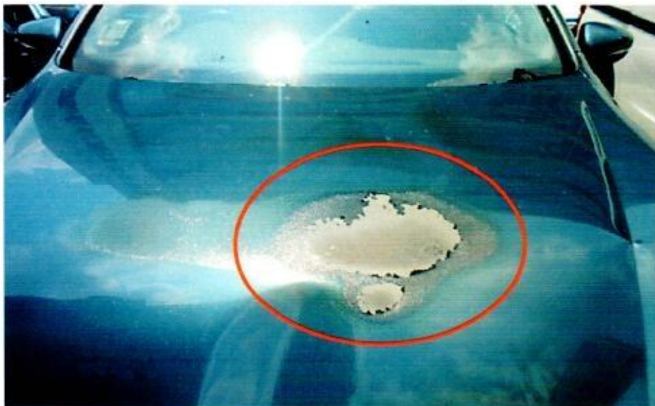
Photo 7 shows the intense burn marks (circled) that were found on the centre of the Insured Vehicle's front bonnet. Such marks are normally formed on steel/metal material body parts that had been exposed to prolong high heat intensity and can usually determine the origin of the fire.
