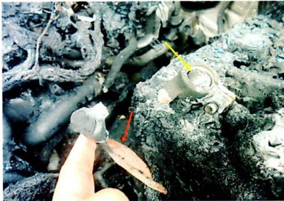
Photo 10 shows a closer view of the burned to copper wire cable (red arrow). The wire cable connects to the battery terminal (yellow arrow) of the Insured Vehicle.
