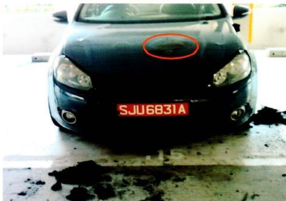
Photo 5 shows the Insured Vehicle at the incident location. The same intense burn mark (circled), that I had observed during my inspection of the Insured Vehicle, can be seen similarly formed on the centre of the front bonnet. My close examination of the photographs provided had also showed no unusual foreign material(s), object(s) and/or fluid accumulation on the ground where the Insured Vehicle was parked.
