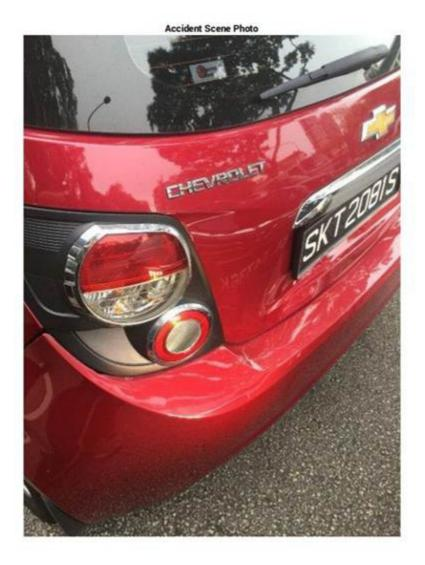
The above photo was taken by Insured at the time of accident (see OI GIA Report). It shows that the deformed rear number plate of TP vehicle.
