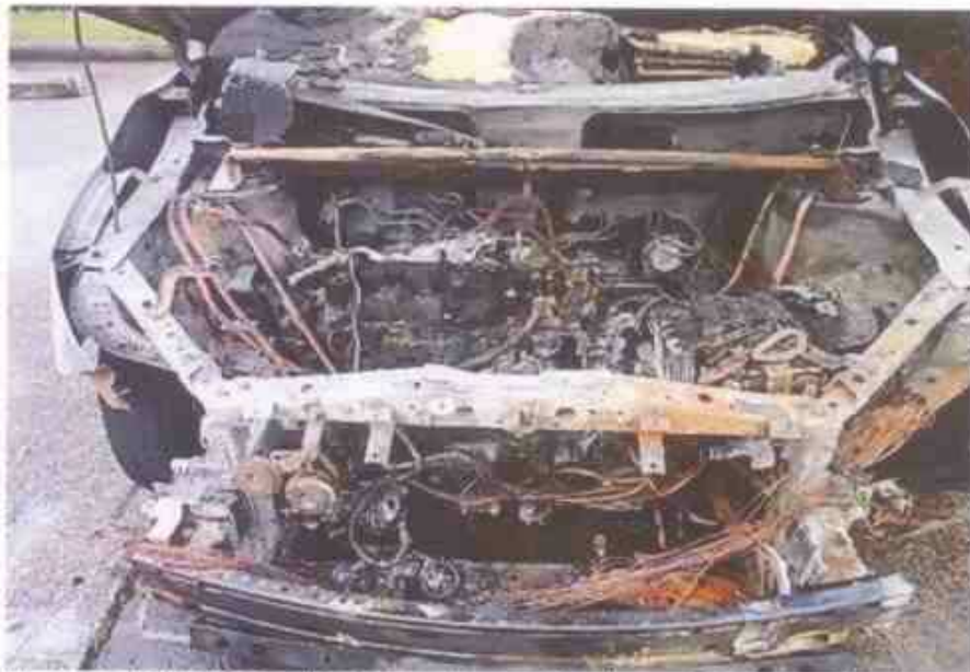
Photo 3 shows the engine compartment of the Insured Vehicle at the time of inspection. All the parts inside the engine compartment were observed to be burnt and/or melted as a result of the fire. These parts had included the radiator, air condenser, cooling fan, intake manifold, fuse box, battery, air duct, hoses and pipes amongst others.
