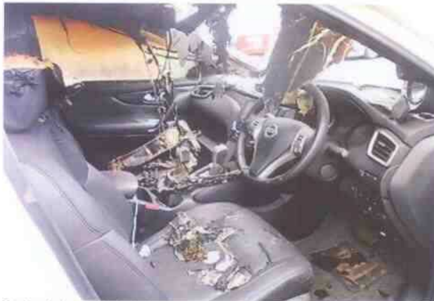
Photo 4 shows the interior compartment of the Insured Vehicle, which was affected at the front area. The front seats, upholstery, carpet and various plastic trims were partially burnt and/or melted by the incident.
