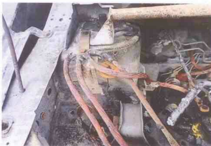
Photo 13 shows a closer view of the wirings at the right rear area of the Insured Vehicle's engine compartment. The wirings were found to be completely burned to its bare copper state. The bright reddish colour of the copper wires suggest that the wirings were exposed to high heat, which is a sign of an electrical short circuit occurring. These wirings were wire cables (grounding cables) that were additionally fitted for the enhanced audio system that was fitted on the Insured Vehicle.
