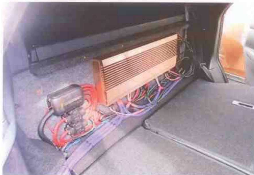
Photo 5 shows the audio amplifier, wire cables and fuses that were found to have been additionally fitted on the Insured Vehicle at the time of my inspection. These were fixed behind the rear seats of the Insured Vehicle, as part of the enhanced car audio system.
