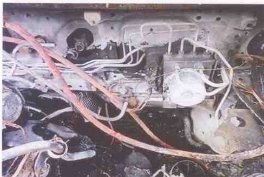
Photo 14 shows another stretch of wirings at the rear centre area of the Insured Vehicle's engine compartment that were bright reddish colour and completely burned to its bare copper state. These wirings were wire cables (grounding cables) that were additionally fitted for the enhanced audio system that was fitted on the Insured Vehicle.
