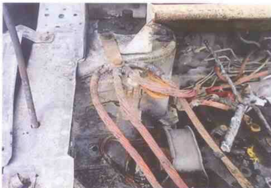
Photo 8 shows the wire cables that were additionally fitted in the engine compartment of the Insured Vehicle. These wire cables appear to be grounding cables for the enhanced audio system that was fitted on the Insured Vehicle.
