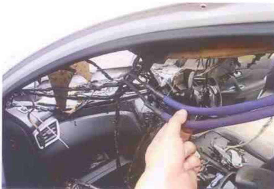
Photo 7 shows the wire cables that were additionally fitted from the rear to the front of the Insured Vehicle, as part of the enhanced car audio system.
