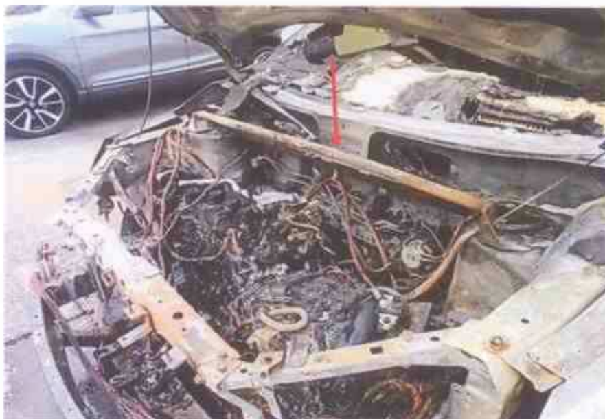
Photo 9 shows the front strut bar (arrowed) that was additionally fitted in the engine compartment of the Insured Vehicle. This strut bar is not a standard item for the Insured Vehicle. The fitting of this strut bar enhances the road stability and handling of the Insured Vehicle.
