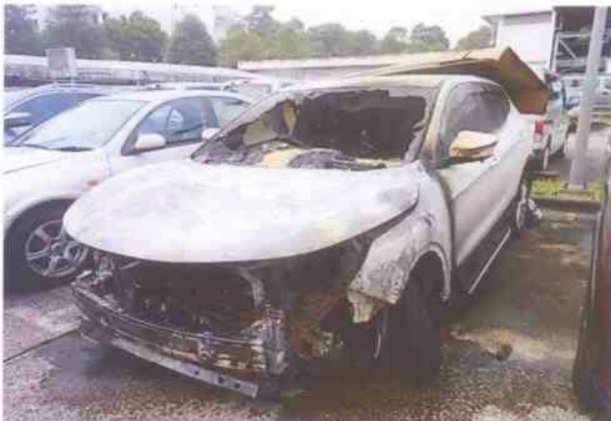
Photo 2 shows a general view of the front left body of the Insured Vehicle at the time of inspection. The Insured Vehicle was observed to have sustained severe fire damage at its frontal body. Its front bumper, front left fender, front left headlamp, front bonnet, front left tyre and front windscreen were amongst the body parts that were found to have been burnt as a result of the fire.
