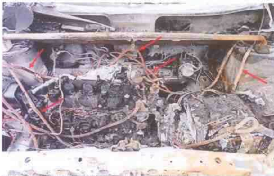
Photo 12 shows the wirings at the Insured Vehicle's engine compartment. Several stretches of wirings (arrowed) were found to be completely burned to its bare copper state. The bright reddish colour of the copper wires suggest that the wirings were exposed to high heat, which is a sign of an electrical short circuit.
