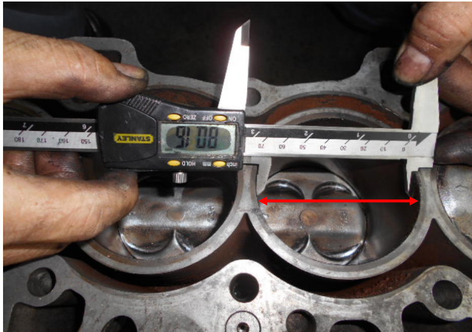
Photo 13 shows measurement being carried out to the bore (arrowed) of cylinder 3 of the Honda engine. The bore and stroke measurements of the Honda engine were carried out using a digital Vernier Caliper. The bore measurement of cylinder 3 was recorded to be 80.16mm.
