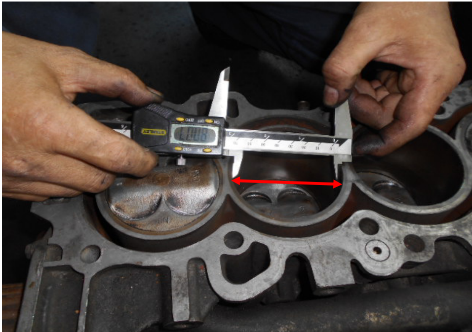
Photo 9 shows measurement being carried out to the bore (arrowed) of cylinder 2 of the Honda engine. The bore measurement of cylinder 2 was recorded to be 80.07mm.
