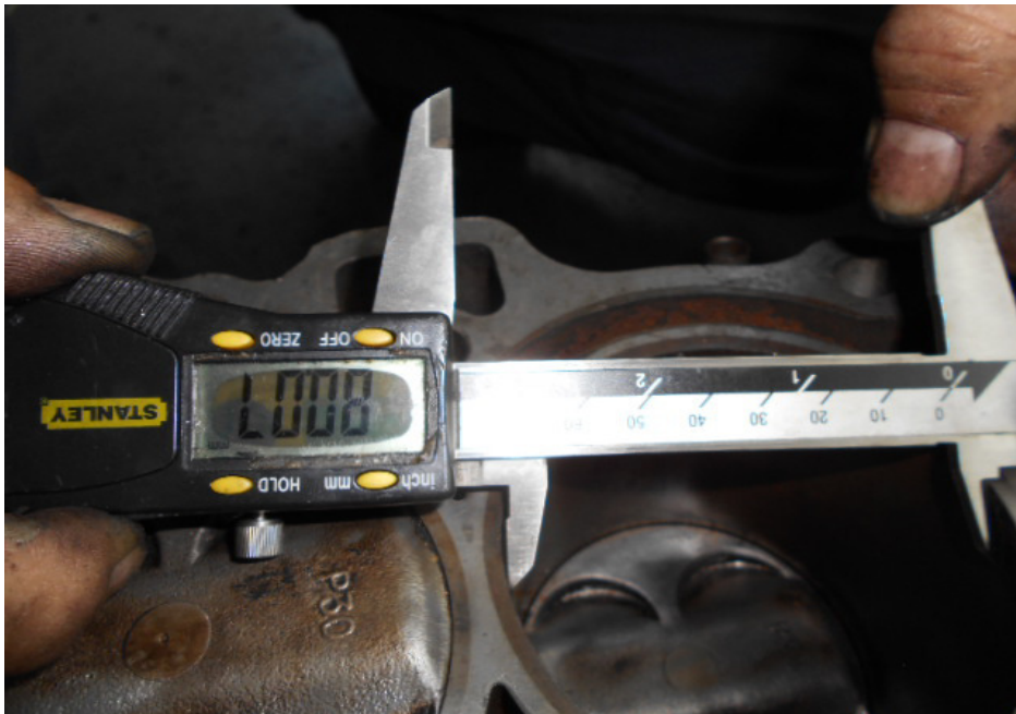
Photo 10 shows the bore measurement of cylinder 2, which was recorded to be 80.07mm.
