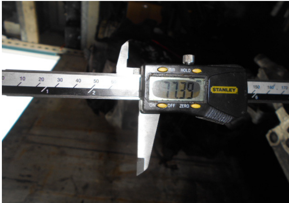
Photo 15 shows the stroke measurement of cylinder 3, which was recorded to be 77.39mm.
