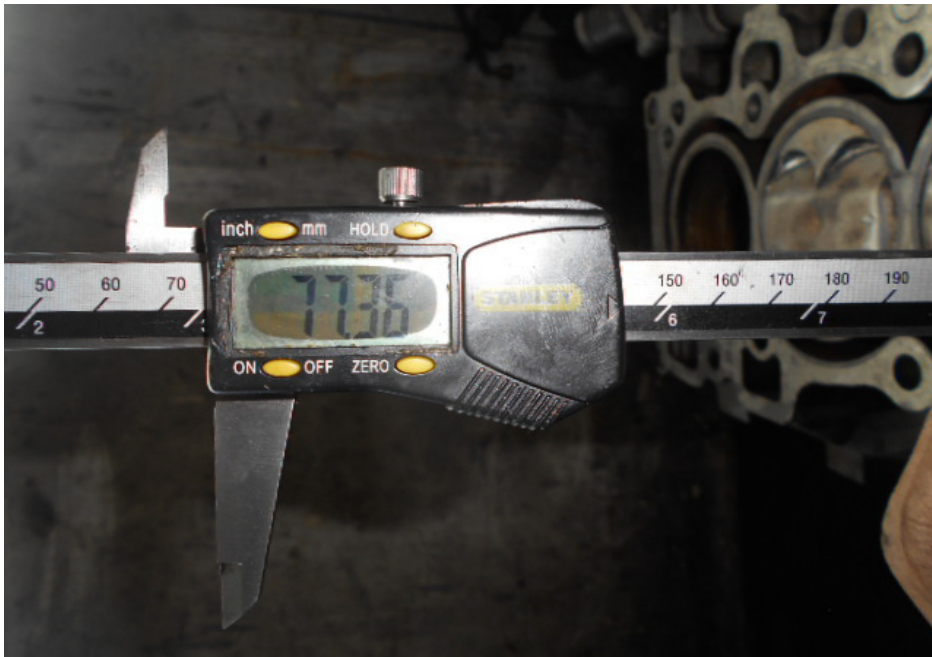
Photo 8 shows the stroke measurement of cylinder 1, which was recorded to be 77.36mm.
