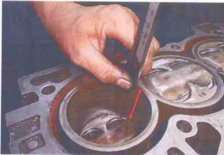
Photo 7 shows measurement being carried out to the stroke (arrowed) of cylinder 1 of the Honda engine. The bore and stroke measurements of the Honda engine were carried out using a digital Vernier Caliper.
