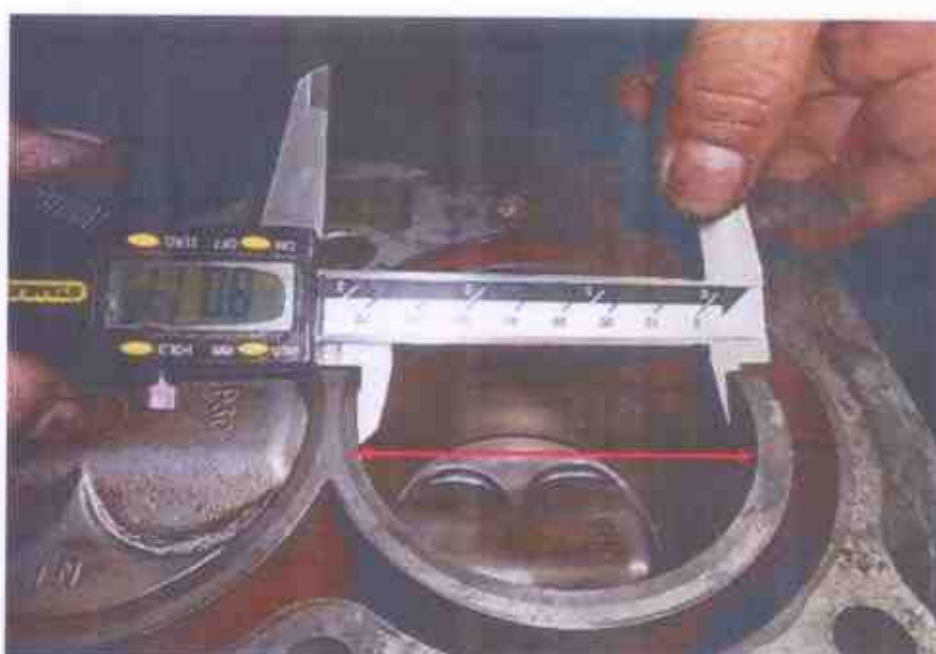
Photo 16 shows measurement being carried out to the bore (arrowed) of cylinder 4 of the Honda engine. The bore and stroke measurements of the Honda engine were carried out using a digital Vernier Caliper. The bore measurement of cylinder 4 was recorded to be 80.11mm.
