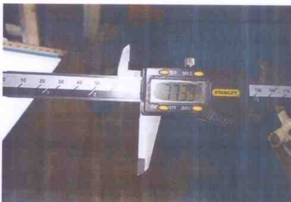
Photo 15 shows the stroke measurement of cylinder 3, which was recorded to be 77.38mm.
