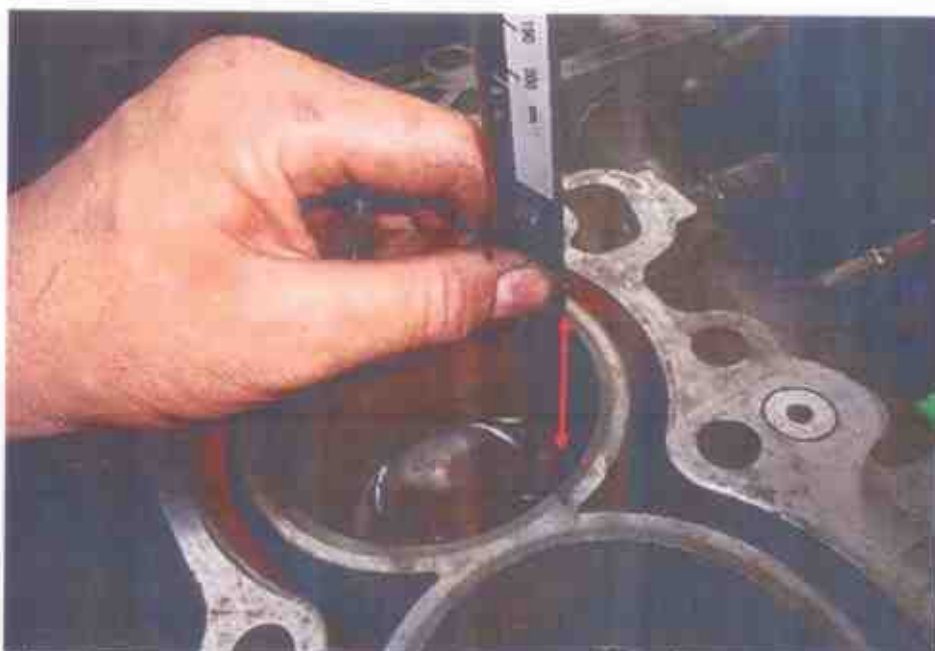
Photo 14 shows measurement of the stroke (arrowed) of cylinder 3 of the Honda engine that I had inspected. The bore and stroke measurements of the Honda engine were carried out using a digital Vernier Caliper that was calibrated before the start of measurements.
