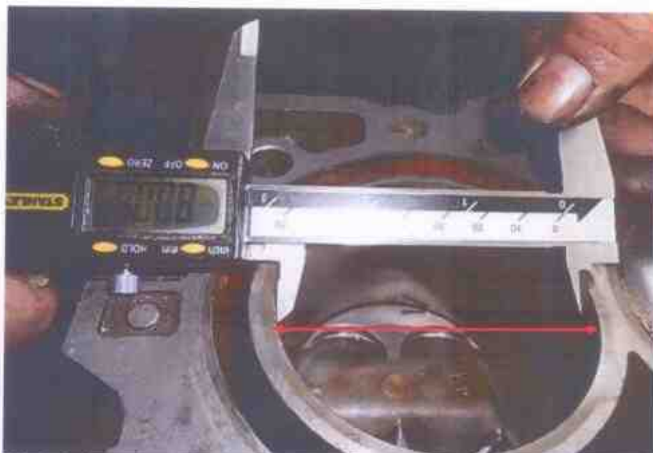
Photo 6 shows measurement being carried out to the bore (arrowed) of cylinder 1 of the Honda engine. The bore measurement of cylinder 1 was recorded to be 80.00mm.
