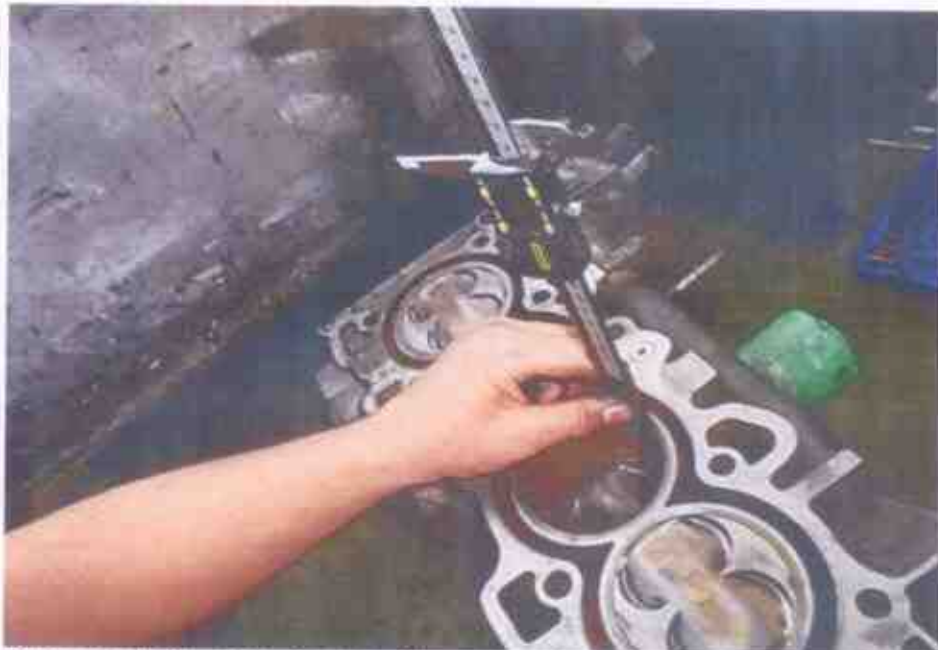
Photo 11 shows measurement of the stroke of cylinder 2 of the Honda engine that I had inspected. The bore and stroke measurements of the Honda engine were carried out using a digital Vernier Caliper, which was calibrated before the start of measurements.
