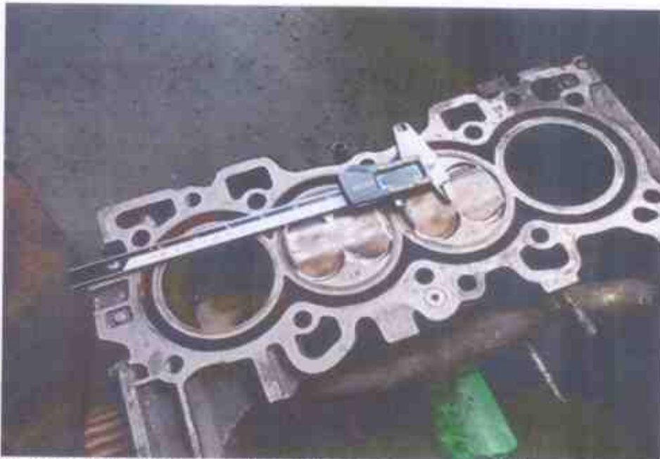
Photo 5 shows the bottom block of the Honda engine and the digital Vernier Caliper that was used to measure the bore and stroke of the Honda engine. The digital Vernier Caliper was calibrated before the start of the measurements.
