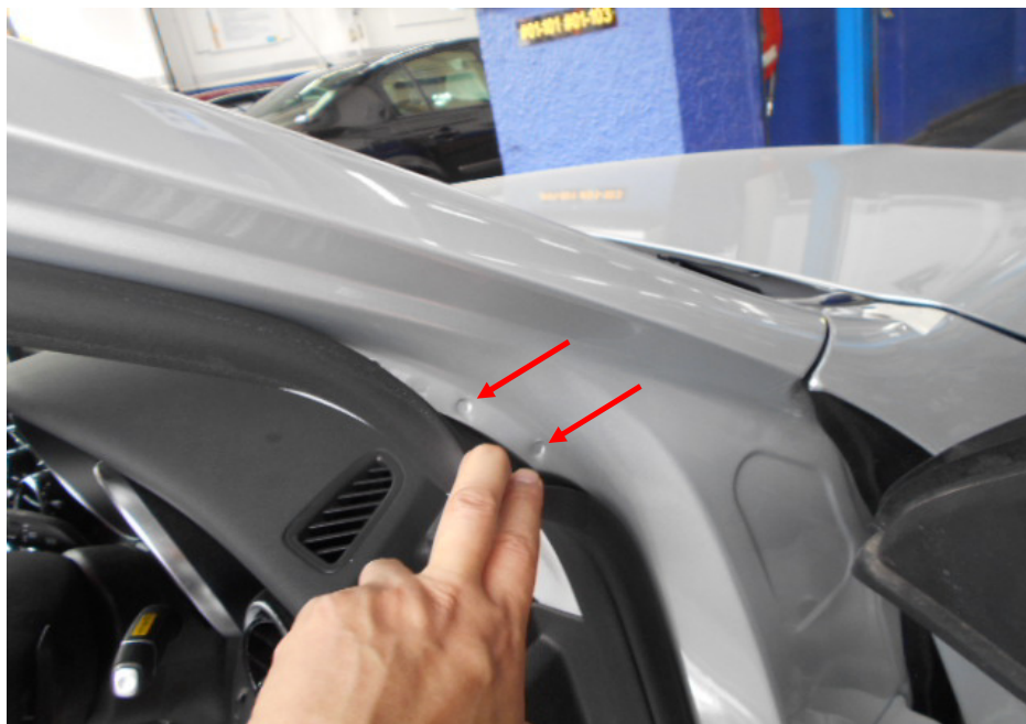
Photo 18 shows the front right “A” pillar of the Motor Car. I did not find any weld marks other than original spot weld marks (arrowed) on the non-detachable body panels of the Motor Car, indicating that there was no re-welding works carried out; and that the non-detachable body panels of the Motor Car were originally fitted.
