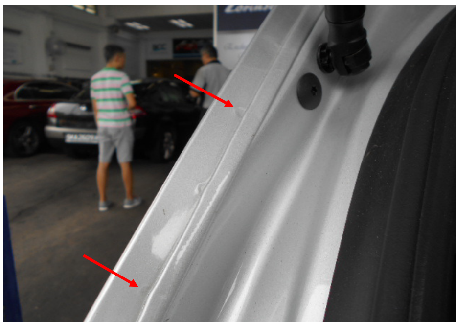
Photo 17 shows the rear left body panel of the Motor Car. I did not find any weld marks other than original spot weld marks (arrowed) on the non-detachable body panels of the Motor Car, indicating that there was no re-welding works carried out; and that the non-detachable body panels of the Motor Car were originally fitted.
