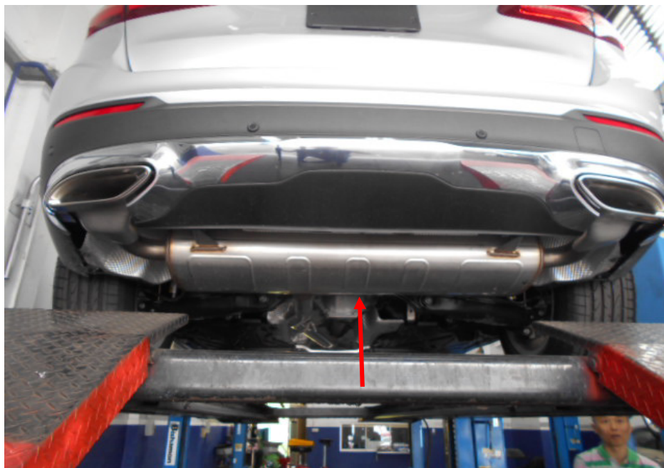
Photo 8 shows the Motor Car hoisted up for checks on its undercarriage. My examination of the Motor Car's exhaust system revealed no sign(s) or indication(s) of any cut or weld marks along its exhaust pipes and on its rear muffler (arrowed).
