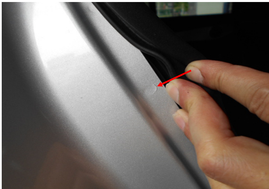
Photo 16 shows the rear right body panel of the Motor Car. I did not find any weld marks other than original spot weld marks (arrowed) on the non-detachable body panels of the Motor Car, indicating that there was no re-welding works carried out; and that the non-detachable body panels of the Motor Car were originally fitted.
