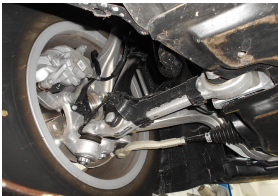
Photo 11 shows the various undercarriage components at the front left wheel of the Motor Car. The mechanical components, control arms and linkages were all found to be intact and secured in an appropriate manner. There was also no fluid leak and/or fluid stain observed on the underside of the Motor Car.
