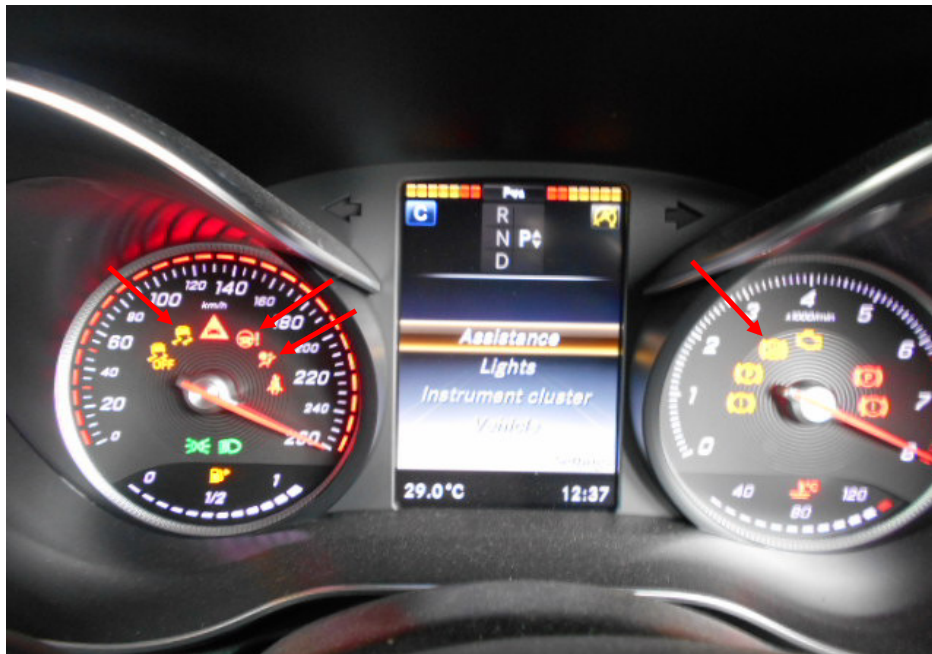
Photo 5 shows the warning lights for the various electronic safety features appearing on the instrument panel of the Motor Car during its self-test when the engine is cranked, in particular the Anti-Brake Lock System (ABS), Supplemental Restraint System (SRS), Power Steering Assist (PSA) and Electronic Stability Program (ESP) (arrowed).
