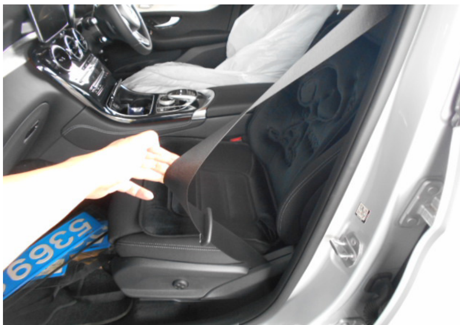
Photo 7 shows the interior compartment of the Motor Car. The seats of the Motor Car were found to be secured to the floor panel of the Motor Car via seat rails that were bolted onto the floor board. Retractable seat belt reels and pre-tensioners were fitted on all seats of the Motor Car. The seat belt reels were able to be fastened securely to the respective pre-tensioner that is fixed to the side of all the seats.
