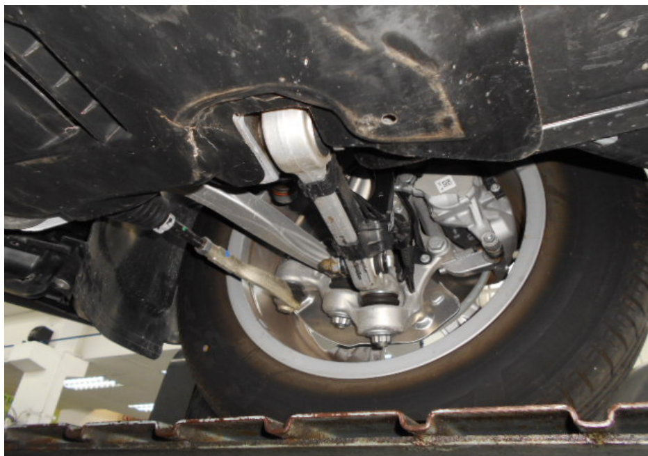
Photo 10 shows the various undercarriage components at the front right wheel of the Motor Car. The mechanical components, control arms and linkages were all found to be intact and secured in an appropriate manner. There was also no fluid leak and/or fluid stain observed on the underside of the Motor Car.
