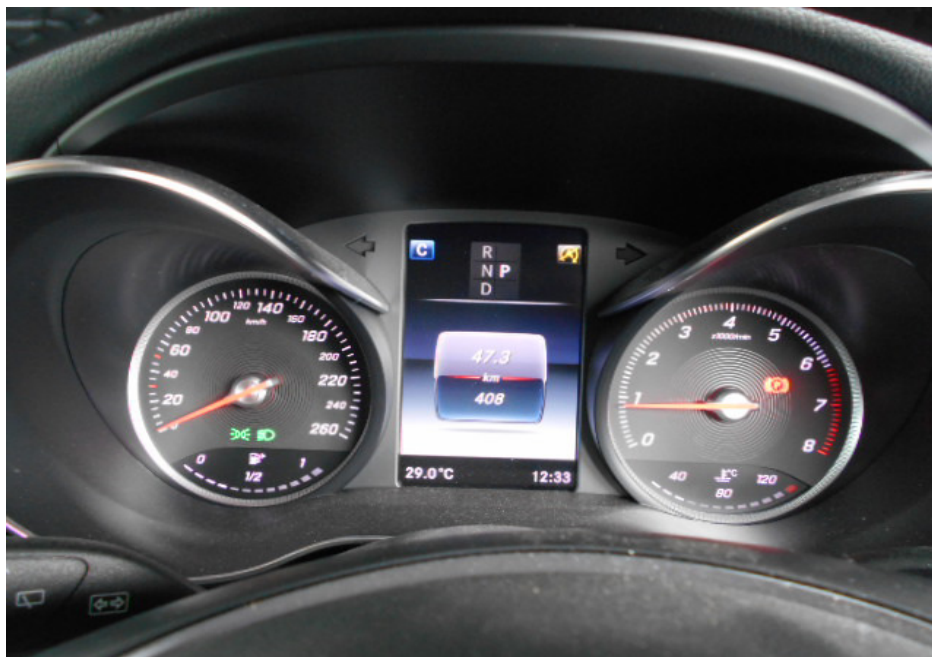
Photo 6 shows the respective warning lights no longer illuminated, indicating that there is no fault detected to the ABS, SRS, PSA and ESP systems of the Motor Car during the self-test. These electronic safety features were hence in working condition at the time of my inspection.
