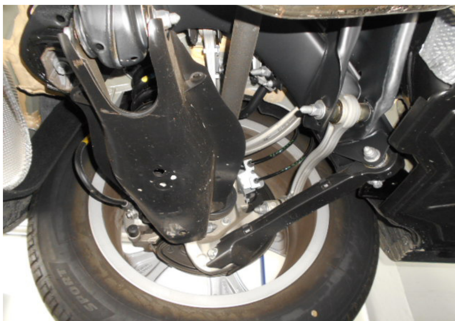
Photo 9 shows the various undercarriage components at the rear left wheel of the Motor Car. The mechanical components, control arms and linkages were all found to be intact and secured in an appropriate manner. There was also no sign(s) or indication(s) of fluid leakage and/or fluid stain(s).
