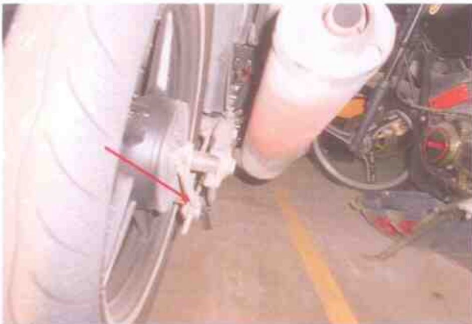
Photo 15 shows our checks on the rear brake mechanical components. It was observed to be unaffected by the accident's impact.
