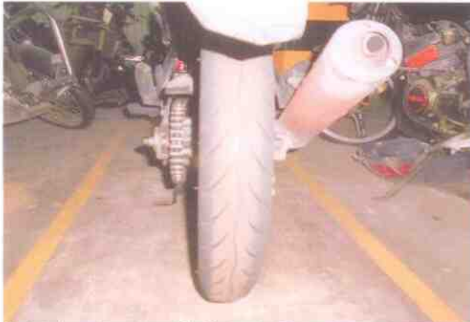
Photo 8 shows the rear tyre of the Motorcycle. The rear tyre was observed to be in serviceable condition with remaining tread depth of approximately 3mm. The tyre was also observed to be sufficiently inflated for vehicular operation.
