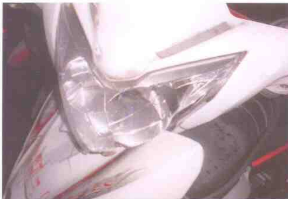
Photo 7 shows a closer view of the front headlamp of the Motorcycle at the time of our inspection. It was observed to have sustained with relatively minor damages due to the accident collision.
