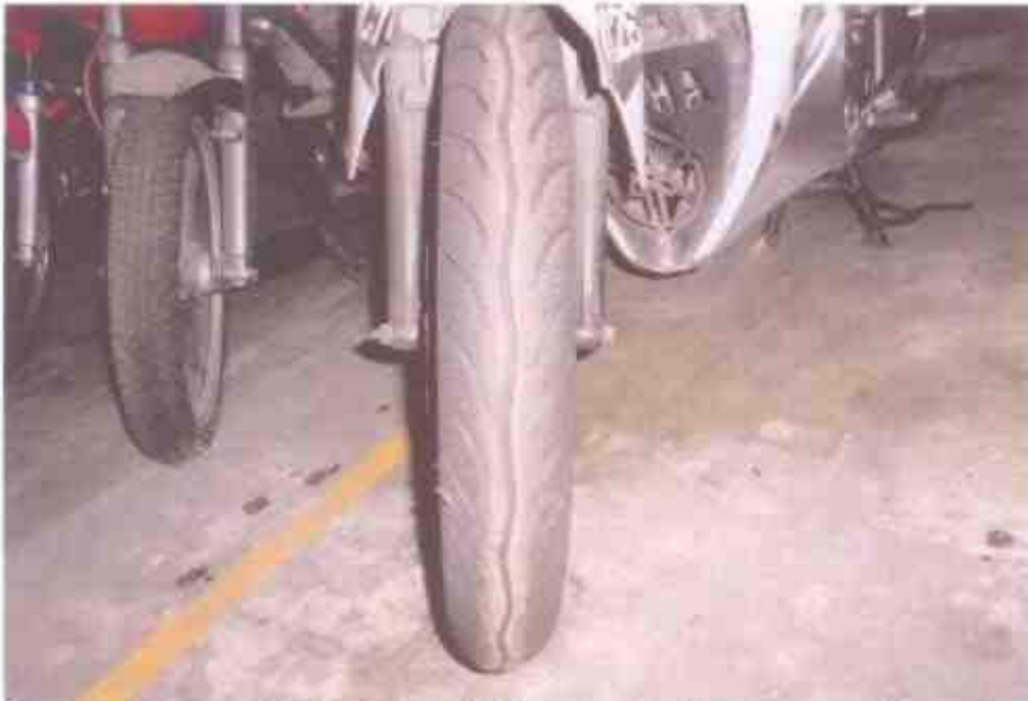
Photo 9 shows the front tyre of the Motorcycle. The front tyre was observed to be in serviceable condition with remaining tread depth of approximately 4mm. The tyre was also observed to be sufficiently inflated for vehicular operation.
