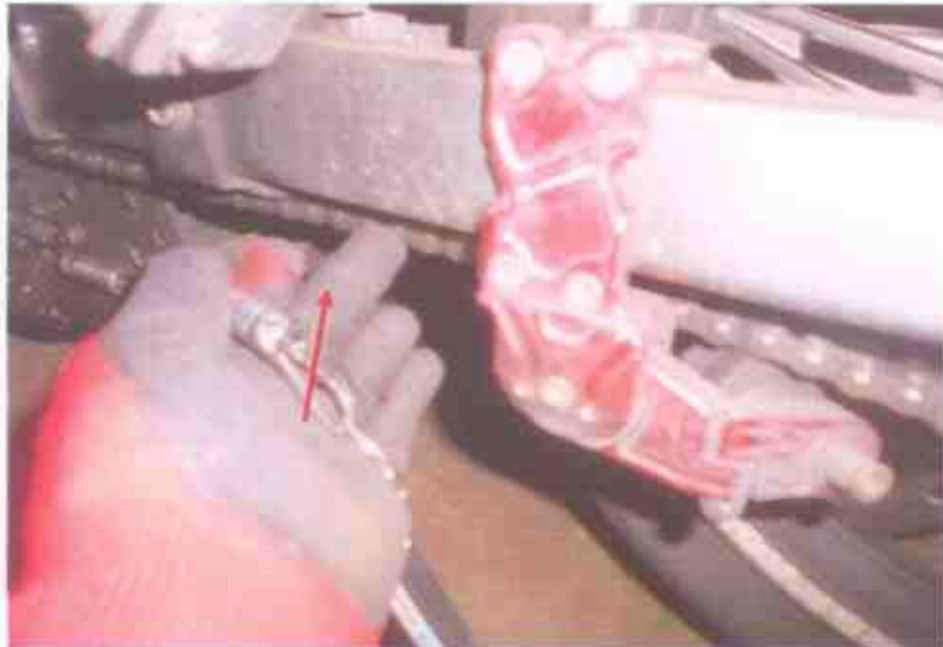
Photo 13 shows the general view of the gear train (arrowed) of the Motorcycle, which was observed to be intact with no misalignment. It was also adequately lubricated for operating purposes. Free play tension was also observed & found adequately acceptable.
