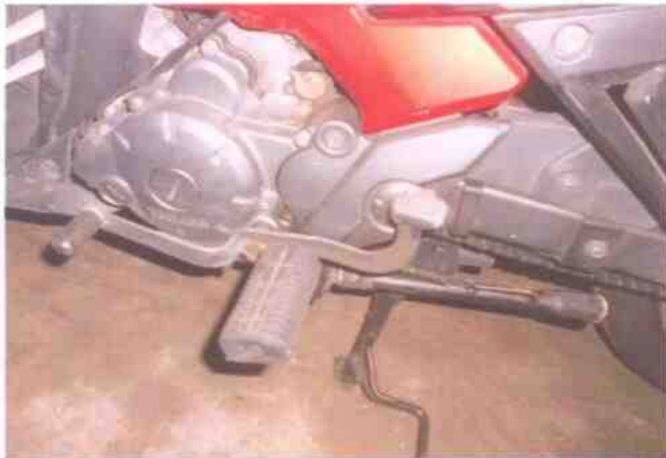
Photo 11 shows no sign(s) or indication(s) of fluid leakage stain observed around the engine area of the Motorcycle.
