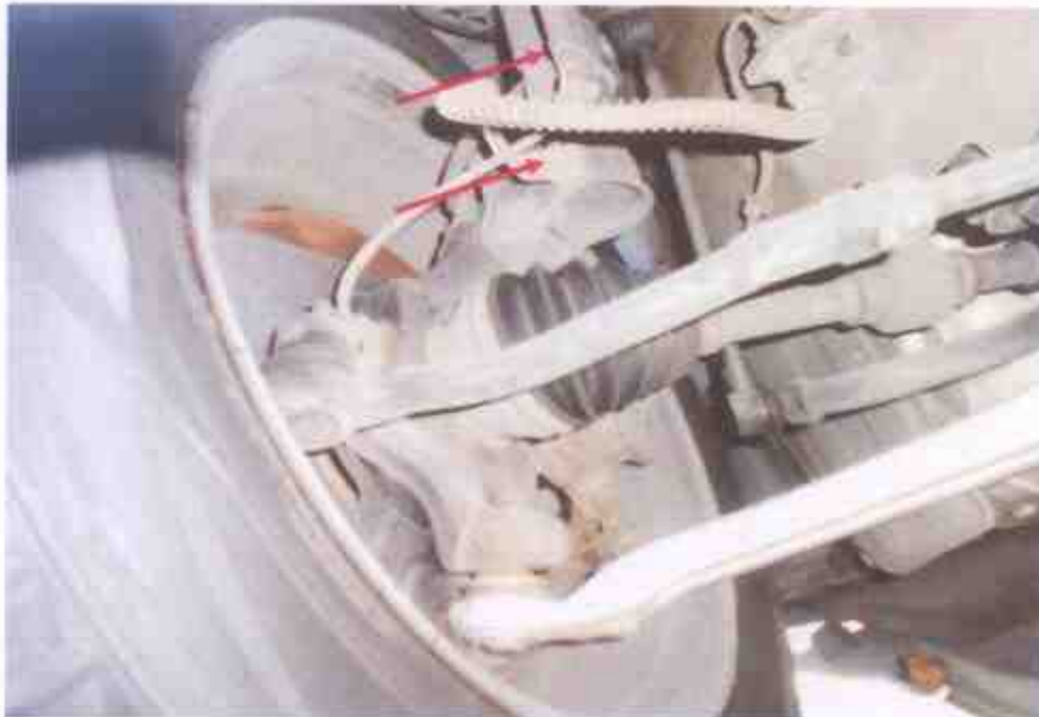
Photo 21 shows the various undercarriage components at the front left wheel of the Motor Taxi. We did not observe any leakage of brake fluid (arrowed) at the time of our inspection of the Motor Taxi. Our visual inspection of the various mechanical components of the Motor Taxi's braking system revealed all to be intact and without visible damage, indicating that the braking system was likely to be in serviceable condition at the material time of accident.
