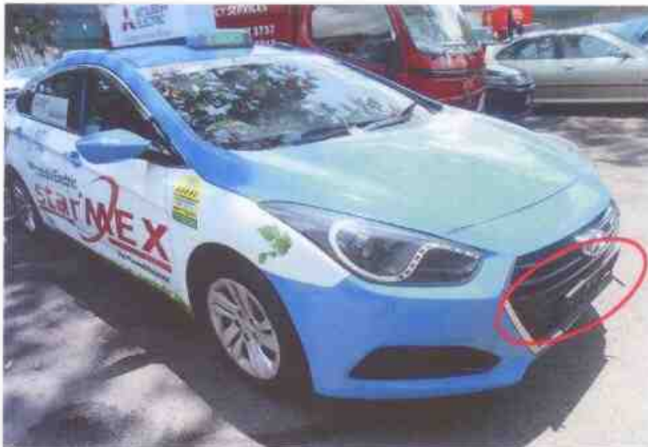
Photo 4 shows a general view of the front right body of the Motor Taxi at the time of our inspection. The Motor Taxi was observed to have sustained a relatively minor impact damages that was confined to its frontal portion.
