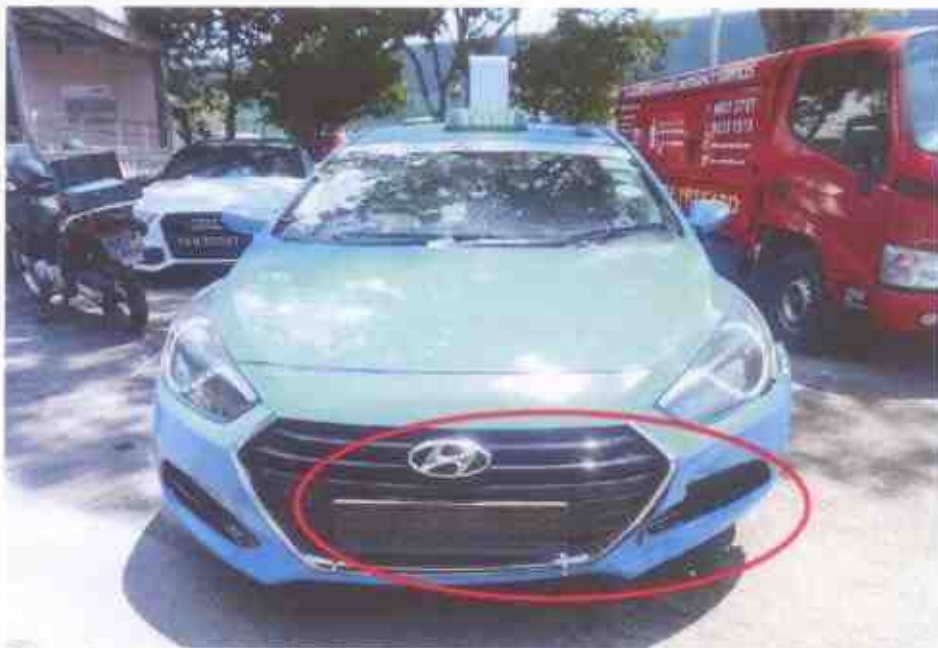
Photo 2 shows a general view of the front body of the Motor Taxi at the time of our inspection. The Motor Taxi was observed to have sustained a relatively minor impact damages that was confined to its frontal left portion. Its front lower bumper was observed to be pushed inwards likely due to the accident's collision impact.
