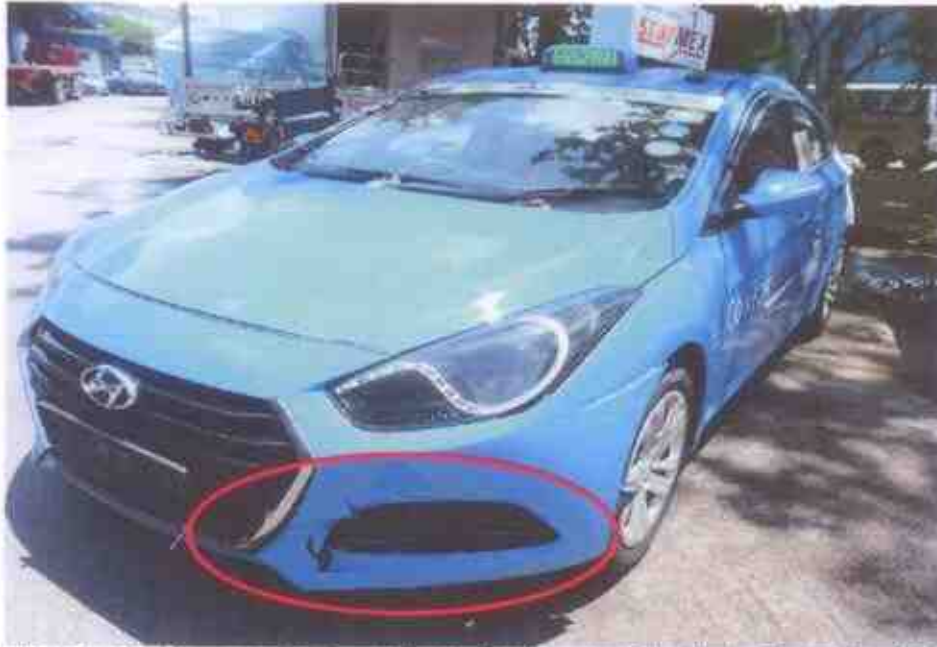
Photo 3 shows a general view of the front left body of the Motor Taxi at the time of our inspection. The Motor Taxi was observed to have sustained a relatively minor impact damages that was confined to its frontal portion.
