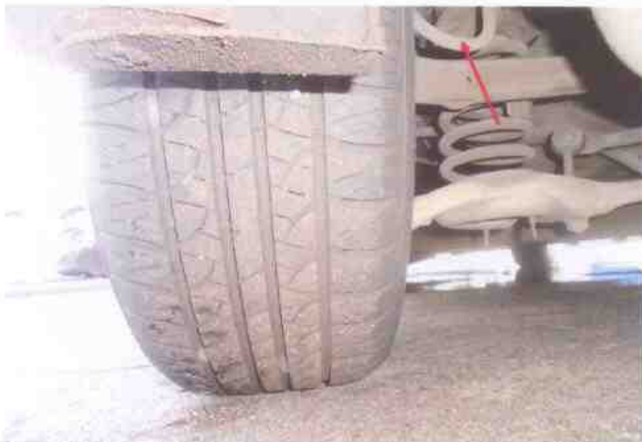
Photo 18 shows the brake hose (arrowed) at the rear left wheel of the Motor Taxi. We did not observe any leakage of brake fluid at the time of our inspection of the Motor Taxi. Our visual inspection of the various mechanical components of the Motor Taxi's braking system revealed all to be intact without visible damage.
