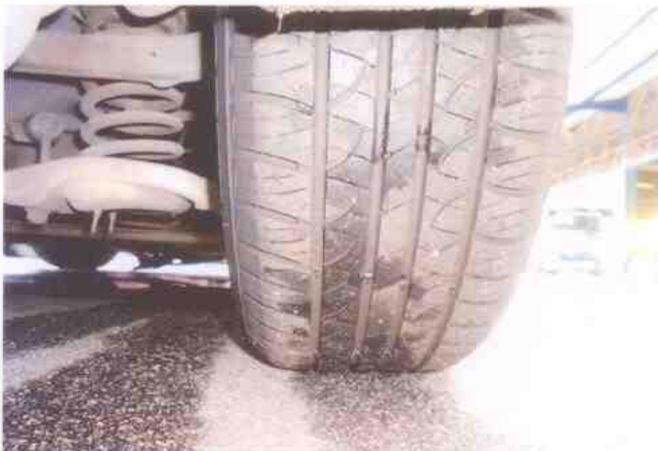
Photo 12 shows the condition of the rear right tyre of the Motor Taxi, which was observed to be in serviceable condition with remaining tread depth of approximately 7mm.
