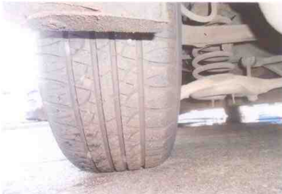
Photo 11 shows the condition of the rear left tyre of the Motor Taxi, which was observed to be in serviceable condition with remaining tread depth of approximately 7mm.
