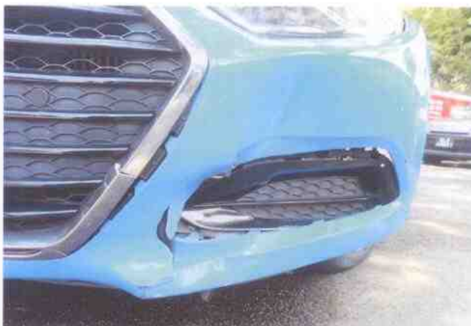
Photo 7 shows a semi close up view of the front left portion of the Motor Taxi at the time of our inspection. The Motor Taxi had sustained relatively minor damages at the front left lower bumper portion likely due to the accident.
