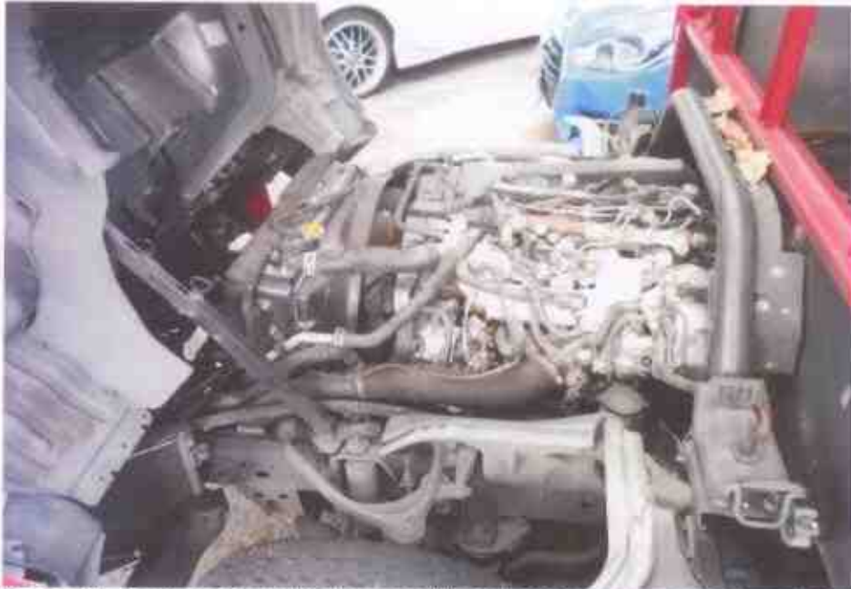
Photo 11 shows a general view of the Motor Lorry's engine compartment. The various parts and components inside the engine compartment were unaffected by the accident. There was also no sign(s) or indication(s) of fluid leakage and/or fluid stain within the engine compartment.
