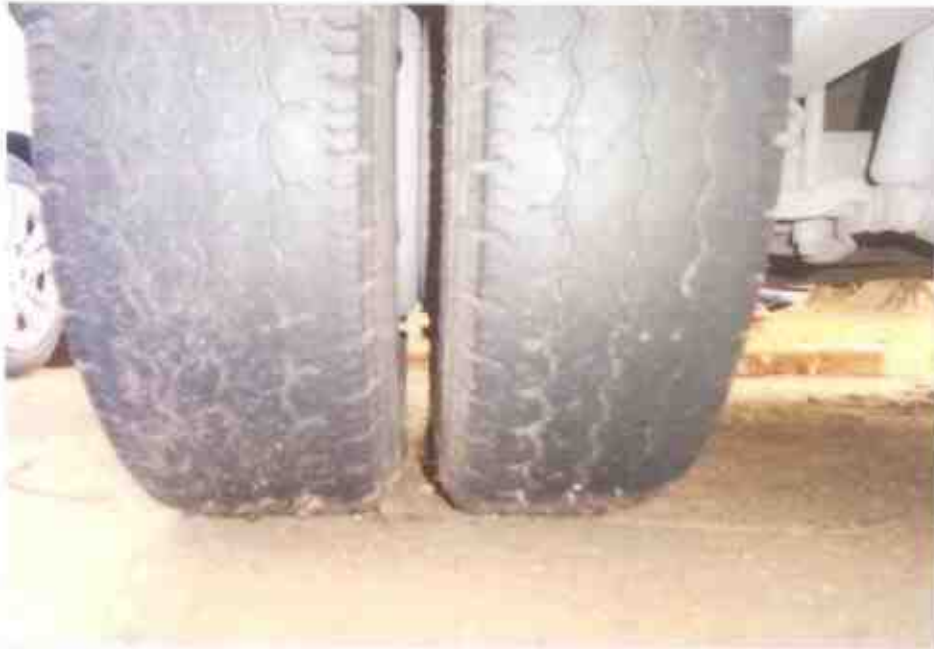
Photo 10 shows the condition of the rear right tyre of the Motor Lorry, which was observed to be in serviceable condition with remaining tread depth of approximately 2mm. There was also no tear, cut or burst mark(s) on the outer and the inner sidewalls as well as across the tread of the tyre, which was also sufficiently inflated for vehicular operation.
