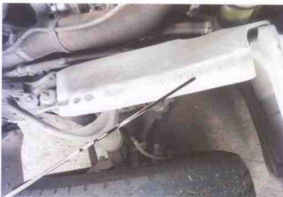
Photo 15 shows the engine dip stick of the Motor Lorry at the time of our inspection. The engine oil was observed to be of sufficient level and without any visible contamination.
