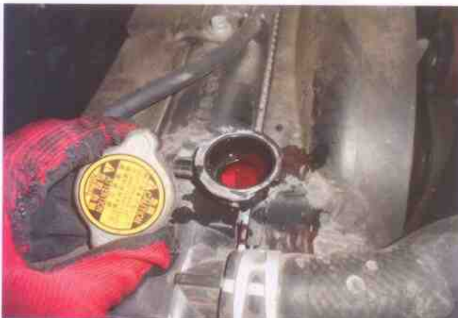
Photo 14 shows the engine coolant reservoir of the Motor Lorry at the time of our inspection. The engine coolant was observed to be of sufficient level and without any visible contamination.
