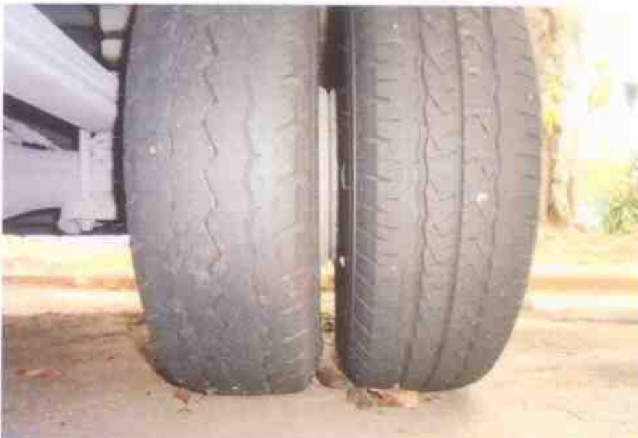
Photo 9 shows the condition of the rear left tyre of the Motor Lorry, which was observed to be in serviceable condition with remaining tread depth of approximately 4mm. The tyre, which was wrapped around standard wheel rim, was also observed to be sufficiently inflated for vehicular operation.
