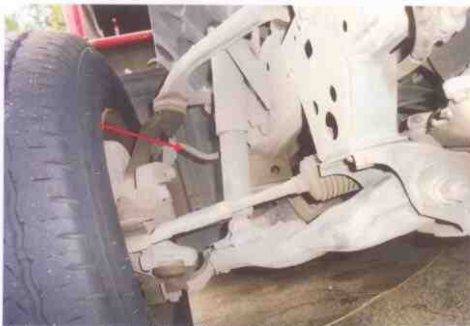
Photo 18 shows the brake hose (arrowed) at the front right wheel of the Motor Lorry. We did not observed any leakage of brake fluid at the time of our inspection of the Motor Lorry. Our visual inspection of the various mechanical components of the Motor Lorry's braking system, including its brake calliper, revealed all to be intact and without visible damage.
