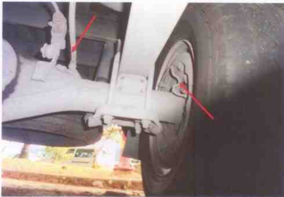
Photo 16 shows the various undercarriage components at the rear left wheel of the Motor Lorry, in particular the brake hose (arrowed). We did not observe any leakage of brake fluid at the time of our inspection of the Motor Lorry.
