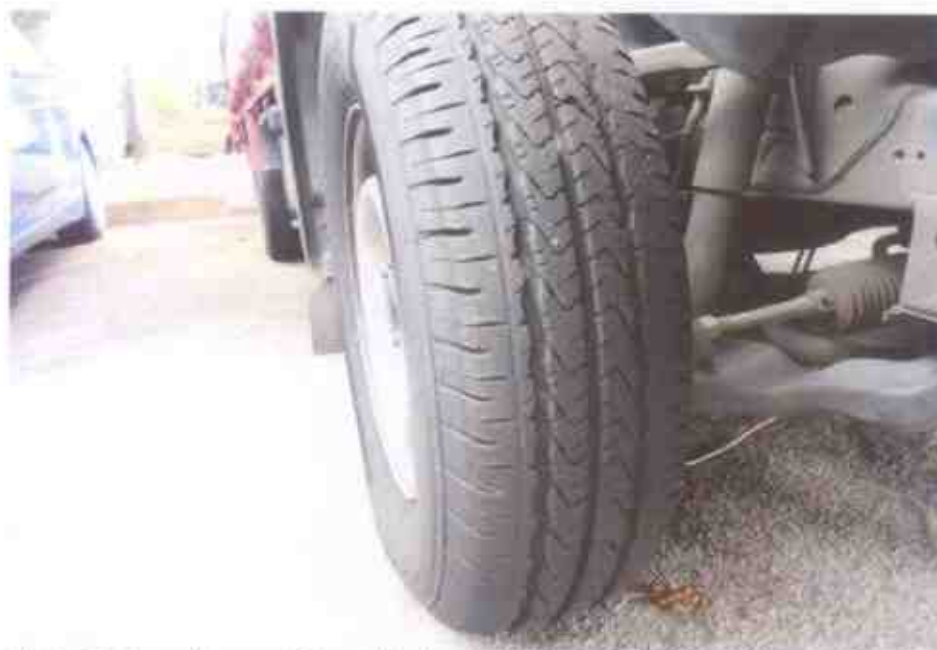
Photo 7 shows the condition of the front right tyre of the Motor Lorry, which was observed to be in serviceable condition with remaining tread depth of approximately 7mm.
