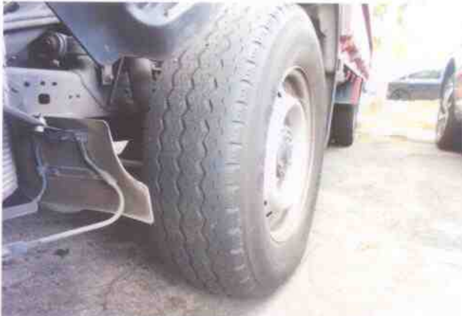
Photo 8 shows the condition of the front left tyre of the Motor Lorry, which was observed to be in serviceable condition with remaining tread depth of approximately 5mm. The tyre, which was wrapped around standard wheel rim, was also observed to be sufficiently inflated for vehicular operation.
