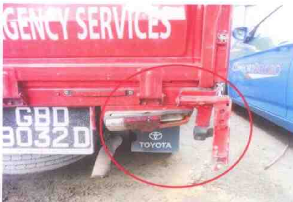
Photo 3 shows the damages to the rear right tail lamp & lock bracket as a result of the accident.
