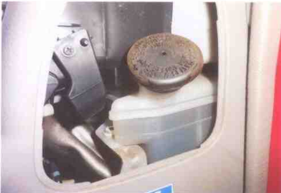
Photo 12 shows the brake fluid reservoir of the Motor Lorry at the time of our inspection. The brake fluid was observed to be of sufficient level and without any visible contamination.
