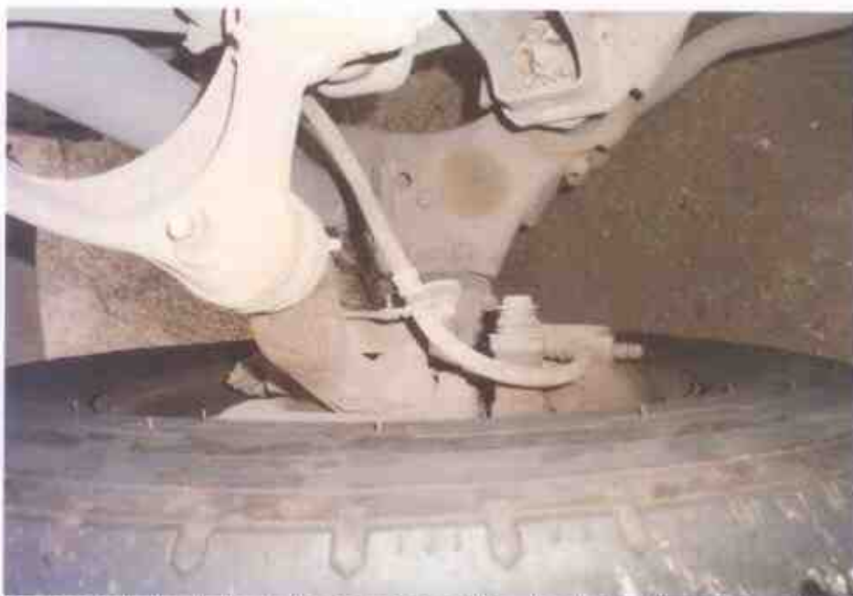
Photo 17 shows the brake hose at the front left wheel of the Motor Lorry. We did not observe any leakage of brake fluid. Our visual inspection of the various mechanical components of the Motor Lorry's braking system revealed all to be intact and without visible damage, indicating that the braking system was likely to be in serviceable condition at the material time of accident.
