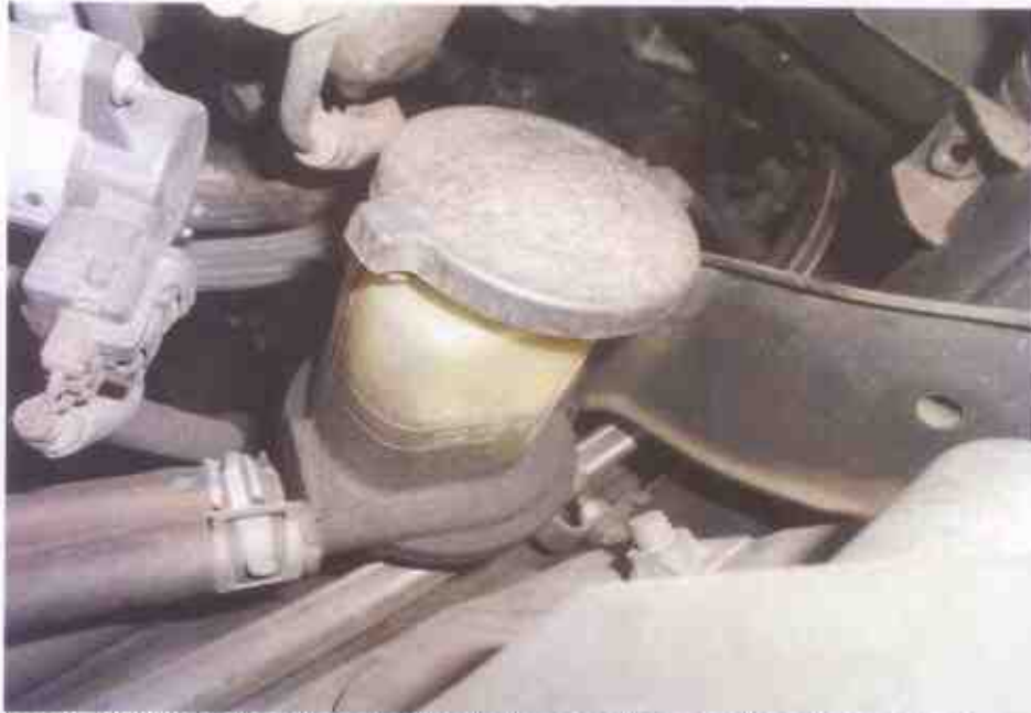
Photo 13 shows the power steering fluid reservoir of the Motor Lorry at the time of our inspection. The power steering fluid was observed to be of sufficient level and without any visible contamination.
