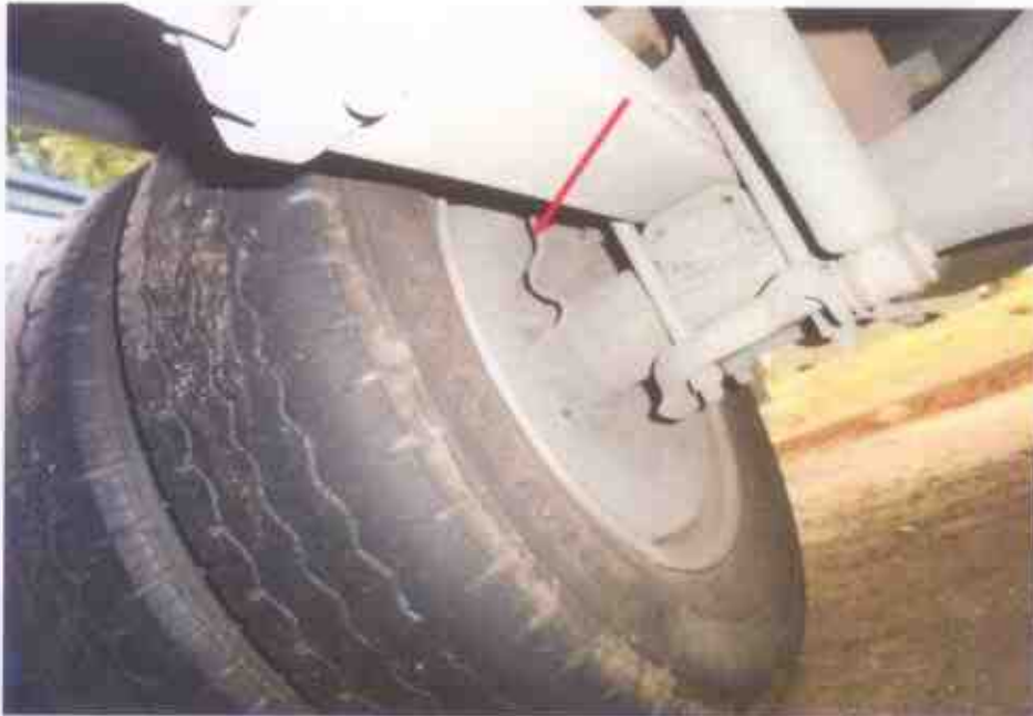
Photo 19 shows the various undercarriage components at the rear right wheel of the Motor Lorry. The various steering components were all found to be intact, suggesting that the steering system of the Motor Lorry was likely to be in serviceable condition at the material time of accident.
