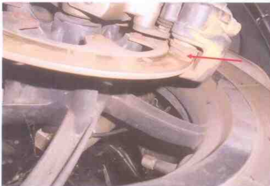
Photo 18 shows the front brake pad of the front wheel was noted to be of sufficient frictional material for operational purposes.
