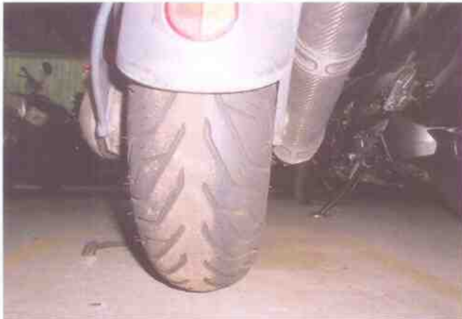
Photo 9 shows the rear tyre of the Motorcycle. The rear tyre was observed to be in serviceable condition with remaining tread depth of approximately 4mm. The tyre was also observed to be sufficiently inflated for vehicular operation.
