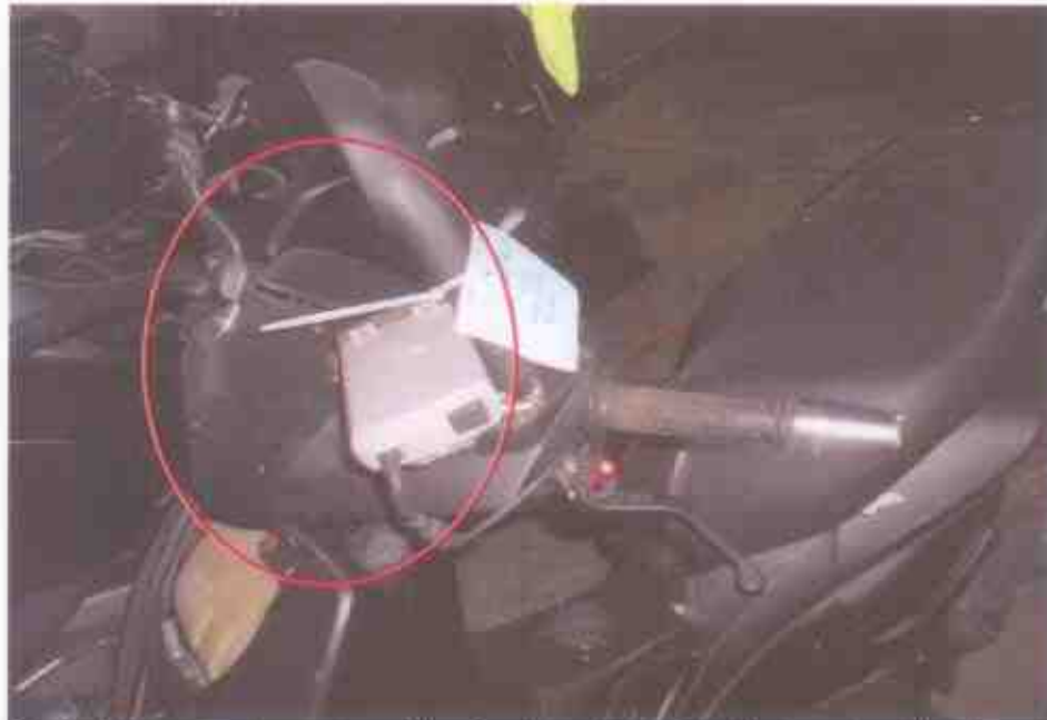
Photo 5 shows a closer view of the frontal portion of the Motorcycle at the time of our inspection. The Motorcycle was observed to have sustained broken front top fairing due to the accident collision. (Circled)
