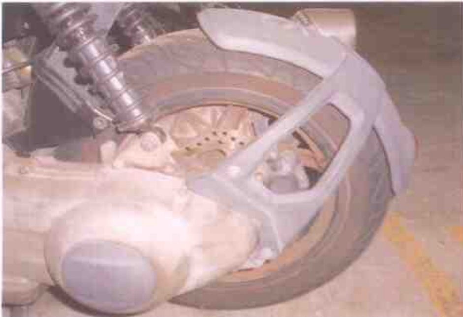
Photo 13 shows the drive train of the motorcycle was found to be intact without any misalignment.
