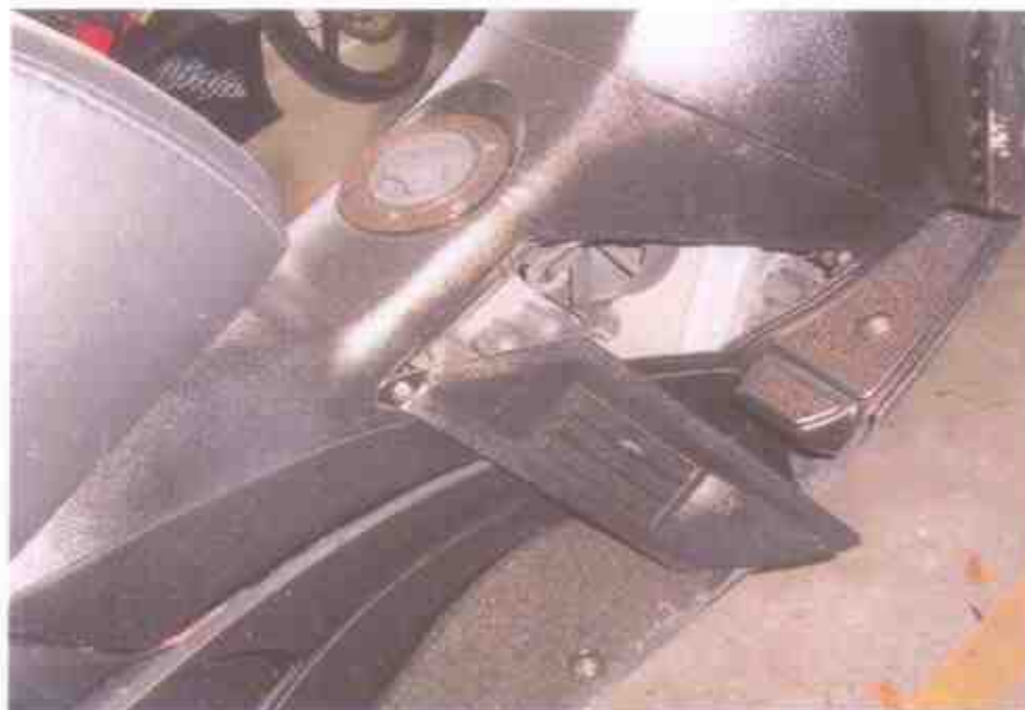
Photo 7 shows a closer view of the right side engine cover of the Motorcycle at the time of our inspection. It was observed to have sustained damages due to the accident collision. (Circled)
