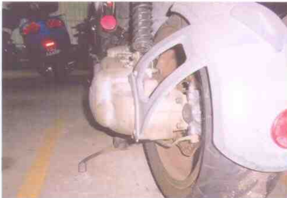
Photo 14 shows the drive train of the motorcycle was found to be intact without any misalignment.
