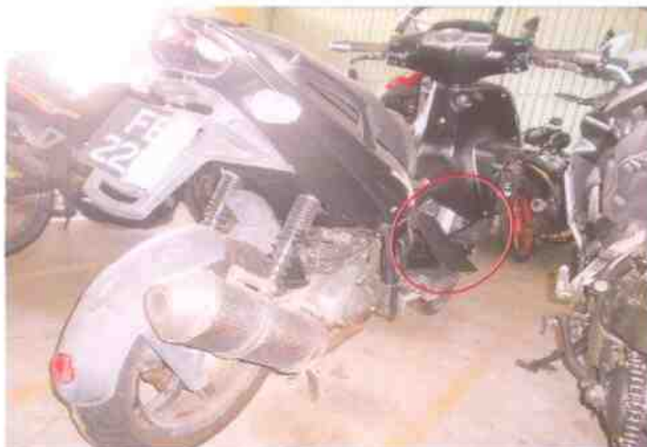
Photo 3 shows a general view of the right body of the Motorcycle at the time of our inspection. The Motorcycle was observed to have sustained minor damages at the frontal portion, along its right side. (Circled)
