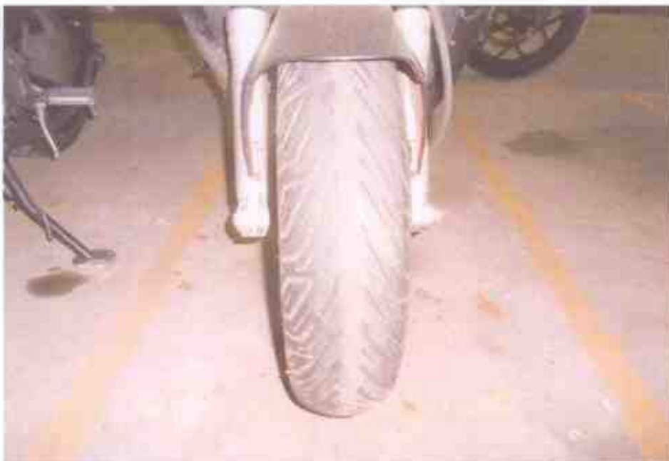
Photo 10 shows the front tyre of the Motorcycle. The pattern of the tread was clearly visible. There was no tear, burst mark(s) and/or punctured hole(s) on the sidewalls as well as across the tread of the front tyre.
