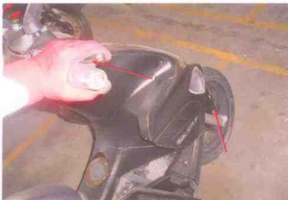
Photo 15 shows the front brake static test. Static braking test was conducted to the front braking system & found to be in serviceable condition.
